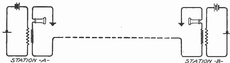
Fig. 125. Local-Battery Stations with Grounded Circuit
