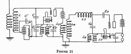
shows the complete circuits for carrying out this method of reception. Here  $C_1L_1L_2C_2$  is an audio frequency system designed to produce audio frequency oscillations; and P is a potentiometer for adjusting the potential of the grid so that on the negative part of the oscillation in the wing circuit, the wing current is reduced practically to zero. The radio frequency
