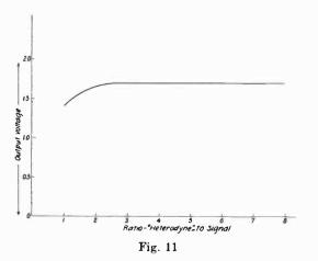
linearity characteristic of the rectifier is shown in Fig. 11 where the voltage produced by the beats between a current of constant amplitude and one whose amplitude is raised from equality with, to many times the value of, the first current is plotted against the ratio of the two. The linearity of the rectifier is such that after the ratio of the current becomes two to one no further increase in rectifier output voltage results. In fact with the levels used in these measurements when the
