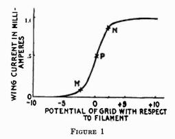
from it we see that a positive charge placed on the grid produces an increase in the wing current, and that a negative charge placed on the grid produces a decrease in the wing current. When the audion is used as an amplifier, and an alternating e. m. f. is impressed between the grid and the filament, the continuous current of the wing circuit will be varied in accordance
