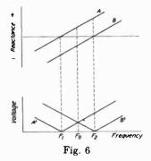
these characteristics may be rendered sufficiently straight within the working range to meet the severest requirements of high fidelity broadcasting. The operation of the system is aperiodic and capable of effecting 100 per cent modulation if desired, this last depending on the separation of the two nonreactive points with respect to the frequency swing. Generally the setting of the nonreactive frequency points should be somewhat beyond the range through which the frequency is swung.
