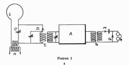
usual tuned receiving circuit, loop or otherwise, H a separate heterodyne, and  $D_1$  a rectifier. A is a radio frequency amplifier designed to operate on some pre-determined frequency. This frequency may be any convenient frequency which is substantially above audibility. The amplifier is connected on its input side to the rectifier  $D_1$ , and on its output side to a second rectifier  $D_2$  and a telephone or other receiver.
