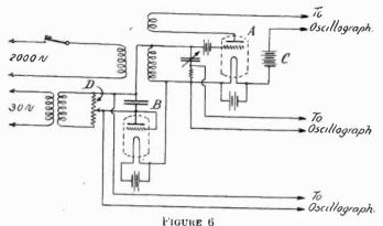
A-4 Western Electric Type L Tubes in parallel B-1 Western Electric Type L Tubes with grid and plate in parallel C-DC Voltage = 160 Volts D-AC Voltage = 30 Volts
