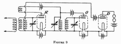
introduced into the positive resistance of the tuned circuit. This is done by means of an oscillating tube O, the grid circuit of which is connected thru the tuned circuit LC of the amplifying tube R. The variation in the resistance of the circuit is effected thru the variation in potential of the grid of the oscillating tube. During that half of the cycle, when the grid of the oscillating tube is positive, energy is withdrawn from the tuned circuit in
