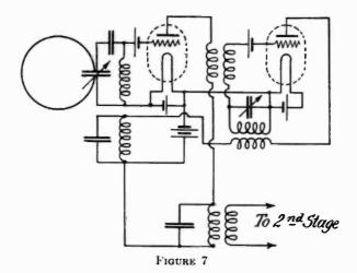
On account of the high amplification, signals from local stations overload the second rectifier and introduce distortion. Control of the amount of intermediate frequency amplification is essential. While there are numerous methods equally effective, the simplest one appears to be the control by means of the filament temperature of the second intermediate frequency amplifier.<sup>6</sup>
