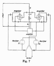
point the combination acts as an inductance; at frequencies below the nonreactive point as a capacity and the phase of the voltage developed across the combination with respect to the current through it
