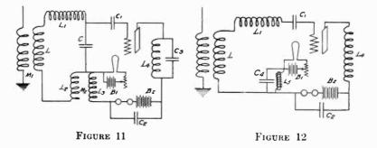
lustrated in Figure 11. Other methods of coupling may be employed between the grid and wing circuits, electrostatic and direct magnetic couplings being illustrated in Figures 12 and 13. The arrangement of Figure 13 operates in the same way as the system with the two coil coupling; but the electrostatic coupling
