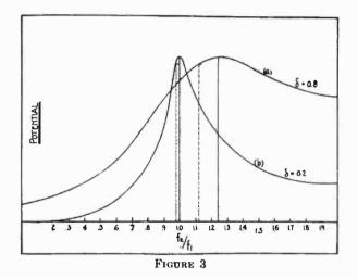
curve "b" corresponding to a decrement of 0.2 represents about as sharp tuning as can be used, and even then it is necessary to use the higher range of available heterodyne frequencies. It is to be noted that this tuning is by no means sharp as judged by the standards usually set for radio circuits.
