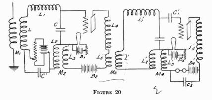
set up oscillations in the second system by means of the coupling  $M_3$  (See Figure 20). The oscillations initially set up in the second system are again amplified, and then rectified in the second audion to produce audible response in the telephones.
