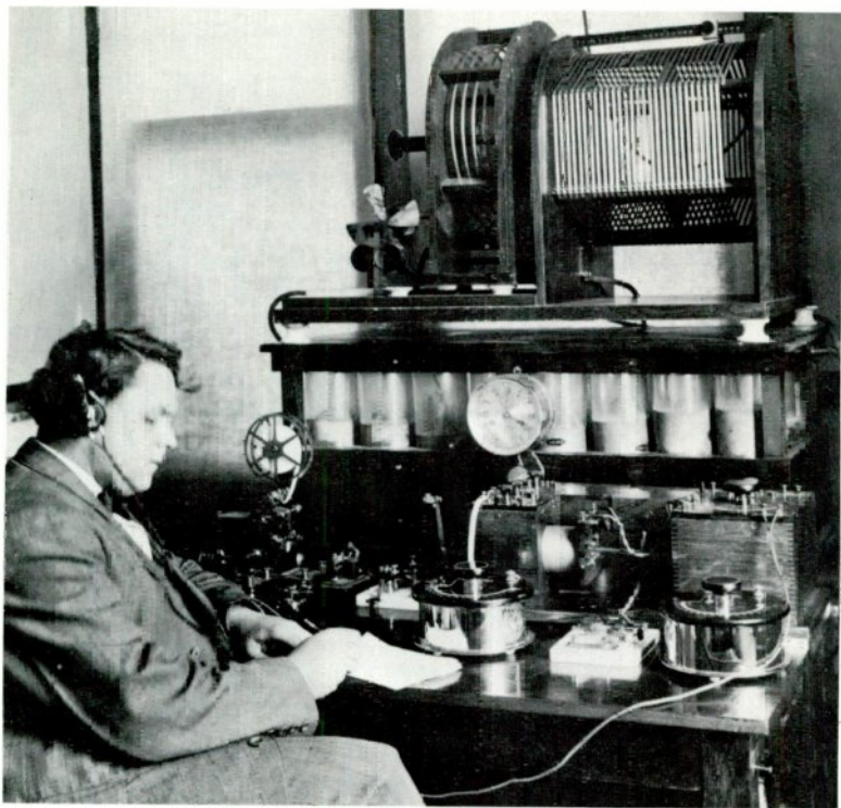
Earle Ennis at his wireless telegraph station in San Francisco's Grant Building, about 1910, the year he installed equipment on an airplane and received the first air-to-ground wireless message.
