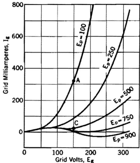
FIG. 52. Grid current curves for an RCA Type 203-A (transmitter-type) triode.
