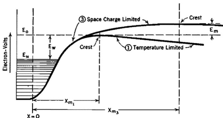
FIG. 78. Valve action at emitter surface; potential-energy details as related to work function. Compare with Fig. 77.
