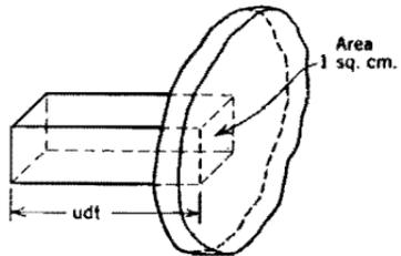
FIG. 93. Rate of arrival at a wall of particles with velocity  $u$ .
