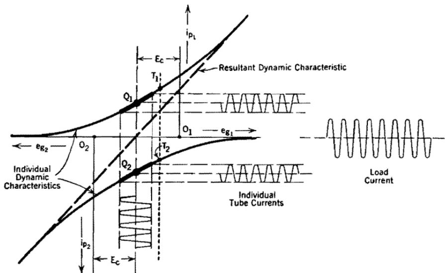
FIG. 121. Dynamic characteristics for push-pull Class A amplifier operation.
