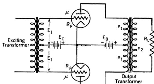
FIG. 119. Push-pull amplifier circuit.
