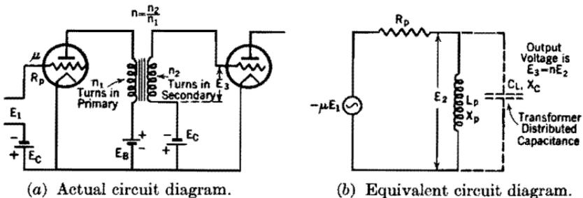
FIG. 127. Transformer-coupled amplifier with infinite load impedance. Transformer turn ratio =  $n = n_2/n_1$ .
