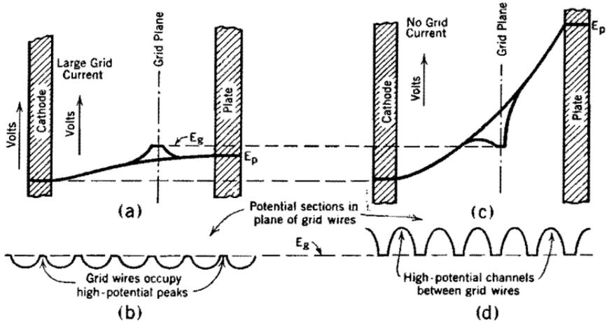
FIG. 51. Space-charge-flow potential distribution in a triode with positive grid, indicating manner of diversion of current from positive grid to plate, at high plate voltages. Plate voltage is low in (a) and (b), high in (c) and (d). See also Fig. 52.
