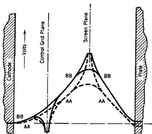
FIG. 58. Space-charge shielding of screen wires.
