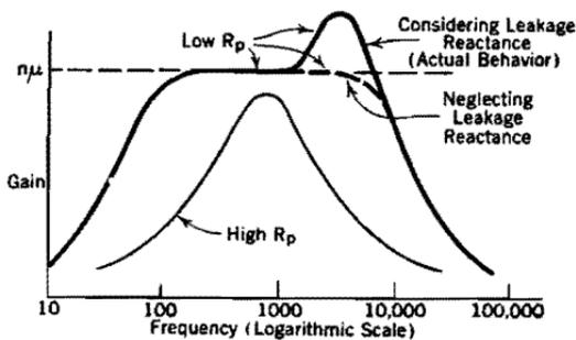
FIG. 129. Frequency response of a transformer-coupled amplifier with infinite load resistance, illustrating the effect of leakage reactance.
