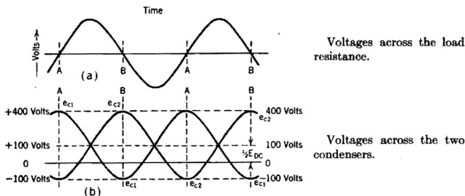
FIG. 200. Voltage wave forms in the series inverter circuit of Fig. 199 when natural frequency of inverter and load is the same as the grid excitation frequency. At the moment *A*, tube No. 1 lights, tube No. 2 goes out. At the moment *B*, the reverse happens.
