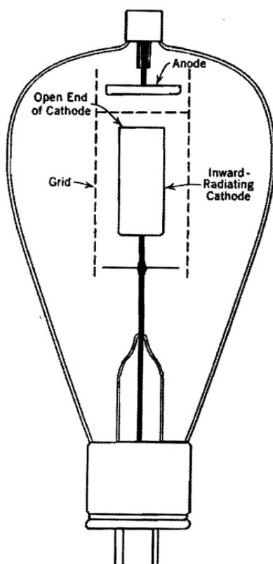
FIG. 175. Typical electrode arrangement in a thyatron.
