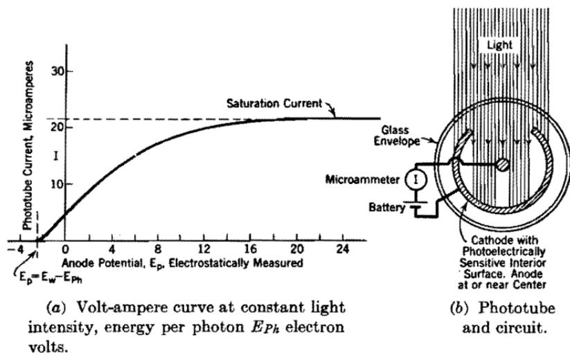
FIG. 151. Central anode vacuum-type phototube with cylindrical cathode.
