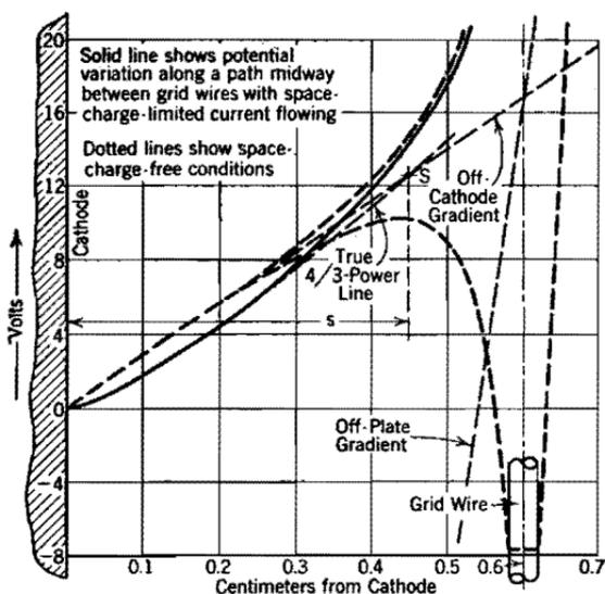
FIG. 44. Space-charge-flow potential distribution in a parallel-plane triode.
