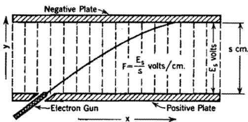
FIG. 27. Electron trajectory in a uniform electric field.
