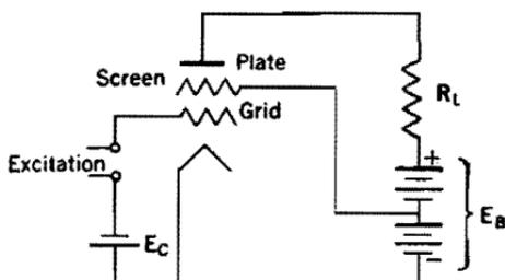
(c) Screen-grid amplifier circuit.
