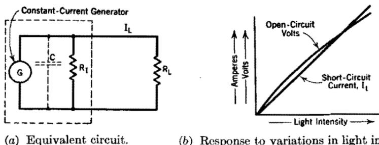
FIG. 163. Rectifier-type photocell properties.
