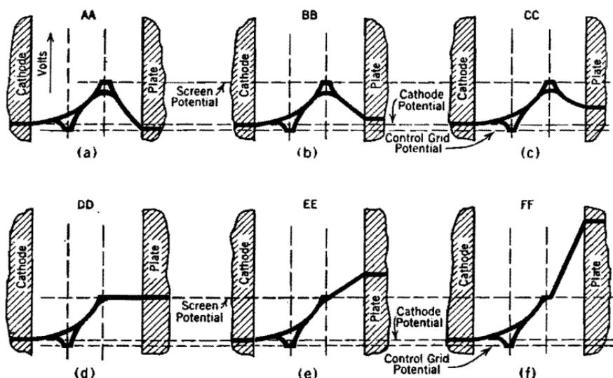
FIG. 57. Space-charge-free potential distributions in screen-grid tube, corresponding to potentials as at A-A, B-B, — F-F, in Fig. 56.
