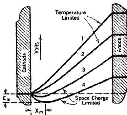
FIG. 77. Potential distribution curves illustrating valve action at emitter surface when current is space-charge-limited.
