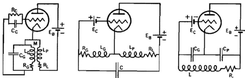
(a) Tuned grid oscillator. (b) Hartley oscillator. (c) Colpitt oscillator.
