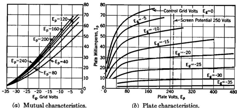
FIG. 60. Average characteristic curves, RCA Type 59 tube, pentode connection, with screen at 250 volts.
