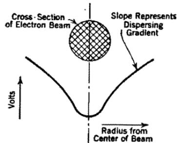
FIG. 38. Potential variation within and near an electron beam, due to the beam's own space charge.
