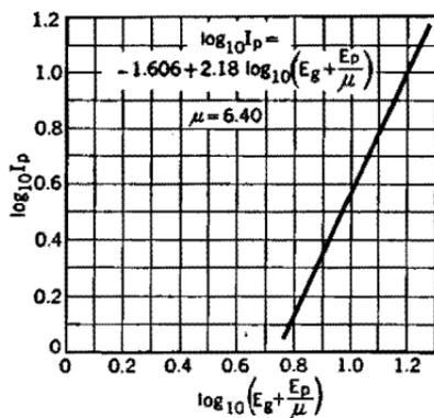
FIG. 49b. Logarithmic relation between plate current and equivalent voltage, Western Electric type 101-F triode. The straight line shown here is a logarithmic graph of the curve shown in Fig. 49a.
