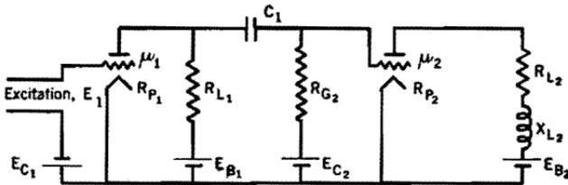
FIG. B. Two-stage amplifier.
