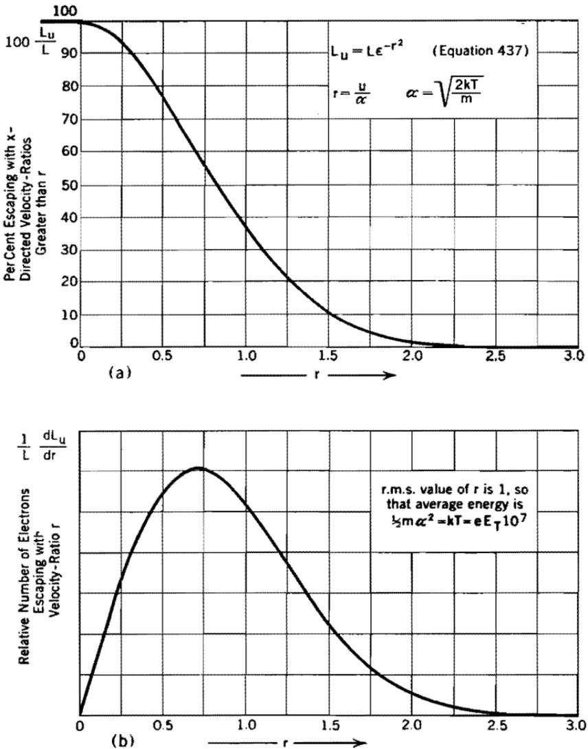
FIG. 94. Time-exposure-over-a-surface velocity distribution of thermionically-emitted electrons, also of Maxwellian gas particles striking a boundary.
