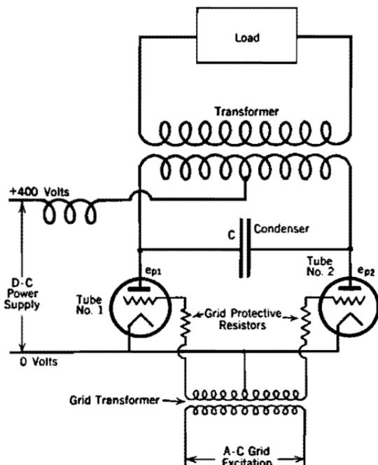
FIG. 196. Typical parallel-type inverter circuit employing thyratrons.
