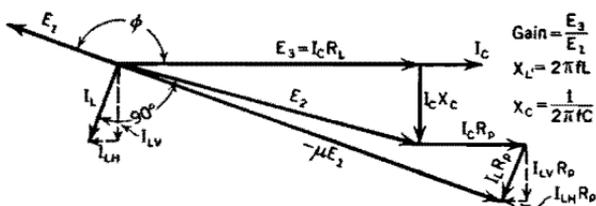
(c) Vector diagram for complete equivalent circuit. Within the normal frequency range the vectors  $E_2$ ,  $E_3$ ,  $-uE_1$ ,  $E_1$ , all lie along a common line, and  $E_3 \equiv E_2$ . Then  $\phi = 180^\circ$ .
