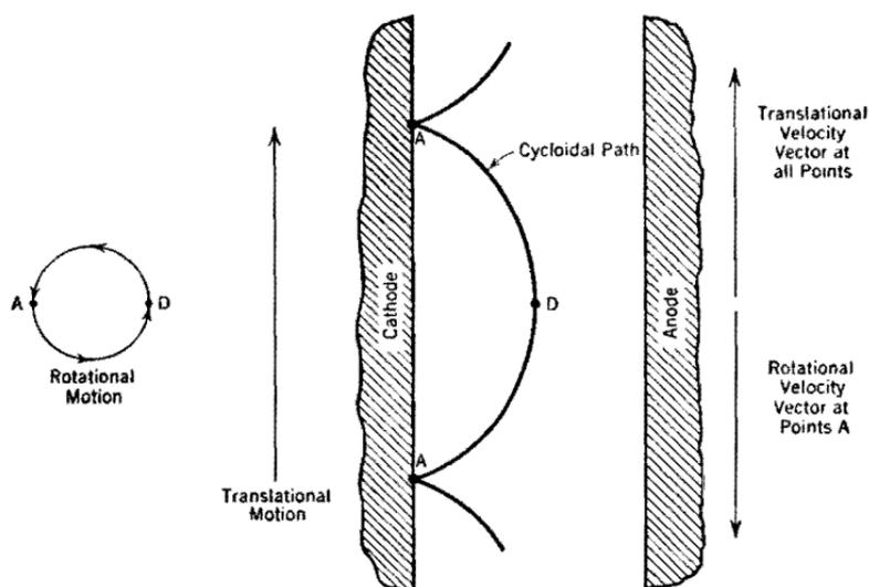
FIG. 31. Cycloidal path of an electron in uniform electric and magnetic fields; zero initial velocity.
