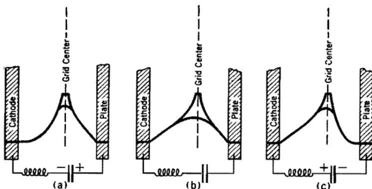
FIG. 62. Coupling between oscillating space charge and external circuit.
