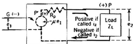
(c) *Equivalent circuit used for predicting electronic amplifier behavior.* To make  $P$  momentarily positive as shown, the alternating load current must flow in the direction indicated by the arrow. This is the *negative* direction for  $i_z$ , the *positive* direction for  $i_z$ . When  $P$  is positive,  $P'$  is still more positive, as in (b), but  $G$  is negative, as in (a). Thus when  $e_2$  and  $i_z$  have positive values,  $e_1$  has a negative value.
