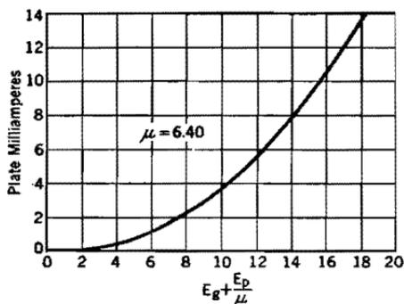
FIG. 49a. Dependence of triode plate current on equivalent voltage, Western Electric type 101-F triode. The curve in this figure represents any of those in Fig. 3b.
