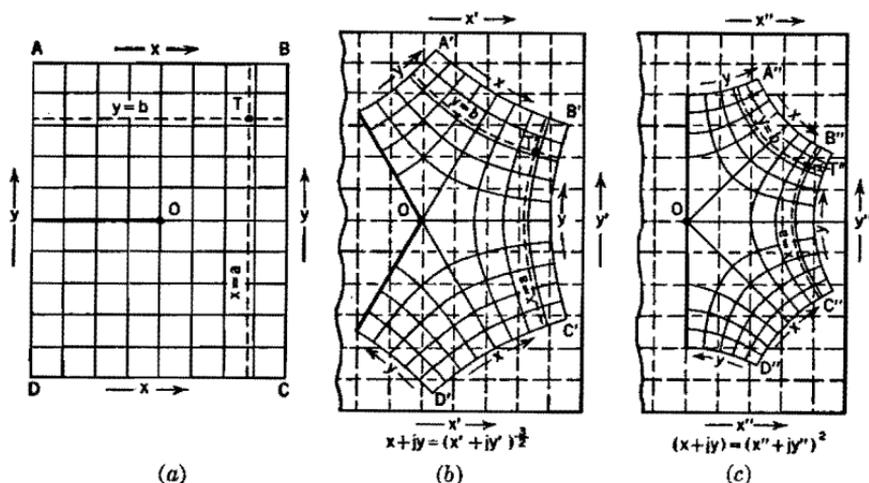
FIG. 11. Conformal transformation of a rectangular sheet marked with rectangular coordinates.
