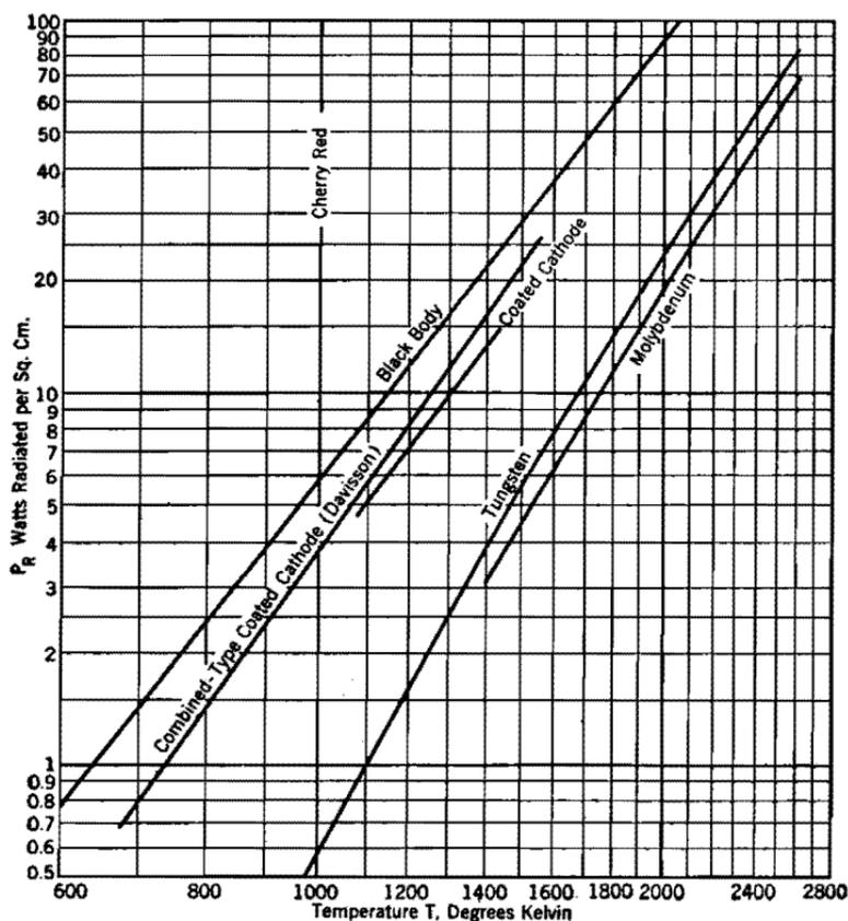
FIG. 67. Radiation from thermionic surfaces.
