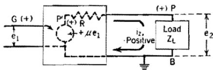
(b) *Ideal amplifier.* To make  $P$  momentarily positive as shown, the alternating load current  $i_z$  flows in the direction indicated by the arrow. This is the *positive* direction for  $i_z$ . When  $P$  is positive,  $P'$  and  $G$  are also positive. No such amplifier as this exists; however, the polarities here shown are the same as in alternating-current transformer circuit diagrams as usually drawn.
