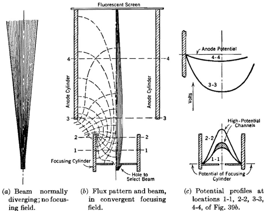
FIG. 39. Electrostatic focusing of a cathode-ray oscillograph beam.
