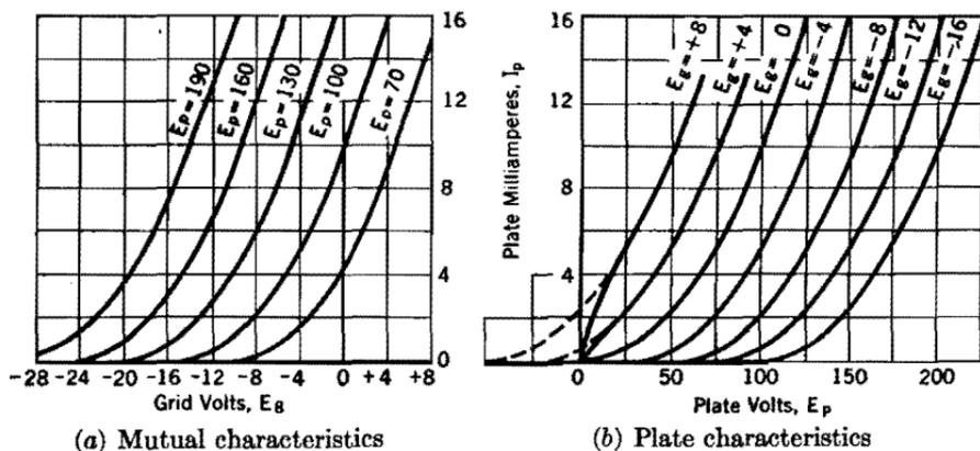
FIG. 3. Average characteristic curves for a triode (Western Electric type 101-F).
