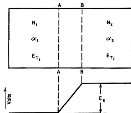
FIG. 97. Equilibrium between electron gases at different potentials.
