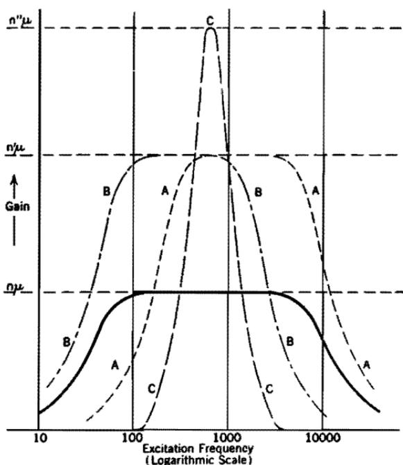
FIG. 128. The heavy solid line illustrates the variation of gain with frequency in a transformer-coupled amplifier with infinite load resistance, turn ratio  $n$ , no leakage reactance. The effects of changes in turn ratio on frequency response are illustrated as follows:
