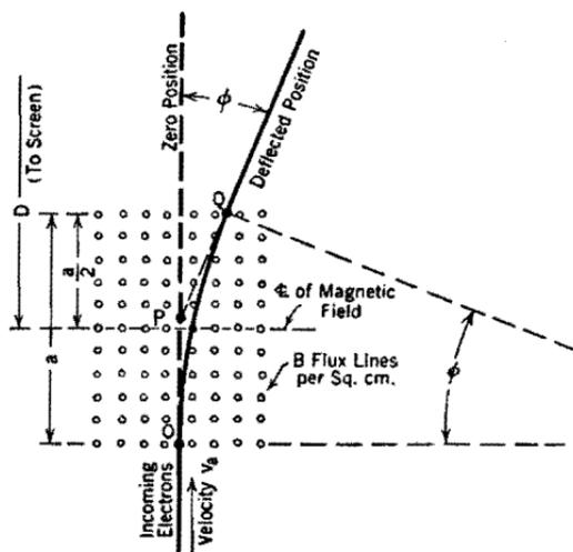
FIG. 37. Magnetic deflection of a cathode-ray oscillograph beam.
