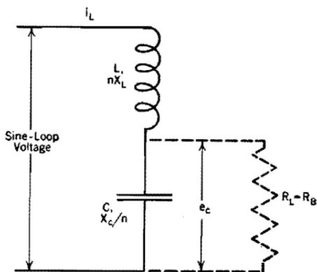
FIG. 190. Circuit diagram for use in analyzing circuit behavior at [point *B*, Fig. 188, for the circuit of Fig. 185.  $R_B$  is shown dotted because the alternating current [through it is neglected in the circuit analysis.
