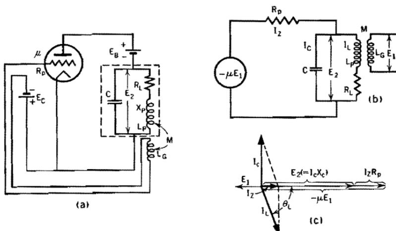
(a) Circuit diagram. The dotted line encloses the "tank circuit." Polarity is correct if  $L_P$  and  $L_G$  are separated sections of a continuously wound coil.
