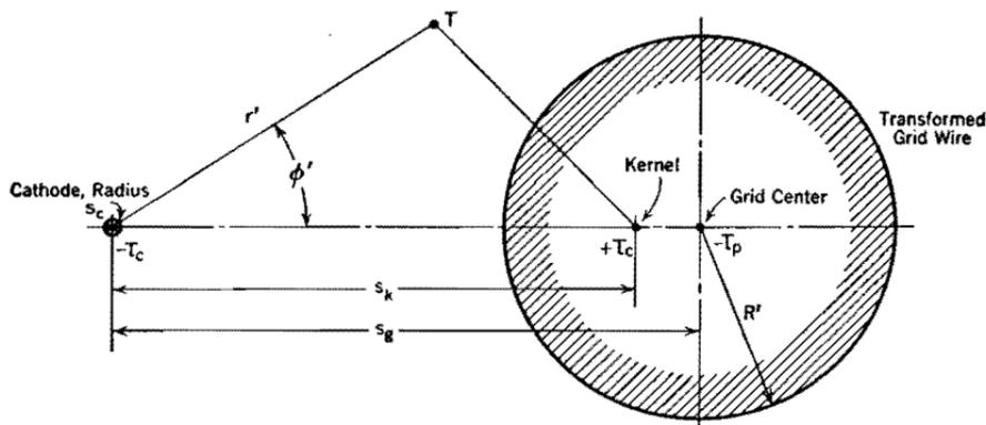
FIG. 19. Detail of placement of Z-plane charges in Fig. 15. Plate circle remote with center at cathode.
