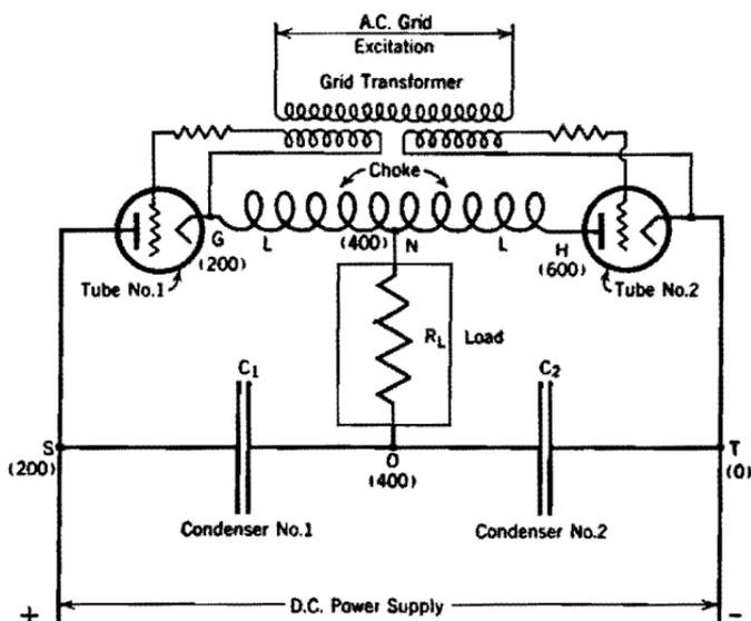
FIG. 199. Typical series-type inverter employing thyratrons.
