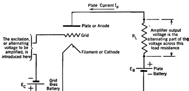
FIG. 1. Triode connections in an amplifier circuit.
