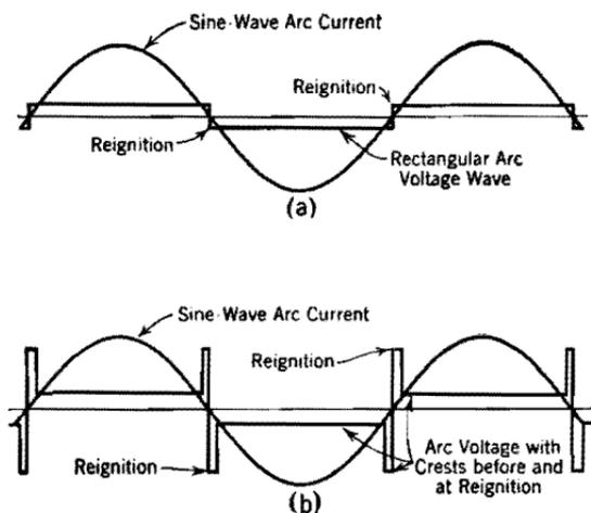
FIG. 168. Wave forms of voltage and current in alternating-current arcs.
