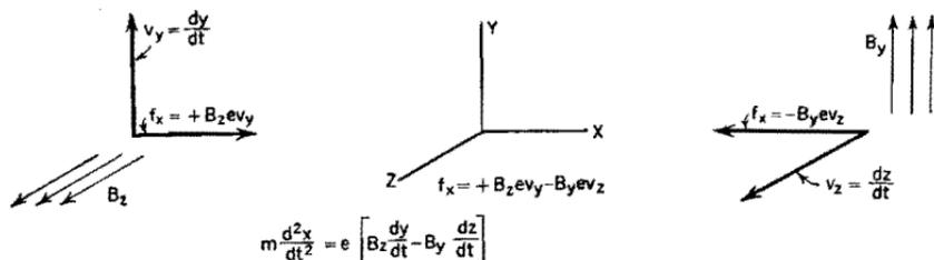
FIG. 35. Components of force on an electron in a curved magnetic field.
