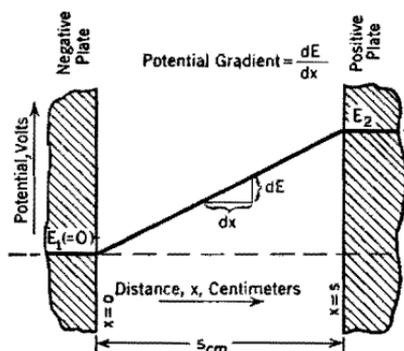
FIG. 5a. Potential distribution between two parallel metal surfaces.
