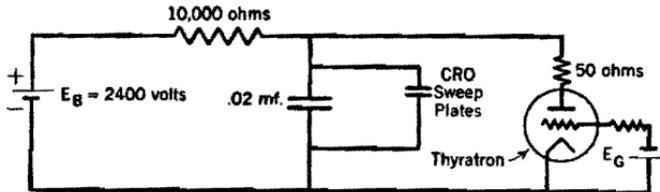
FIG. *F*. Sweep circuit for cathode-ray oscillograph.
