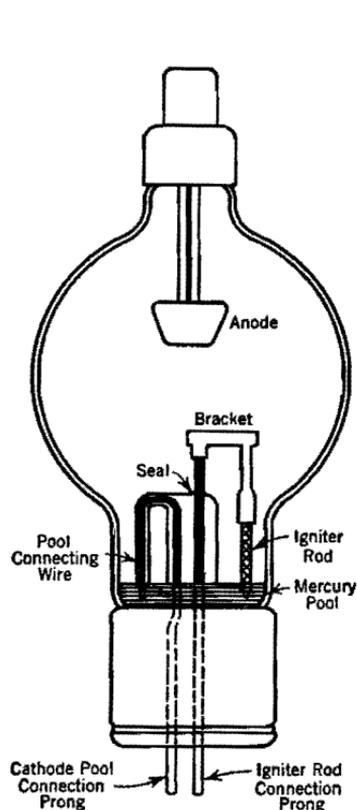
FIG. 174. Electrode arrangement in a Westinghouse Type KU-637 ignitron.
