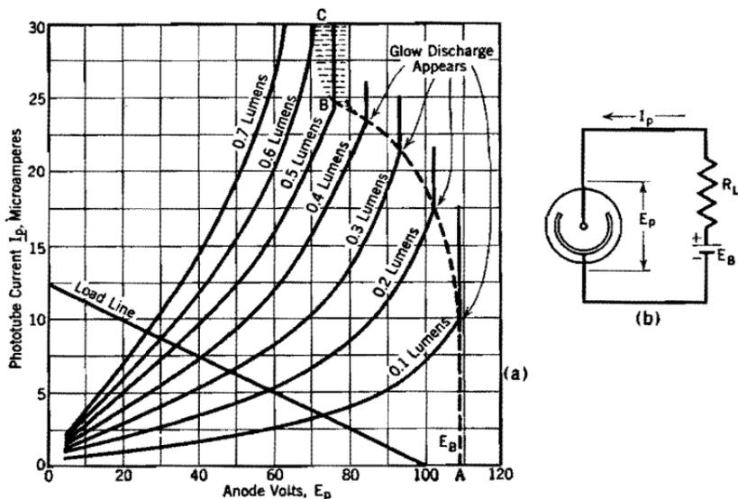
FIG. 158. Volt-ampere characteristic curves for a gas-filled phototube, for various intensities of illumination; also, load line corresponding to a simple direct-current circuit.
