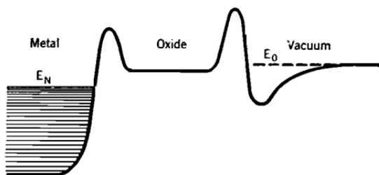
FIG. 84. Potential-energy variation through an oxide-coated surface.
