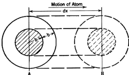
FIG. 98. Increment  $dx$  of an atom's free path. Volume swept out in distance  $dx$  by imaginary sphere of radius  $2b$  is  $\pi(2b)^2 dx$ . Chance of collision therein is  $N\pi(2b)^2 dx$ .
