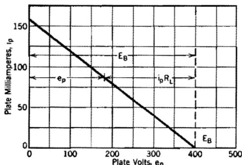
FIG. 103. Load line, for the circuit of Fig. 102, when  $E_B = 400$ ,  $R_L = 2,500$ .
