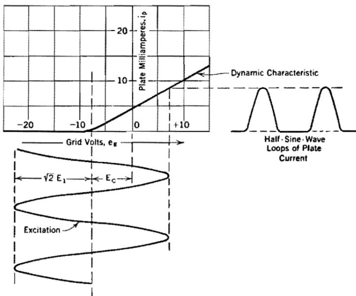
FIG. 118. Class B amplifier operation. Grid is biased to cut-off.
