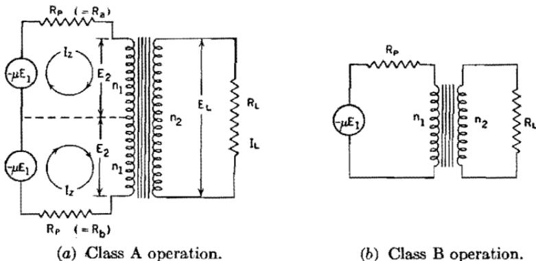
FIG. 122. Equivalent circuit diagrams for push-pull amplifiers.
