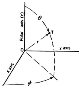
FIG. 9. Spherical coordinates of the point  $T$ .
