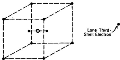
FIG. 68. Locations of the eleven electrons of a sodium atom's "atmosphere."
