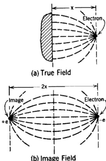
FIG. 72. The electric field around an escaping electron.
