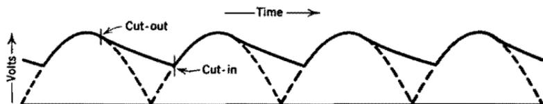
FIG. 187. Load and condenser voltage, for a rectifier using a filter consisting of condenser only. Circuit as in Fig. 185 except that choke is omitted. Dotted lines follow the sine-loop voltage,  $f = 60$  cycles,  $R_L = 2,000$  ohms,  $C = 4$  microfarads,  $R_B = \infty$ .
