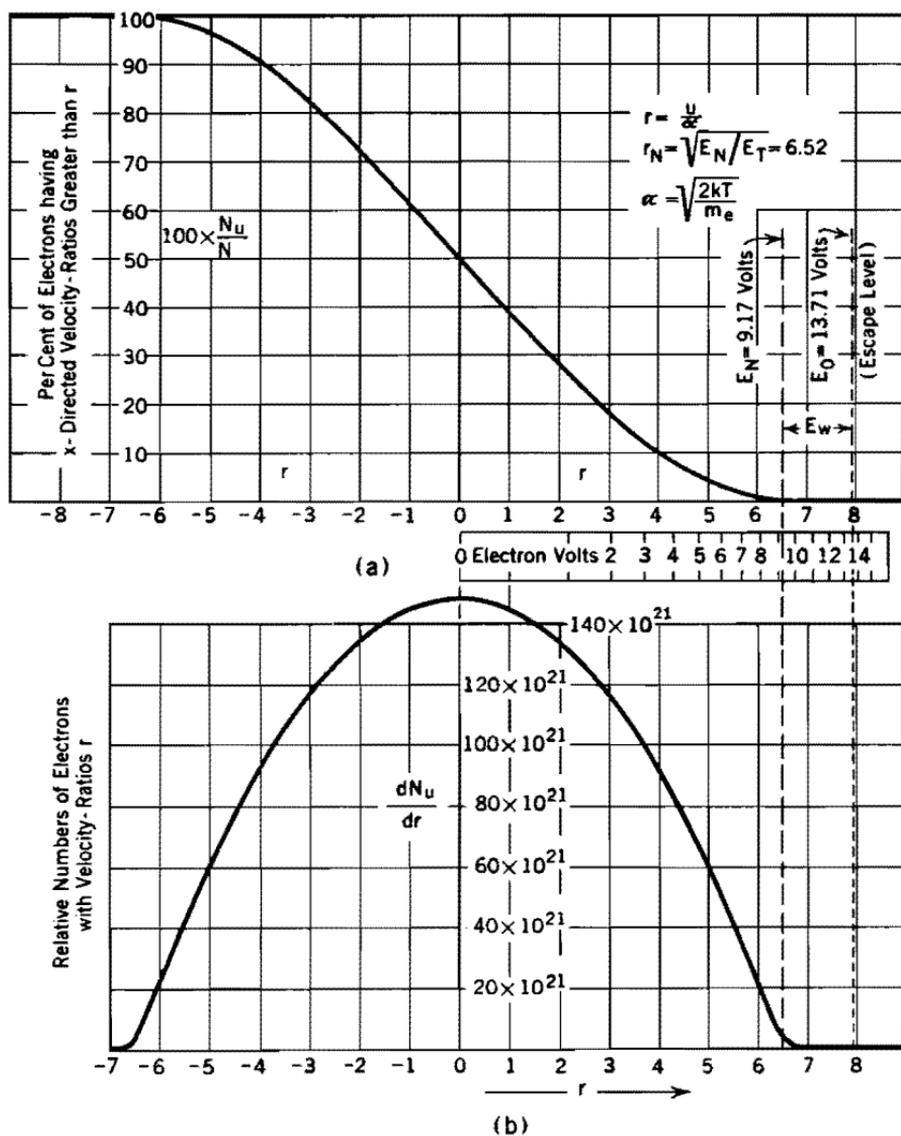
FIG. 92.  $x$ -directed velocity distributions among electrons in tungsten at  $2500^\circ \text{K}$ , two electrons per atom.
