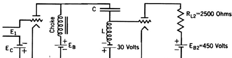
FIG. C. Two-stage tuned amplifier employing a series resonant circuit in the first stage.
