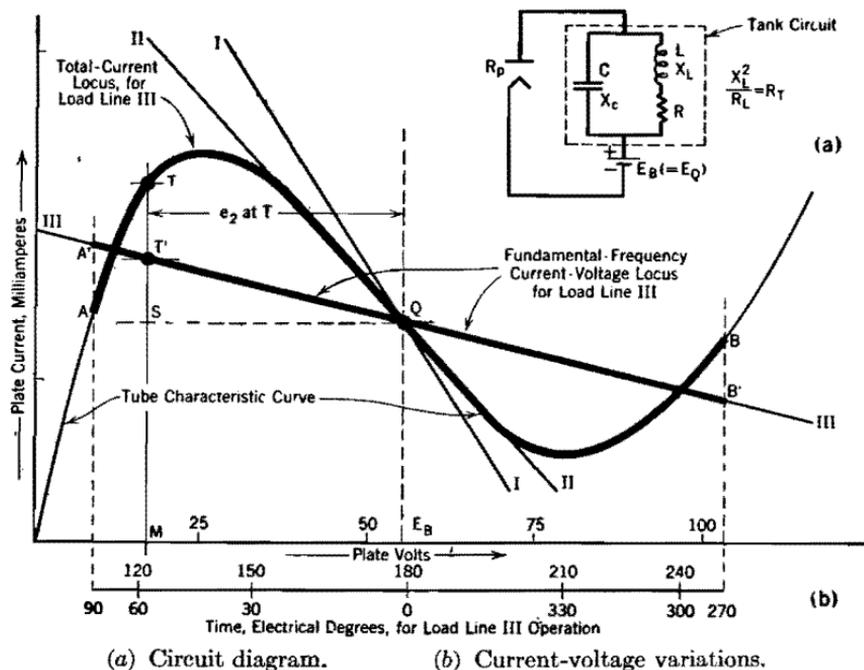
FIG. 134. Dynatron oscillator.
