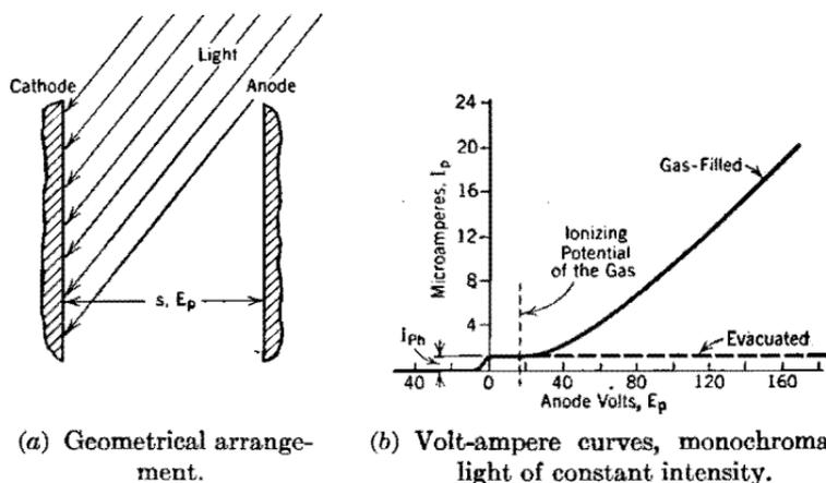
FIG. 152. Effect of inert gas in a phototube with parallel plane electrodes.
