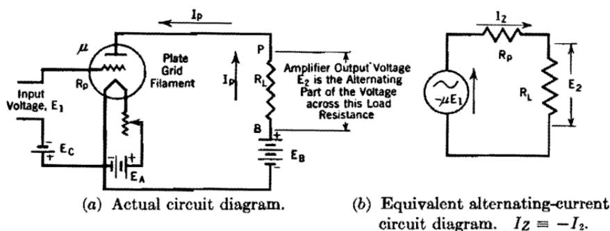
FIG. 102. Amplifier circuit with resistance load.
