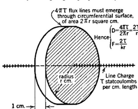
FIG. 16. One-centimeter cylinder around a line charge.  $D$  = electric flux density,  $F$  = electric field intensity,  $k$  = dielectric constant.
