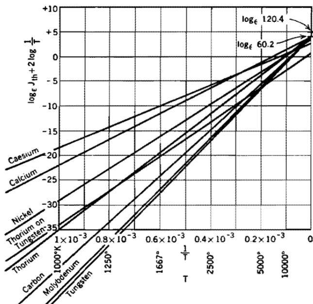
FIG. 64. Logarithmic temperature-emission chart, illustrating method of determining thermionic emission constants. For each line, the slope is  $b_0$ , and the infinite-temperature intercept is  $\log_e A_0$ . Plotted according to Equation (307).
