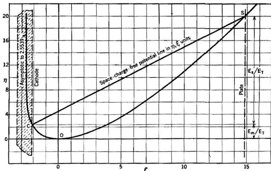
FIG. 95. Effect of initial electron velocities on the space-charge-limited potential distribution outside a plane cathode. See Equations (445) and (446).  $\eta$  is a measure of potential,  $\xi$  of distance.
