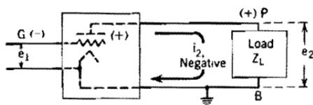
(a) *Electronic amplifier.* To make  $P$  momentarily positive as here shown, the alternating load current must flow in the direction indicated by the arrow. However, this direction of current flow corresponds to a *negative* value of  $i_z$ , so also to a negative value of  $e_1$ . Thus for the instant here shown  $G$  is negative. (See Section 138.)
