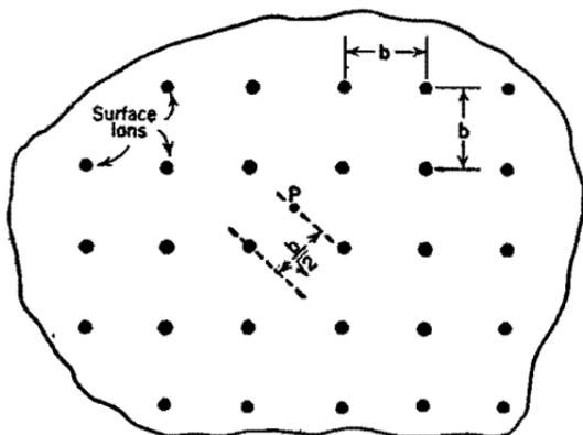
FIG. 75. Array of surface ions of a metal.
