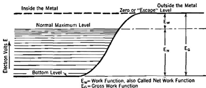
FIG. 69. Energy levels for the electron gas in a cold metal (normal state).
