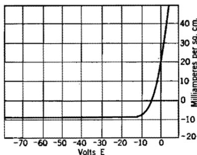
FIG. E. Current density to the case of a mercury-arc rectifier.
