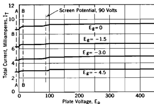
FIG. 54. Curves of total current (screen current plus plate current) vs. plate voltage, for an RCA Type 24 screen-grid tube.
