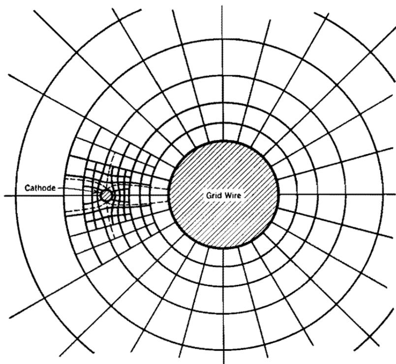
FIG. 21.  $Z$ -plane representation of the electric field map, in the neighborhood of grid and cathode, for a triode at cut-off. No charge on cathode (see Fig. 4c).
