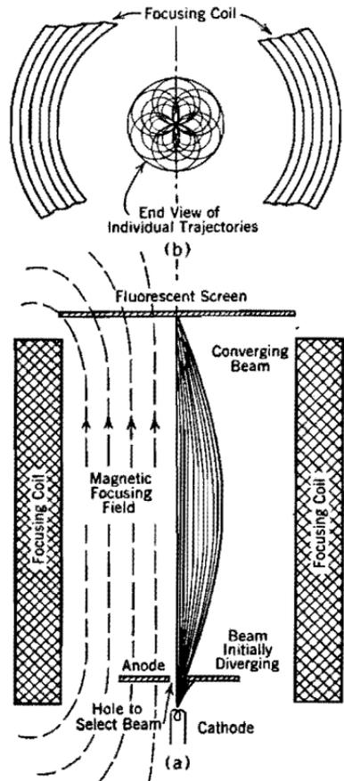
FIG. 40. Magnetic focusing of a cathode-ray oscillograph beam.
