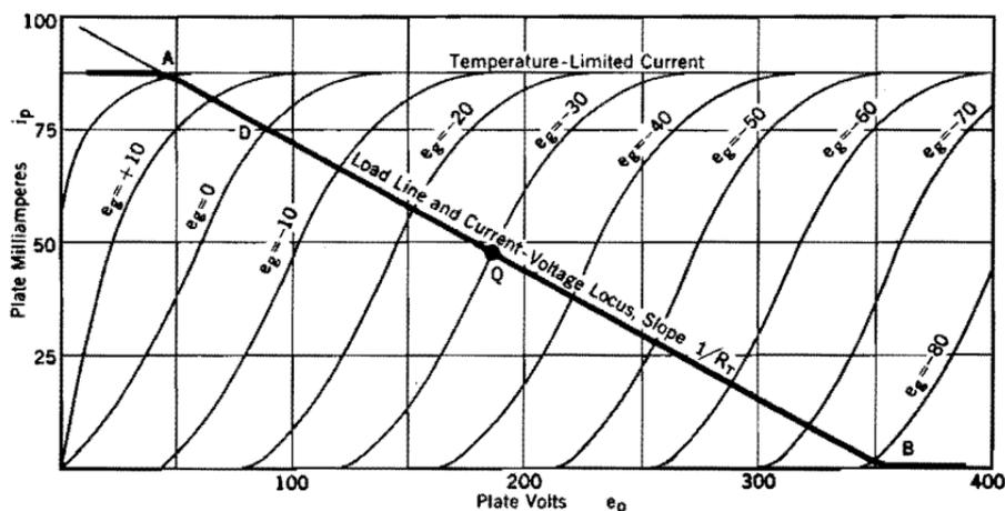
FIG. 132. Current-voltage locus for a tuned plate oscillator.
