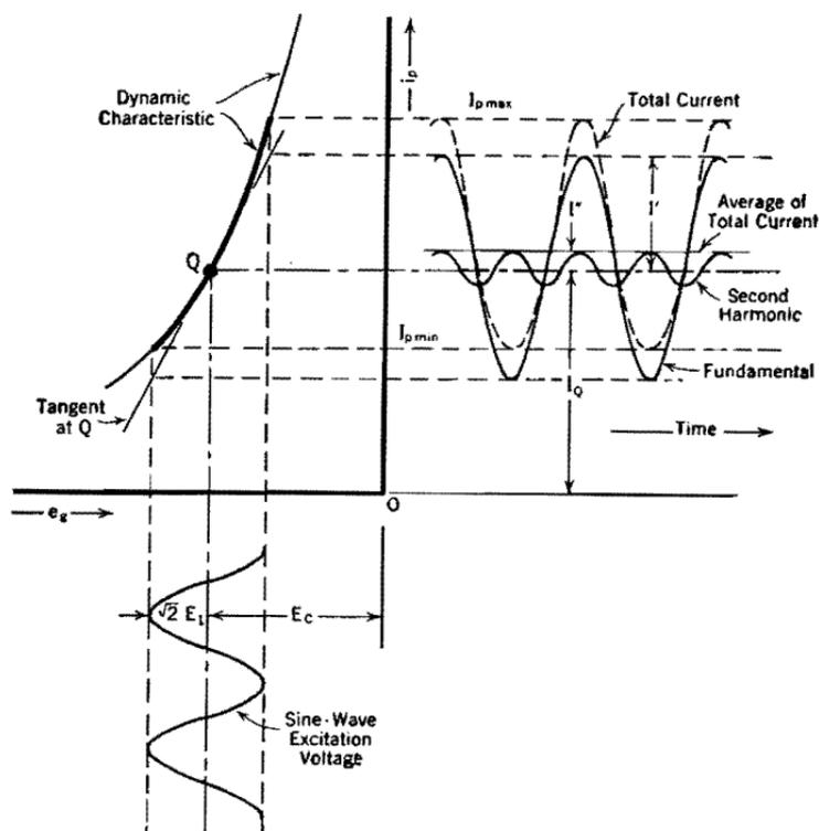
FIG. 116. Production of second harmonic and shift of average current when dynamic characteristic is parabolic.
