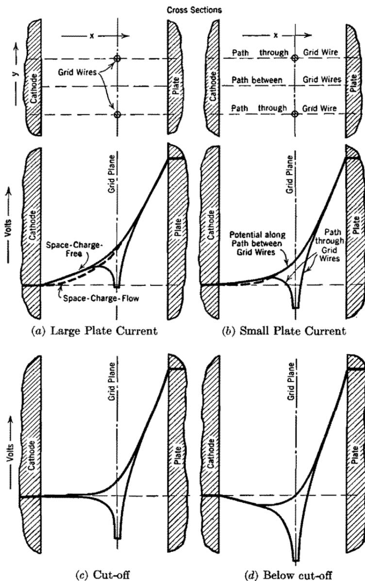
FIG. 4. Potential distribution diagrams for a parallel-plane triode at various grid voltages.
