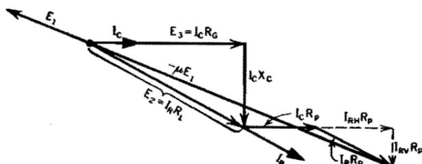
FIG. 126. Resistance coupling, with blocking condenser.
