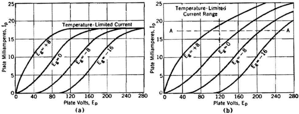
“ Saturation ” with a tungsten filament.
