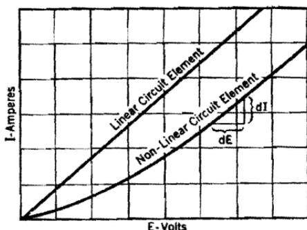
FIG. 100. Contrast between linear and non-linear circuit elements.
