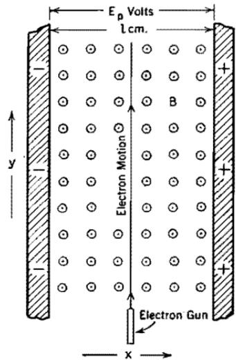
FIG. 30. Straight-line electron motion with balanced uniform electric and magnetic fields.
