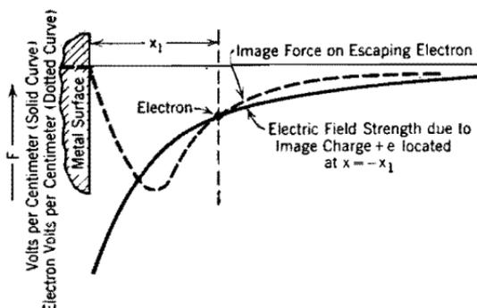
FIG. 74. Contrast between the curve of electric force and that of electric field strength in the continually changing field set up by an escaping electron.
