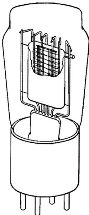
FIG. 24. Triode with grid-like filament construction.
