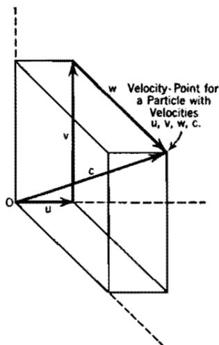
FIG. 90. Coordinate system for velocity points.
