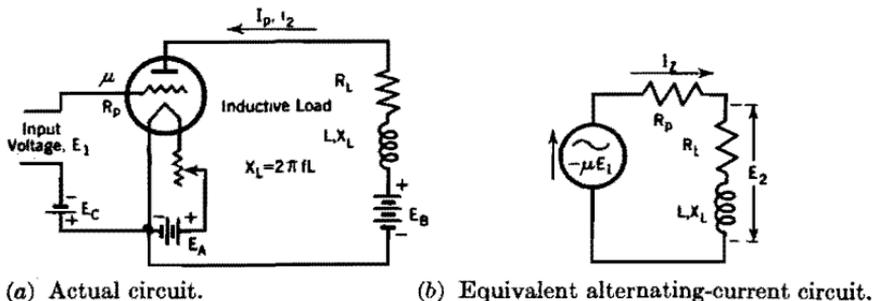
FIG. 107. Class A amplifier circuit with inductive load.
