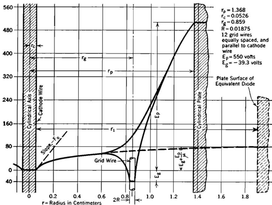
FIG. 26. Space-charge-free potential distribution in cylindrical triode like that of Fig. 25.
