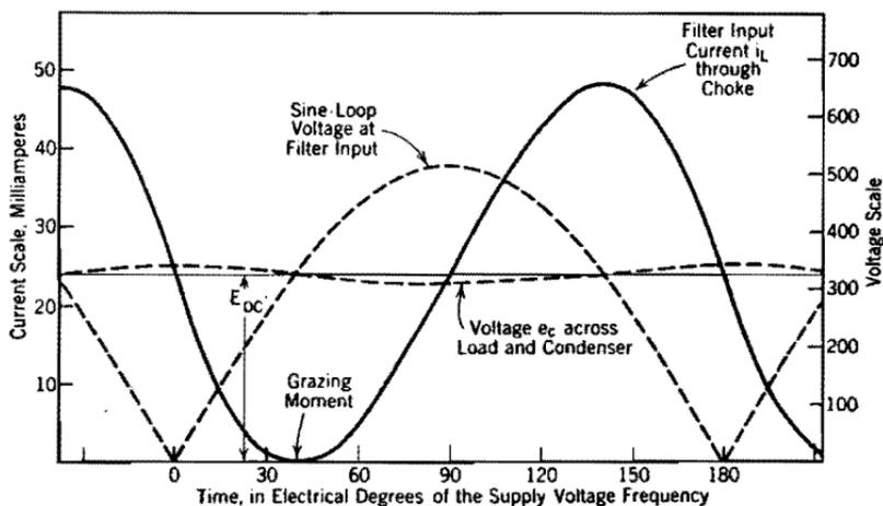
FIG. 189. Voltage and current waves corresponding to point *B*, Fig. 188, with *B* and *C* chosen to give 9.4 per cent ripple at that load.  $X_L/X_C = 3.8$ .
