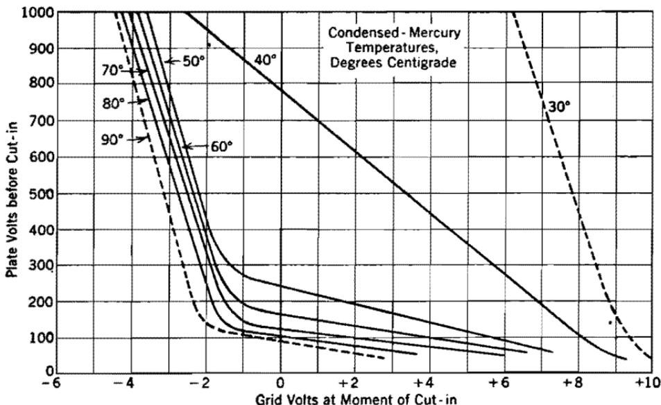
FIG. 182. Typical grid-control curves for a General Electric type FG-67 thyatron.
