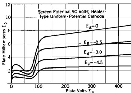
FIG. 55. Plate characteristic curves for an RCA Type 24 (heater-type cathode) screen-grid tube.
