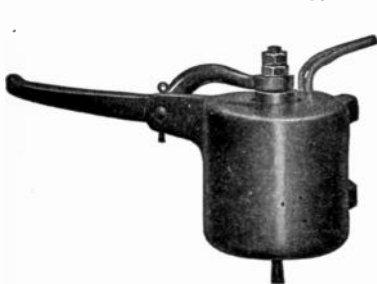
FIG. 2,271.—General Electric shunt trip attachment. The shunt trip attachment has been designed to provide for conditions under which the low voltage attachment cannot be successfully applied. It resembles the low voltage attachment in construction, but differs in that it trips the circuit breaker when energized. The shunt trip should be allowed to remain only momentarily in circuit; hence it should be so connected that the opening of the circuit breaker immediately disconnects it from the circuit. Whenever it is impossible to connect the shunt trip in this manner, the circuit opening auxiliary switch should be used in connection with it.
