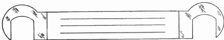
FIG. 2,242.—Notched end fuse. This is a simple form of fuse consisting of a strip of metal (or wire) fixed between two end pieces to fit around the terminals. This type is often proportioned so that it is only possible to place the correct size of fuse in the terminals. Sometimes, in place of the end pieces as shown, the fuse metal is fixed between two clamping screws.
