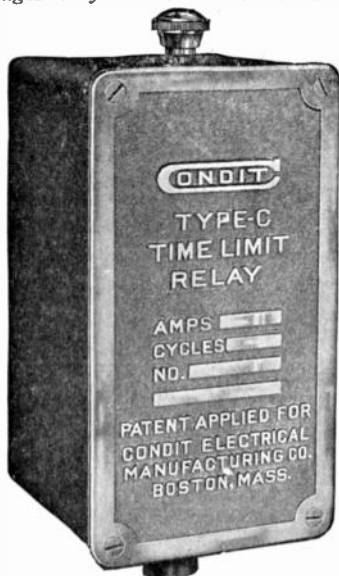
FIG. 2,342.—Condit time limit relay, designed primarily for use in connection with feeder circuits, where close selection or discrimination of circuit breakers is not required. It may be used satisfactorily on lighting and power circuits and also where there are sudden, momentary fluctuations of current. This relay is used in connection with series transformers. The contact arrangements are provided so that therelays may be used as circuit closing or circuit opening relays. The delayed action is produced by an air vacuum dash pot with a graphite piston. The piston of the dash pot is connected to an arm arranged to be moved by the armature. When the current reaches a point where it overcomes the weight of the armature and lifts the same, the magnetic force tending to lift the armature is opposed by the pull of the vacuum created in the interior of the shell into which fits the graphite piston. As the magnetic pull continues the vacuum is overcome due to the leakage of air past the piston, and the armature gradually moves until it reaches a point where it causes the circuit breaker to trip, either by closing the contacts in the circuit closing type, or by opening the contacts in the circuit opening type. If, at any portion of its travel, the current drop to normal, the armature immediately resets. The time adjustment consists of an arrangement whereby the distance through which the armature moves before tripping the breaker, may be changed, thus altering the time of tripping. The current adjustment is made by changing the effective turns of the actuating coil, the travel of the armature and the force exerted by it being the same for all current adjustment. The winding is designed to carry 5 amperes continuously with a temperature rise not exceeding 68° Fahr. standard calibration is provided so that the relay will start to operate at 5, 6, 8 and 12 amperes.
