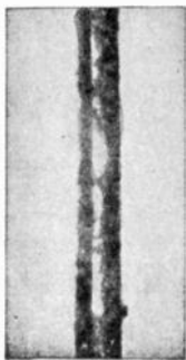
FIGS. 3-438 to 3-440. —Behavior of tantalum filament. Fig. 3-438, unburned tantalum filament; fig. 3-439, tantalum filament after burning 800 hours on alternating current. The new filament is smooth and without regular structure, while after burning for some time, it begins to take on a crystalline appearance. This change takes place less rapidly with direct than with alternating current, so that the life of the lamp is somewhat greater in the former case. When the filament finally burns out, it is supposed to be due to the change from the amorphous to the crystalline state, as indicated in the illustrations.
