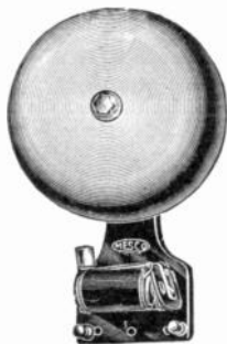
FIG. 3,204.—Mesco single stroke bell. The hammer rod has a short leverage but a long sweep, thus enabling it to give rapid and powerful blows. A stiff flat spring causes the hammer to leave the bell immediately after striking. The magnets of this bell are regularly wound for 6 ohms, and special for incandescent lighting circuit. Sizes 3 to 18 inch.
