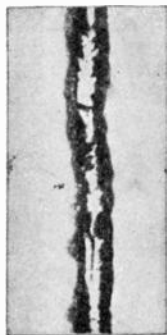
FIGS. 3-438 to 3-440. —Behavior of tantalum filament. Fig. 3-438, unburned tantalum filament; fig. 3-439, tantalum filament after burning 800 hours on alternating current. The new filament is smooth and without regular structure, while after burning for some time, it begins to take on a crystalline appearance. This change takes place less rapidly with direct than with alternating current, so that the life of the lamp is somewhat greater in the former case. When the filament finally burns out, it is supposed to be due to the change from the amorphous to the crystalline state, as indicated in the illustrations.
