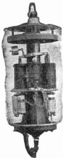
FIGS. 3,383 and 3,384.—Westinghouse series parallel circuit metallic flame arc lamp with case removed showing mechanism, and circuit diagram of same. In operation, fig. 3,384, when current is turned on it energizes the shunt coils A, bringing the electrodes B and C together. Current then flows through the series resistance D, and the series cut out coil E to the series coils F, thence to positive electrode C, negative electrode B, and negative terminal. The series coils F, and cut out coils E, now being energized, pull apart electrodes B and C, and contacts G and H, striking the arc. The shunt coils A, being connected across the arc, are regulated by the arc voltage. The voltage across the arc will increase as the electrodes are pulled apart, and the series magnets F will separate the electrodes until the voltage across the arc (approximately 65 volts) which is impressed across the shunt coils A, is high enough to energize the shunt magnet coils sufficiently to balance the series coils F when 5 amperes flow. If the electrodes burn out or fail to contact, no current will traverse the cut out coils E or series coils F. The contacts G and H will therefore remain in contact and current will then flow through the series resistance D, contacts G and H substitutional resistance I, and pass to the negative terminal. The automatic cut out and substitutional resistance arc provided on the series parallel circuit lamp but are not necessary on the parallel circuit lamp.
