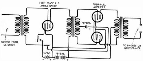
FIG. 66.-An audio-frequency amplifier circuit employing push-pull amplification.
