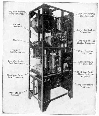
Fig. 27.-Rear view of RCA vacuum tube transmitter type ET-3626.
