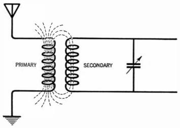
FIG. 57.-Magnetic or inductive coupling.
