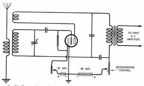
FIG. 54 .-- Regenerative receiver employing variable resistance to control regeneration.
