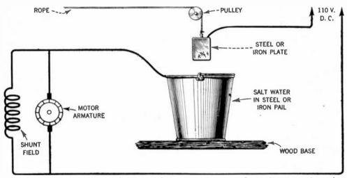
F1G. 77.—A water rheostat may be employed as an emergency starting resistance as shown in this illustration.
