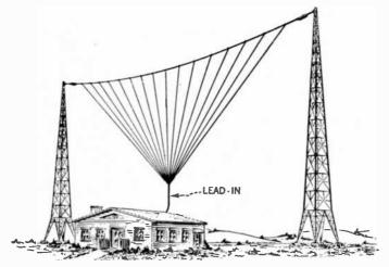
FIG. 45.—The vertical fan-type antenna.
