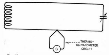
Fig. 65.-A wavemeter circuit using a thermo-galvanometer.
