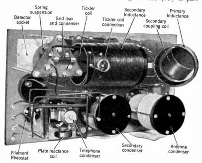
FIG. 3.-Rear view of the IP-501 receiver.
