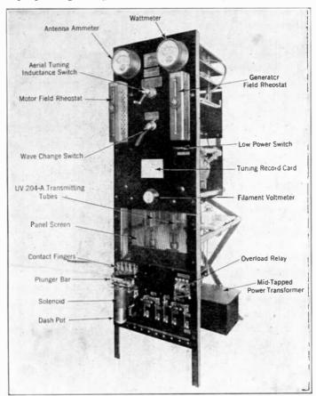
Fig. 2.-Front panel view of P-8 converted tube transmitter, type ET-3628.
