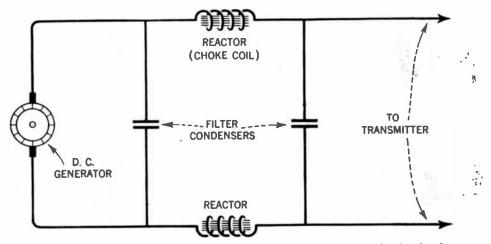
Fig. 16.—A fundamental filter system suitable for use in the plate supply circuit of a vacuum tube transmitter.
