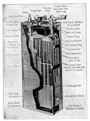
FIG. 85.—Cross-sectional view of the Edison storage cell.
