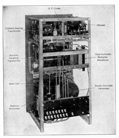
FIG. 8.-Rear view of ET-3627A tube transmitter.
