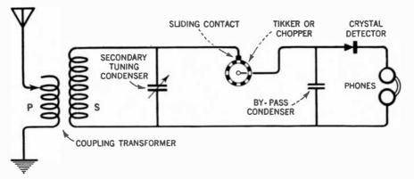
FIG. 62.-A crystal detecter may be used with a tikker or chopper to receive c.w. signals.
