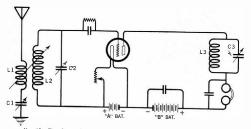
Fig. 63.-Showing various uses of variable condensers in a receiving circuit.
