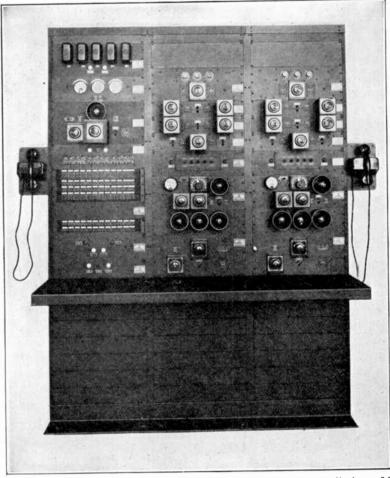
Fig. 14.—Control room speech input apparatus for a double studio installation. Monitoring (volume control) rheostats and speech amplifiers are shown on this control room speech input apparatus for a double radio installation. The high-level switching arrangement provides for rapid changeover from one program to another.
