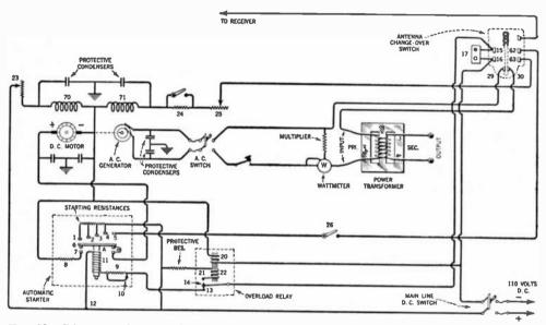
FIG. 80.—Diagram of a complete motor-generator installation and "finger" type automatic starter connected in the power circuit of a spark transmitter.
