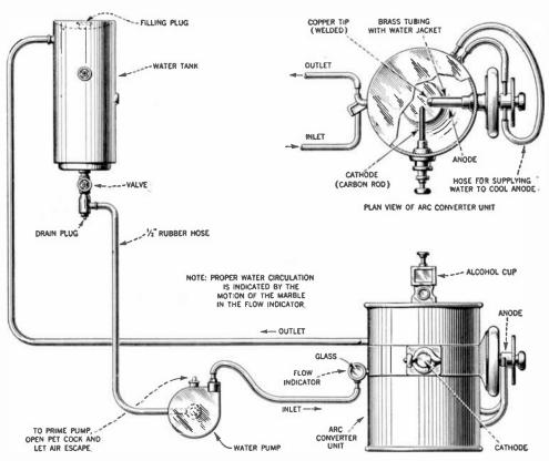
FIG. 30.—An illustration of the circulating system of the Federal arc transmitter.
