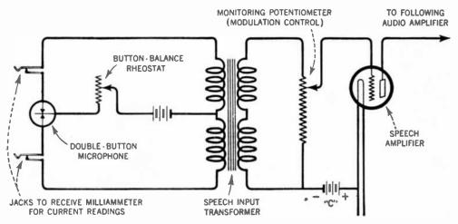
FIG. 21.—A double-button carbon-type microphone connected in an amplifier circuit.
