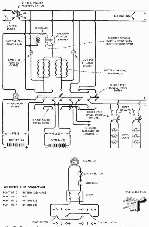
FIG. 87.-Diagram of a complete battery charging circuit of the type used on shipboard.
