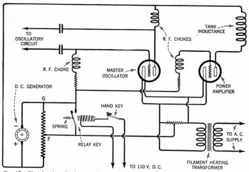
FIG. 17.—Showing how keying may be accomplished in a tube transmitter by the application of a high negative bias voltage on the grids.
