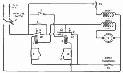
FIG. 78. -Automatic starter used with a compound-wound motor.
