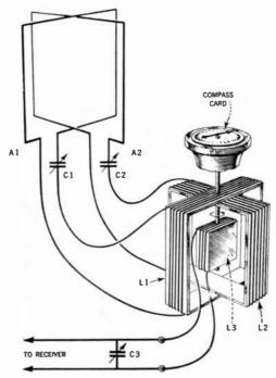
FIG. 70.-The Bellini-Tosi Goniometer. One type of radio direction finder.
