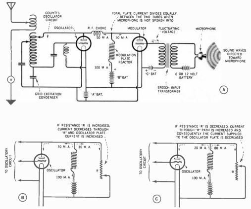
FIG. 25.—Diagrammatic explanations of the Heising (constant current) system of modulation.
