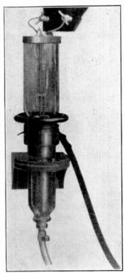
FIG. 50.—A water-cooled tube mounted in its water jacket.
