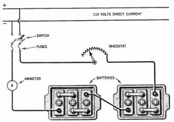
F16. 82.—One method of charging "A" batteries. A variable rheostat is inserted in series in the 110-volt line to regulate the charging current.
