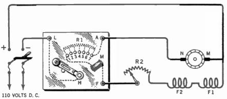
FIG. 79.-Cutter-hammer hand starter connected to a shunt-wound motor.
