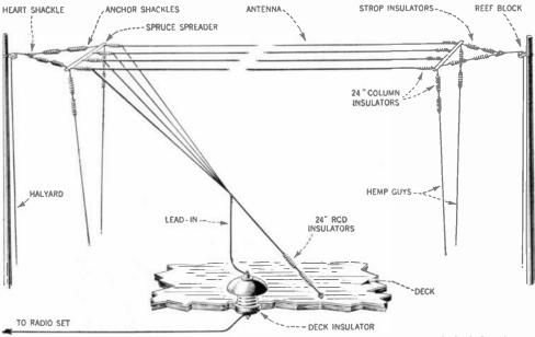
FIG. 42.—A detailed sketch of the flat-top inverted "L" antenna, lead-in and deck-insulator of the type commonly installed on shipboard.
