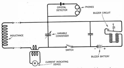
F16. 59.—A wavemeter circuit with current indicating device, crystal detecter, phones, battery and buzzer.
