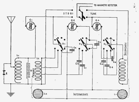
Fig. 169-Detailed Wiring Diagram of Multiple Tuner.
