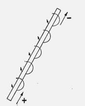
Fig. 12a-Showing Lines of Force Around a Conductor with the Current Flowing Away from Reader.
