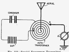
Fig. 333-Special Emergency Transmitter.
