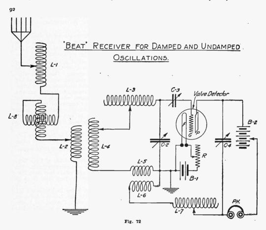
Fig. 294-Complete Circuits of a Beat Receiver.
