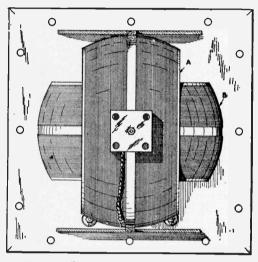
Fig. 192-The Construction of the Variometer.
