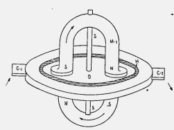
Fig. 83-Motor of Ampere Hour Meter.
