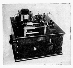
Fig. 268-The Tuned Receiver for the Direction Finder.
