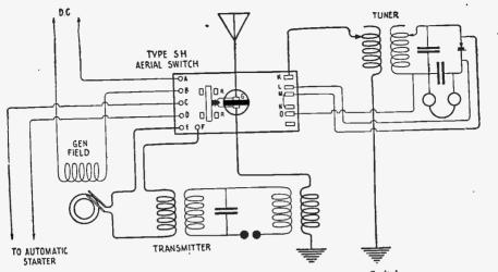
Fig. 136-Connections of a Modern Aerial Changeover Switch.
