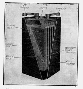
Fig. 86a-Detail of Exide 11 M. V. Storage Cell.
