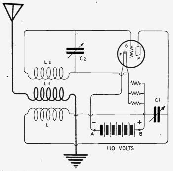
frequency can be generated by proper variation of inductance and capacity; in fact, current at frequencies from 60 to 1,000,000 cycles per second can be obtained.
