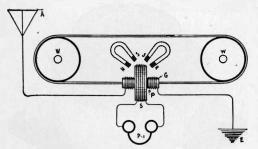
Fig. 167-Marconi's Magnetic Detector.
