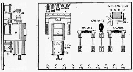
Fig. 251-Automatic Starter Panel (2 K. W. 500 Cycle Transmitter).
