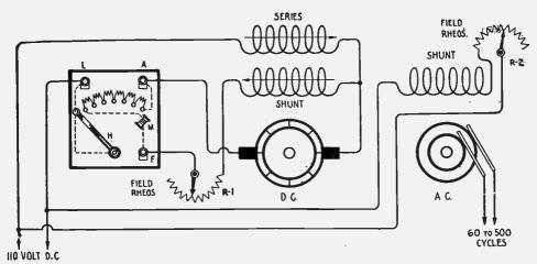
Fig. 76-Hand Starter Connected to Motor Generator with Differential Motor Winding.
