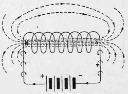
Fig. 15-Magnetic Field of Solenoid Winding.
