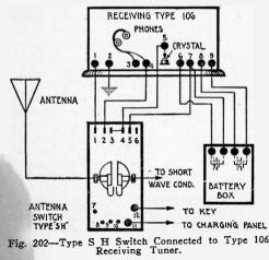
former from the aerial during the period of reception, preventing the incoming oscillations leaking to earth. The various circuits closed by the discs mounted on the hard rubber rod place the detector and head telephone on short circuit during the period of transmission. They may also be employed to start and stop a motor blower or an automatic motor starter. The type I switch is supplied with Marconi transmitting sets up to 5 K. W. capacity.
