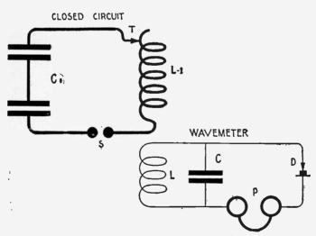
open circuit and the wave length noted by adjusting the wavemeter to resonance.
