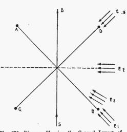
Fig. 273-Diagram Showing the General Layout of the Direction Finder Aerials.
