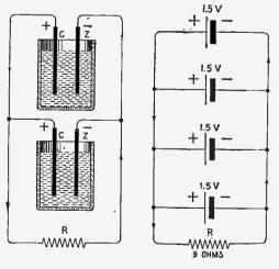
Fig. 7-Electric Cells Joined in Parallel.
