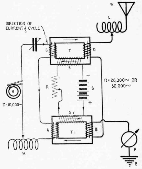
Fig. 284-The Joly-Arco Undamped Wave Transmitter.
