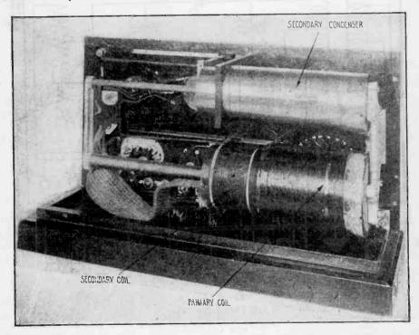
Fig. 203b-Rear View of Marconi Type 112 Receiving Tuner (The American Marconi Company).
