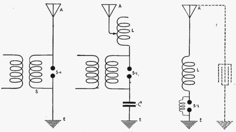
Fig. 97a—Plain Aerial Excitation. Fig. 97b—Showing Position of Short Wave Condenser and Aerial Tuning Inductance. Fig. 97c—Illustrating the Effective Capacity of an Aerial.
