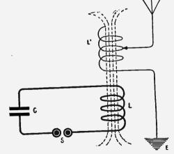
Fig. 106--Inductively Coupled Transmitter.
