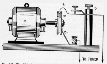
D, of Fig. 289. The circuit is completed through the brush, B-1, in contact with the wheel W. When the wheel is in rotation, there is a constant slipping and gripping of the brush B on the wheel which makes a contact of variable resistance, causing the charge accumulated in the telephone condenser to vary in accordance. The note in the telephone will have a pitch in accordance. Both the tikker and
