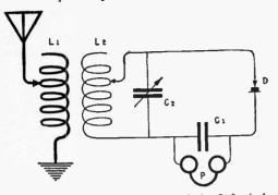
Fig. 150.—Fundamental Diagram of the Inductively Coupled Receiver.
