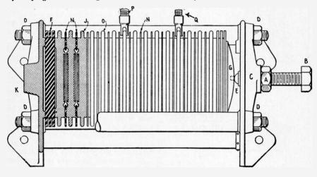
Fig. 253-Detailed Sketch of Marconi Quenched Spark Gap.
