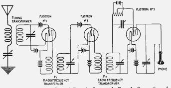
Fig. 296, which is a method of connection particularly suited to the pliotron oscillators of the General Electric Company.
