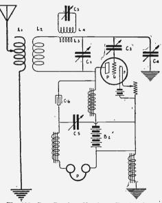
vacuum valves, have been found suitable to the reception of undamped oscillations; in fact, the majority of these circuits are equally well adapted for the reception of damped oscillations, but, as mentioned previously, the normal note of a spark transmitter is distorted when the maximum amplification is obtained.
