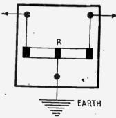
Fig. 78-Protective Resistance Rod.
