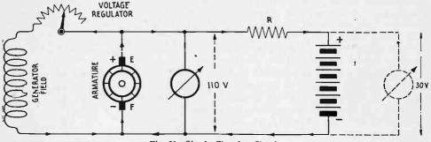
Fig. 81-Simple Charging Circuit.
