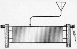
Fig. 127-Drum Type Aerial Tuning Inductance.
