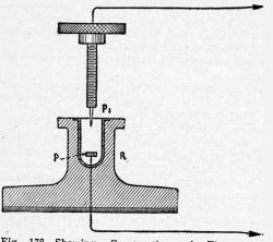
Fig. 178—Showing Construction of Electrolytic Detector.
