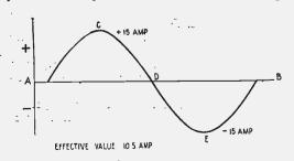
Fig. 41-Rise and Fall of Alternating Current.
