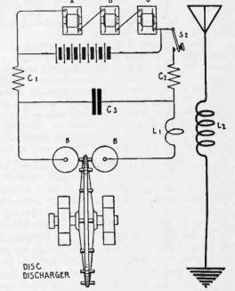
Fig. 302-Fundamental Circuit of the Glace Bay Type of Transmitter.
