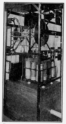
Fig. 146a-3 Kilowatt Non-Synchronous land station type of transmitter (American Marconi Company).
