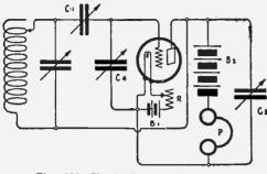
Fig. 184-Simple Regenerative Circuit.
