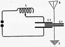
Fig. 108-One Method of Capacitive Coupling.
