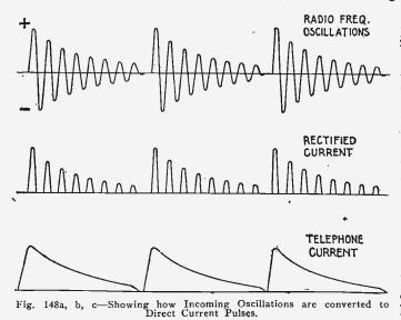
Now, if continuous oscillations of unvarying amplitude were induced in the receiver aerial, the rectified current would merely displace the telephone diaphragm and hold it in this position until the current is turned off, but since in the damped systems of radiotelegraphy, the oscillations are discontinuous, or occur in groups, the current falls to zero at the end of each group, and, hence, the diaphragm of the telephone is released, creating a single sound.
