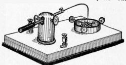
Fig. 160—Detector Holder for Galena and Silicom Crystals.
