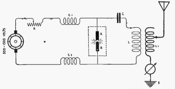
into the generator. C is the usual condenser of the closed oscillation c i r c u i t and L the variable inductance. In the usual manner, the oscillations generated in this circuit are transferred to the antenna circuit by means of an oscillation transformer.
