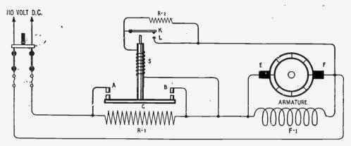
Fig. 73-Circuit of Automatic Starter for Marconi 1/2 K. W. 120 Cycle Set.
