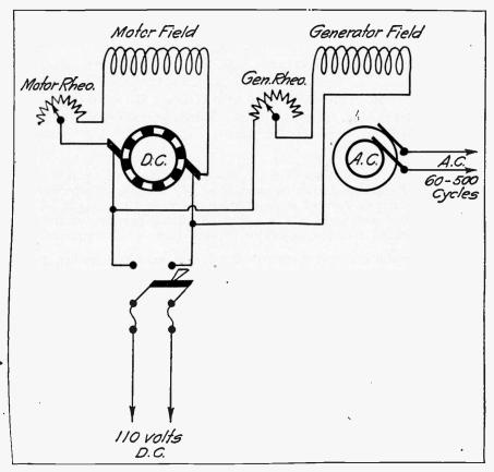
Fig. 64--Simple Shunt Wound Motor Generator.
