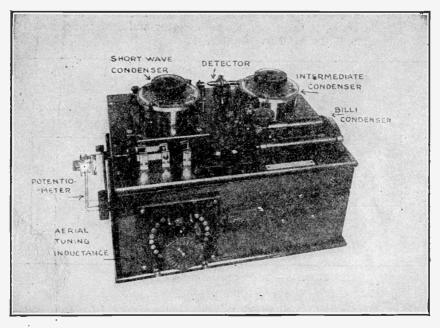
Fig. 166-Type 107a Tuner (Modified Valve Tuner).
