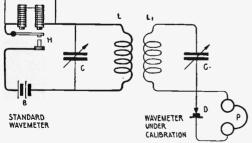
Fig. 234—Simple Method of Calibrating a Wavemeter from a Standard.
