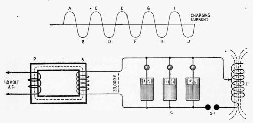
Fig. 93 .- Apparatus for Production of Radio Frequency Oscillations.
