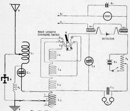
Fig. 176-Wiring Diagram Marconi Universal Receiver.
