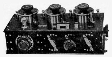
Fig. 167a-Marconi Multiple Tuner.
