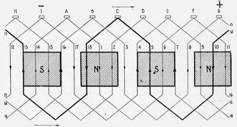
Fig. 34-Development of Wave Winding.
