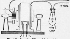
Fig. 328-Locating "Grounds" in a Motor.
