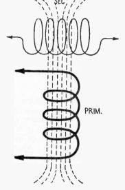
Fig. 120—Showing the Effect of Turning Secondary at Right Angles to Primary.
