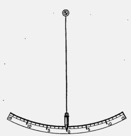
Fig. 105a-Pendulum for Illustrating Damping.
