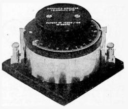
Fig. 166a-Marconi Disc Variable Condenser.
