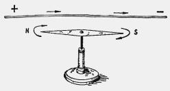
Fig. 11-Deflection of Compass Needle by Electric Current.
