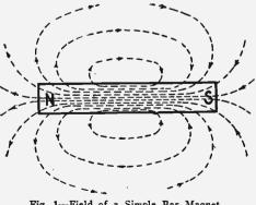
Fig. 1--Field of a Simple Bar Magnet.
