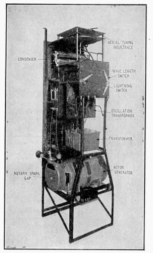
Fig. 259-Rear View of the Marconi ½ K. W. 500 Cycle Panel Transmitter.
