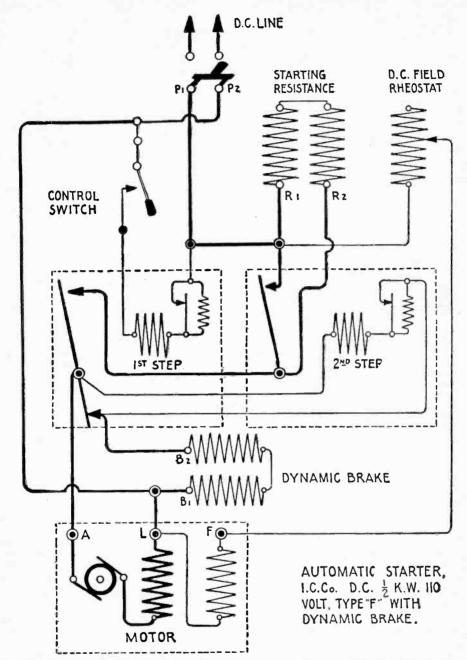
Fig. 255—Fundamental Wiring Diagram of the Automatic Starter Furnished With the Marconi 1/2 K. W. 500 Cycle Transmitter. (See Fig. 74 and Section J in Appendix)
