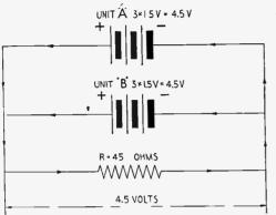
Fig. 8-Cells Grouped in Series Parallel.
