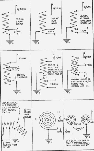
Fig. 244—The Method of Checking un Coupling and Turns of a Helix as Authorized by the U. S. Government.
