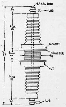
Fig. 146-Electrose Moulded Insulator.
