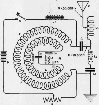
Fig. 283—Complete Circuit of the Goldschmidt Alternator. 217. Goldschmidt Radio-frequency Alternator.—By adopting the simple principles of electrical resonance, Dr. Goldschmidt has designed an alternator which, by the use of a single armature, generates radio current at frequencies from 30,000 to 75,000 cycles per second. The great advantage of this alternator is the low speed of the armature, which, even in the 200 K. W. sizes, does not exceed 3,100 R. P. M.
