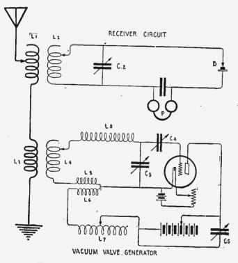
Fig. 293-The Vacuum Valve Heterodyne Receiver.
