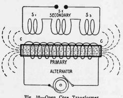
Fig. 38-Open Core Transformer.
