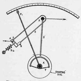
Fig. 53-Mechanism of Hot Wire Ammeter.
