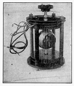
Fig. 272-Detail of the Radio Goniometer.
