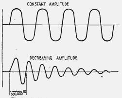
Fig. 89-Oscillations of Decreasing Amplitude.
