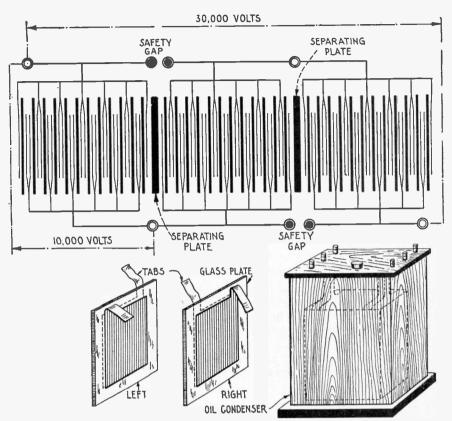
Fig. 129-Assembly of the Oil Plate Condenser.
