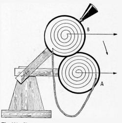
Fig. 123-Showing Fundamental Principle of the Variometer.
