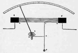
Fig. 54-Hot Wire Ammeter with Internal Shunt.
