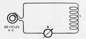
Fig. 43-Alternating Current Circuit with Concentrated Inductance.
