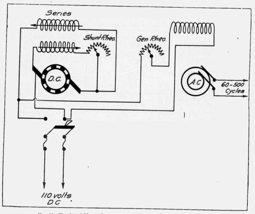
Fig. 66-Circuits of Motor Generator with Differential Motor Field Winding.
