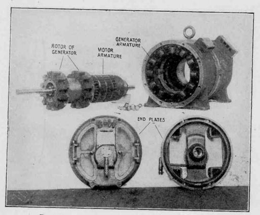
Fig. 67c-Details of 1/2 K. W. 500 Cycle Crocker Wheeler Motor Generator.
