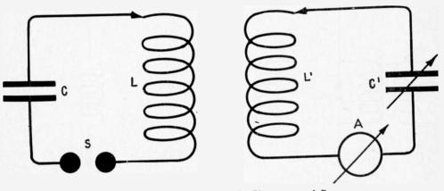
Fig. 96-Circuits for Demonstrating the Phenomenon of Resonance.
