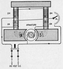
Fig. 29-Motor with Differential Field Winding.
