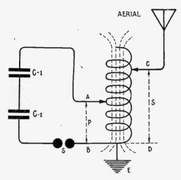
Fig. 107-Conductively Coupled Transmitter.
