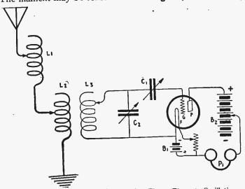
The circuit generally adopted for the three element valve appears in Fig. 179, where the primary and secondary circuits of a receiving tuner are represented by the usual notations and the grid, plate and filament of the valve by G, P, and F, respectively. An important part of this circuit is the so-called grid condenser C-1, which generally has low capacity, varying between .00003 and .0005 microfarads.
