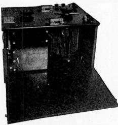
Fig. 267-The Radio Goniometer.
