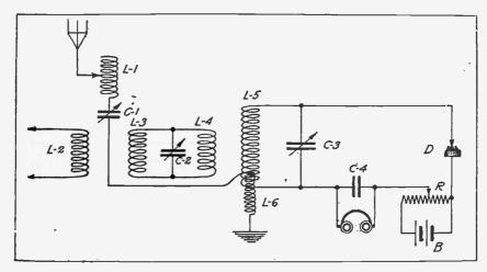
Fig. 165c-"Standby" Short Wave Circuits of 107a Tuner.
