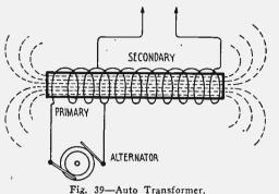
copper strips, the tubing being from 1/2 to 3/4 inch in diameter for the small size sets. Winding S may have several turns, a dozen or more of insulated wire or small copper tubing. On the other hand, if the auto transformer is used in receiving sets, winding P may consist of several hundred turns of No. 24 B. & S. wire, and winding S may have several hundred turns of No. 32 B. & S. wire.
