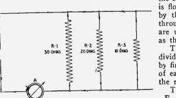
the 3 branches. If a current of 9 amperes is flowing in the main circuit as indicated by the ammeter A, 3 amperes will flow through each branch. If the resistances are unequal, the current divides inversely as their relative resistance.
