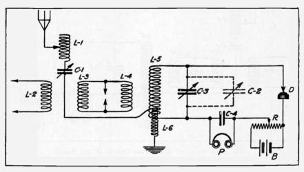
Fig. 165a-"Standby" Long Wave Adjustment of Marconi Type 107a Tuner.
