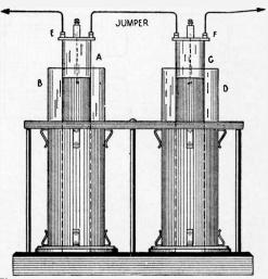
Fig. 128-Short Wave Condenser American Marconi Company.
