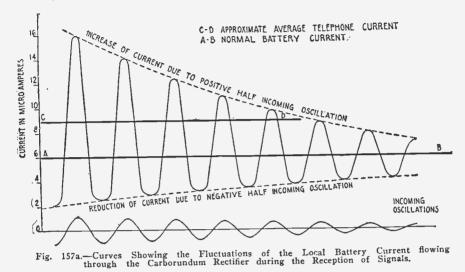
pressed upon the crystal is greater than the subtracted voltage and that the final effect of this is an increase of current through the head telephone circuit over the duration of one wave train.
