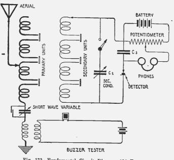
Fig. 172-Fundamental Circuit Diagram 106 Tuner.
