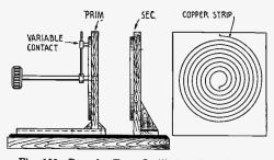
Fig. 122-Pancake Type Oscillation Transformer.
