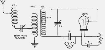
when the terminals of the closed or secondary circuit of a receiving tuner are connected to the negative side of the filament and to the plate of the valve, the alternating current of radio-frequency flowing in the receiver circuits will be converted into a uni-directional current which may affect a head telephone or other recording instrument. More clearly, the oscilla-
