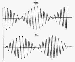
Fig. 109.—Showing Complex Oscillations in Improperly Adjusted Transmitter.
