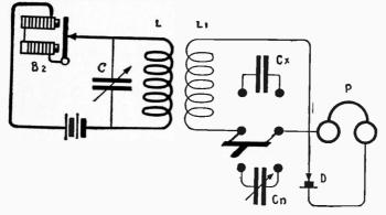
If the aerial and earth wire of an antenna system be substituted for the condenser C-x, its electrostatic capacity may thus be determined, but it should be borne in mind that the simple electrostatic capacity of an aerial and its "effective" capacity when traversed by alternating current of radio-frequency are of different value. This is due to the non-uniform distribution of current and voltage throughout the open cir-
