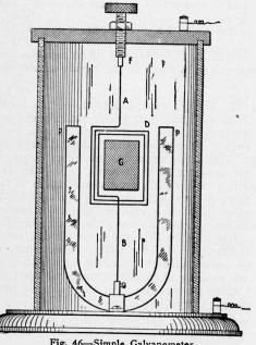
Fig. 46-Simple Galvanometer.
