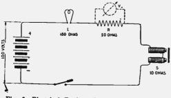
Fig. 9-Electrical Devices Connected in Series.
