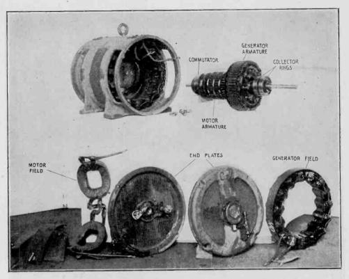
Fig. 67a-Details of Crocker Wheeler 2 K. W. 500 Cycle Motor Generator.
