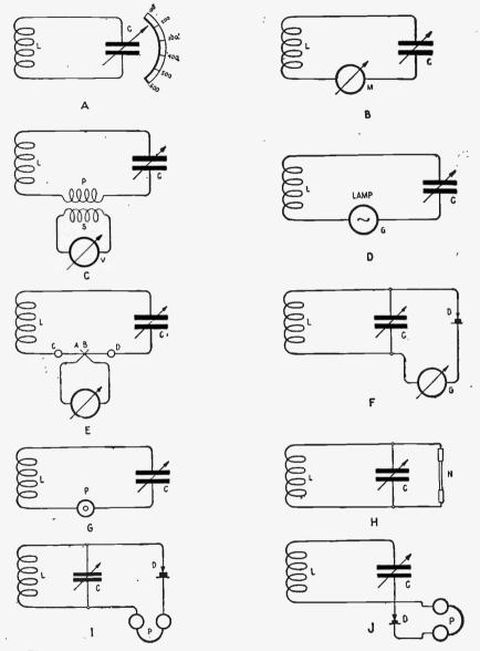
Fig. 210a, b, c, d, e, f, g, h, i, j-Methods for Determining Resonance Between Wavemeter and Circuit Under Measurement.
