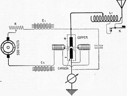
Fig. 279-Complete Circuits of a Modern Arc Transmitter.
