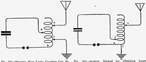
Fig. 241-Showing How Loose Coupling Can Be Fig. 242-Another Method for Obtaining 1 Obtained With an Auto Transformer. Coupling With an Auto Transformer.
