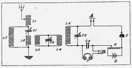
Fig. 165b-"Tune" Circuits of Type 107a Tuner.
