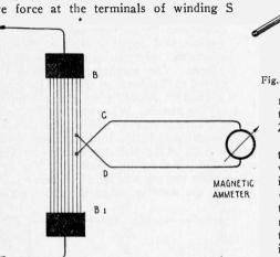
Fig. 55-Aerial Ammeter with Thermo-Couple.
