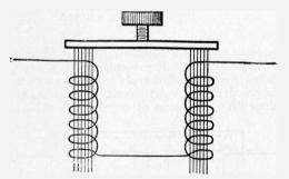
Fig. 135-U Shaped Reactance Coil.
