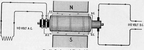
Fig. 70-Fundamental Circuit of Dynamotor,
