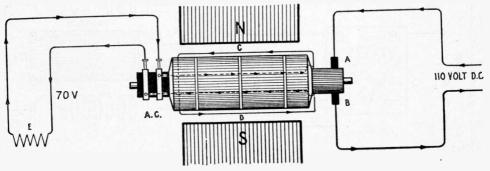
Fig. 69-Fundamental Circuit of Rotary Converter.
