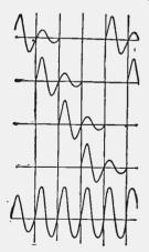
Fig. 286—Showing How Groups of Damped Oscillations Can Be Made to Overlap One Another. Marconi and his engineering staff have developed an exceedingly novel method for generating continuous oscillations, doing away with many of the problems encountered in the construction of intricate high frequency alternators.
