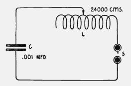
Fig. 95-Closed Oscillation Circuit.
