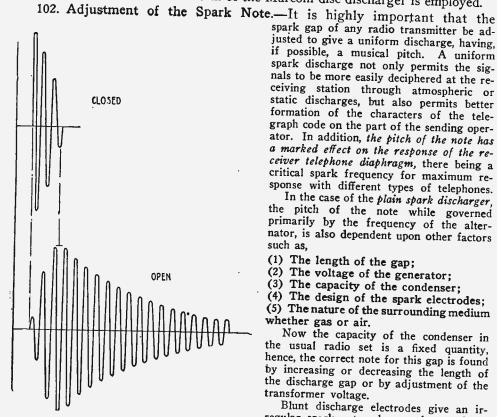
. 118—Showing the Oscillations in Closed and Open Circuits of a Properly Adjusted Transmitter.
