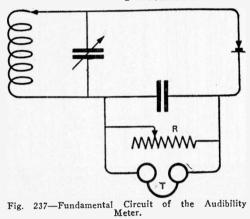
Now the value of C-a for the least audible signal varies with the frequency of the current flowing through the telephone, the impedance of its windings, and the sensitiveness of the human ear to weak sounds. Hence at a given station the value of C-a is ignored and the strength of the signal spoken of as being so many times audibility.
