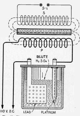
Fig. 59—Electrolytic Interrupter Connected to an Induction Coil.
