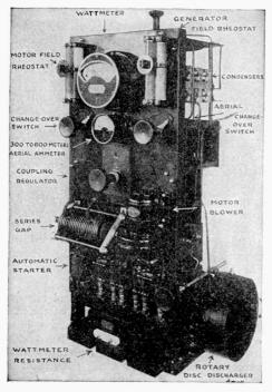
Fig. 264—Front View of the Marconi 1/2 K. W. 120 Cycle Transmitter.
