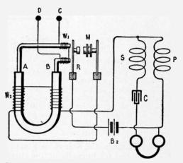
Fig. 197b-Supersensitive Brown Amplification Relay.
