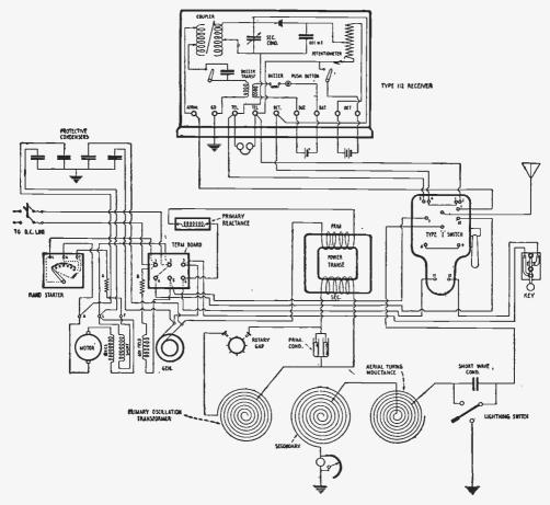
Fig. 266d—Complete Wiring Diagram of the ¼ K. W. Cargo Transmitting Set with Type 112 Receiving Tuner and Type I Aerial Changeover Switch.
