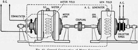
Fig. 63-General Construction of Motor Generator.
