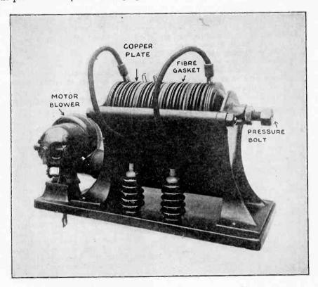
Fig. 117-Modern Quenched Spark Discharger with Motor Blower.
