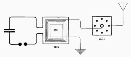
Fig. 125-Square Coil Type Oscillation Transformer.
