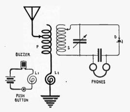
Fig. 194-Buzzer Excitation System.
