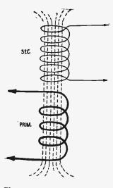
Fig. 121—Showing Position ot Maximum Coupling of Type A Oscillation Transformer,
