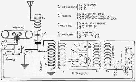
Fig. 168-Fundamental Circuit Marconi's Multiple Tuner.
