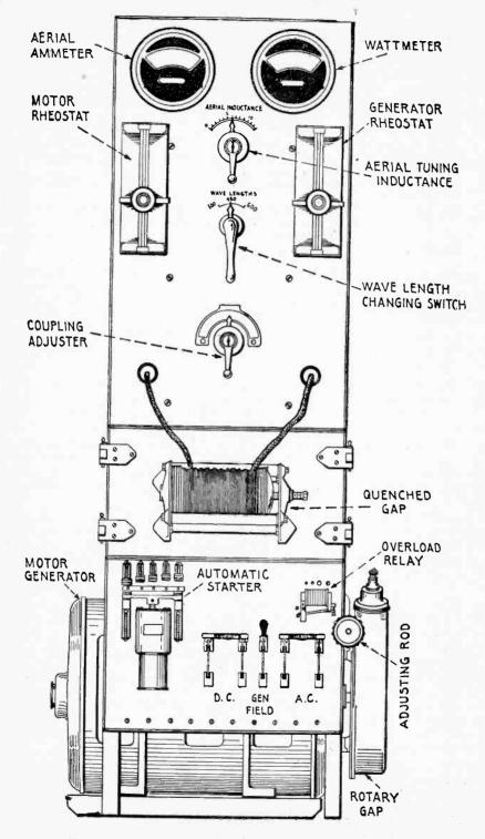
Fig. 247-Front View Marconi 2 K. W. 500 Cycle Transmitting Set.
