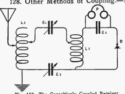
Fig. 152-The Capacitively Coupled Receiver.
