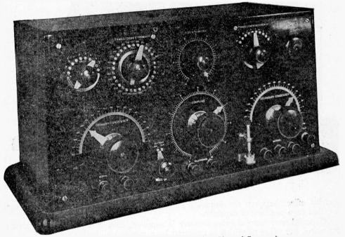
Fig. 170-Type 106 Receiving Tuner (American Marconi Company).
