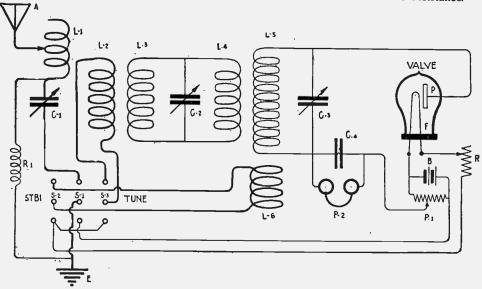
Fig. 162-Fundamental Circuit of Marconi Valve Tuner.
