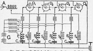
Fig. 285-Marconi's Method of Generating Continuous Oscillations.
