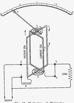
Fig. 51-Mechanism of Wattmeter.
