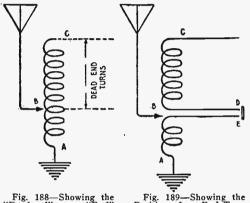
Fig. 188—Showing the "Dead-end" or "End" Dead-end" or "End" Turns of a Receiver Tun-ing Coil.
