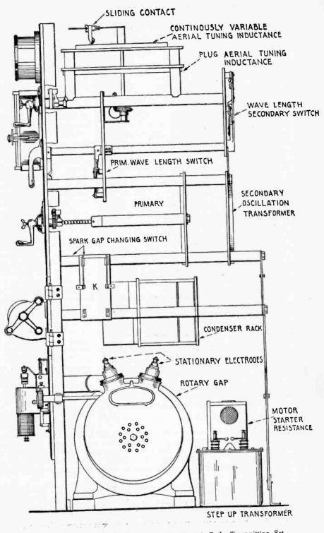
Fig. 248-Side View Marconi 2 K. W. 500 Cycle Transmitting Set.
