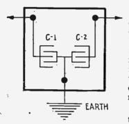
Fig. 77-Protective Condensers.
