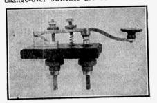
Fig. 137-A Hand Manipulated Telegraph Key.
