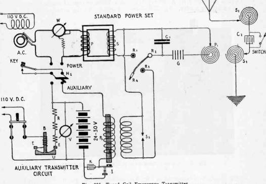
Fig. 205-Tuned Coil Emergency Transmitter.
