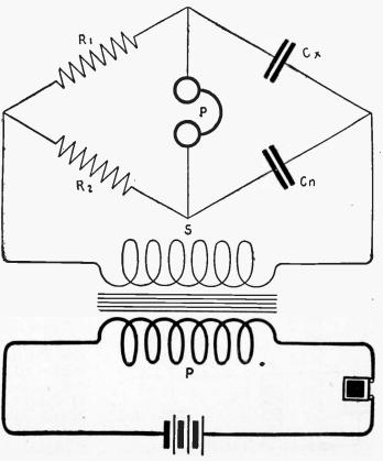
Fig. 227-Diagram for the Measurement of Electrostatic Capacity.
