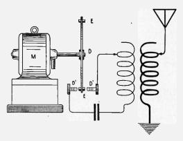
Fig. 113-Non-synchronous Rotary Discharger.
