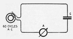
Fig. 44—Alternating Current Circuit with Condenser in ance exceeds the inductance reactance, the Series.
