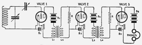
Fig. 185-Vacuum Valves Connected in Cascade.
