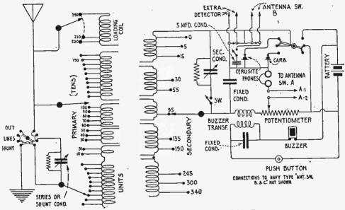
Fig. 175-Fundamental Diagram Type 101 Receiving Tuner.
