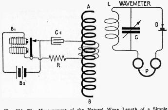
Fig. 226—The Measurement of the Natural Wave Length of a Simple Tuning Coil.
