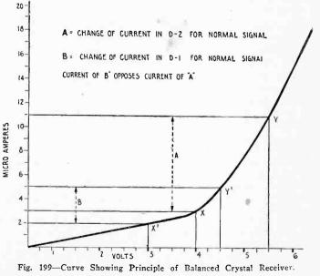
Under these conditions, if an extra severe discharge of static excites the aerial circuit, almost equal effects are produced in the head telephone P by both crystals, and the crashing sounds ordinarily experienced are partially eliminated.
