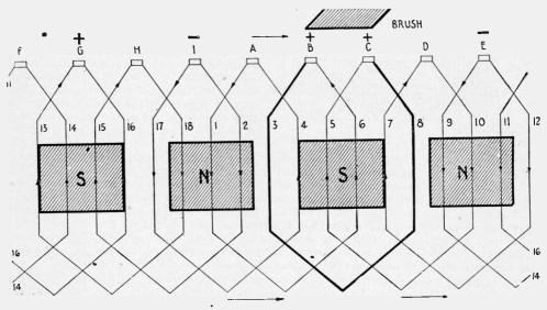
Fig. 32-Development of Lap-Wound Armature.
