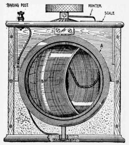
Fig. 193-The Tuning Variometer Complete.
