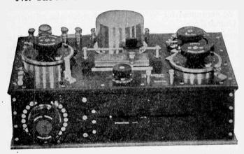
The complete circuits of the Universal Crystal Receiver are indicated in the diagram, Fig. 176, and a photograph of the finished instrument in Fig. 177, the tuner having for been designed wave lengths between 300 and 3,000 meters. The circuits are applicable to all types of crystal rectifiers, particularly those of carborundum, zincite, bornite. etc.
