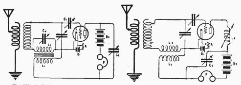
Fig. 182-Audio-Frequency Repeater Circuit. Fig. 183-Tuned Regenerative Vacuum Valve Circuit.
