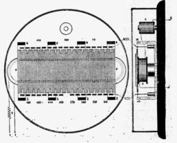
Fig. 52-Mechanism of Frequency Meter.
