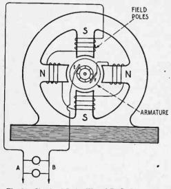
Fig. 26-Circuit of Series Wound D. C. Generator.
