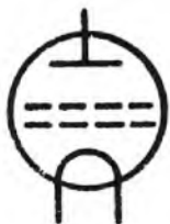
A tetrode (4 elements/filament, 2 grids & anode).
