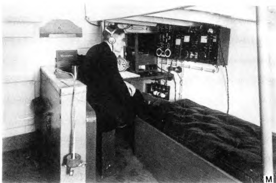
One of the original Sparks in his radio-shack. Coils, spark-gap, earphones, etc. All crude but working — plus alarm clock!
