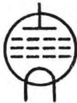
Pentode (5 elements), and so on. More grids — more sophistication/control, etc.
