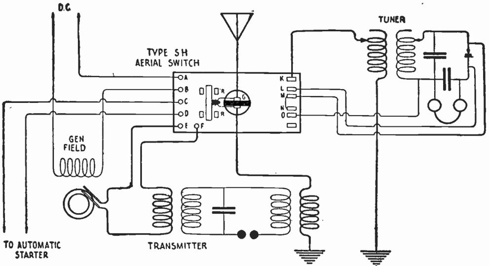
Fig. 35.—Wiring Diagram for Type "S" Antenna Switch.
