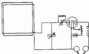
Fig. 72-A.—Diagram of Loop Aerial and Audion Detector.
