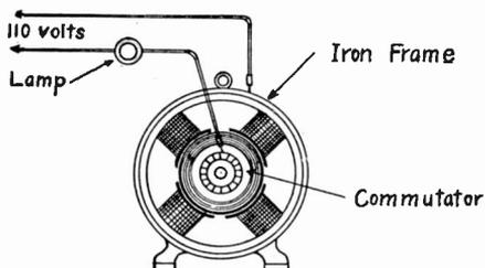
Fig. 25.—Test for Grounded Coil.
