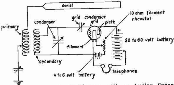
Fig. 66.—Receiving Circuit Diagram with an Audion Detector.
