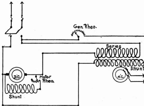
Fig. 17.—Motor Generator with Compound Generator Field Windings.
