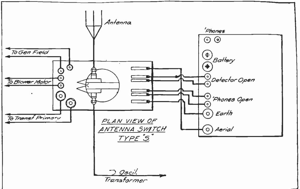
Fig. 36.—Connections of Type "S" Antenna Switch.
