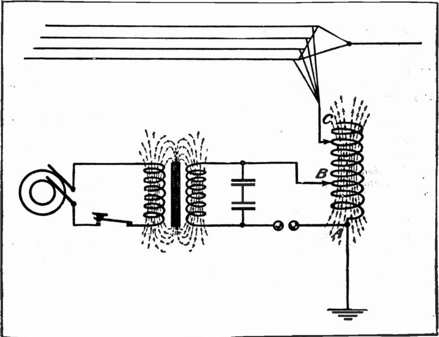
Fig. 28.—Conductively Coupled Transmitter.
