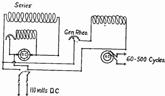
Fig. 18.—Circuits of Motor Generator with Differential Field Winding.
