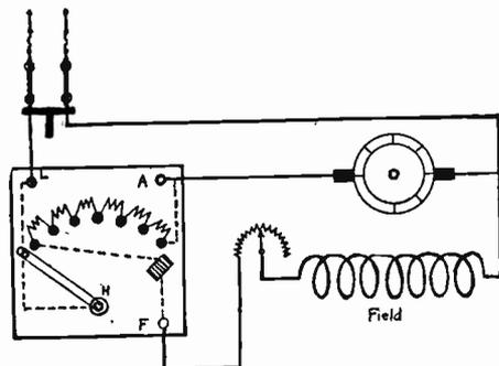
Fig. 12.—Simple Shunt Wound Motor Generator.
