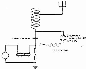
Fig. 44.—Connection of Chopper Commutator and Resistor.
