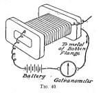
partial, and is probably caused by moisture, so that, before unwinding the coil or removing any wires, an attempt should be made to dry up any moisture by waiming the coil, and then the test should be made again in order to ascertain if there is any improvement. If the needle moves quickly to one side and gives a large deflection, the leak is caused by metallic contact and is called a 'dead earth', no amount of drying will remedy it, but the place must be sought for and a repair made.
