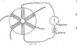
they belong. Apply the continuity test by joining one wire from the battery to the end of one coil, then, taking the free wire from the detector galvanometer in your hand, touch the bared ends of all the other coils, one at a time, as soon as the needle moves you know you have found the other end of the coil to which the battery wire is joined.
