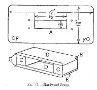
13); these may be cut out with an ordinary fret saw and finished up with a smooth file A hardwood frame is now made the end pieces C being  $1\frac{1}{2}$  by  $\frac{2}{3}$ by 5, they must be dead true and square. This is best done with file and square as if metal was being worked, thus avoiding the use of inaccurate planes and chisels. The side pieces D may be cut from thm
