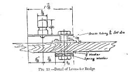
of the unknown resistance, and place the levers accordingly afterwards moving them about until no deflection of the galvanometer is observed when both keys are tapped. Then if the 20-ohm resistance be short-circuited so that the ratio arms are equal the unknown resistance will be equal to the sum of the resistances in the various incostats. If the unknown resistance be estimated at over 100 ohms, short circuit the 2 ohm resistance, making the ratio
