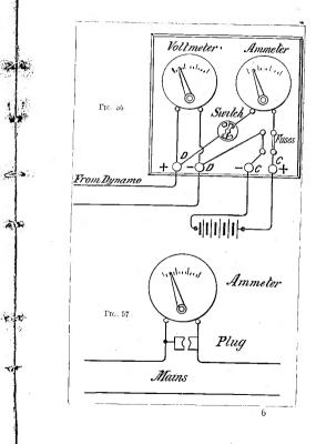
Ammeters and voltmeters must always be set so that their needles are pointing to zero before any current is passing through them  $\Lambda$  gravity-controlled instrument must be set upright—it will not indicate in any other but a vortical position, a springcontrolled instrument, on the contrary, can be used in any position (see Chapter VI) Many instruments
