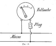
instruments, with a voltmeter the plug opens the voltmeter encouts and cuts aff all current from the instrument. Figs 57 and 58 show the connections; fig 59 shows an enlarged view of the plug and block, which consists of a pair of brass blocks drilled with a taper hole into which fits a brass plug; when the plug is pushed into the hole the five blocks are connected together, when it is taken out they are disconnected from one another.
