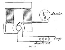
of current which the generator ought to give, and then continue the test as long as desired. When a wire resistance is used you will find that after a short time the current will fall, this may be owing to loss in the generator but it may also be caused by increase of resistance due to the passage of the current through the wire developing heat, so that before condemning the generator you should try and bring the current up to its full value again by
