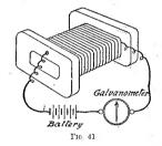
is a sign that there is no break in the wire, but if there is no movement of the needle at all it shows that the wire is broken somewhere or if there is a very slight movement it shows that the break is partial, such as might be caused by a crack through the wire. This test is termed a continuity test, and may be generally used to ascertain if encuts through switchboards, instruments, arrangements of wires for highting etc. are complete
