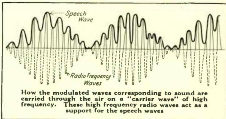
vary with the sound vibrations. Once the sounds have thus been converted into electric waves, some method must be adopted at the receiving stations to convert the electric waves back into sound waves, so that the man listening at the phones will have the words translated for him in the sender's own voice.
