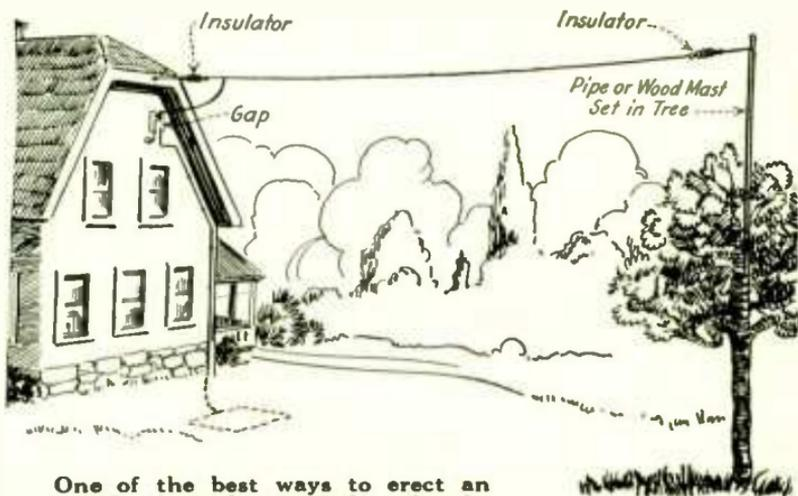
One of the best ways to erect an aerial. A single wire is best for the receiving set. Many other methods of suspension may be used, providing the wire is insulated from all objects
