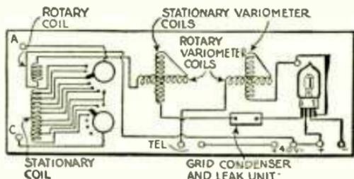
Wiring diagram for the vacuum tube outfit
