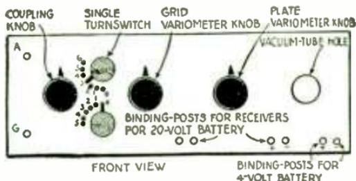
of a set. The panel may be of hard wood, fiber, hard rubber, or any of the patented compositions on sale at radio shops. Plan out the appearance of the front and then bore holes for the rods. When completed, the panel will look like the sketch above.
