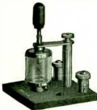
The sensitiveness of a crystal detector is seriously affected by dust, dirt and oil. The interesting detector at the left is made with a glass covering over the crystal, to protect it from these substances. The normal receiving range of such a set, properly installed and under favorable conditions, is about 10 to 25 miles
