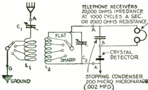
**Fig. 5—Wiring diagram of crystal detector set described in this chapter. Its receiving range is limited to 25 miles**
