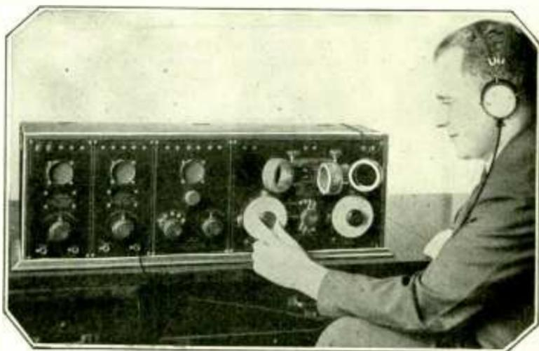
**At the upper right of this set are three honeycomb coils, which make it possible to tune in any station by substituting the proper coil. Sets of this quality cannot be bettered for the advanced amateur**
