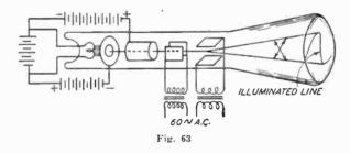
Thus, it is seen that the stream of electrons is deflected in accordance with the nature of the charge on the deflecting vanes and may be moved either upward, downward, or from side to side. It is evident then that if a charge is placed upon both sets of vanes, the stream may be directed to other positions on the fluorescent screen.
