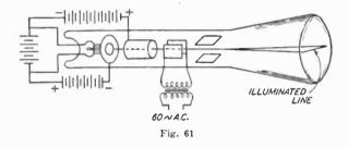
the vanes is charged positively, the other will be negative so that the electronic stream will be deflected toward the vane which has the positive charge. When the direction of flow of the current reverses and the vane that was formerly charged negatively takes a positive charge, the stream of electrons will move toward the other vane, and so on. If the alternations are impressed fast enough, the illumination on the fluorescent screen will appear as a line.
