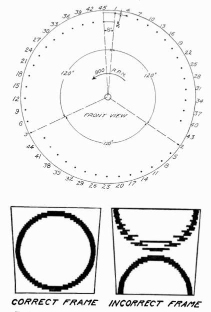
Fig. 47. (Above) Arrangement of holes in multiple-spiral disc. (Below) Illustrating the discrepancies caused by incorrect framing when three-spiral disc is used. The upper portion of the incorrectly framed picture is out of frame by approximately one-sixth revolution of the disc.
