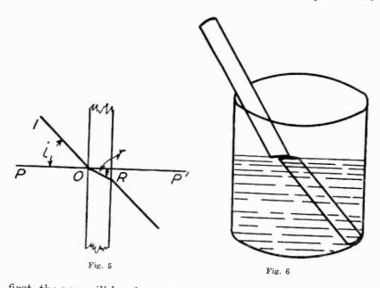
first, the ray will bend toward the perpendicular; while if the second medium has the greater density of the two, the ray will bend away from the perpendicular, the perpendicular in each instance being considered relative to the surface of the medium, otherwise known as *normal*.
