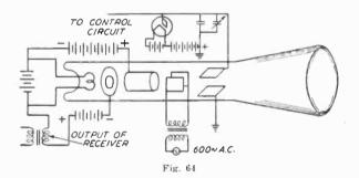
taneously when the condenser is discharged. The circuit referred to is used more or less extensively in vacuum tube relay devices and is shown graphically in Fig. 64.
