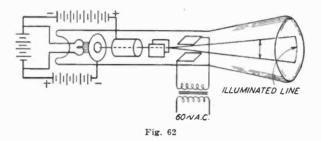
vertical deflecting vanes, as shown in Fig. 62, the illuminated line on the fluorescent screen will be vertical and, again, if the frequency of the alternations were slow enough for the eye to follow, the illumination would appear as a spot of light moving vertically on the screen.
