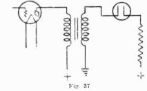
acteristic chart that accompanies the cell. One cell of commercial make, the Eveready-Raytheon Kino lamp, is specified to work with 200 volts direct current as a minimum potential.
