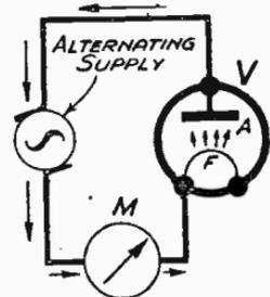
Fig. 82.— Illustrating diode acting as rectifier
