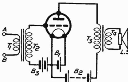
Fig. 103—Use of output transformer to match valve and speaker
