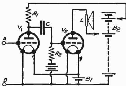
Fig. 144—A complete and practical resistance-coupled low-frequency amplifier
