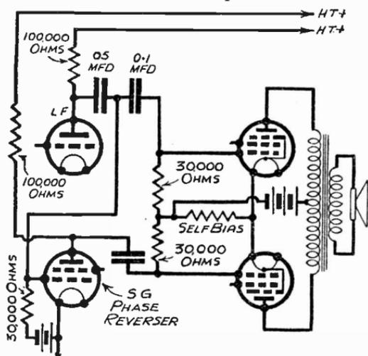
Fig. 281—Another push-pull circuit using a valve for phase reversal
