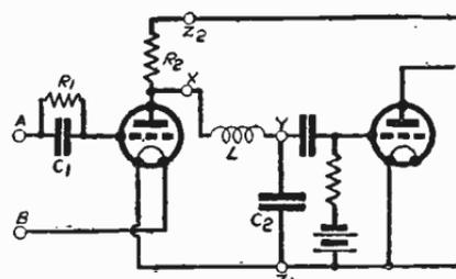
Fig. 215—Use of H.F. choke and condenser  $C_2$  to keep out H.F.
