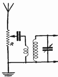
Fig. 331 — Combining series and parallel resistance
