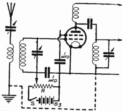
Fig. 268—Potentiometer connections for a variable-mu S.G. valve
