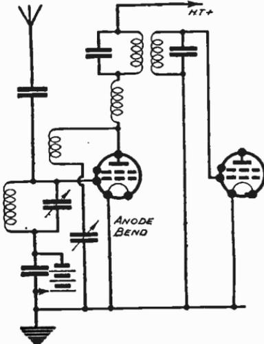
Fig. 496—Use of S.G. valve as first detector; screen connections are not shown
