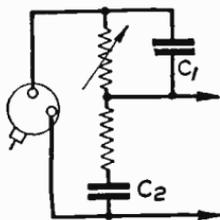
Fig. 408—Condenser  $C_1$  prevents excessive reduction of "top"
