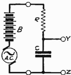
Fig. 241—Separating the A.C. from a D.C. supply
