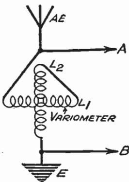
Fig. 28—A variometer gives very accurate aerial tuning
