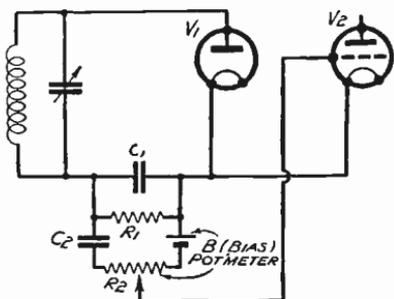
Fig. 344b—A separate potentiometer is here connected across the diode resistance
