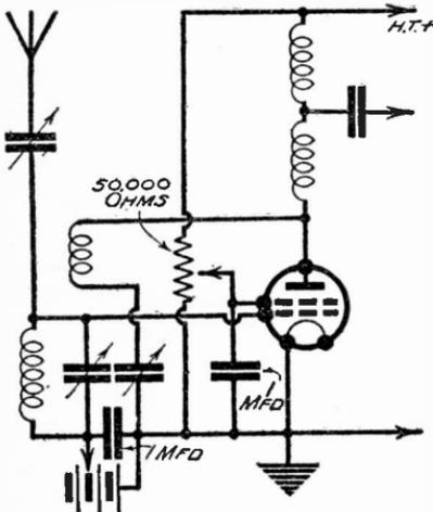
Fig. 494—Superheterodyne adaptor for wavelengths below 100 metres
