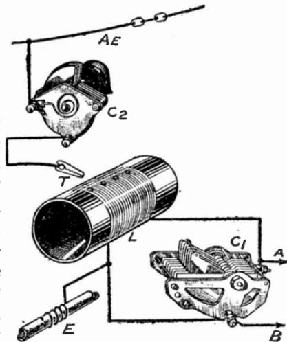
Fig. 47—Pictorial form of Fig. 45. Note solid dielectric condenser
