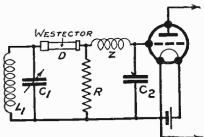
Fig. 192—The Westector—a metal rectifier—is here shown as a wireless detector
