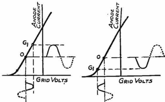
Fig. 279—Ordinary push-pull circuit operates both valves on straight part of curve
