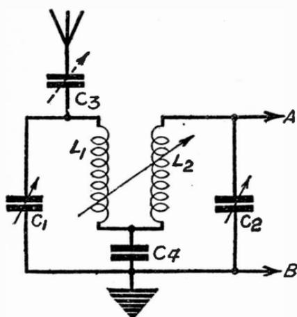
Fig. 71—Mixed band-pass filter. Transfer is by capacity and also by inductive coupling
