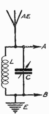
Fig. 32—Parallel aerial condenser tuning method
