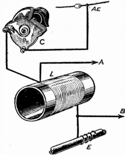
Fig. 31—A pictorial form of the circuit of Fig. 30
