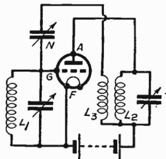
Fig. 293—Use of neutralising winding and condenser
