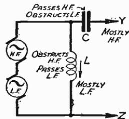
Fig. 236—Simple arrangement for filtering out low-frequency currents
