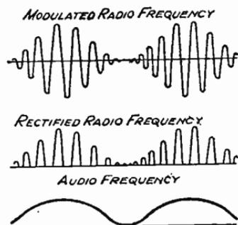
Fig. 18—To illustrate the rectification process in reception
