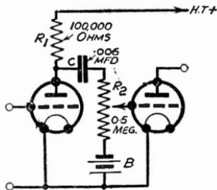
Fig. 350—Grid circuit potentiometer controls volume
