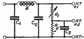
Fig. 313—The second H.T. voltage is varied by  $R_1$
