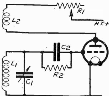
Fig. 155—The reaction is varied by an adjustable resistance in the anode circuit
