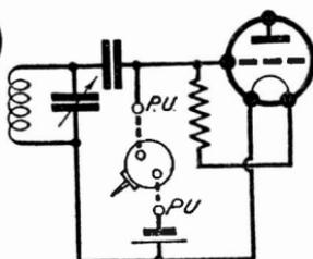
Fig. 412—Suitable for occasional use of pick-up
