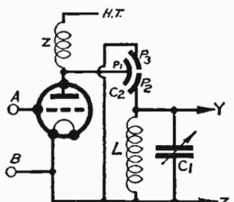
Fig. 120a—Differential anode coupling for greater selectivity and control
