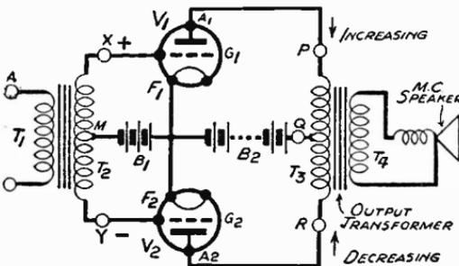
Fig. 278—Simple ordinary push-pull arrangement giving good quality
