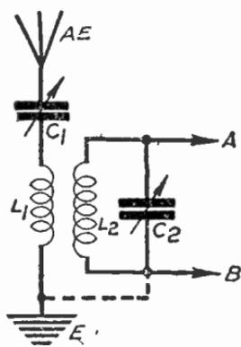
Fig. 42—Here greater selectivity is obtained by varying the feed to  $L_1$  by  $C_1$
