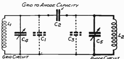
Fig. 292—Theoretical network showing valve capacities
