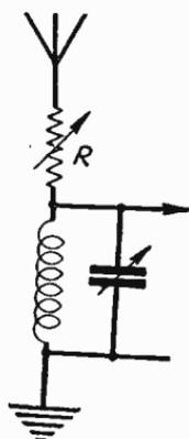
Fig. 325—Series resistance controlling volume
