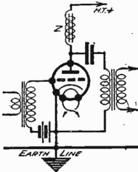
Fig. 443—Indirectly-heated cathode-valve circuit with grid-bias battery
