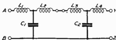
Fig. 399—A sharper cut-off is obtained by using two filters
