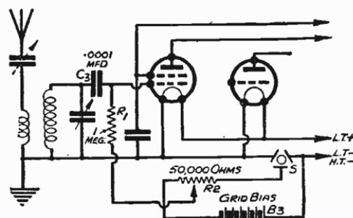
Fig. 270—Parallel system of applying bias to variable-mu valve
