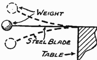
Fig. 14—A steel blade with weight oscillates, if flicked
