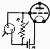
Fig. 354—Unsatisfactory method of reducing pick-up voltage
