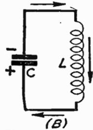
Fig. 13(b)—Condenser discharging in opposite direction
