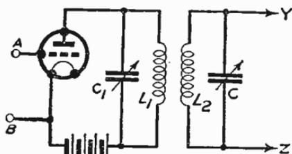
Fig. 124—Loose-coupled tuned circuits between valves give greater selectivity
