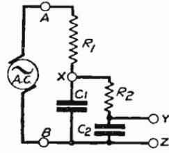
Fig. 240—Two resistance-capacity filters
