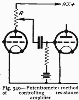
Fig. 349—Potentiometer method of controlling resistance amplifier
