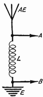
Fig. 21—Use of choke as aperiodic aerial circuit
