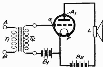
Fig. 129—The simplest form of low-frequency amplifier; note grid-bias battery  $B_1$ .
