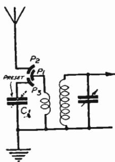
Fig. 329 — Differential condenser reduces mistuning
