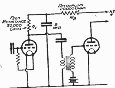
Fig. 256—How a resistance-fed transformer may be decoupled
