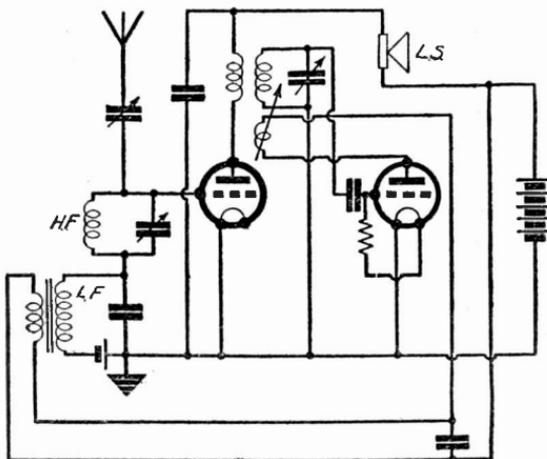
Fig. 301—Use of a valve as detector in a reflex receiver
