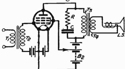
Fig. 276—Use of tone-corrector and step-down output transformer
