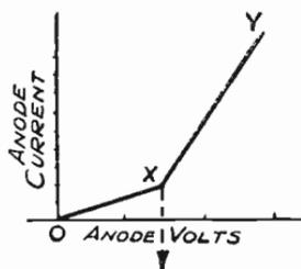
Fig. 180—An exaggerated anode current curve of diode to show rectification at bend
