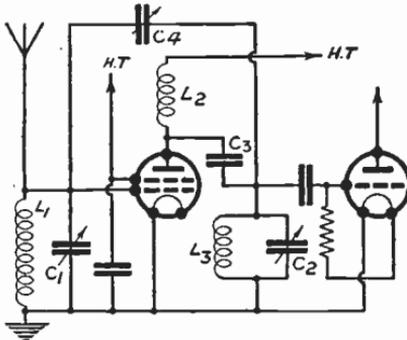
Fig. 171—Reaction may be obtained by capacity coupling between tuned anode and grid circuits
