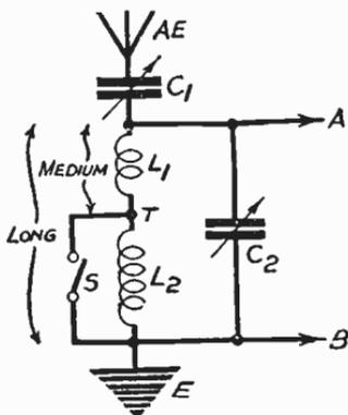
Fig. 51—A simple waveband switch which shorts the long-wave coil
