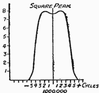
Fig. 66—Suitable coupling produces a band-pass tuning effect
