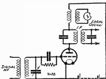
Fig. 475—Applying the anode injector system to a "leaky-grid condenser" first detector
