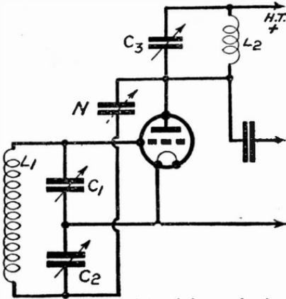
Fig. 298—A special split input circuit prevents parasitics
