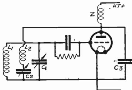
Fig. 160—A condenser  $C_3$  reduces adverse Miller effect when reaction is at zero
