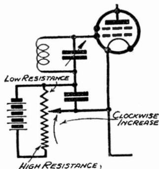
Fig. 338—Use of graded potentiometer with variable- $\mu$  S.G. valve
