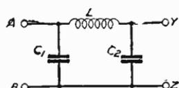
Fig. 398—An alternative symmetrical L.F. filter
