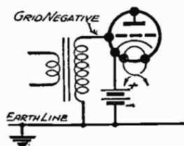
Fig. 445— Explaining how an earthed grid may be negative
