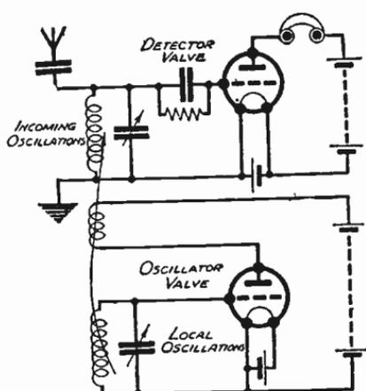
Fig. 465—A local oscillating valve heterodynes incoming continuous oscillations
