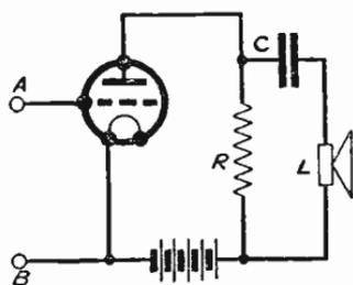
Fig. 138—Resistance-fed loudspeaker. This arrangement possesses several disadvantages
