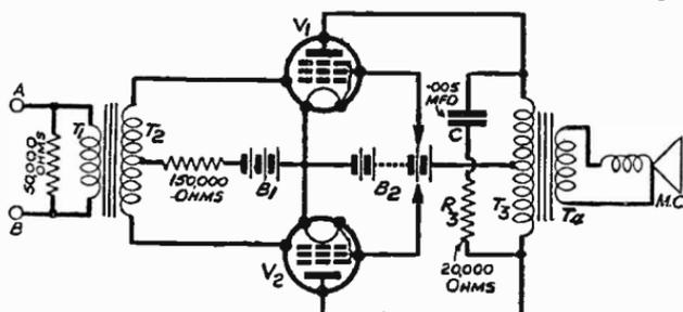
Fig. 283—Two pentodes arranged in quiescent push-pull. Matching of valves is effected by adjusting screen voltages
