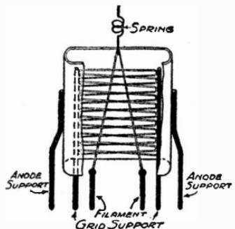
Fig. 91—A more modern construction of valve.
