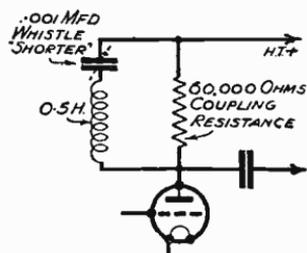
Fig. 401—A tuned acceptor circuit reduces a heterodyne whistle
