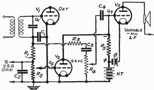
Fig. 437—A quiet A.V.C. circuit in which a separate valve cuts down the amplification of a variable-mu L.F. valve
