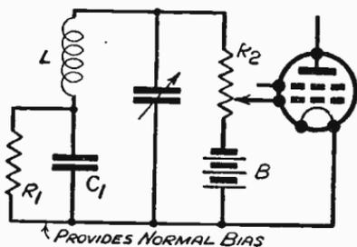
Fig. 339—Combined H.F. potentiometer and variable grid bias
