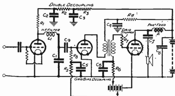
Fig. 251—Very complete deroupling is applied to both anode and grid circuits
