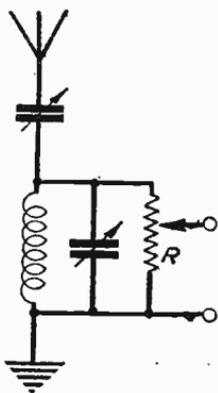
Fig. 332—Use of H.F. potentiometer to control volume
