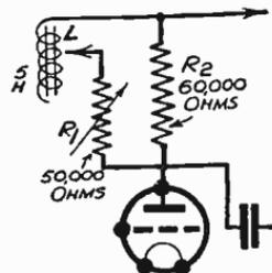
Fig. 382—Reducing the bass in a resistance amplifier
