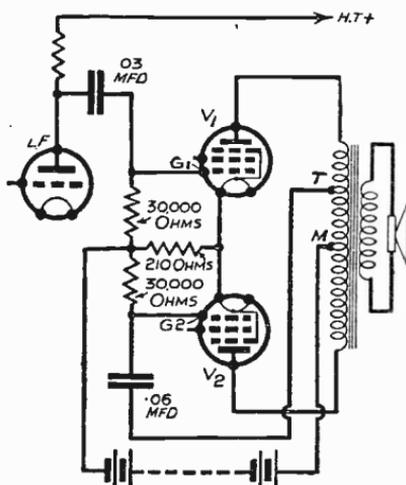
Fig. 280—Special form of push-pull circuit used in U.S.A.
