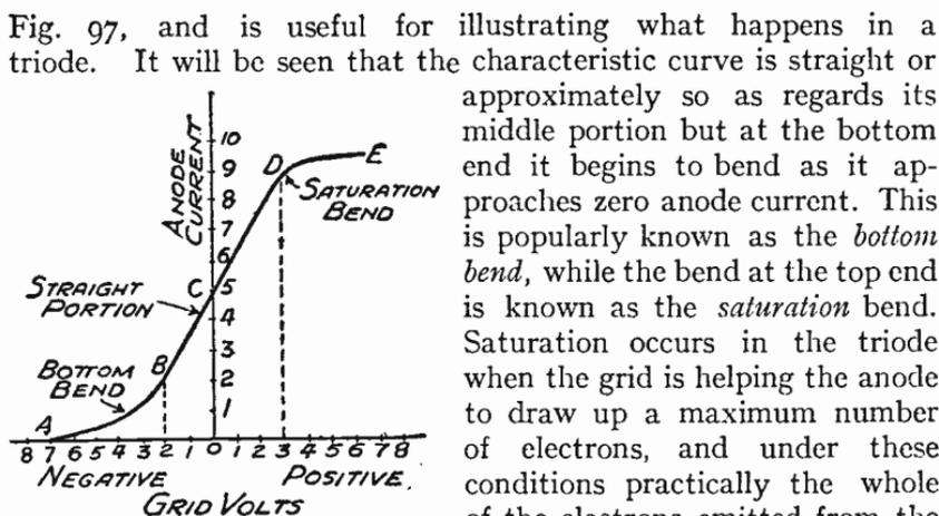
Fig. 97—Characteristic curve of a three-electrode valve
