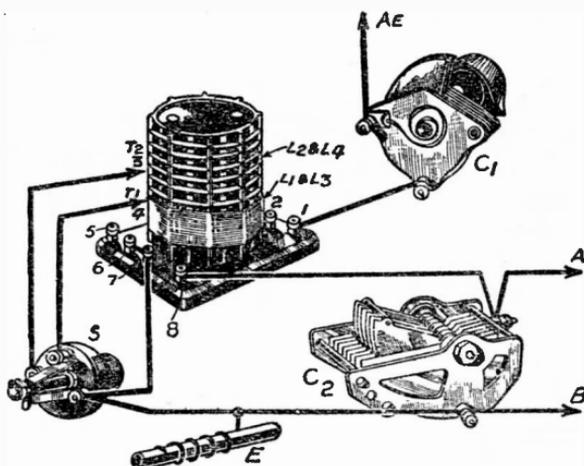
Fig. 58—The above pictorial form of Fig. 57 shows how both long-wave coils are shorted
