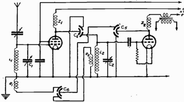
Fig. 306—A reaction distributor system is here illustrated ; reaction is applied to both tuned circuits
