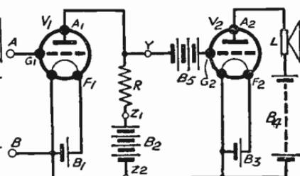
Fig. 141—Insertion of H.T. in position shown requires a grid battery B<sub>5</sub>
