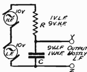
Fig. 212—Connections to give an L.F. output
