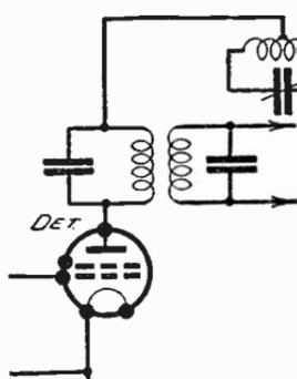
Fig. 476—The applied local oscillator voltages may be reduced by tapping the oscillator circuit
