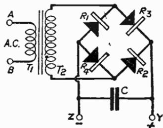
Fig. 318—Metal rectifiers arranged in bridge formation
