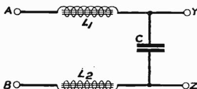
Fig. 245—Use of two L.F. chokes and one condenser for special cases
