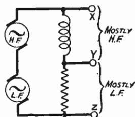
Fig. 226—Theoretical arrangement of inductance-resistance filter
