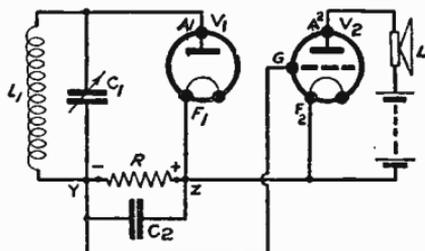
Fig. 181—The L.F. potentials across  $R$  are passed on to the L.F. valve
