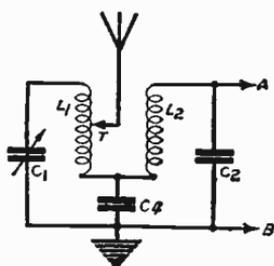
Fig. 68—Capacity-coupled band-pass with tapped aerial coil
