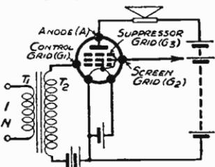
Fig. 272—Suppressor gr.d prevents negative resistance
