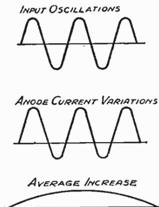
Fig. 198—An approximate graphical representation of anode-bend detection
