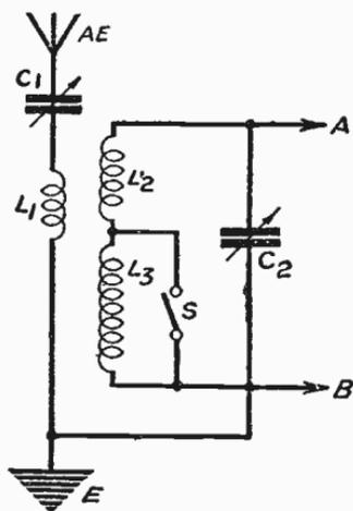
Fig. 59—An aperiodic-coupled circuit with wave-change switch
