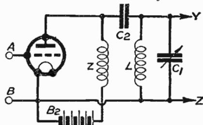
Fig. 117—A practical arrangement which employs an H.F. choke feed system
