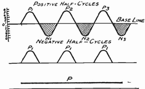
Fig. 176—Graphical representation of the rectification process; only positive half-cycles pass
