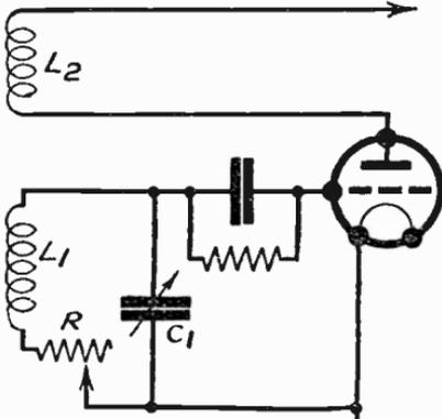
Fig. 168—Excessive fixed reaction is reduced by a resistance
