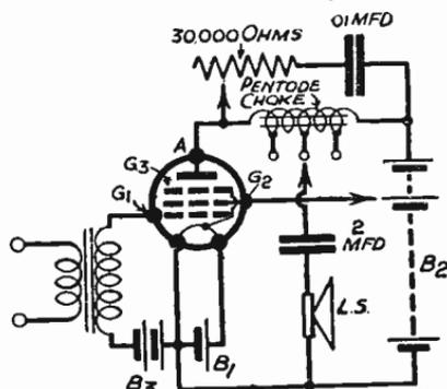
Fig. 275—Tone-corrector circuit applied to output choke
