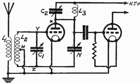
In Fig. 296, the opposing e.m.fs. are fed from the anode of the H.F. valve,
