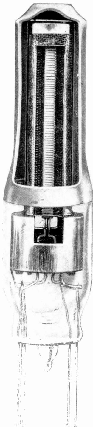
SHOWING CONSTRUCTION OF CATKIN VALVE FOR RECEPTION
