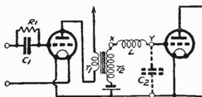
Fig. 221—Showing use of choke as a means of filtering out H.F.
