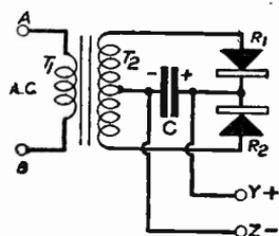
Fig. 317—A full-wave metal rectifier system
