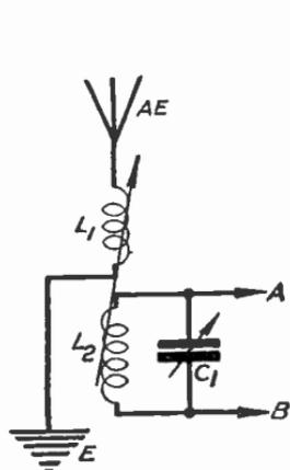
Fig. 40—Variable coupling is effected by moving the aerial coil
