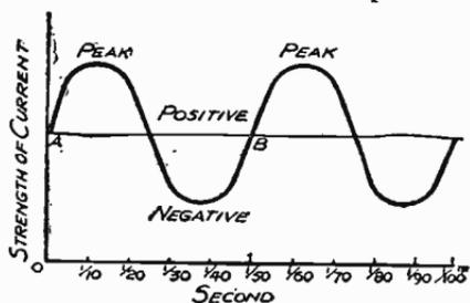
Fig. 6—Two complete cycles of alternating current. The inverted peaks are negative current
