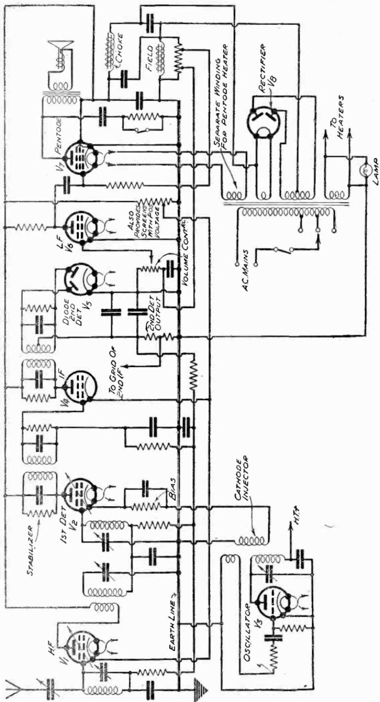
Fig. 503.—The general arrangement of the Murphy A.8 receiver. Note the band-pass arrangement between the first two valves and the automatic volume control circuit
