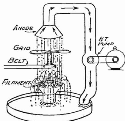
Fig. 98—A mechanical analogy to explain the action of the triode
