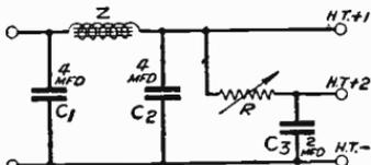
Fig. 311—Use of dropping resistance to provide extra H.T. terminal
