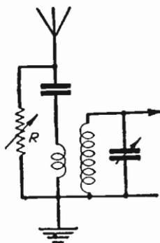
Fig. 330 — Parallel resistance reduces signal strength
