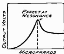
Fig. 388—Resonance increases the bass response
