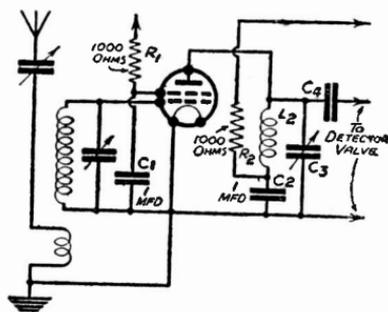
Fig. 264—This improvement keeps one side of C3 at earth potential
