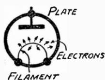
Fig. 77—Showing the introduction of a metal plate
