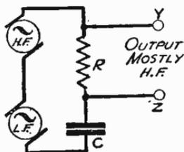
Fig. 213—The same circuit with H.F. output
