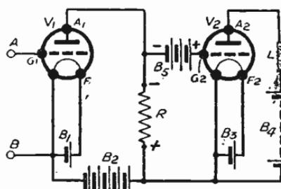
Fig. 140—Use of battery B<sub>5</sub> to prevent excessive negative grid voltage
