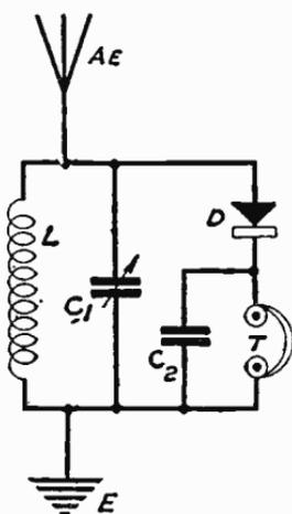
Fig. 16 (a)—A simple crystal-detector receiver
