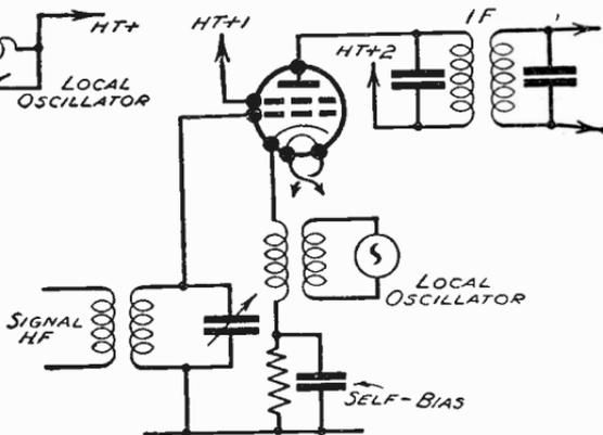
Fig. 477—The cathode injector system which is commonly used in mains valve superheterodynes
