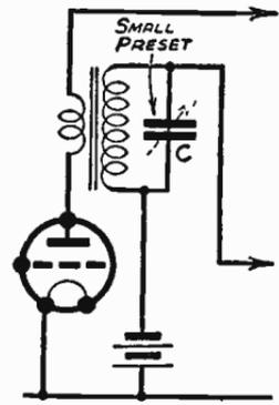
Fig. 376—Reducing treble by condenser across secondary
