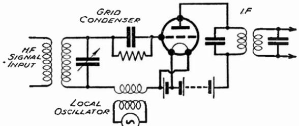
Fig. 473—Application of the grid injector system to a "first detector" operating with grid condenser and leak
