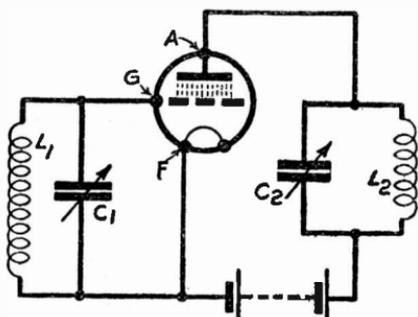
Fig. 291—Capacity coupling inside triode promotes self-oscillation
