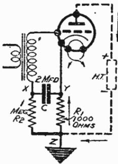
Fig. 446 — Decoupling the self-bias resistance
