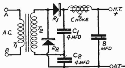
Fig. 319—The most usual arrangement involves voltage doubling
