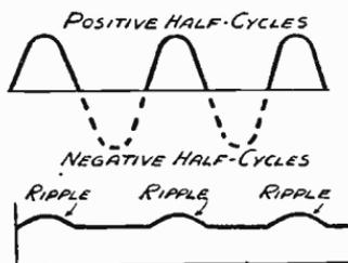
Fig. 308—This illustrates the A.C. ripple obtained with half-wave rectification
