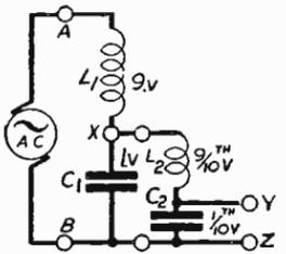
Fig. 239—Use of two filters in series
