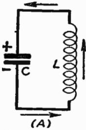
Fig. 13(a)—Condenser discharging through an inductance
