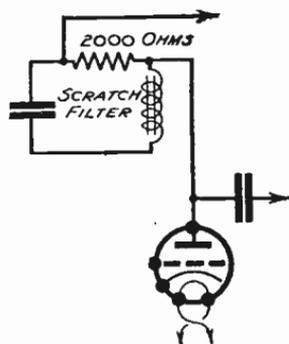
Fig. 491—A change of connections provides a scratch filter but poorer amplification
