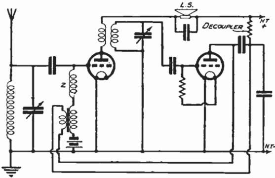
Fig. 302—Another reflex receiver in which, however, the L.F. is fed to the first grid by a parallel circuit
