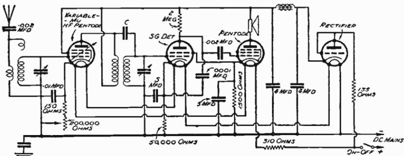
Fig. 463—Simple American universal receiver which can be connected to D.C. or A.C. mains. On D.C. the rectifier valve acts simply as a resistance
