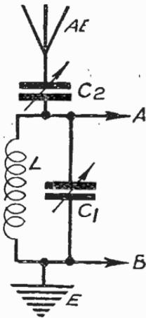
Fig. 34—Use of a small series condenser
