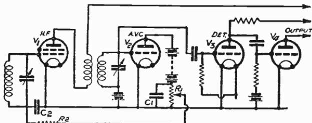
Fig. 427—The A.V.C. valve operates as an anode-bend rectifier and is separate from the detector
