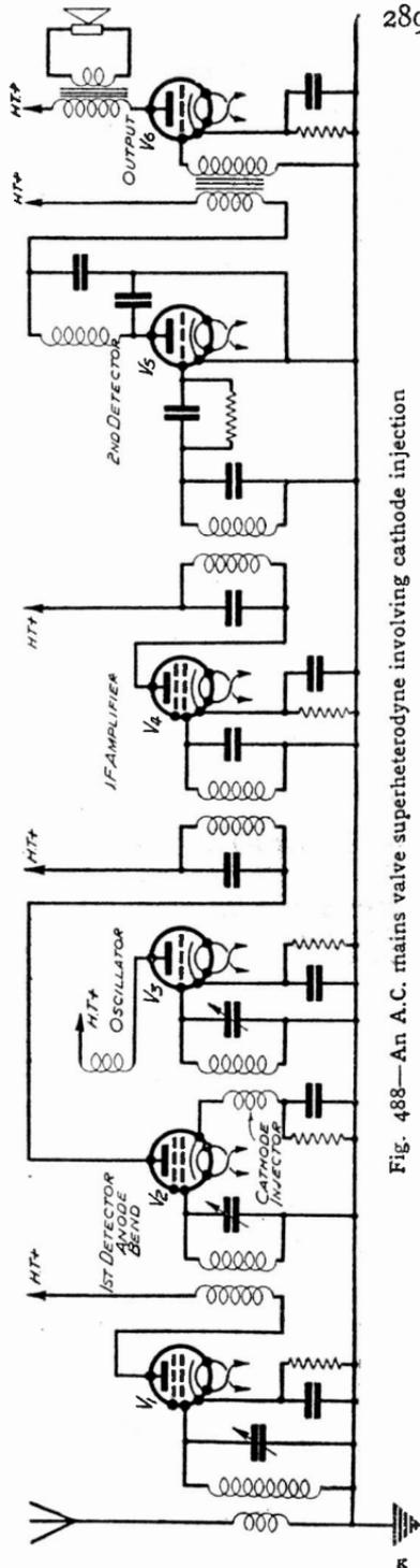
Fig. 488—An A.C. mains valve superheterodyne involving cathode injection
