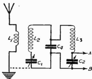
Fig. 69—Here the capacity-coupled band-pass circuit is supplemented by aperiodic aerial coupling
