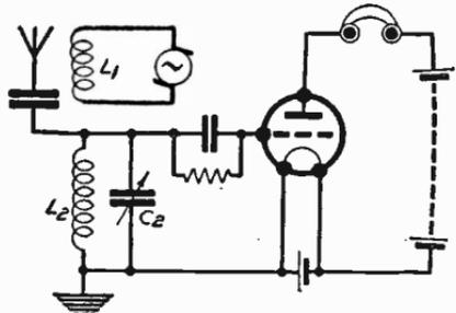
Fig. 464—A heterodyne receiver for the reception of continuous wave Morse
