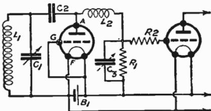
Fig. 187—Another diode detector circuit with H.F. choke and grid stopper
