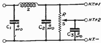
Fig. 312—Use of potentiometer to provide a second H.T. voltage
