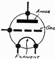
Fig. 88—Method of indicating a three-electrode valve
