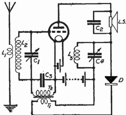
Fig. 300—Crystal detector reflex receiver giving double amplification
