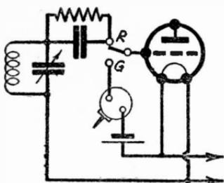
Fig. 414—Change-over radiogram switching system
