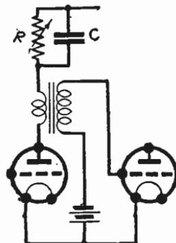
Fig. 351—Anode voltage variation may reduce volume; not a good method
