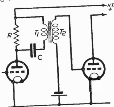
Fig. 258—This connection reduces interaction and hum
