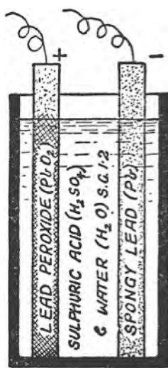
FIG. 19.—State of cell when charged.
