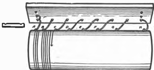
FIGS. 356 and 357.—(Left) Details of the "Jockey," and (Right) the Former on which the Resistance is wound.
