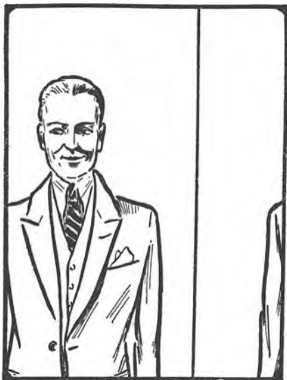
FIG. 418.—The image split vertically, due to the synchronising mechanism pulling the disc into place when its holes are out of phase with those at the transmitting end.
