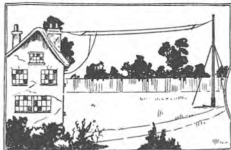
TWIN "L" TYPE AERIAL WITH WOODEN SPREADERS.
