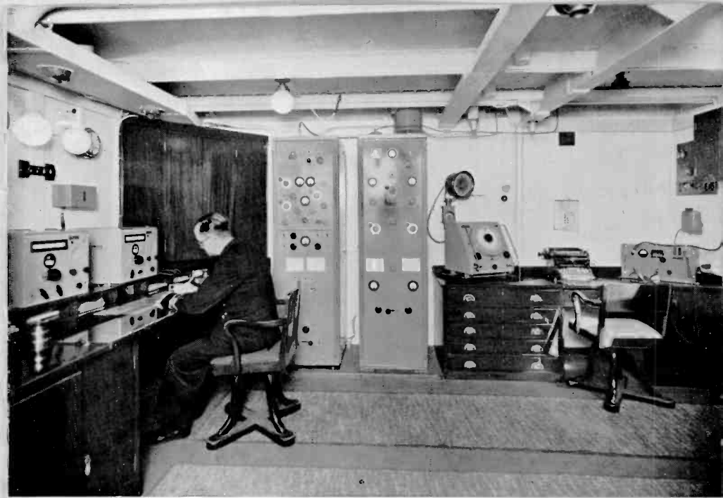
The Radio room of R.M.S. 'Orion' showing, left to right, two Marconi 'Yeoman' receivers, 'Worldspan' transmitter, 'Lodestone' direction finder, and Marconi broadcast receiver
