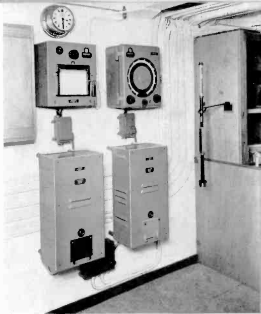
left: The Marconi 'Oceanic' sound reproducing equipment, fitted in a passenger ship. It can be used to provide music for dancing, orchestral music, talks, and ship's announcements
