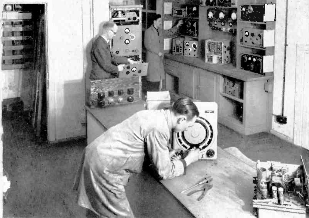
The Repair Shop in Marconi House, St. Vincent Street, Glasgow. Testing gear mounted in racks facilitates the overhauling of equipment
