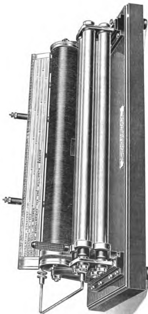
FIG. 10.—A Cymometer for measuring Wave Lengths up to 10,000 Feet.
