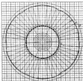
*Enclosed for copper loss in individual coils. Copper coil represented by radius vector measured between C' and a'. Area between C' and a' represents total heating. Area between C' and B' represents D.C. heating same output.*
