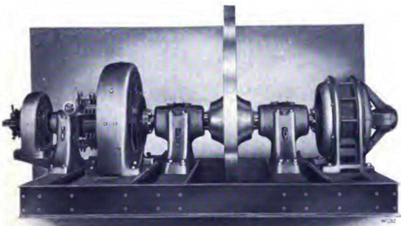
Flywheel Motor-Generator Set for Mine Hoist
