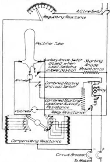
Fig. 4. Diagram of Connections
