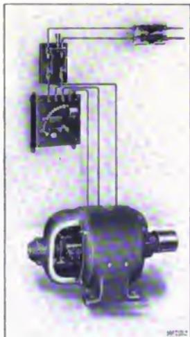
A 10 H.P. MOTOR WITH GENERAL ELECTRIC STANDARD RHEDSTAT SWITCH AND FUSES
