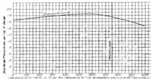
Pressure Curve of Centrifugal Compressor for Different Loads
