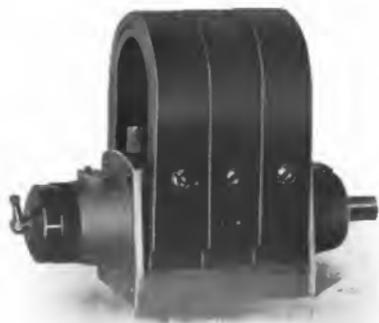
Fig. 1. Low Tension Magneto
