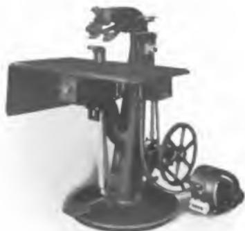
Fig. 8 Paging and numbering machine operated by a one-eighth horsepower motor. This motor is stopped and started by means of the snap switch shown at the side of the machine head
