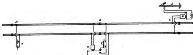
Fig. 12. Track Circuit with Cut Section
