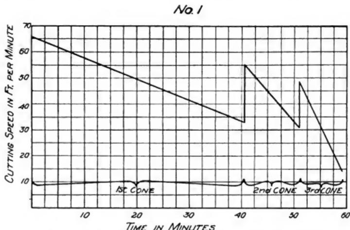
Fig. 1. Cutting Speeds and Time Required to Face a 72-inch Cast Iron Disk Using Three Steps on the Cone Pulley
