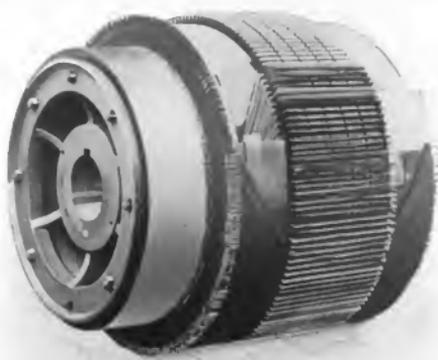
Fig. 3. Armature Partly Wound
