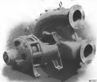
Centrifugal Compressor Driven by 11 h.p. Induction Motor
