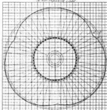
Area for copper loss in individual coils (loss per coil represented by radius vector measured between C and D)
