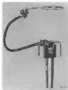
Fig. 3. Upper Carbon Holder, Cable and Terminal
