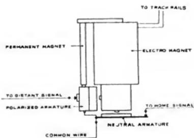
Fig. 3. Diagram of Polarized Relay
