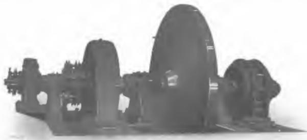
Fig. 3. Flywheel Motor-Generator Set for Mine Hoist
