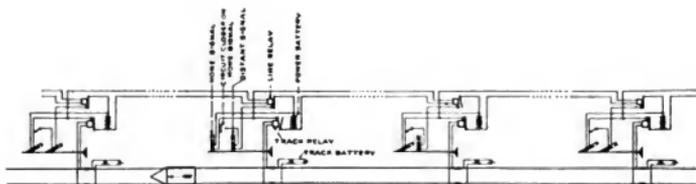
Fig. 1. Circuits for Home and Distant Signals with Line Relay
