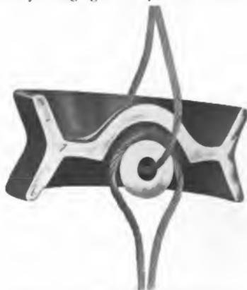
Fig. 3. Cross Section of Link Strain Insulator
