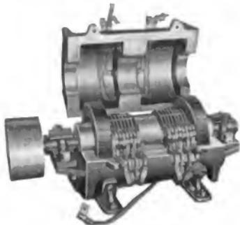
Fig. 1. Unipolar Dynamo
