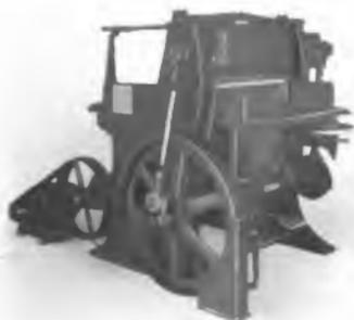
Fig. 7 Thirty-eight inch paper cutter, driven by a standard compound wound motor, the controller being situated directly beneath the feed board
