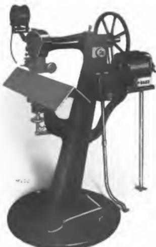
Fig. 13. Wire stitchee operated by a one-eighth horse-power motor. This motor is started and stopped by means of a snap switch in a similar manner to the one driving the numbering machine.
