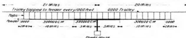
Fig. 1. Diagram Showing Arrangement of Feeders
