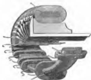
Fig. 5. Gramme Ring Showing Core Made Up of Iron Wire
