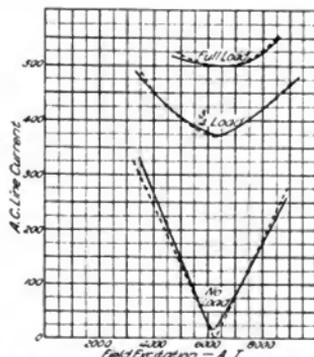
Fig. 18. Phase-Characteristic of 300 Kw. Rotary Converter
