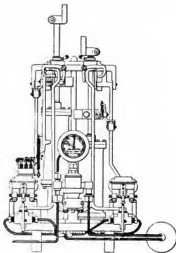
Fig. 7. Elevation of Two-arm Electro-gas Signal
