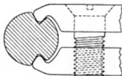
Fig. 5. Suspension for Grooved Trolley Wire
