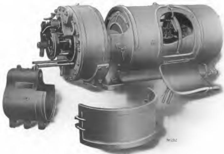
Fig. 1. 20 kw. Curtis Turbine Set—Locomotive Type
