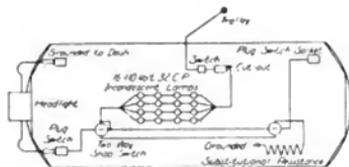
Fig. 3. Diagram of Car and Headlight Wiring
