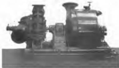
Fig. 5. Turbine Driven Pump for New York City Fire Boat
