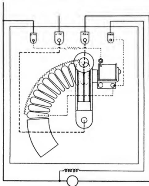
Connection Diagram for Type SA Rheostat
