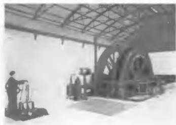
Fig. 3. Induction Motor Hoisting Engine at Pit Preussen II
