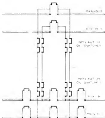
Fig. 2. High Tension Connections between Waterside Stations, New York Edison System
