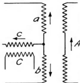
because such an arrangement would introduce a large leakage flux, the effect of which is to increase the reactance of the transformer. The primary and secondary coils are always placed as near together as good insulation permits in order to reduce to a minimum the flux which does not link both coils.
