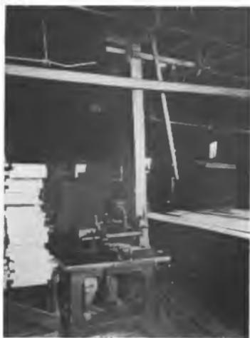
Fig. 2. Automatic Rip Saw, Belt Driven
