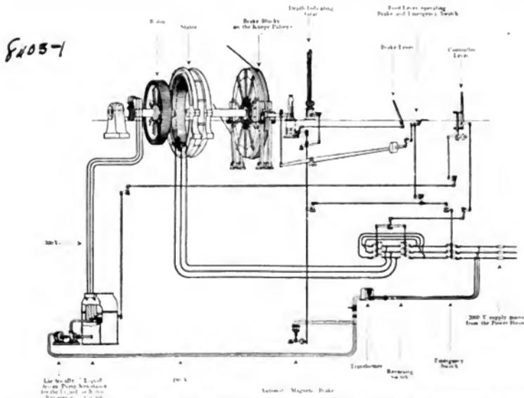
Diagram showing patented arrangement of Electrical Winding Plant as installed at "Fruessen II" Coal Mine, by the Allgemeine Electricitäts-Gesellschaft, Berlin.
