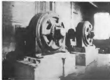
Fig. 8. 2-1-18-100-156 2 3-K-440 volt motors direct connected to countershaft of raw material tube mills through six arm flexible couplings, in Universal Portland Cement Co., Plant No. 4. These motors were started four months ago and have run continuously ever since without any shut down
