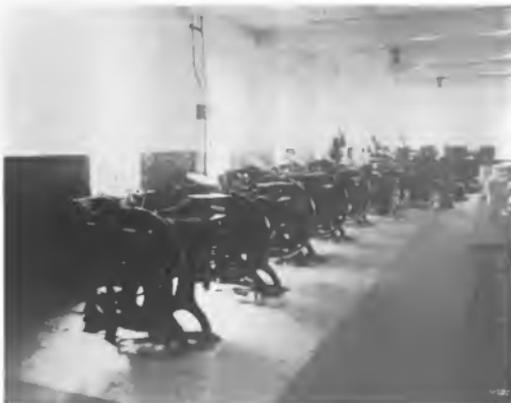
Fig. 12. Row of Gordon Job Presses driven by Individual Motors
