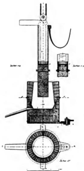
Fig. 11. Experimental Electric Furnace
