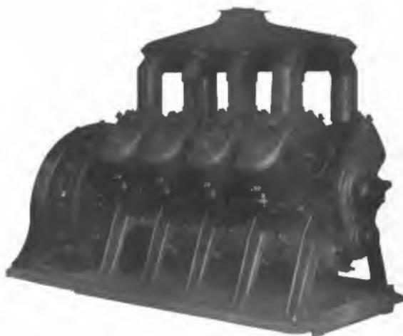
Fig. 3. GE-8-100 125-550 Gasolene Motor
