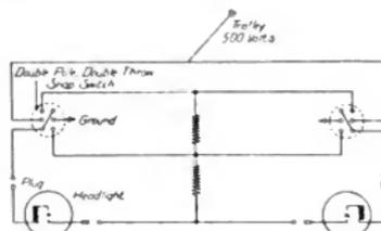
Fig. 4. Reversing Switch and Wiring
