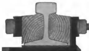
Fig. 5. Insulated Section
