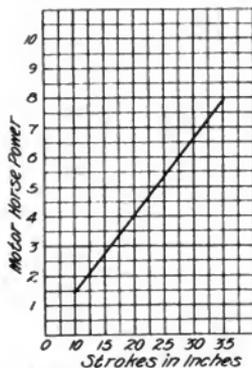
Fig. 2. Shaper 15 to 20 Ft. per Min.
