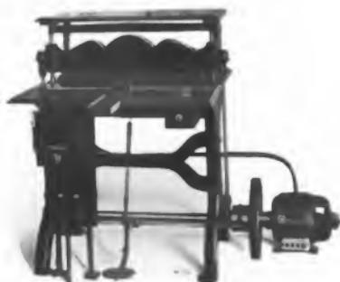
Fig. 9 Perforator driven by a one-half horsepower motor, the controller being situated directly beneath the feed board
