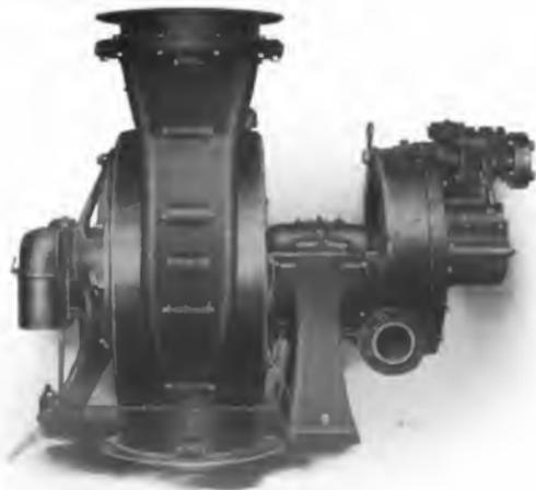
Fig. 1. Curtis Turbine Driven Air Compressor
