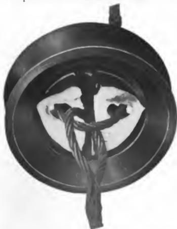
Fig. 4. Link Strain Insulator which has been broken under a load of five tons.
