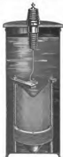
Fig. 6. One Phase Leg of a Gap Aluminum Arrester, Showing the Form of the Cones, Method of Holding them Apart, and the Position of the Electrolyte, Oil, and Tank
