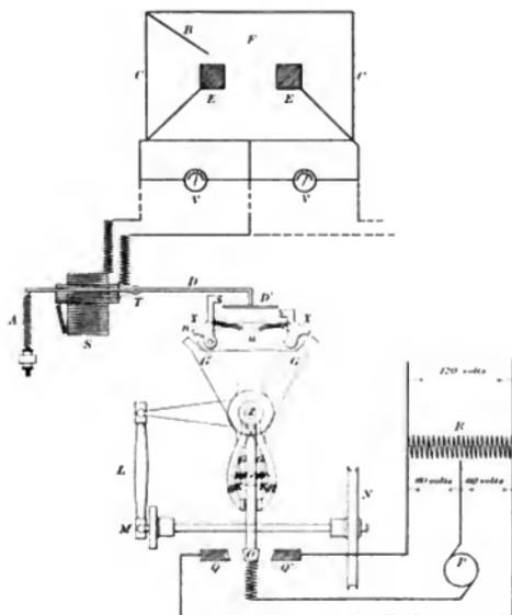
Fig. 2. Diagram of Automatic Regulator for Heroult Furnace
