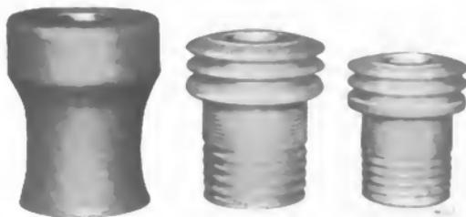
Fig. 5. Green Porcelain Blank; Same Cut to Shape; Machined Porcelain after Firing
