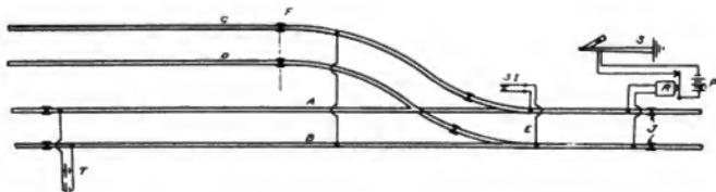
Fig. 3. Elementary Track Circuit
