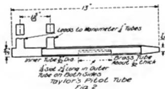
tests. This consists of an inner tube open toward the approaching air and closed at the back end, but provided with a branch leading to a manometer. The outside tube is closed at both ends, but provided with slits in the side and a branch leading to another manometer. The inner tube measures the total impact pressure of the air, which consists of its velocity head and the static pressure; the outside tube is assumed to measure the static pressure only.
