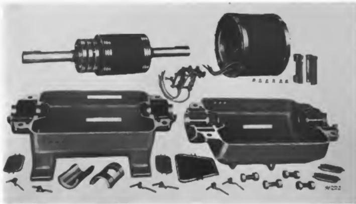
Fig. 3. Exploded View of MI-107, 75 H.P. Motor
