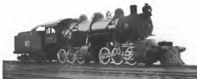
Fig. 2. Articulated Type of Freight Locomotive. Twelve Drivers. Weight of Engine 206,000 lbs.; Weight of Tender 90,000 lbs. Tractive Effort, 42,400 lbs.
