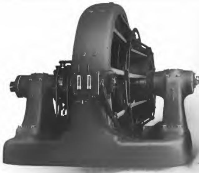
Fig. 2. 10 Pole, 1500 Kw., 300 R.P.M., 575 Volt Six-Phase Rotary Converter
