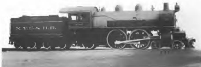
Fig. 1. Atlantic Type of Passenger Engine. Weight of Engine 200,000 lbs.;
