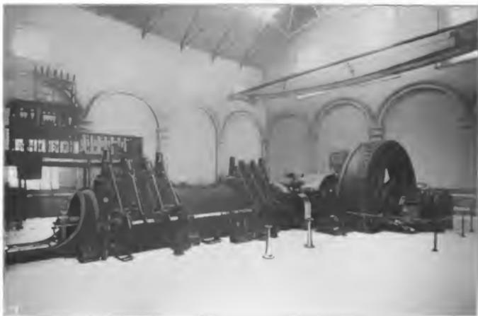
1200 H. P. Nürnberg Double-Acting Single Tandem Gas Engine Driving 825 Kw.
