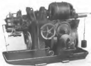
Fig. 2. Gridley Lathe. Front View showing Feed Motor
