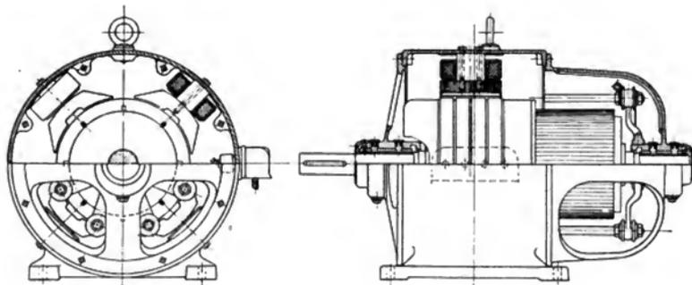
Fig. 6. Sectional Elevation of a Series-Excited Rosenberg Generator Designed for Welding Purposes
