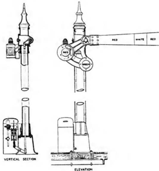
Fig. 5. Electro-pneumatic Semaphore
