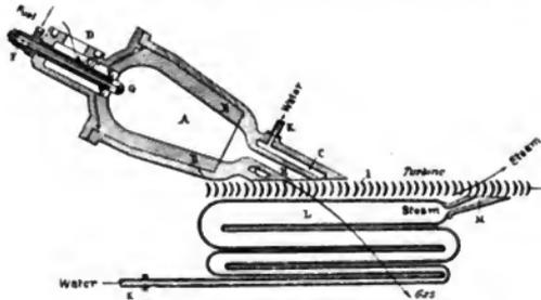
Fig. 6. Mixed Gas and Steam Turbine
