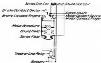
Fig. 11. Diagram of Connections, Type M-113 Signal
