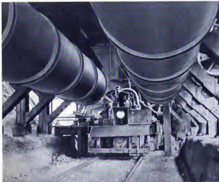
Motor-Driven Scale Car, Operating Under Ore and Limestone Pockets
