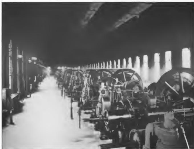
8-1000 Kw. Gas Engines in the Power Plant of the Lackawanna Steel Co.
