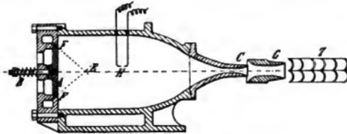
General Arrangement of Explosion Gas Turbine
