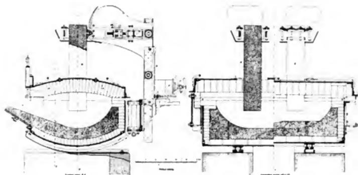
Fig. 1. Heroult Steel Furnace
