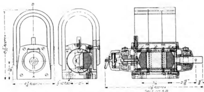
Fig. 3. Elevation and Cross Sections of Magneto
