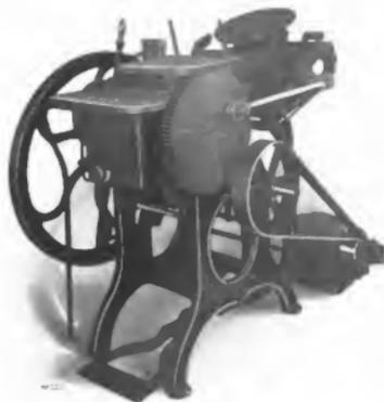
Fig. 1. Gordon Job Press driven by 1 4 h. p. motor.
