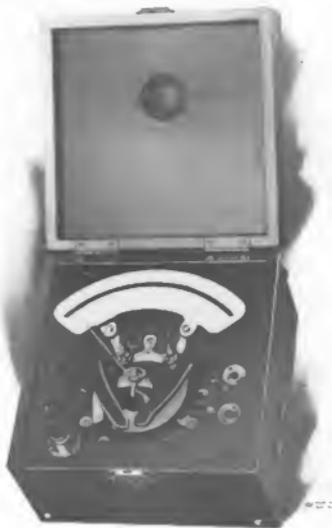
Type P-3 Portable Wattmeter with Cover Removed
