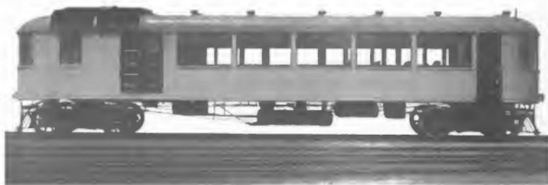
Fig. 1. Gas-Electric Car
