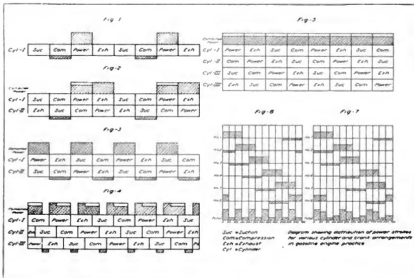
the relation of events in four-cycle engines having cylinders and cranks arranged according to the more usual practice met in explosion-engine design. No attempt is made to show the variation of pressure during the several strokes, but each is represented by a rectangle. The sectioned rectangles above the lines represent positive or useful work, while those below show negative effort in compressing the charge of vapor. Explosion strokes are indicated by
