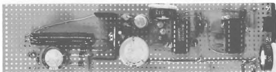
Figure 6-2. Step-Down Switching Power Supply +12V to +5V
