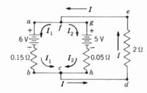
Fig. 22 • 15 Circuit of Example 4 Labeled with Known Values
