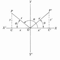
Fig.  $25 \cdot 1$   $\theta$  and  $\phi$  Are Supplementary Angles;  $\theta + \phi = 180^{\circ}$
