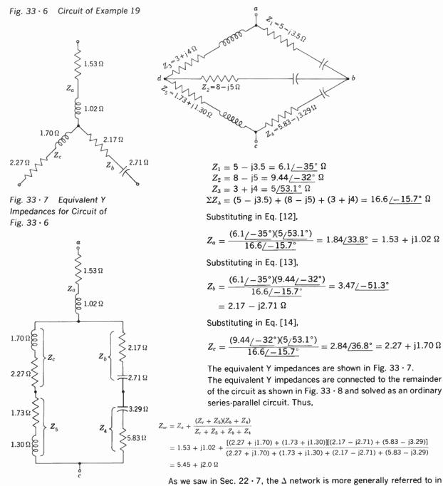
Fig. 33 · 8 Equivalent Y Impedances Connected to Remainder of Circuit of Fig. 33 · 6 As we saw in Sec. 22  $\cdot$  7, the  $\Delta$  network is more generally referred to in electronics as a  $\pi$  network and the Y or star network is often known as the T network. In the problems which follow, the two sets of expressions are used interchangeably.
