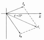
Fig.  $32 \cdot 21$  I<sub>1</sub> Is the Phasor Sum of I<sub>a</sub> and I<sub>b</sub>
