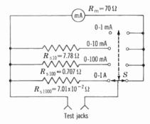
Fig. 14 · 8 Method of Switching Shunts
