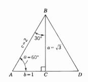
Fig. 24 · 3 Equilateral Triangle Divided into Two Equal 30°-60°-90° Right Triangles
