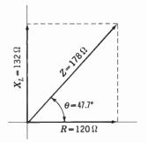
Fig. 31 · 17 Impedance Phasor Diagram for Circuit of Example 9
