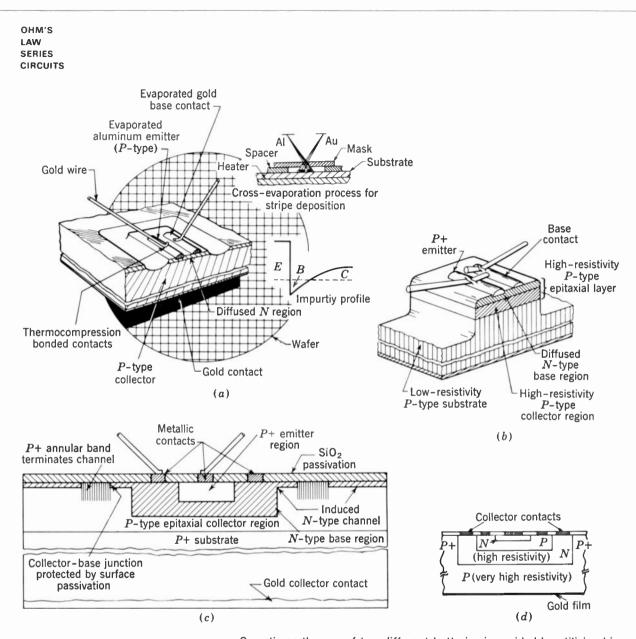
Fig. 8 · 26 Evolution of Transistors (Courtesy of Lothar Stern, "Fundamentals of Integrated Circuits," Hayden Book Co., Inc., 1968)
