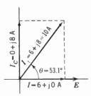
Fig.  $32 \cdot 11$  Phasor Diagram for Circuit of Fig.  $32 \cdot 10$
