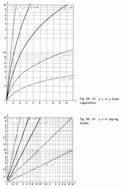
Now, in Fig.  $38 \cdot 15$ , see how the curves, of varying steepness, diverge from the point (1,1) when the *y* values are plotted logarithmically. Then, in Fig.  $38 \cdot 16$ , see how the divergent *curves* of Fig.  $38 \cdot 14$  become divergent *straight lines* emerging from the point (1,1) with their steepness proportional to the power *a*.
