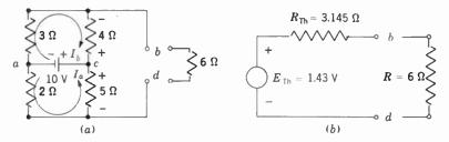
Fig. 22 · 37a Redrawn from Fig. 22 · 24 for Thevenin's Solution of Current Is Through Resistor Across Points bd
