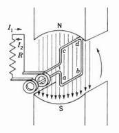
Fig. 30 · 1 Representation of Elementary Alternator
