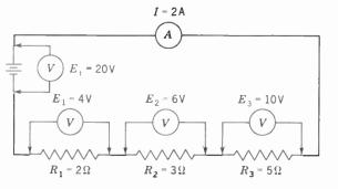
Fig. 8 • 13 Schematic Diagram of the Circuit Represented in Fig. 8 · 12
