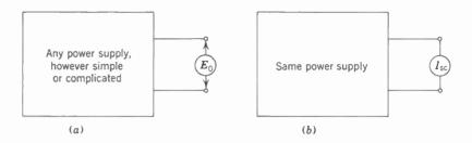
urement of the open-circuit EMF which the power supply generates. And an ammeter with very low resistance can make a reasonable measurement of the short-circuit current which the power supply can deliver. Two such models of power supplies are available to us:
