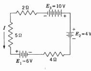
Fig. 22 · 3 Circuit of Example 1
