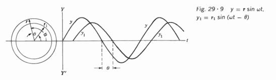
angle  $\theta$ . The phase angle between the two curves is  $\theta$ , but in this case,  $y_1$  lags y. Hence the equation for the curve generated by  $r_1$  is
