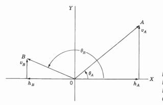
Fig. 28 · 19 Summation of Nonrectangular Phasors By Resolution into Rectangular Components
