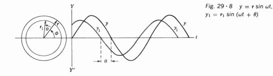
When t = 0, r starts from the horizontal axis to generate the curve  $y = r \sin \omega t$ . At the same time,  $r_1$  is ahead of r by an angle  $\theta$ ; hence,  $r_1$  generates the curve  $y_1 = r_1 \sin (\omega t + \theta)$ . It will be noted that this *displaces* the  $y_1$  curve along the horizontal by an angle  $\theta$  as shown in the figure.
