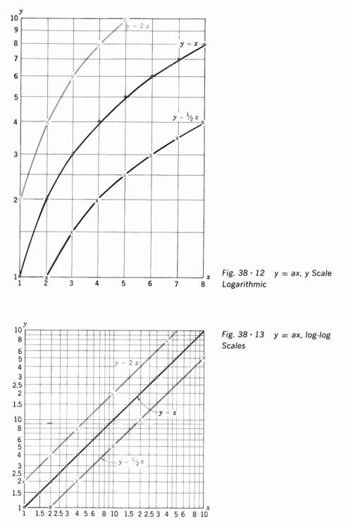
*y* values are plotted logarithmically (Fig.  $38 \cdot 12$ ). Notice the spacing of the *y* dimensions like a slide rule scale, the distances between 1 and 2, 2 and 3, etc., being logarithmically divided. Observe that what were straight lines now appear curved and that the amount of curvature will vary according to the horizontal scale used. The lines still appear to converge to some lower-left origin, but their divergence to the upper right is less pronounced than in Fig.  $38 \cdot 11$ .
