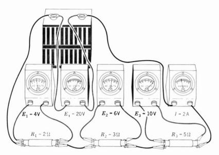
Fig.  $8 \cdot 12$  Three Resistors Connected in Series with a Voltmeter Connected across Each Resistor. The Sum of the Voltages across the Resistors is Equal to the Battery Voltage
