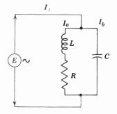
Fig. 32 · 31 Parallel LC Circuit R Represents Effective Resistance of L.
