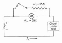
Fig.  $14 \cdot 4$  Total Current I<sub>1</sub> Flows through The Milliammeter, Which Indicates a Full-Scale Deflection of 1 mA.
