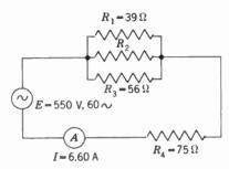
Fig. 31 · 4 Circuit of Probs. 2 and 3
