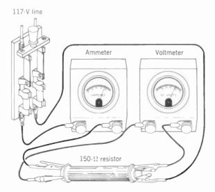
Fig. 8 · 1 Sketch of the Circuit of Example 1 Showing How the Parts Are Connected to Form the Circuit
