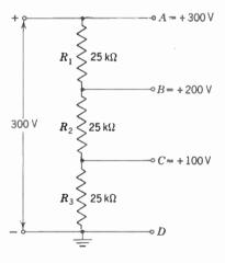
Fig. 15 • 1 Voltage Divider Consisting of Three 25·kΩ Resistors Connected Across 300-V Power Supply
