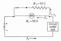
Fig. 14 · 5 Total Current I<sub>t</sub> Divides Equally between Meter Resistance  $R_m$  and Shunt Resistance  $R_s$ .  $I_t = I_m + I_s = 1 \text{ mA and}$  $I_s = I_m = 0.5 \text{ mA}.$
