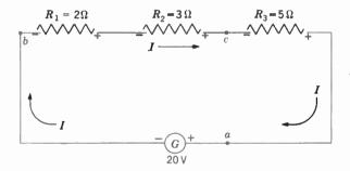
Fig. 22 · 2 The Sum of the Voltage Drops across the Resistors Is Equal to the Applied EMF.
