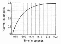
Fig.  $34 \cdot 3$  Graph of Current in RL Circuit of Prob. 28
