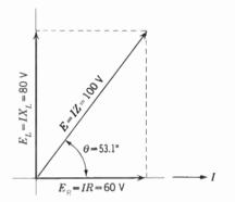
Fig.  $31 \cdot 15$  Phasor Diagram for Circuit of Fig.  $31 \cdot 14$
