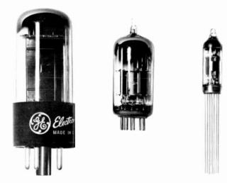
Fig. 8 · 17 Evolution of Vacuum Tubes: (a) T-9 Octal Base, (b) Glass Miniature, (c) Glass Subminiature, and (d) Ceramic Microminiature (Shown Approximately Three-Fourths of Actual Size) (Courtesy of General Electric Company)
