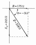
Fig. 31 · 20 Impedance Phasor Diagram for Example 10
