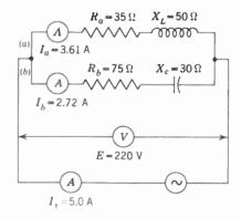
Fig. 32 · 19 Impedances in Parallel
