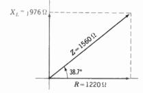
Fig. 32 • 17 Impedance Phasor Diagram for Equivalent Series Circuit
