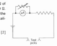
Fig. 14 · 18 Ohmmeter Circuit with Variable Shunt Resistance.
