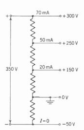
Fig. 15 · 8 Voltage Divider of Example 3
