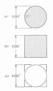
Fig. 9 · 1 Comparison of the Circular Mil and the Square Mil: (a) Circular Mil, (b) Square Mil, (c) Circular and Square Mils Compared
