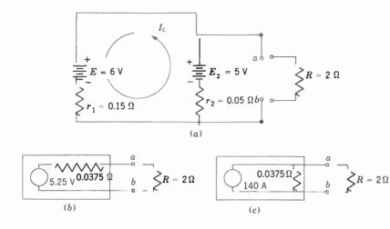
Fig. 22 · 35a Redrawn From Fig. 22 · 14 for Thevenin's Solution
