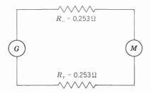
Fig. 9 • 4 Simplified Form of Circuit Shown in Fig. 9 • 3
