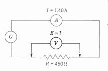
Fig. 8 · 4 Circuit of Example 3
