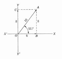
Fig. 28 • 13 Vertical and Horizontal Components of Vector
