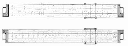
Fig. 6 • 1 Front and Back Views of Cooke Radio Slide Rule (Courtesy of Keuffel and Esser Company)
