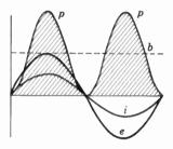
Fig. 31 · 3 Power Curves for Circuit Containing Only Resistance
