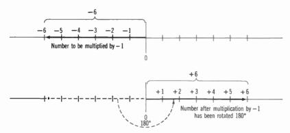
Fig.  $4 \cdot 4$  Illustration of -6Rotated Counterclockwise through 180° to Become +6 Due to Multiplication by -1
