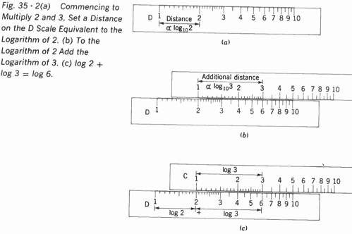
Multiply 2 and 3, Set a Distance on the D Scale Equivalent to the Logarithm of 2. (b) To the Logarithm of 2 Add the Logarithm of 3. (c) log 2 +  $\log 3 = \log 6$ .
