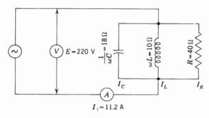
Fig. 32 · 12 L, C, and R in Parallel
