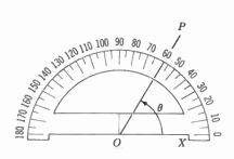
Fig.  $23 \cdot 7$  Using Protractor to Measure Angle XOP of Fig.  $23 \cdot 6$
