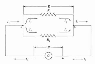
Fig.  $13 \cdot 3$  Resistors  $R_1$  And  $R_2$ Connected in Parallel across Generator G, Which Maintains a Potential of E V
