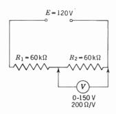
Fig.  $14 \cdot 15$  A  $30,000 \cdot \Omega$ Voltmeter Connected across R<sub>2</sub>. Total Circuit Current Is Now 1.5 mA, and the Voltage Across R<sub>2</sub> Is 30 V.
