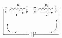
Fig. 22 • 1 Current I Flowing from – to + through the Connected Circuit
