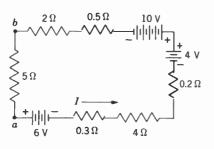
Fig. 22 • 4 Circuit of Example 1 Illustrating Internal Resistances of the Batteries
