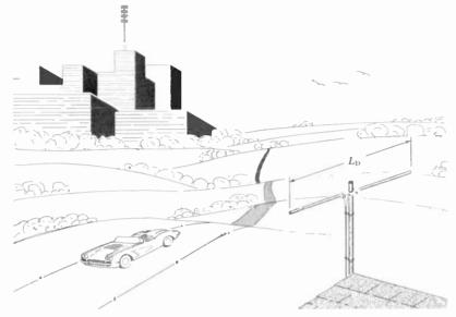
one-half wavelength long  $(0.5\lambda)$ , as illustrated in Fig. 7 · 3. The actual length is slightly less than a half wave owing to "end effect" caused by the capacitance of the antenna, and it has been determined that dipoles used for television reception should be approximately 6% shorter than one-half wavelength. Use the formula derived in Prob. 12 to derive a formula for the length of a dipole antenna in inches when the frequency is in megahertz.
