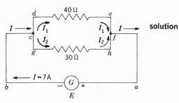
Fig. 22 · 10 Circuit of Example 2
