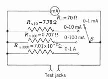
Fig. 14 • 7 Circuit for Extending Range of 0–1 Milliammeter. Test Leads from Jacks Are Connected in Series with Circuit in Which Current Is to Be Measured.
