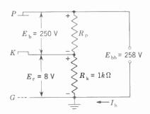
Fig. 8 • 21 Equivalent Circuit of Fig. 8 • 20 results in a voltage of 8 V across this resistor. The polarity is such that the cathode is 8 V positive with respect to the negative source of plate voltage, ground potential, and the grid, since all are connected together. This is the same as saying that the grid is 8 V negative with respect to the cathode. The remaining 250 V exists between plate P and cathode K, with the plate 250 V positive with respect to cathode.
