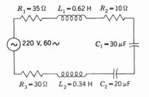
Fig. 31 · 26 Series Circuit of Example 13
