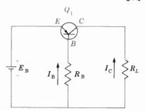
Fig.  $8 \cdot 27$  Simple Single-Battery Transistor Biasing Circuit for PNP Transistor  $Q_1$
