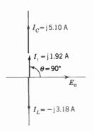
Fig. 32 · 7 Phasor Diagram for Circuit of Example 2
