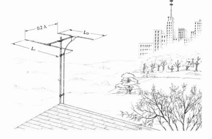
as illustrated in Fig. 7  $\cdot$  5. This wire or tube, which is known as a director, is usually placed one-tenth wavelength (0.1 $\lambda$ ) from the dipole, and it should be about 5% shorter than the dipole. Derive a formula for the length of a director in feet when *f* is in megahertz.
