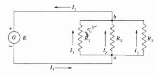
Fig. 13 · 5 Resistors R<sub>1</sub>, R<sub>2</sub>, And R<sub>3</sub> Connected in Parallel
