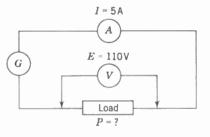
Fig. 8 • 7 Circuit of Example 6
