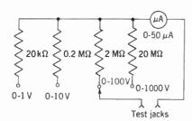
Fig. 14 · 16 A 0–50 Microammeter Used with Multipliers for Multirange Voltmeter.
