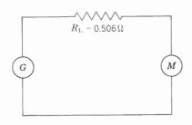
Fig.  $9 \cdot 5$  Equivalent Circuit of Circuits Shown in Figs.  $9 \cdot 3$  and  $9 \cdot 4$
