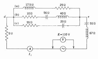
Fig. 32 · 25 Circuit of Example 5
