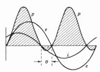
Fig. 31 · 23 Voltage, Current, and Power Relations for Circuit of Fig. 31 · 21
