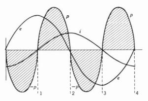
Fig. 31 · 13 Voltage, Current, and Power in an Inductive Circuit
