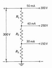
Voltage Divider of Fig. 15 · 6 Example 2
