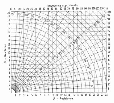
Fig. 38 • 24 Rectangular-polar Phasor Diagram
