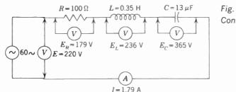
Fig. 31 · 21 Series Circuit Consisting of R, L, and C
