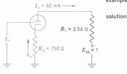
Fig. 8 + 23 Circuit of Example 15
