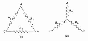
If these two circuits are to be made equivalent, then the resistance between terminals A and B, B and C, and A and C must be the same in each circuit. Hence, in Fig.  $22 \cdot 25a$  the resistance from A to B is
