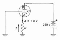
Fig.  $3 \cdot 2$  The Grid G is Negative with Respect to Cathode K
