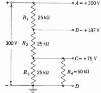
Fig. 15  $\cdot$  3 Load of 50 k  $\Omega$  Connected across Terminals C and D
