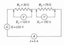
Fig. 31 · 1 Alternator Supplying Resistive Circuit
