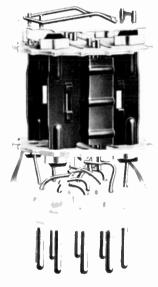
Fig. 8 • 18 Cutaway of Type GL-5751 Vacuum Tube. Shown Approximately  $2\frac{1}{2}$  Times Actual Size (Courtesy of General Electric Company)
