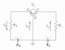
Fig. 8 · 28 PNP Transistor  $Q_1$ Biased by Means of Two Batteries,  $E_e$  and  $E_c$
