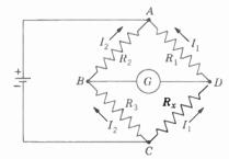
Fig. 15 · 15 Schematic Diagram of Wheatstone Bridge
