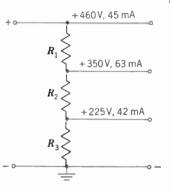
Fig. 15 • 13 Circuit of Probs. 6, 7, and 8
