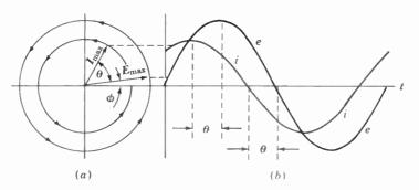
Fig. 30 · 8 Current i Leads Voltage e by Phase Angle  $\theta$
