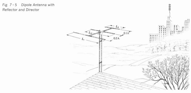
dipole, (b) length of reflector, (c) length of director, (d) spacing between dipole and reflector, and (e) spacing between dipole and director.
