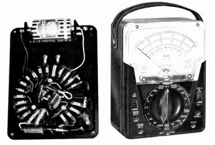
corporated into one instrument called a multimeter, one type of which is illustrated in Fig.  $14 \cdot 20$ . If the test leads are plugged into the proper pin jacks and the rotary switch is switched to the proper function and range, the instrument can be utilized for several functions.
