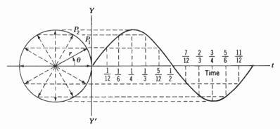
Fig. 29 · 5 Radius Vector Generating Sine Curve.
