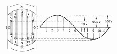
Fig. 30 · 2 Generation of Voltage Sine Wave ALTERNATING CURRENTS FUNDAMENTAL IDEAS
