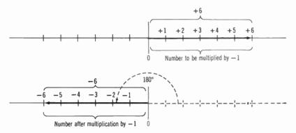
Fig.  $4 \cdot 3$  Multiplication by -1Rotates Multiplicand Counterclockwise through 180°
