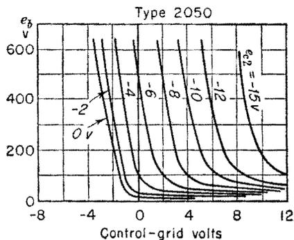
FIG. 13-17. Firing characteristics for a shield-grid thyatron.
