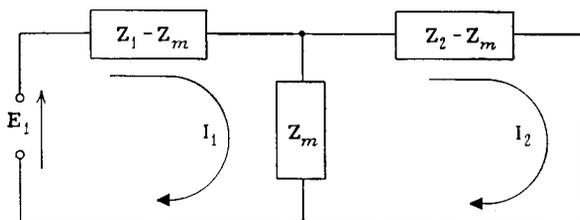
FIG. 7-82. Equivalent circuit of a simple coupled circuit.
