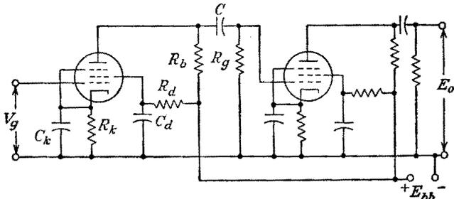
FIG. 7-11. An  $R$ - $C$ -coupled pentode amplifier.
