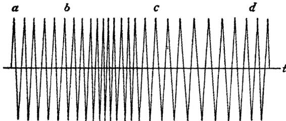
FIG. 5-2. Angle-modulated wave.
