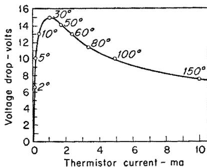
FIG. 16-5. Static volt-ampere curve for a typical thermistor. (Courtesy of Bell Laboratories.<sup>3</sup>)
