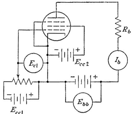
FIG. 4-24. Circuit for obtaining dynamic transfer characteristics.
