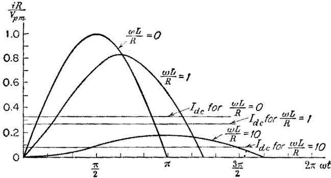
FIG. 14-16. Waveforms of current for a half-wave rectifier with a smoothing inductor.
