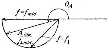
FIG. 7-21. Polar plot of  $A_{low}/A_{mid}$  vs.  $\theta_A$ .
