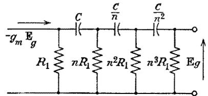
FIG. 11-20. Norton's equivalent of the phase-shift oscillator.
