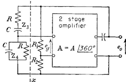
FIG. 11-21. Schematic diagram of a Wien-bridge oscillator.
