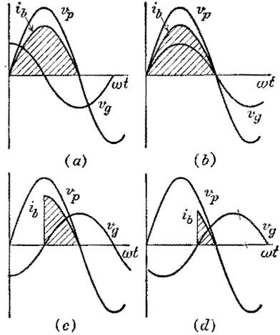
FIG. 14-26. Waveshapes illustrating phase-shift control.
