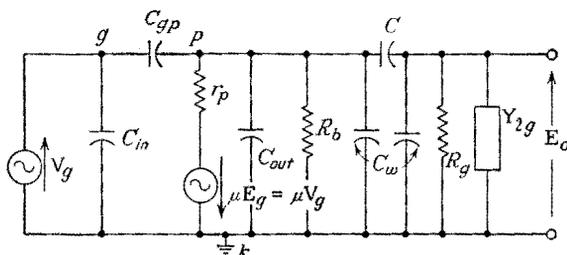
FIG. 7-12. Equivalent circuit for the entire frequency band.
