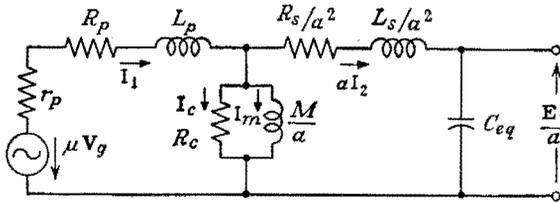
FIG. 7-68. Another equivalent circuit for a transformer-coupled amplifier.
