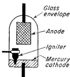
FIG. 13-10. A small sealed-off ignitron.
