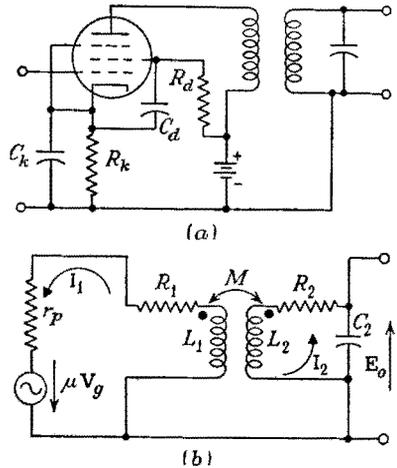
FIG. 7-81. (a) Tuned-secondary r-f amplifier. (b) Equivalent circuit of (a).
