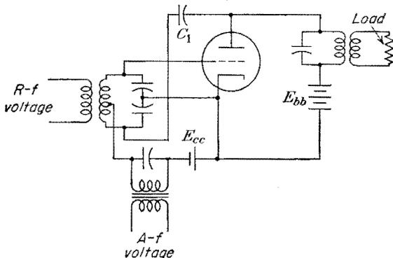
FIG. 12-9. A grid-bias-modulated class C amplifier.
