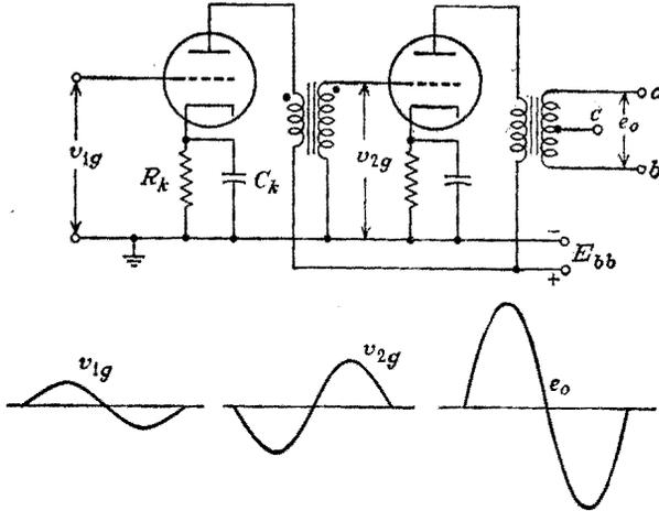
FIG. 5-11. A two-stage transformer-coupled amplifier with cathode bias.
