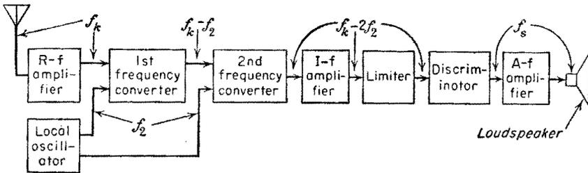
FIG. 12-28. A block diagram of an f-m receiver.
