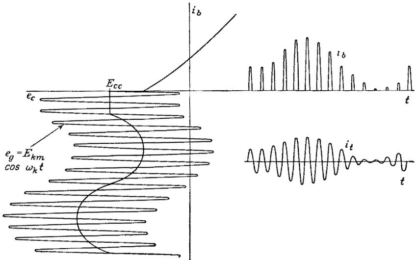
FIG. 12-10. Action of a grid-bias-modulated class C amplifier.
