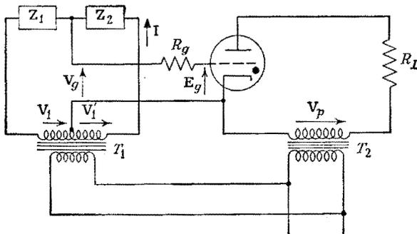
FIG. 14-27. A thyatron with phase-shift control.
