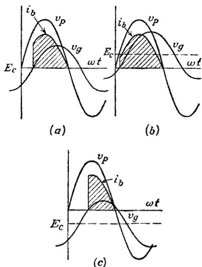
FIG. 14-32. Wave shapes for bias phase control.
