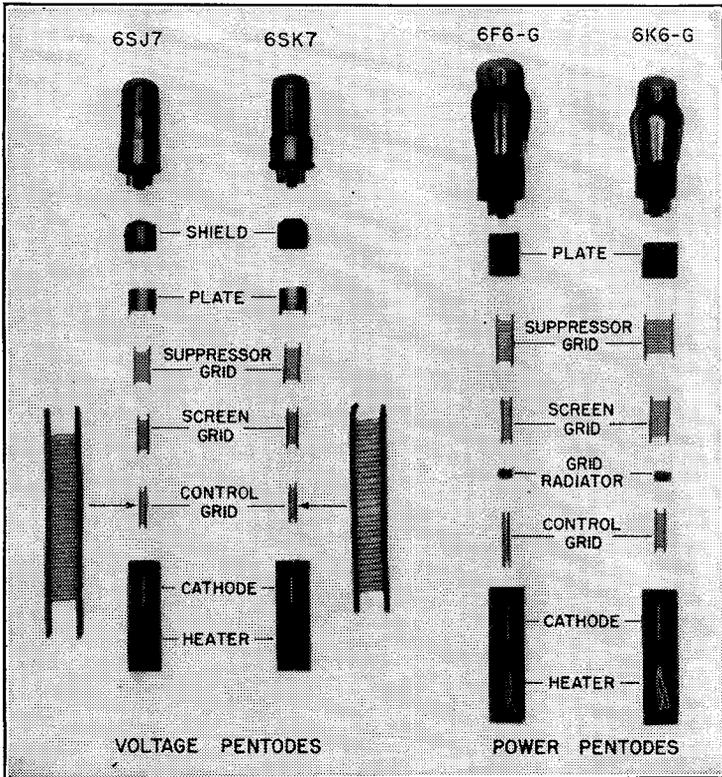
FIG. 4-28. Elements of voltage and of power pentodes.
