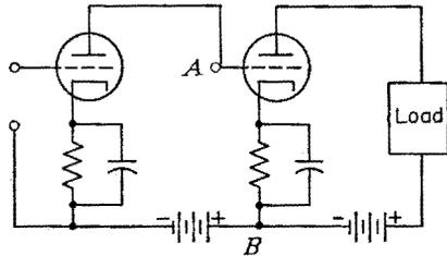
FIG. 7-6. A circuit like this will not work.
