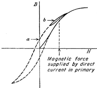
Fig. 7-66. Magnetic operation of a transformer.
