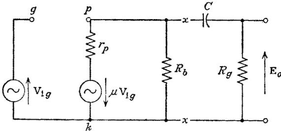
FIG. 7-17. Equivalent circuit for the l-f range.
