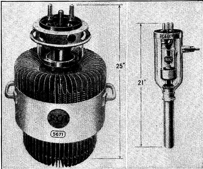
FIG. 3-9. Large transmitting tubes. (Courtesy of RCA.)
