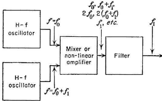
FIG. 11-18. Block diagram for a beat-frequency oscillator.
