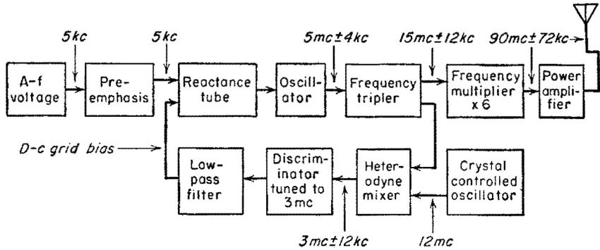
FIG. 12-25. A reactance-tube frequency-modulator system with a frequency stabilizer.
