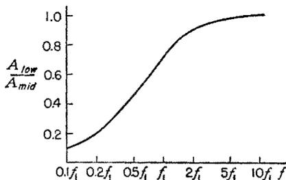
FIG. 7-19. Gain vs. frequency in the l-f range.
