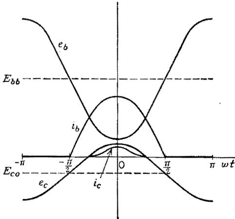
FIG. 9-2. Approximate waveforms for class B operation.
