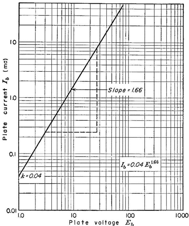
FIG. 3-8. Curve used to determine the coefficients in the Child-Langmuir equation.
