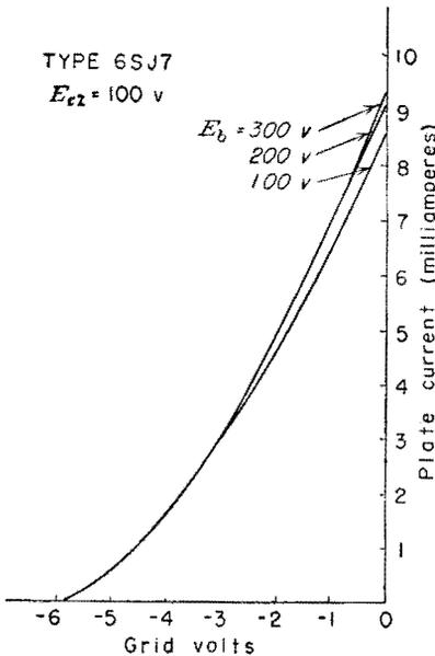
FIG. 4-23. Transfer characteristics for a 6SJ7 pentode.
