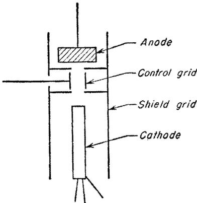
FIG. 13-16. Typical electrode structure for a shield-grid thyatron.
