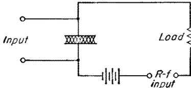
FIG. 16-28. Basic circuit for a dielectric amplifier.
