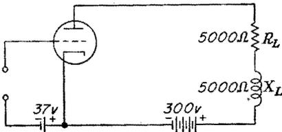
FIG. 6-6. A triode with an inductive load.
