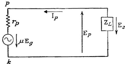
FIG. 6-20. Thévenin's equivalent circuit for sinusoidal voltages.
