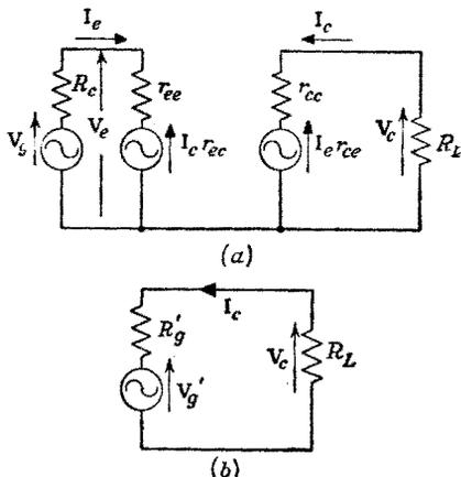
FIG. 16-17. Equivalent circuits for a transistor used as an amplifier.
