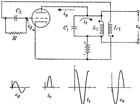
FIG. 5-20. A feedback oscillator.
