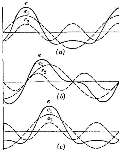
Fig. 7-38. The effect of phase shift on waveform. (a) Input voltage and its components. (b) Output voltage and its components. Each component shifted a constant angle of  $90^\circ$ . (c) Output voltage and its components.  $e_1$  shifted  $90^\circ$ ;  $e_2$  shifted  $2 \times 90^\circ$ .
