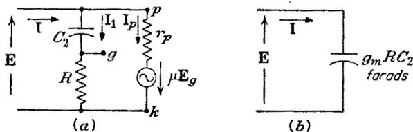
FIG. 12-24. Equivalent circuits for a reactance tube.
