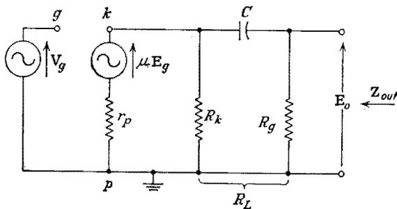
FIG. 7-52. The equivalent circuit for low frequencies.
