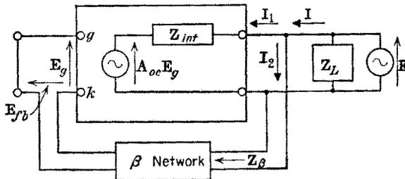
FIG. 10-10. Testing a voltage-feedback circuit for output impedance.
