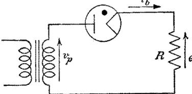
FIG. 14-7. Circuit diagram of a half-wave gas-diode rectifier with a resistance load.
