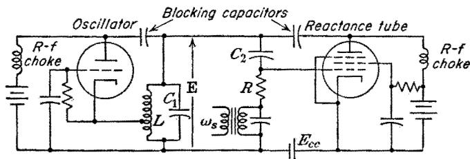
FIG. 12-23. A reactance tube modulating a Hartley oscillator.
