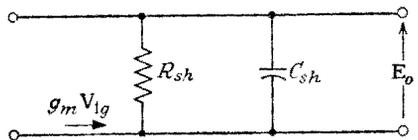
FIG. 7-23. Norton's equivalent circuit for high frequencies.
