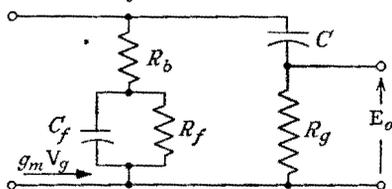
FIG. 7-43. Norton's equivalent of the circuit of Fig. 7-42.
