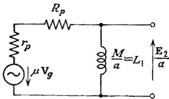
FIG. 7-69. Low-frequency equivalent circuit for a transformer-coupled amplifier.
