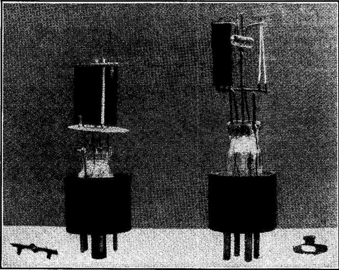
FIG. 3-1. Radio-receiver-type diodes.
