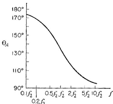
FIG. 7-25.  $\theta_A$  vs. frequency in the h-f range.
