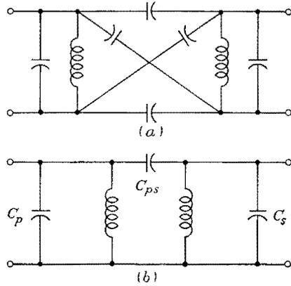
FIG. 7-63. Distributed capacitances in a transformer.
