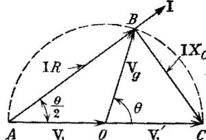
FIG. 14-29. Vector diagram for a phase-shift circuit for  $V_g$  leading  $V_1$  by an angle  $\theta$ .
