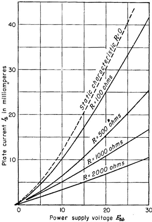
FIG. 3-12. Dynamic plate characteristics for a type 6H6 diode with various load resistors.
