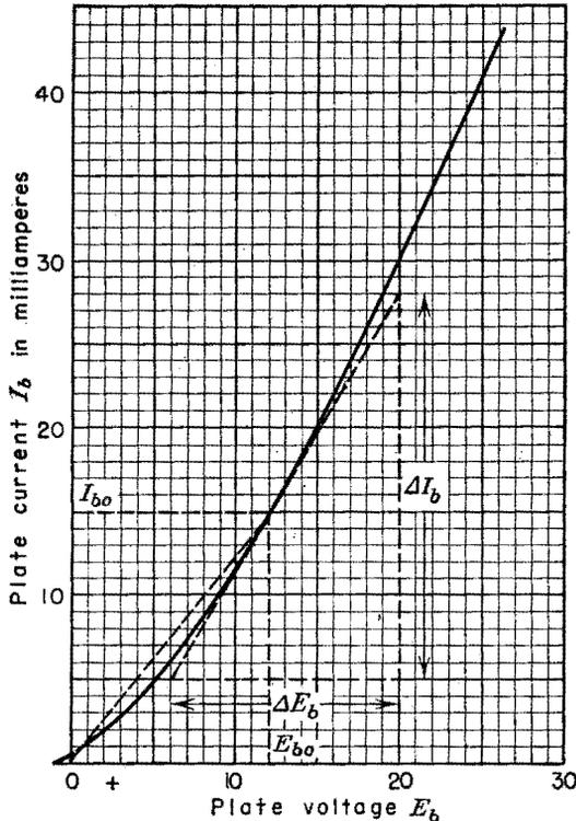
FIG. 3-10. Plate characteristic of a type 6H6 diode.
