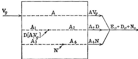
FIG. 10-3. Block diagram of a nonfeedback amplifier.
