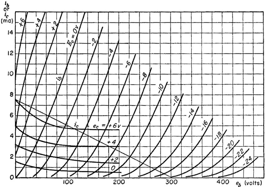
FIG. 11-24. Characteristics of a 6SN7 (one section).
