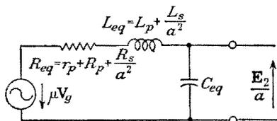
FIG. 7-70. High-frequency equivalent circuit for a transformer-coupled amplifier.
