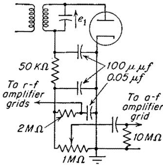
FIG. 12-19. A diode detector and AVC circuit.
