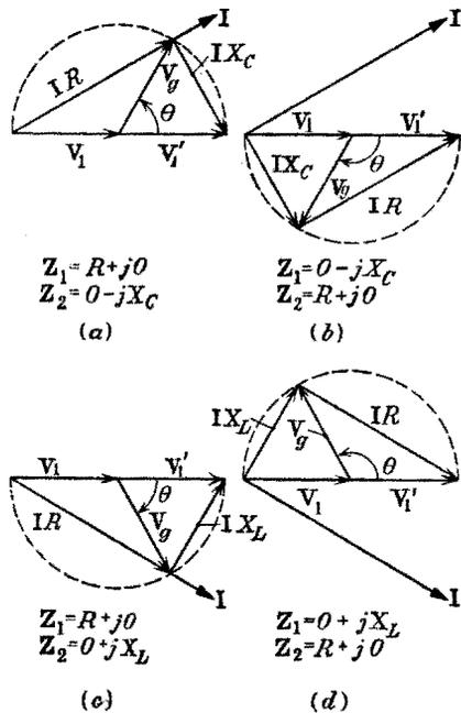
FIG. 14-28. Vector diagrams for the phase-shift circuit.
