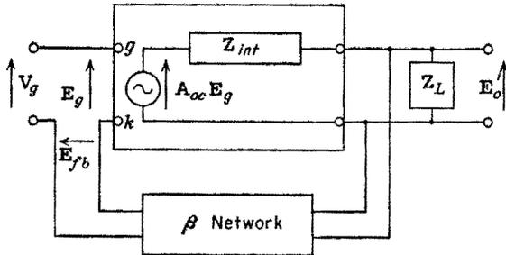
FIG. 10-9. A representation of a general voltage-feedback circuit.
