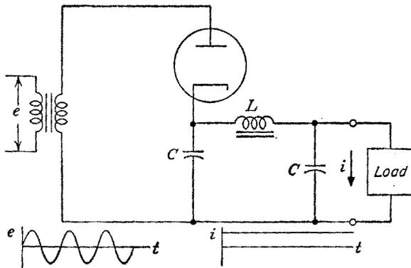
FIG. 5-6. A half-wave rectifier with a filter.
