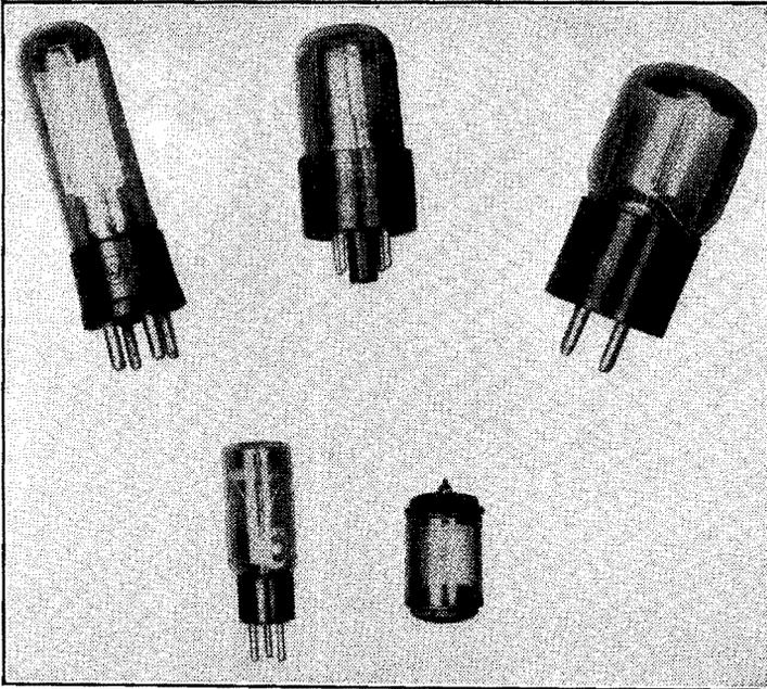
FIG. 15-5. Photoemissive cells.
