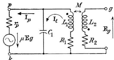
FIG. 11-10. Equivalent circuit for a tuned-plate oscillator.
