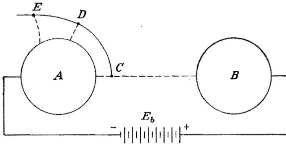
Fig. 1-1. Plotting equipotential lines between two parallel cylinders.
