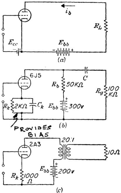
FIG. 6-3. Some common plate-load arrangements.
