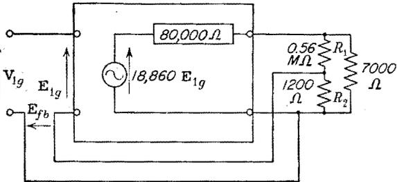
FIG. 10-21. An equivalent circuit for the amplifier of Fig. 10-20.
