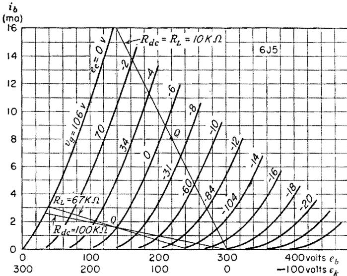
FIG. 7-57. Graphical analysis of a cathode follower.
