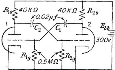
FIG. 11-23. An alternate representation for the multivibrator.
