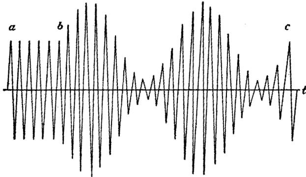
FIG. 5-1. Amplitude-modulated wave.
