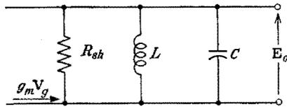
FIG. 7-77. Norton's equivalent circuit for the single-tuned amplifier.
