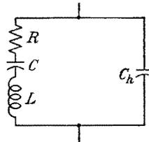
FIG. 11-9. The equivalent circuit for a crystal.
