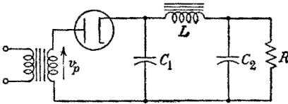
FIG. 14-21. A half-wave rectifier with a  $\Pi$ -section filter.
