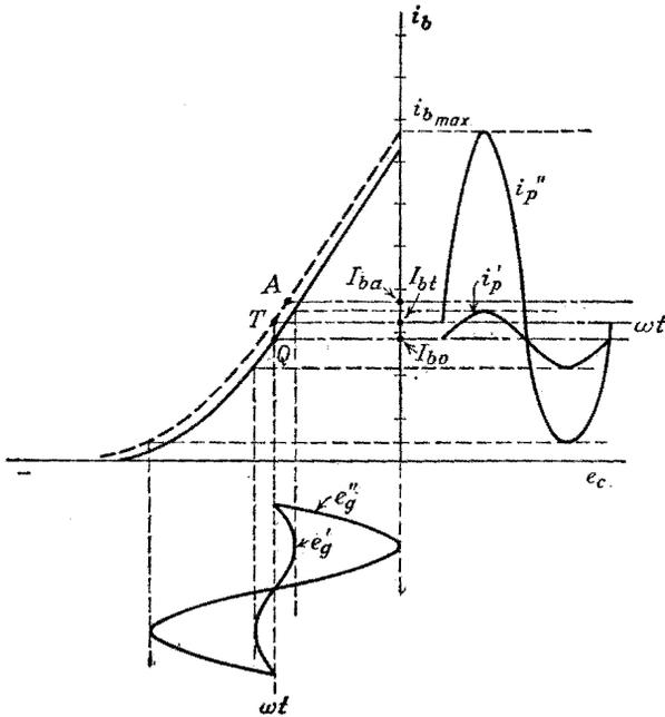
FIG. 6-11. A dynamic transfer characteristic for a triode with fixed grid bias, for linear and for nonlinear operation.
