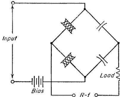
FIG. 16-30. A practical circuit for a dielectric amplifier.
