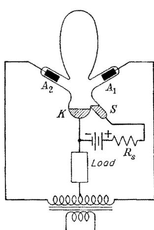
FIG. 13-9. An old-type mercury-arc tube and its circuit.
