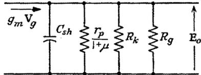
It can be shown that this is identical to formula (7-89). FIG. 7-55. Another h-f equivalent circuit for a cathode follower.
