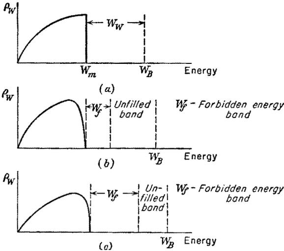
FIG. 16-2. Density of energy states in (a) a good conductor, (b) a semiconductor, (c) an insulator.
