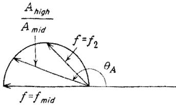
FIG. 7-26. Polar plot of  $A_{high}/A_{mid}$  vs.  $\theta_A$  for the h-f range.
