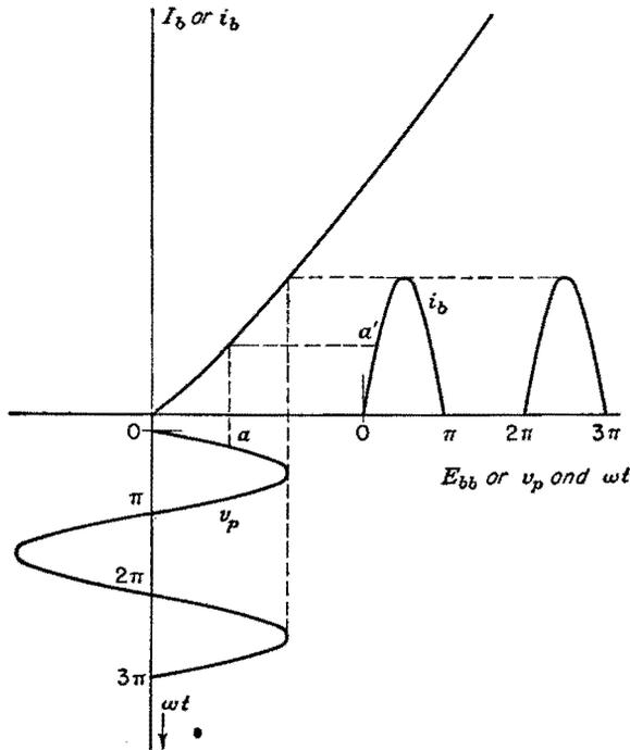
FIG. 3-13. Graphical method of determining the plate current in a diode when an alternating voltage is applied.
