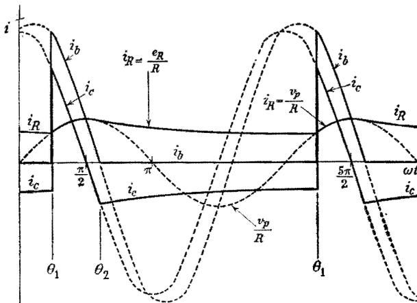
FIG. 14-13. Waveforms for  $i_R$ ,  $i_C$ , and  $i_b$ ;  $RC$  moderately large.
