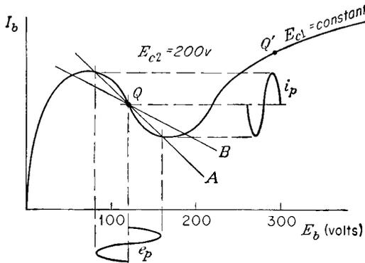
FIG. 11-17. The tetrode can be a negative-resistance device.
