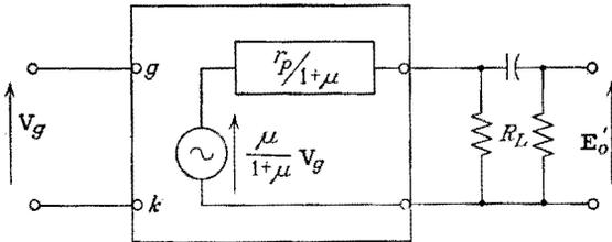
FIG. 10-15. A nonfeedback equivalent of the cathode follower.
