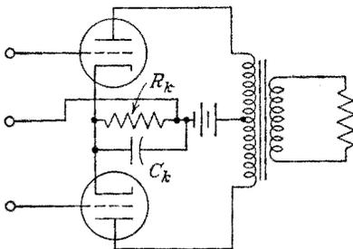
FIG. 8-23. A push-pull amplifier employing cathode bias.
