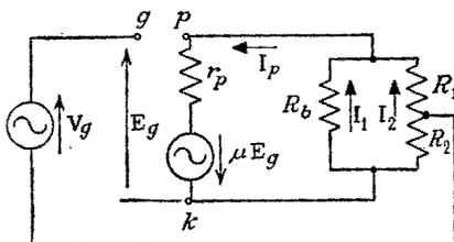
FIG. 6-25. Thévenin's equivalent for the circuit of Fig. 6-24.
