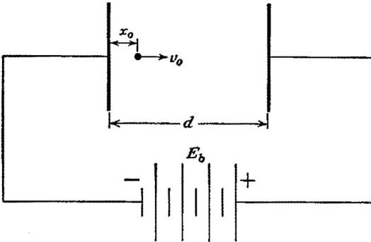
FIG. 1-8. Action of a uniform electric field on an electron with an initial velocity.
