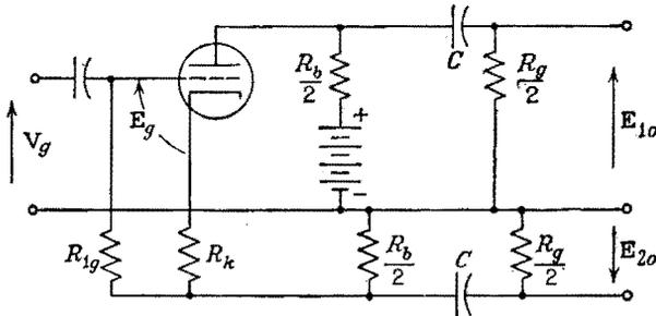
FIG. 7-48. A split-load type of phase inverter.
