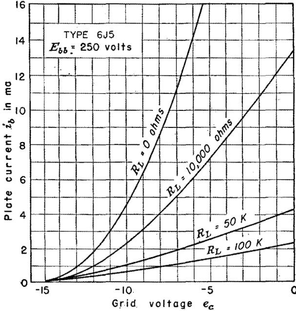
FIG. 4-11. Dynamic transfer characteristics for a 6J5 tube.
