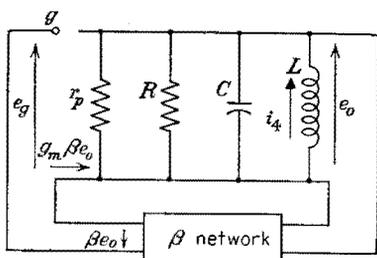
FIG. 11-2. The equivalent circuit for a regenerative-feedback oscillator.
