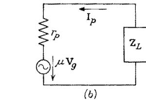
FIG. 8-5. (a) A power amplifier. (b) Its linear equivalent circuit.
