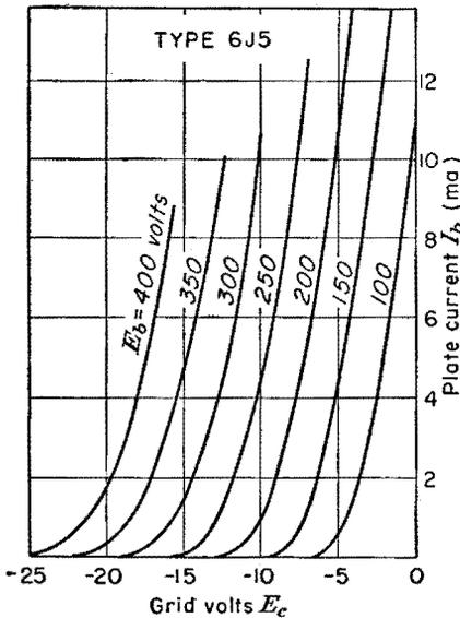
FIG. 4-5. Transfer characteristics of a 6J5 triode.
