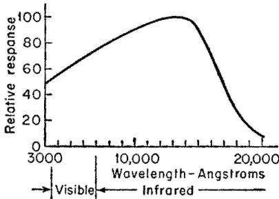
FIG. 16-18. Spectral response of a selenium photoconductive cell.
