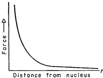
FIG. 2-1. Force on an electron in the vicinity of an isolated nucleus.
