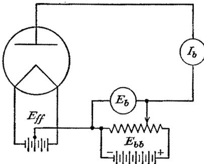
FIG. 3-7. Circuit used to evaluate the constants of the Child-Langmuir equation.
