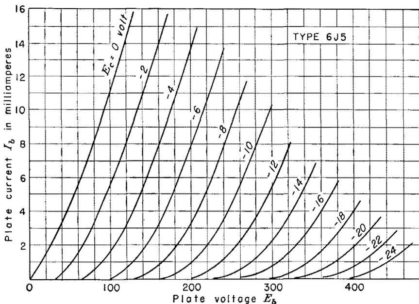
FIG. 4-4. Plate characteristics of a 6J5 triode.
