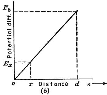
FIG. 1-7. Potential distribution between parallel plane plates.
