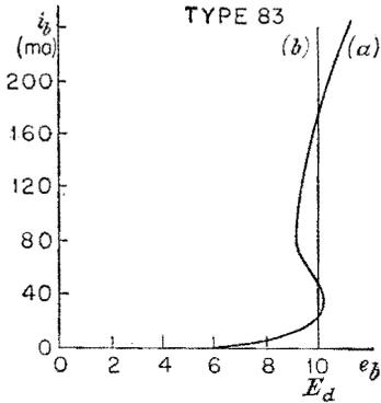
FIG. 14-8. Volt-ampere characteristic for a hot-cathode mercury-vapor rectifier.
