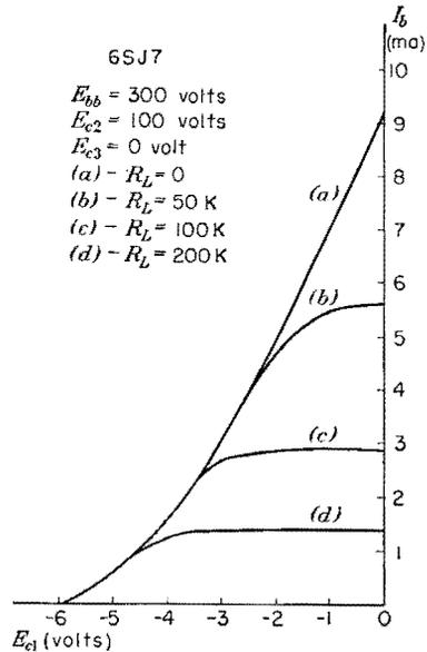
FIG. 4-25. Dynamic transfer characteristics for a 6SJ7 pentode.
