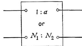
FIG. 7-60. An alternate symbol for an ideal transformer.
