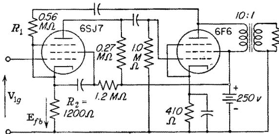
FIG. 10-20. A two-stage feedback circuit.
