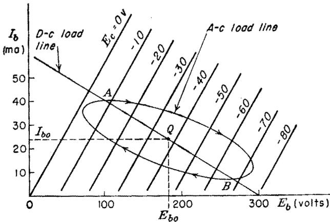
FIG. 6-7. Plate diagram for the circuit of Fig. 6-6.
