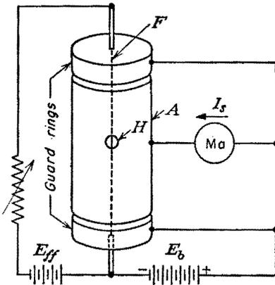
FIG. 2-3. Tube for determining the emission characteristics of a filament.
