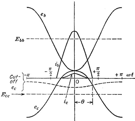
FIG. 9-3. Approximate waveforms for class C operation.
