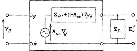
FIG. 10-12. A nonfeedback representation of a current-feedback amplifier.
