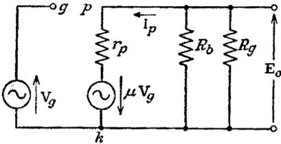
FIG. 7-13. Thévenin's circuit for the mid-frequency range.
