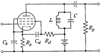
FIG. 7-76. An amplifier with a single-tuned load.
