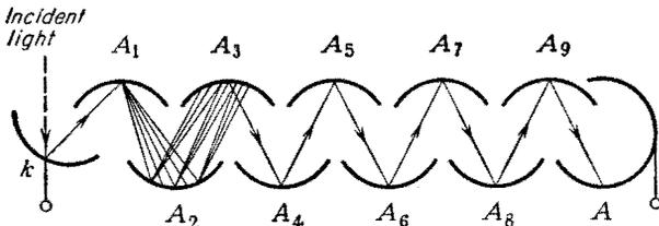
FIG. 15-13. Cross-section plan drawing of a photomultiplier tube.
