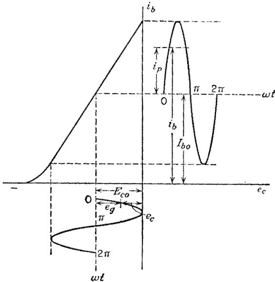
FIG. 6-9. Dynamic transfer characteristics of a triode amplifier with waveforms of current and voltage.
