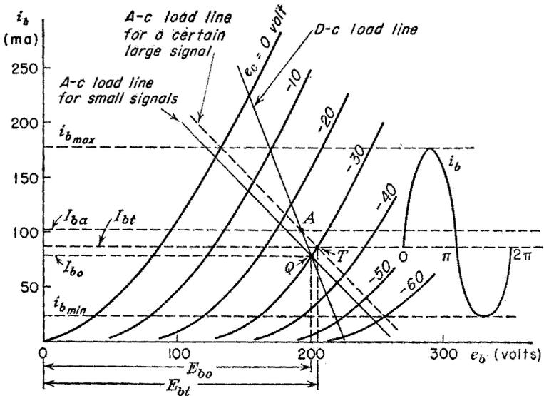
FIG. 6-10. Plate diagram of a triode with fixed grid bias and nonlinear operation (exaggerated).
