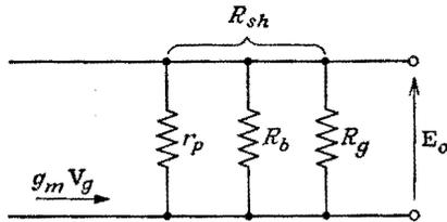
FIG. 7-14. Norton's equivalent circuit for the mid-frequency range.
