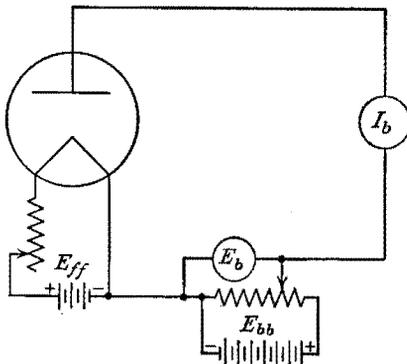
FIG. 3-2. Circuit for determining the characteristics of a diode.
