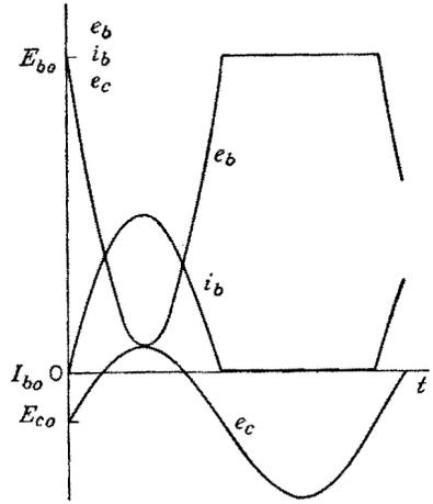
FIG. 8-4. Waveforms for class B operation.
