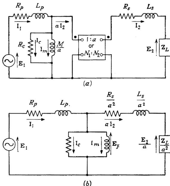
FIG. 7-65. Equivalent circuits for a power transformer.
