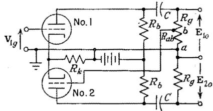
FIG. 7-47. A two-tube type of phase inverter.
