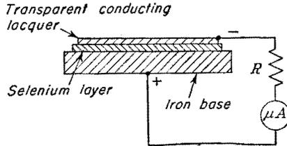
FIG. 16-19. Construction of a selenium-iron photovoltaic cell.
