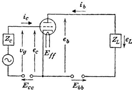
FIG. 6-1. A triode with a plate load.
