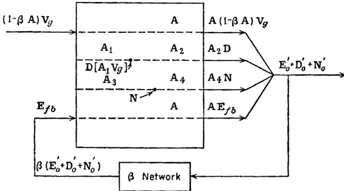
FIG. 10-4. A feedback amplifier with increased signal.
