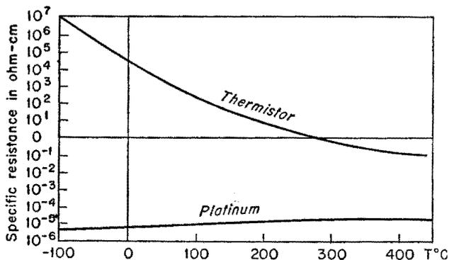
FIG. 16-4. Resistance-temperature curve of a typical thermistor and of platinum. (Courtesy of Bell Laboratories.<sup>3</sup>)
