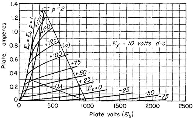
FIG. 8-25. Class B operation with an 830-B tube.
