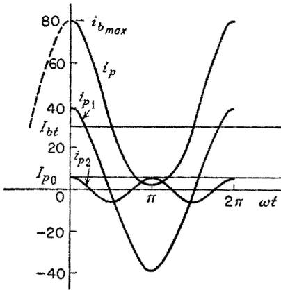
FIG. 6-27. Composition of plate current from its components.
