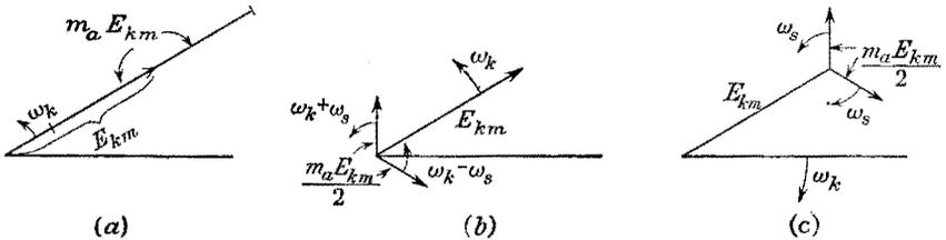
FIG. 12-3. Vector diagrams for an a-m wave.
