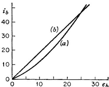
FIG. 14-2. The volt-ampere characteristic for a 6H6 tube.
