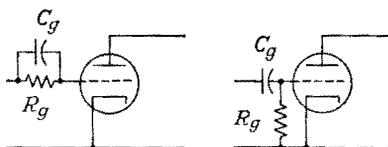
FIG. 9-12. Grid-leak-bias arrangements.
