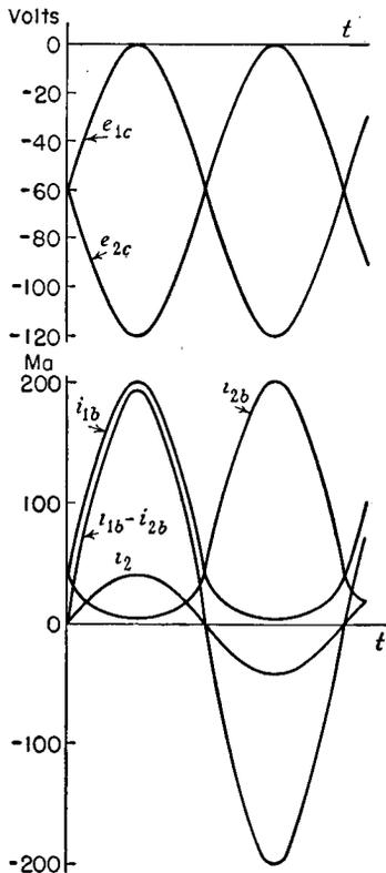
FIG. 8-22. Waveforms associated with the example of Art. 8-10.
