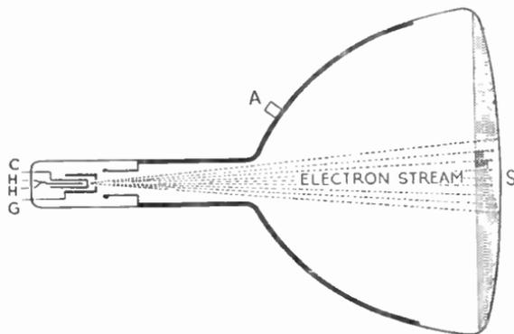
Fig. 21.1—Section of typical cathode-ray tube. H = heater; C = cathode; G = grid; A = anode; S = fluorescent screen
