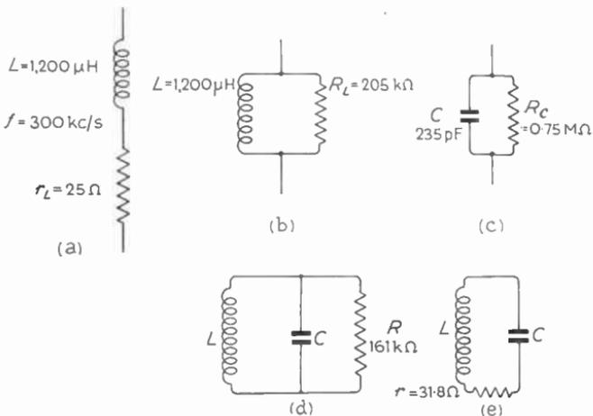
Fig. 8.15—Example to illustrate series and parallel equivalents.  $b$  is equivalent to  $a$ ; and  $d$  and  $e$  are alternative ways of expressing the result of combining  $c$  with  $b$
