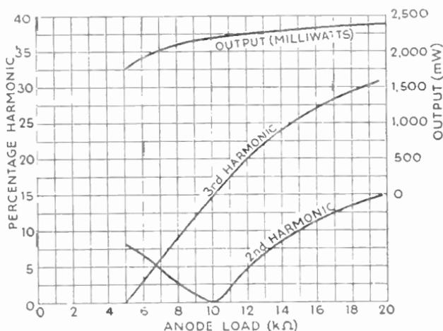
Fig. 20.15—Output and harmonic distortion related to load resistance for a pentode
