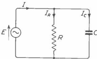
Fig. 6.11—The branch currents in this circuit,  $I_R$  and  $I_C$ , are  $90^\circ$  out of phase with one another
