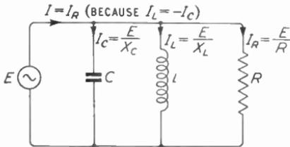
Fig. 8.14—An alternative way of representing a circuit such as Fig. 8.12 (a). If  $r$  is small compared with  $X$ ,  $R = X^2/r$
