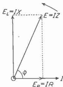
Fig. 7.4—Vector diagram relating to Fig. 7.3
