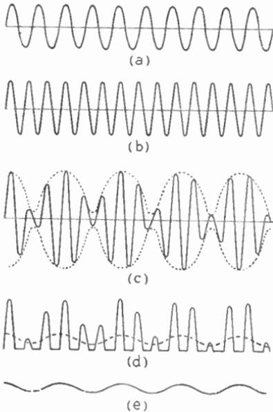
Fig. 19.1—Showing the action of a frequency-changer
