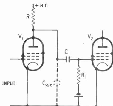
Fig. 20.6—Simple form of resistance-coupled amplifier.  $C_{ae}$  denotes unavoidable stray capacitance
