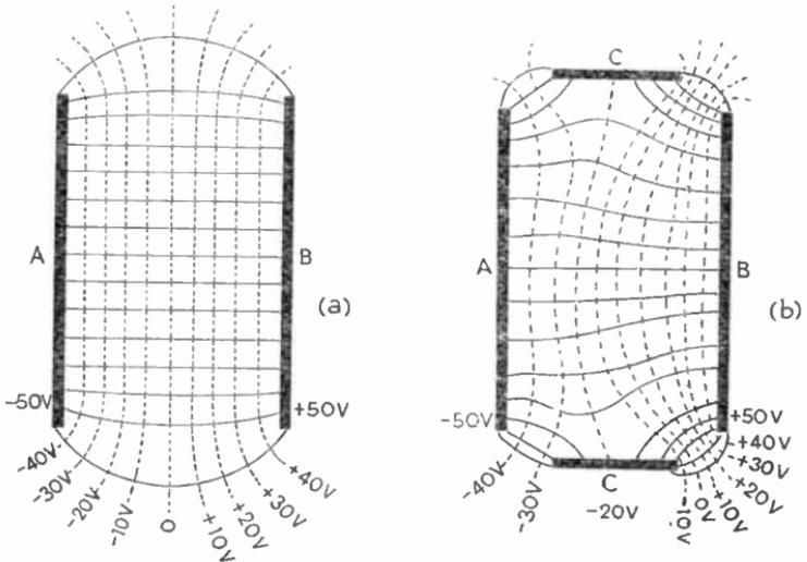
Fig. 21.2—Diagrams to illustrate electrostatic focusing
