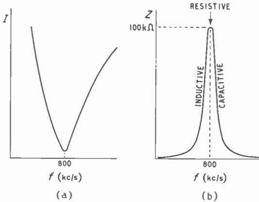
Fig. 8.13 — Plotting the current and impedance of the Fig. 8.12a circuit as a whole at various frequencies gives the shapes shown here: (a) current, (b) impedance
