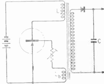
path through the  $p-n-p$  transistor. When it can rise no more, the e.m.f. ceases, the transistor is cut off, and the falling current charges  $C$ . When it ceases, the small  $I_{c0}$  through  $L$  starts the cycle all over again.
