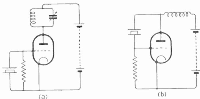
Fig. 13.4—Two types of crystal-controlled oscillator circuit
