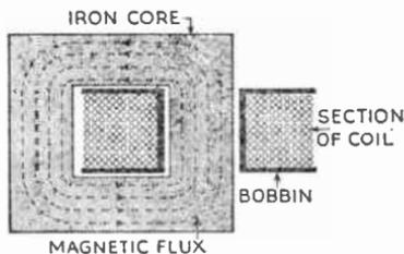
Fig. 4.7—Showing how a closed iron core links with the turns of the coil and carries nearly all the flux set up by the coil
