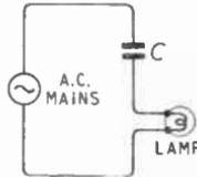
series—can easily be demonstrated by bridging the open contacts of an electric light switch by a capacitor; say  $2\ \mu\text{F}$  for a 40 W lamp (Fig. 6.3). The lamp will light and stay alight as long as the capacitor is connected. But its brilliance will be below normal.
