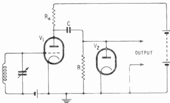
Fig. 17.1—This resistance-coupled amplifier is of little or no value for r.f. amplification
