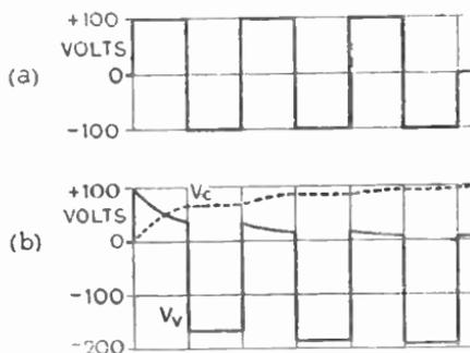
Fig. 16.6—Analysis of application of a square alternating voltage (a) to the circuit Fig. 16.5. The dotted line in b represents the voltage across  $C$ ; the full line, that across the diode
