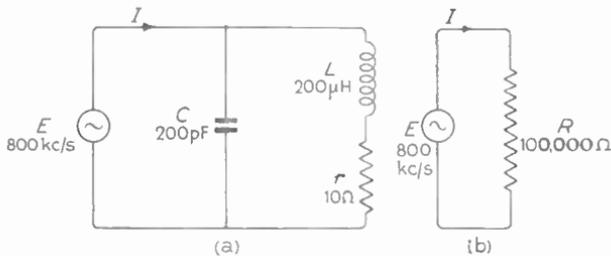
**Fig. 8.12**—The circuit composed of  $C$ ,  $L$  and  $r$  having the values marked (a) can at 800 kc/s be replaced by a high resistance (b), so far as the phase and magnitude of the current taken by the generator is concerned
