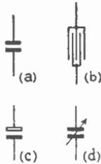
Fig. 3.4—Standard symbols for (a) fixed capacitor, (c) the same (electrolytic), in which the white plate is positive, and (d) variable capacitor. The symbol (b) denoting one of large capacitance is generally obsolete
