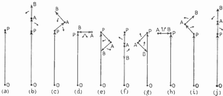
Fig. 18.3.—Progressive series of vector diagrams, showing how adding a pair of oppositely-rotating vectors ( $PA$  and  $AB$ ) alternately lengthens and shortens the original vector ( $OP$ ) without affecting its phase
