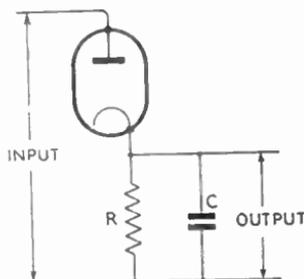
Fig. 16.5—Diode rectifier with the load resistor ( $R$ ) shunted by a reservoir capacitor,  $C$
