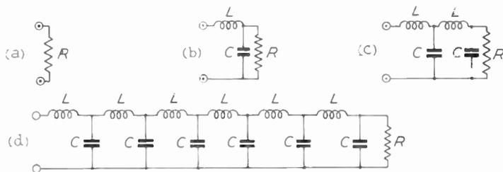
Fig. 14.3—Synthesis of transmission line from basic circuit elements
