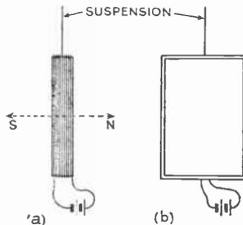
**Fig. 4.4—A coil carrying current, and free to rotate, sets itself with its axis pointing N and S. *a* is a side view and *b* an end view**
