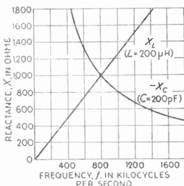
Fig. 8.5—Reactances of the coil and capacitor in Fig. 8.4 plotted against frequency
