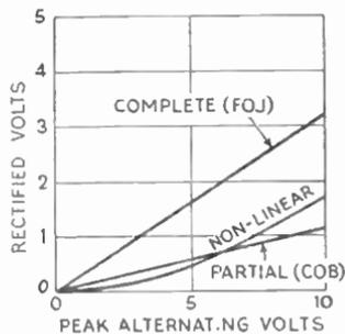
**Fig. 16.4**—The rectified outputs obtained by applying alternating voltages to various rectifiers are shown in these characteristic curves, lettered to correspond with Figs. 16.2 and 16.3
