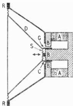
Fig. 20.22—Cross-section of a moving-coil loudspeaker
