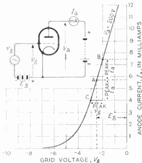
is larger than the alternating grid voltage that caused it, we have a voltage amplifier. Alternatively, if the alternating current is strong enough it can be used to operate a loudspeaker or other device, in which case the valve is described as a power amplifier. It is this ability to amplify that has made modern radio and the many kindred developments comprised in electronics possible. The subject is so important that several chapters will be devoted to it, beginning with Chapter 11.
