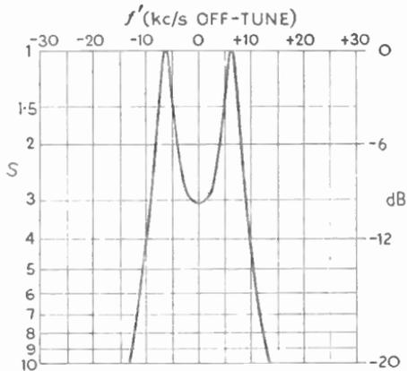
Fig. 19.14—The result of trying to maintain sidebands when using excessively selective coils in a bandpass filter—the “rabbit’s ears” produced by over-coupling
