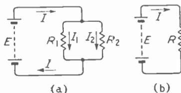
Fig. 2.8—Resistances in parallel. The circuit b is equivalent to the circuit a in the sense that both take the current from the battery, if  $1/R = 1/R_1 + 1/R_2$ .
