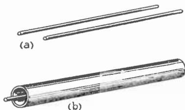
Fig. 14.1—The two main types of r.f. transmission line or feeder cable: (a) parallel-wire, and (b) coaxial
