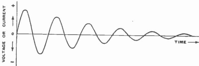
Fig. 12.3.—The first few cycles of a train of damped oscillations
