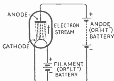
Fig. 9.1—Electron flow from cathode to anode in a directly-heated diode valve
