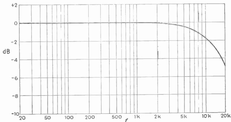
Fig. 20.7—Frequency curve of the amplifier of Fig. 20.6 when  $r_a$  of  $V_1$  is 1.5 M $\Omega$ ,  $R$  and  $R_1$  in parallel is 0.5 M $\Omega$ , and  $C_{ae}$  is 30 pF, showing falling-off (in decibels) at the top audio frequencies due to  $C_{ae}$
