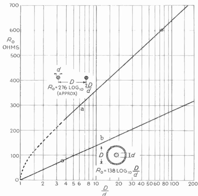
Fig. 14.4—Graphs showing characteristic resistance ( $R_o$ ) of (a) parallel-wire and (b) coaxial transmission lines in terms of dimensions
