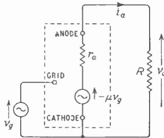
in place of a parallel resonant circuit (Fig. 8.12). And now this trick of the *valve equivalent generator*, which is one of the most important and useful of all.
