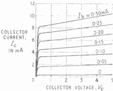
Fig. 10.14—Collector current/voltage characteristic curves of an *n-p-n* junction transistor
