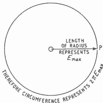
that P's motion represents  $2\pi f E_{\max}$  volts per second (Fig. 6.5). But we have just seen that it also represents the maximum rate at which PQ, the instantaneous voltage, is growing. So, fitting this information into our equation, we have
