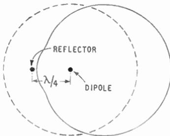
Fig. 15.9—Showing how the equal-all-round radiation of Fig. 15.8 (a) (repeated here dotted) is modified by an unconnected dipole placed quarter of a wavelength away from the first, and of such a length as to have a 45° phase angle
