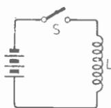
Fig. 23.6—The basic principle of inductive d.c.-to-a.c. converters can be illustrated by this simple circuit
