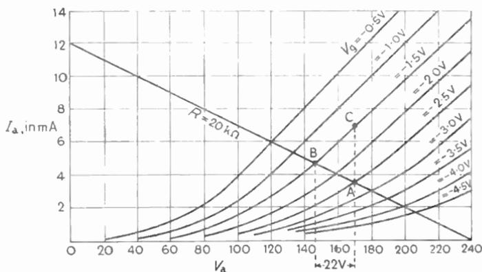
Fig. 11.2—The problem of finding the amplification of the valve in Fig. 11.1 is here worked out on an  $I_a/V_a$  curve sheet
