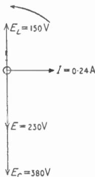
Fig. 8.2—Vector diagram relating to Fig. 8.1, when  $E = 230$  V,  $X_C = 1,590 \Omega$  and  $X_L = 628 \Omega$
