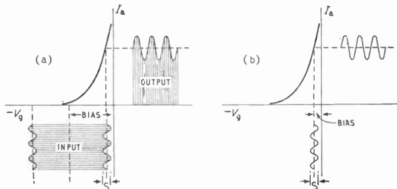
Fig. 19.7—Diagram showing how conversion conductance compares with mutual conductance
