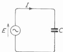
Fig. 6.1—Circuit consisting of an a.c. generator with a purely capacitive load
