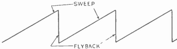
Fig. 21.5—Sawtooth waveform used for c.r. tube time-base deflection
