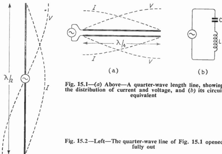
Fig. 15.1—(a) Above—A quarter-wave length line, showing the distribution of current and voltage, and (b) its circuit equivalent
