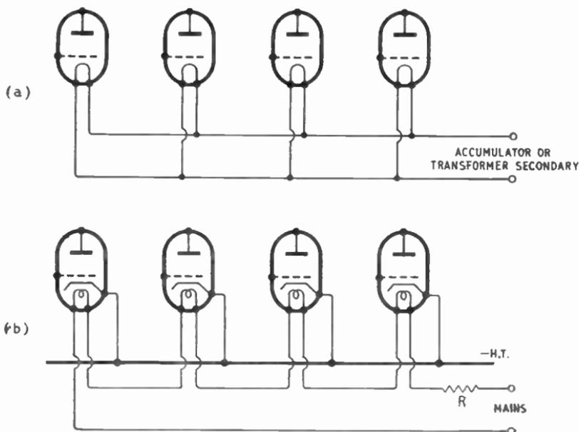
**Fig. 23.2**—Diagram *a* shows the usual method of connecting the filaments of battery valves or heaters of a.c. valves, namely, in parallel. To run heaters direct from either d.c. or a.c. mains, they are connected in series, as at *b*. Note that in spite of the different potentials of the heaters all cathodes can be joined to -b.t.
