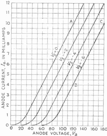
Fig. 9.5—Characteristic curves of triode valve, at different grid voltages. (These curves are somewhat idealized, being straighter and more parallel than in actual practice)
