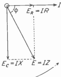
e.m.f. Its length represents the voltage of the e.m.f. ( $=IR$ ) to any convenient scale. The length of the  $E_C$  vector represents  $E_C$  ( $=IX$  or  $I/2\pi fC$ ) to the same scale, and since we know the current is  $90^\circ$  ahead of it we must draw it  $90^\circ$  behind the current vector. The vector representing  $E$  in magnitude and phase is then easily found as explained in connection with Fig. 5.7.
