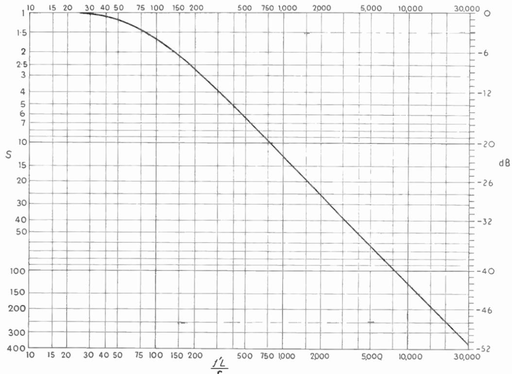
Fig. 18.6—Generalized resonance curve for any single tuned circuit. To make it refer to any particular circuit, divide the numbers on the horizontal scale by  $L/r$  (or by  $Q/2\pi f_i$ ) to convert them to a scale of  $f'$ . The units are:  $L$  in  $\mu\text{H}$ ;  $r$  in  $\Omega$ ;  $f'$  in kc/s;  $f_i$  in Mc/s
