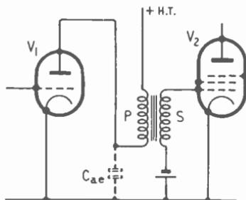
Fig. 20.8 — Simple transformer-coupled amplifier circuit
