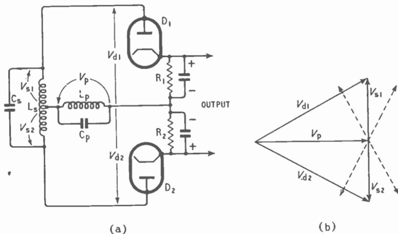
Fig. 16.17—(a) Circuit of phase discriminator for f.m. detection, arranged to bring out the principle:  $L_p$  and  $L_s$  are the primary and secondary windings of the input r.f. transformer; (b) vectors of voltages marked, for carrier wave frequency. Dotted lines indicate the effect of f.m. deviation
