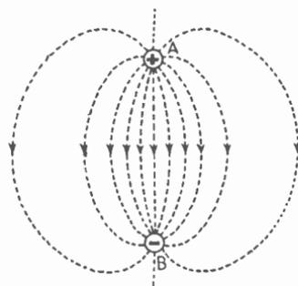
Fig. 3.2—The dotted lines indicate the direction and relative intensity of electric field between two oppositely-charged terminals, A and B
