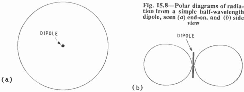
Fig. 15.8—Polar diagrams of radiation from a simple half-wavelength dipole, seen (a) end-on, and (b) side view
