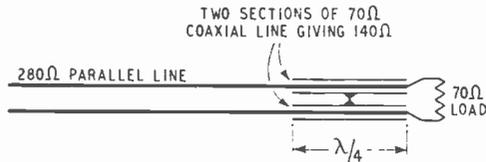
Fig. 14.7—Example of a quarter-wave length of line being used as a matching transformer
