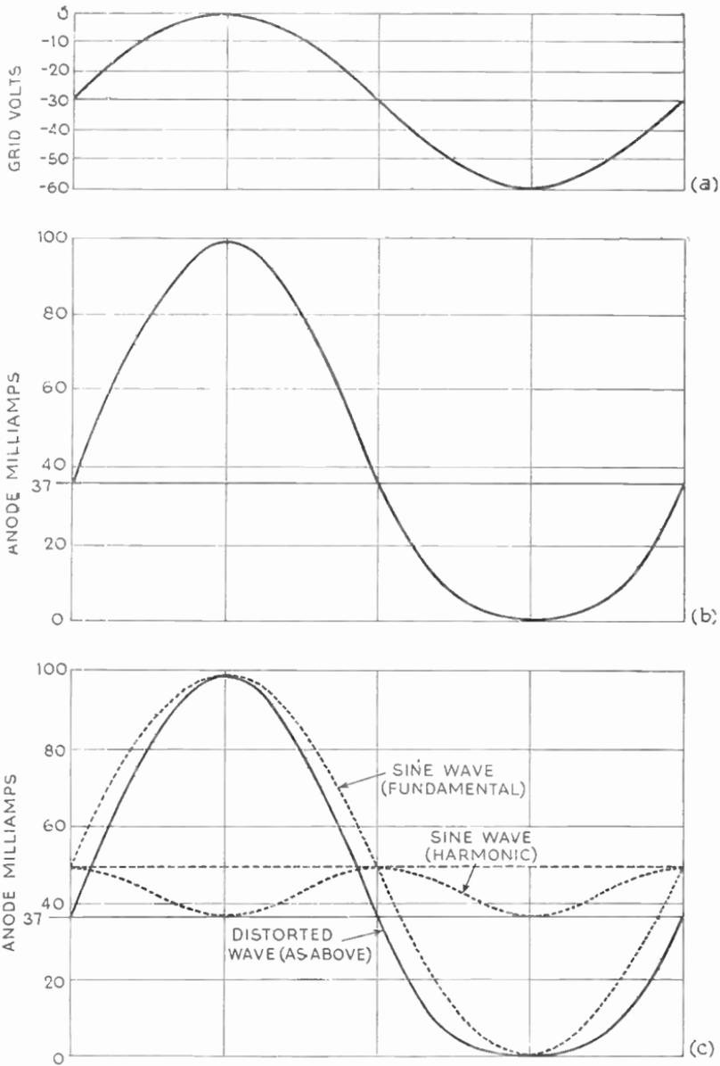
**Fig. 20.3**—Showing that the distorted output (b) resulting from applying the input (a) to the valve whose characteristics are given in Fig. 20.2 is equivalent to (c) the combination of an undistorted wave with its second harmonic
