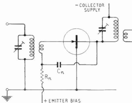
Fig. 22.13—Method of neutralizing a transistor stage of r.f. amplification
