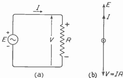
Fig. 5.8—(a) A.c. circuit at the instant when the e.m.f. is at its positive maximum, and (b) the corresponding vector diagram
