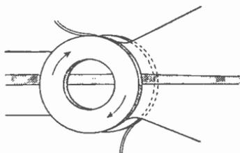
Fig. 21.4—Arrangement of deflector coils in a cathode-ray tube
