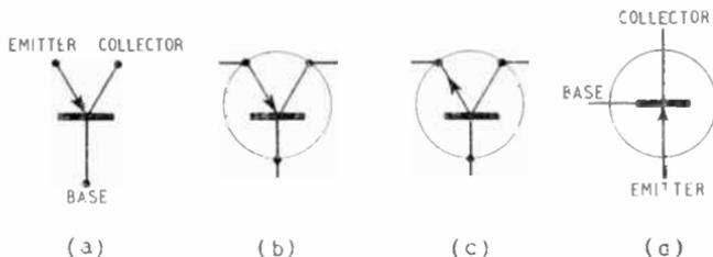
Fig. 10.16—(a and b) Usual symbol for transistor (point-contact or *p-n-p* junction types); the “envelope” is optional. The *n-p-n* type is distinguished by a reversed arrow head (c). Symbol *d* is more appropriate to represent *p-n-p* junction types
