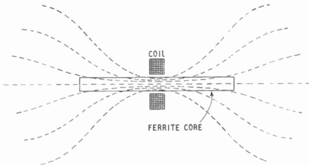
**Fig. 15.17—The concentrating effect of a suitable magnetic core on the magnetic field of the waves greatly increases the effectiveness of a small coil as an aerial**
