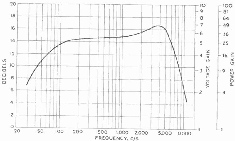
Fig. 20.1—A typical a.f. gain/frequency curve, with logarithmic scales in both directions
