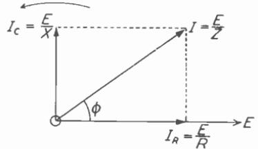
Fig. 6.12—Vector diagram relating to Fig. 6.11
