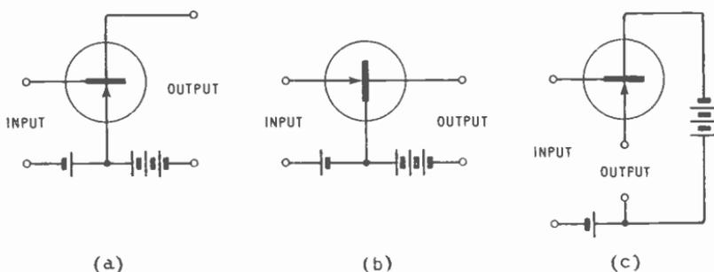
Fig. 22.4—The three basic amplifier configurations of a transistor, corresponding to Fig. 22.3
