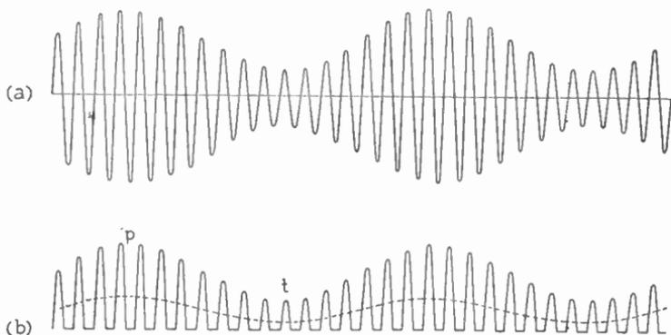
Fig. 16.1—(a) Sample of an amplitude-modulated carrier wave, similar to Fig. 13.5 c. The average value of each cycle is zero; but if one half of each is eliminated (b) the average value of the other halves, shown dotted, fluctuates in the same manner as the modulating waveform (e.g., Fig. 13.5 a)
