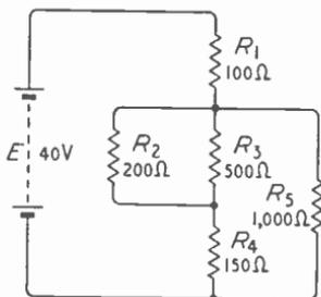
Fig. 2.9—The current through and voltage across each resistor in this complicated network can be calculated by applying the two simple rules derived from Figs. 2.7 and 2.8
