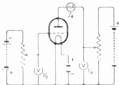
Fig. 9.4— Circuit for taking characteristic curves of a triode
