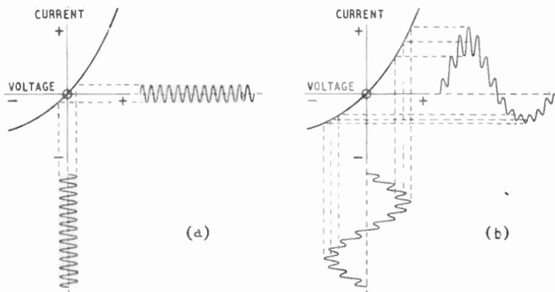
Fig. 19.4—Showing the effect of adding a strong signal to a weak signal through a non-linear device such as a valve. The amplitude of the weak signal is varied (or modulated) by the strong
