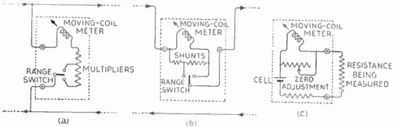
Fig. 2.13—Showing how a single moving-coil indicating instrument can be used for measuring (a) voltage, (b) current, (c) resistance. The moving coil and pointer attached are shown diagrammatically
