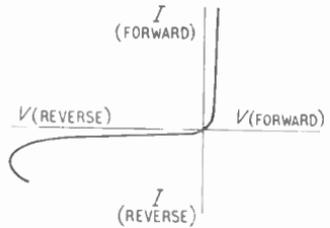
Fig. 10.10—Typical characteristic curve of a germanium rectifier
