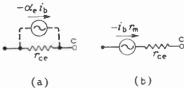
Fig. 22.7 — If common-emitter symbols are used, these collector arms should be substituted for those in Fig. 22.6
