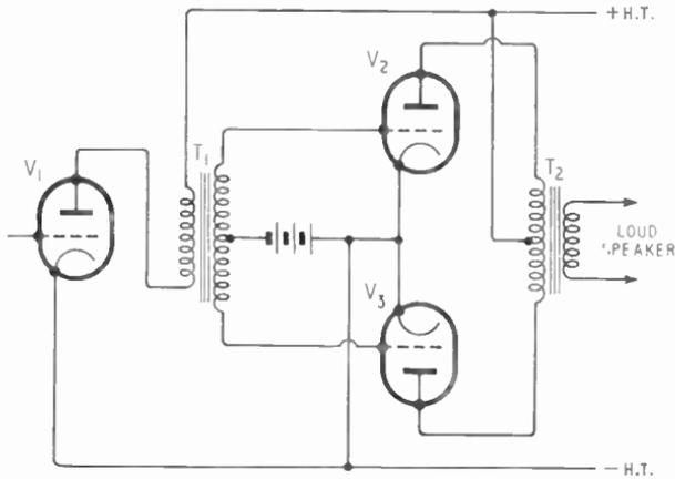
Fig. 20.20—Two output valves,  $V_1$  and  $V_2$ , in push-pull
