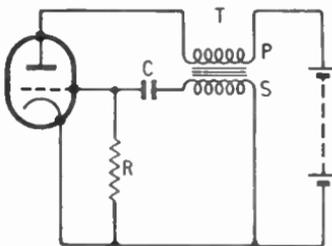
Fig. 21.8—Blocking oscillator circuit
