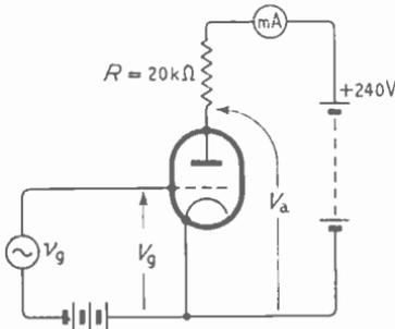
Fig. 11.1—Simple voltage-amplifier circuit
