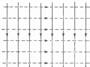
Fig. 15.6—Relative direction of electric (full line) and magnetic (broken line) fields in an electromagnetic wave advancing towards the viewer
