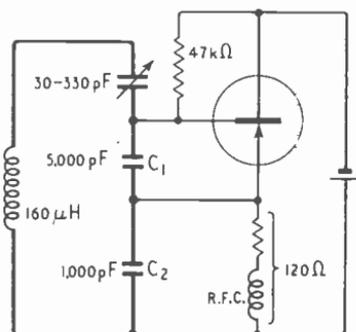
Fig. 22.14—A transistor r.f. oscillator, using the Gouriet circuit to stabilize frequency
