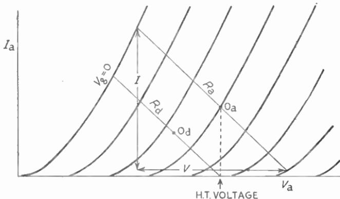
Fig. 20.10— $R_d$  is a typical load line for a direct resistance load.  $R_a$  represents a load having negligible resistance to d.c. and the same resistance to a.c. as  $R_d$
