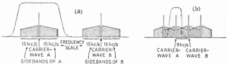
Fig. 18.4—At (a) is shown how broadcasting stations' carrier waves ought to be spaced on the frequency scale in order to permit full reception of each without interference from others. How they actually are spaced (b), shows that interference is almost inevitable if full reception of sidebands is attempted
