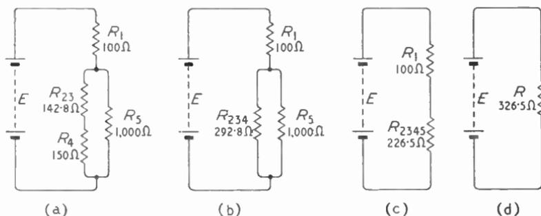
Fig. 2.10—Successive stages in simplifying the circuit of Fig. 2.9.  $R_1$  stands for the single resistances equivalent to  $R_1$  and  $R_3$ ; and so on.  $R$  represents the whole system
