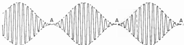
Fig. 13.6—Carrier-wave modulated to a depth of 100%. At its minima (points A) the r.f. current just drops to zero
