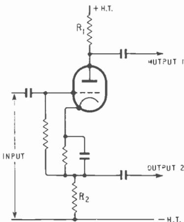
Fig. 20.21—The "concertina" phase-splitter circuit as an alternative to the transformer  $T_1$  in Fig. 20.20
