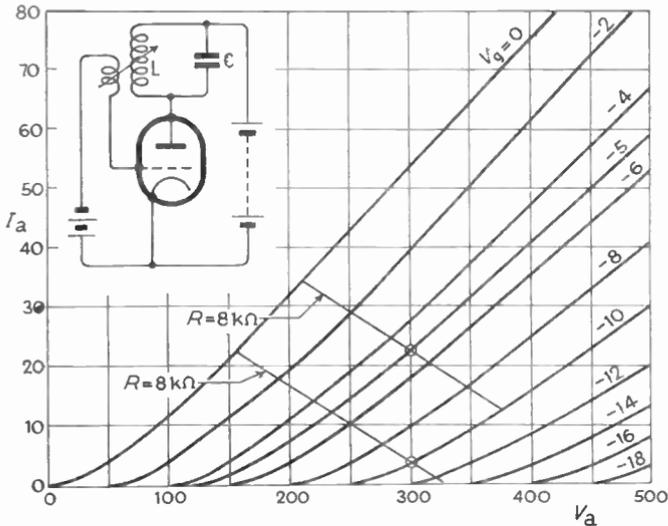
**Fig. 12.10**—The oscillatory circuit LC is equivalent at resonance to a high resistance  $R$  and the voltage across it can be derived from a load line on the valve characteristic curves. From this follows the proportion to be fed back to the grid to sustain oscillation
