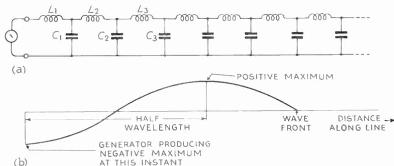
Fig. 14.5—(a) Electrical representation of the generator end of a transmission line, and (b) instantaneous voltage (and current) diagram  $\frac{1}{2}$  of a cycle from the start of generating a sine wave
