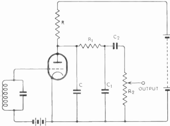
Fig. 16.16—Anode-bend detector circuit, which should be compared with Fig. 16.12
