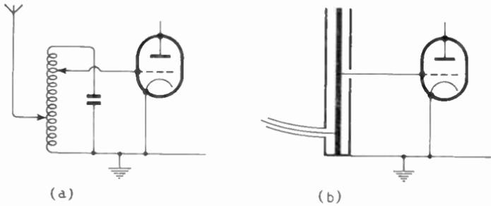
Fig. 14.9—(a) Conventional aerial input circuit using “lumped” components, and (b) distributed equivalent using a quarter-wave coaxial line
