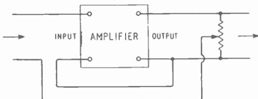
Fig. 20.16—Showing in principle how negative voltage feedback is applied to an amplifier
