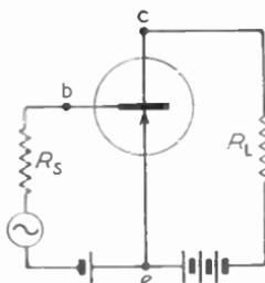
Fig. 22.8—Theoretical common-emitter transistor circuit showing source and load resistances,  $R_s$  and  $R_L$ .
