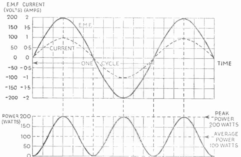
Fig. 5.2—Time graphs of e.m.f., current and power in the circuit Fig. 5.1
