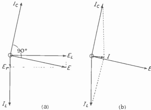
Fig. 8.11—(a) Modification of Fig. 8.9 to allow for the presence of resistance as in Fig. 8.10
