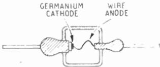
Fig. 10.9—Construction of a point-contact germanium rectifier
