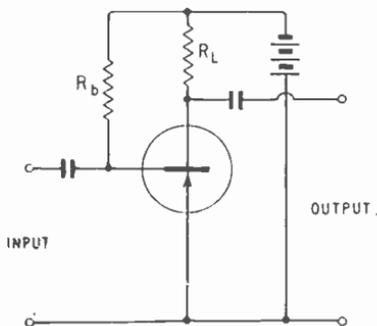
Fig. 22.9—This method of applying base current bias to a transistor, via  $R_b$ , is unsatisfactory in practice
