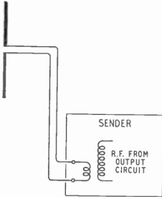
Fig. 15.13 (left)—A simple dipole connected to a sender (or receiver) by means of a matched-impedance transmission line
