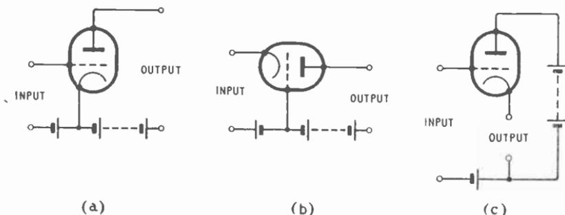
Fig. 22.3—The three basic amplifier configurations of a valve
