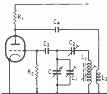
parallel-fed via  $C_4$ .  $R_2$  and  $C_3$  are the usual grid leak and capacitor for making the oscillation generate its own negative bias (p. 217).
