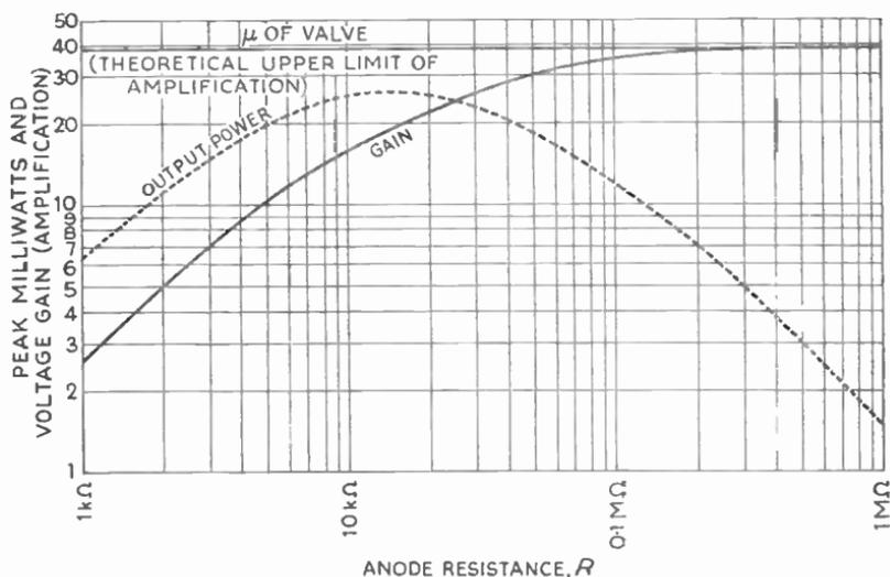
Fig. 11.4—The full line shows how the voltage amplification depends on the value of load resistance  $R$ . It is calculated for a valve with  $\mu = 39$  and  $r_a = 14.5\text{ k}\Omega$ . The dotted line shows the peak milliwatts delivered to  $R$  for a grid input of  $1\text{ V}$  peak.
