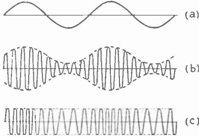
Fig. 13.8—Curve (a) represents 2 cycles of audio frequency used to modulate a r.f. carrier wave. If amplitude modulation is used, the result is represented by (b); if frequency modulation, by (c)
