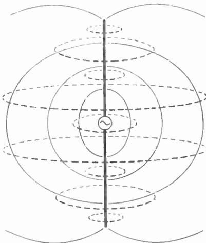
Fig. 15.4—The distributed inductance and capacitance in Fig. 15.2 are better indicated by drawing a few lines of force. The full lines are electric and the broken lines magnetic
