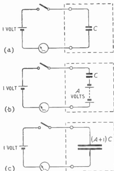
already there, and the energy fed through  $C_{ag}$  would tend to damp out and reduce the signal voltage. In a third case the voltage fed back from the anode might be  $90^\circ$  out of phase with that already present, and would therefore produce the same effect on the grid signal as a reactance.
