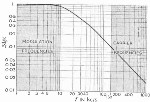
Fig. 16.11—The filtering action of  $R_1$ ,  $C_1$  in Fig. 16.10 is here shown as a graph of  $V_0/V_1$  against frequency
