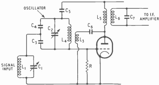
**Fig. 19.5**—Typical additive frequency-changer, in which a single valve serves as both modulator and generator of the local oscillations
