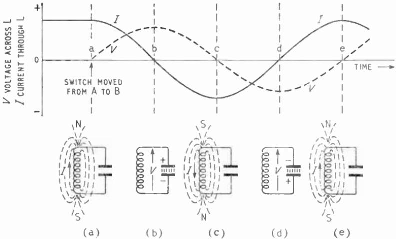
**Fig. 12.2**—Sequence of events in Fig. 12.1 after the switch has been moved to B. Stages *a* to *e* cover one complete cycle of oscillation
