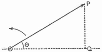
Fig. 5.5—The Fig. 5.4 vector after having turned through an angle,  $\theta$
