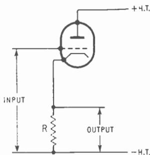
must be less than 1, no matter what the characteristics of the valve and the value of  $R$ . The value of  $B$  in the formula given on p. 312 is 1, so the "gain" is  $A/(1 + A)$  as just found. If  $A$  is made large by using a high- $\mu$  valve and high  $R$ , the output is very nearly as much as the input, but never quite as much. A stage that gives out less voltage than is put in may not appear worthy of further attention; but it is too soon to jump to such a conclusion.
