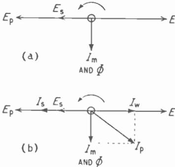
Fig. 7.8—Simplified vector diagrams for a transformer; (a) unloaded, and (b) loaded
