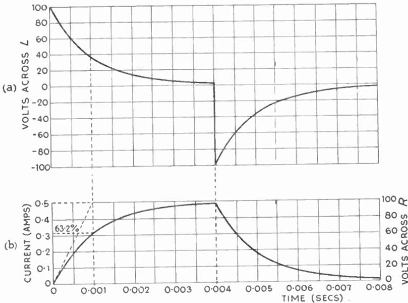
Fig. 4.9—Curves showing the current and voltage in the circuit of Fig. 4.8 when the switch is moved first to A and then to B
