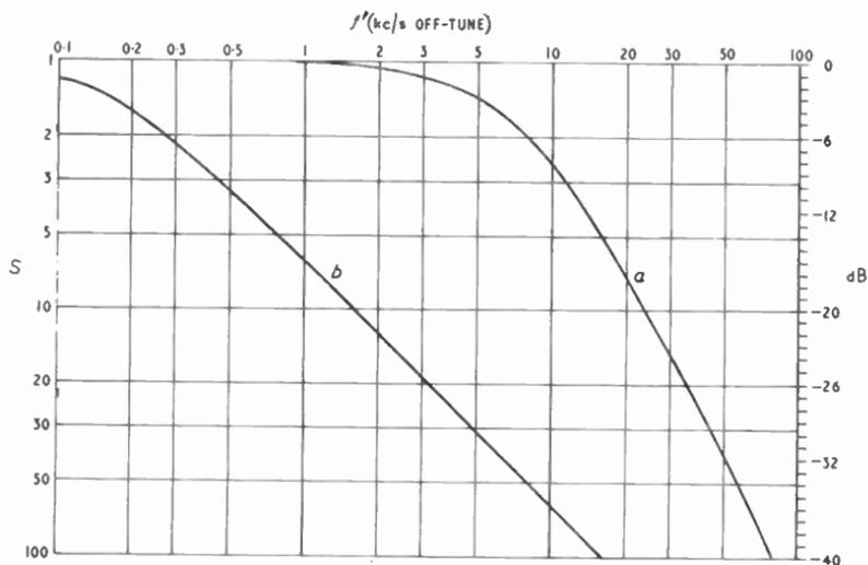
**Fig. 18.7**—Comparison on an equal-gain basis of a stage of amplification with two tuned circuits (curve  $a$ ) with a single tuned circuit given a high magnification by positive feedback ( $b$ )
