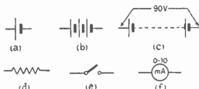
Fig. 2.4—A first instalment of circuit-diagram symbols, representing (a) a cell, (b) a battery of three cells, (c) a battery of many cells, (d) a resistor, (e) a switch, and (f) a milli-ammeter
