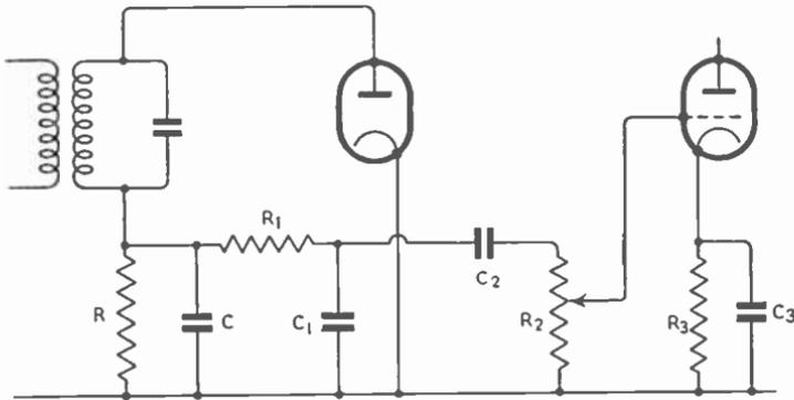
Fig. 16.12—Typical detector circuit, in which R is the load resistor, C the reservoir,  $R_1$ ,  $C_1$  the r.f. filter,  $R_2$ ,  $C_2$  the z.f. filter,  $R_2$  the volume control,  $R_3$  the biasing resistor, and  $C_3$  its by-pass
