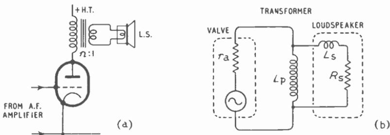
Fig. 20.9—(a) Circuit of output stage in its simplest form. Electrically this can be approximately represented by the generator circuit (b)
