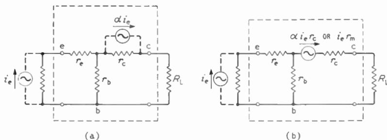
Fig. 22.5—Equivalent T circuits of a common-base-connected transistor: (a) current generator; (b) voltage generator
