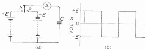
Fig. 6.2—If the generator in Fig. 6.1 consisted of the periodically switched batteries as shown at *a*, the waveform would be as at *b*, and the current (assuming a certain amount of resistance) could be calculated as discussed in connection with Fig. 3.6
