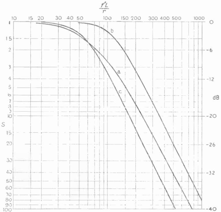
Fig. 19.12—Comparison between the overall resonance curve for a pair of similar tuned circuits, (a) uncoupled, and (b) “critically” coupled. Curve c is the same as b but shifted to the left to represent a halving of resistance
