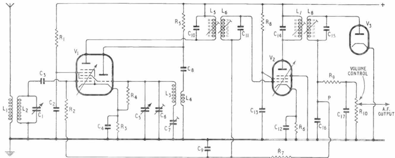
Fig. 19.21—Circuit diagram of a typical superheterodyne receiver from aerial to volume control, including frequency-changer, i.f. amplifier and detector stages, with automatic gain control
