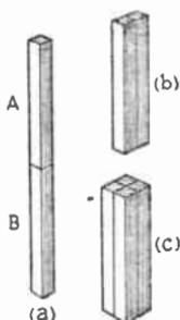
Fig. 2.11—The rule for resistances in series proves that doubling the length of a uniform conductor doubles its resistance (a). By the rule for resistances in parallel, doubling its cross-section halves its resistance (b); and doubling its diameter quarters its resistance (c)
