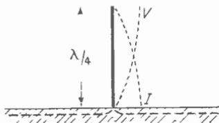
imperfectly conducting earth, it is a common practice to connect the lower end of the aerial to a radial system of copper wires. An insulated set of wires stretched just above the ground is known as a *counterpoise*. Alternatively, to avoid tripping up people or animals, the wires are often buried just below the surface, as shown dotted in Fig. 15.12.
