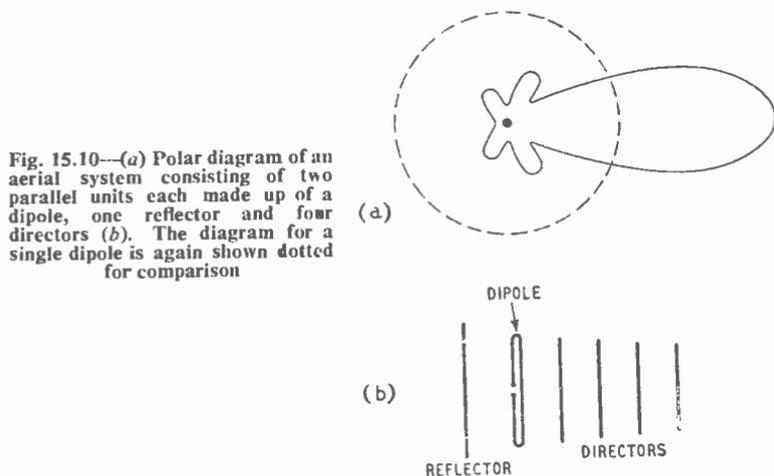
Fig. 15.10—(a) Polar diagram of an aerial system consisting of two parallel units each made up of a dipole, one reflector and four directors (b). The diagram for a single dipole is again shown dotted for comparison
