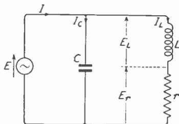
another.) The angle between  $E$  and  $I_L$  is now less than  $90^\circ$ , but since we are assuming that the resistance in the  $C$  branch is negligible we must draw the  $I_C$  vector at right angles to  $E$ . We are also assuming that  $I_C = I_L$ , but as they are now not exactly opposite in phase the result of combining them is a small current  $I$ , being the current supplied by the generator. To avoid confusing Fig. 8.11*a* this combining process has been transferred to Fig. 8.11*b*.
