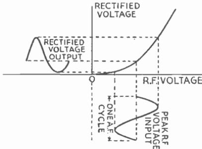
Fig. 16.15—Graph of one-way or z.f. voltage derived from a rectifier is plotted against r.f. input voltage. It enables the distortion of the modulation to be ascertained for any r.f. amplitude and depth of modulation. The input curve here represents 50% modulation
