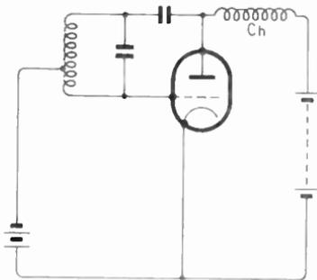
Fig. 12.7—Parallel-fed Hartley circuit with the anode current supplied through a choke  $C_h$ . The grid bias is series-fed
