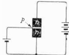
Fig. 10.12 — Applying bias of the right polarity to the middle layer causes increased current between the outers
