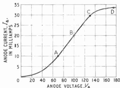
Fig. 9.3—Characteristic curve of a diode
