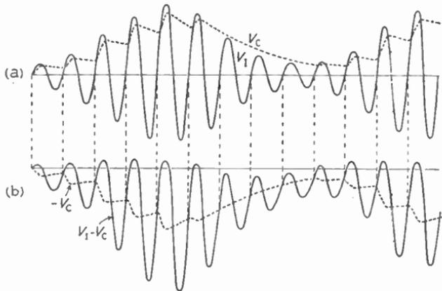
Fig. 16.7—In diagram *a*,  $V_I$  represents a modulated r.f. input voltage and  $V_C$  the resulting output voltage. In diagram *b*, the full line shows  $V_I - V_C$ ; i.e., the voltage across the diode
