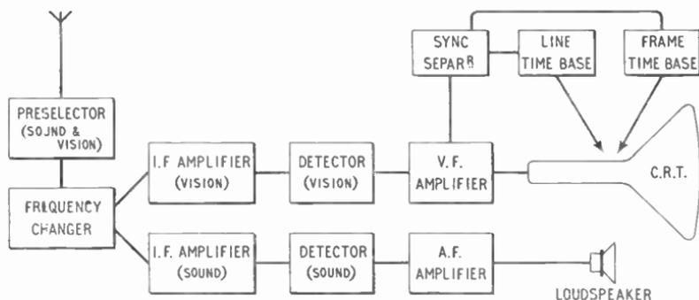
Fig. 21.10—Block diagram of a television receiver
