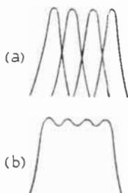
Fig. 19.15—"Stagger-tuning," in which the separate tuned circuits are set to "peak" at slightly different frequencies (as shown at (a)), so that the combined result (b) has a fairly flat top and sharp cut-off
