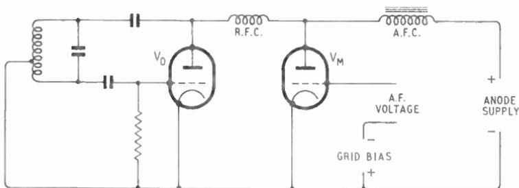
Fig. 13.7—Anode modulation, sometimes called “choke control” modulation. RFC is a r.f. choke for keeping r.f. current out of the modulator circuit
