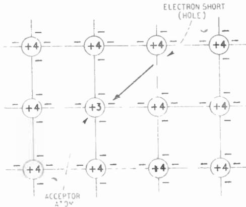
Fig. 10.4—Showing how the perfect crystal is modified when an impurity atom with three valency electrons occupies a place
