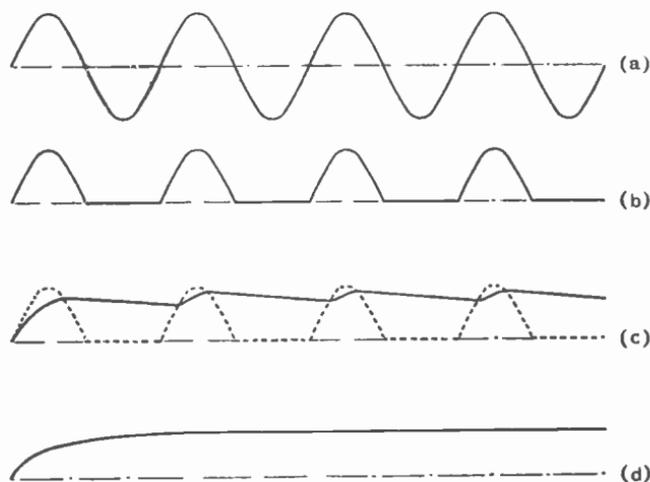
Fig. 23.3—(a) Original a.c.; (b) after rectification; (c) the effect of a reservoir capacitor; (d) after passing through a smoothing filter
