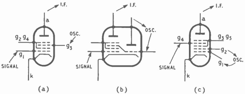
Fig. 19.6—Some frequency-changer valves: (a) hexode; (b) triode-hexode; (c) heptode
