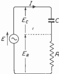
Fig. 6.9—For finding the current,  $I$ , caused by  $E$  to flow in a circuit comprising  $C$  and  $R$  in series, it is helpful to split  $E$  up into the two parts needed to drive  $I$  through  $C$  and  $R$  separately
