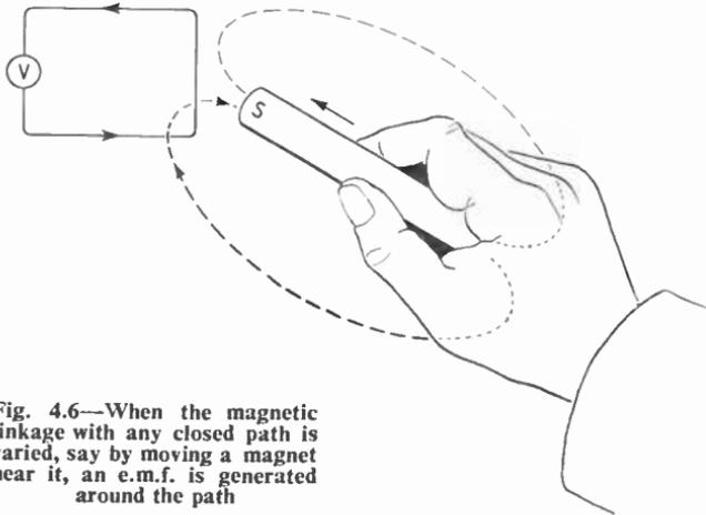
Fig. 4.6—When the magnetic linkage with any closed path is varied, say by moving a magnet near it, an e.m.f. is generated around the path
