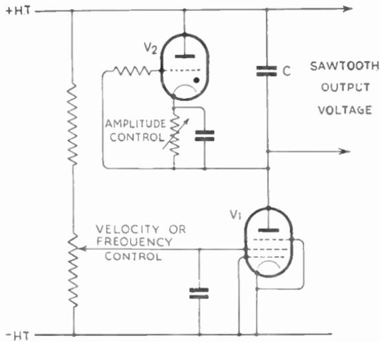
Fig. 21.7—Outline circuit of sawtooth generator
