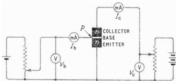
Fig. 10.13—Arrangement, similar to Fig. 9.4, for obtaining characteristic curves of a transistor
