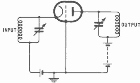
Fig. 19.9—Common-grid amplifier circuit
