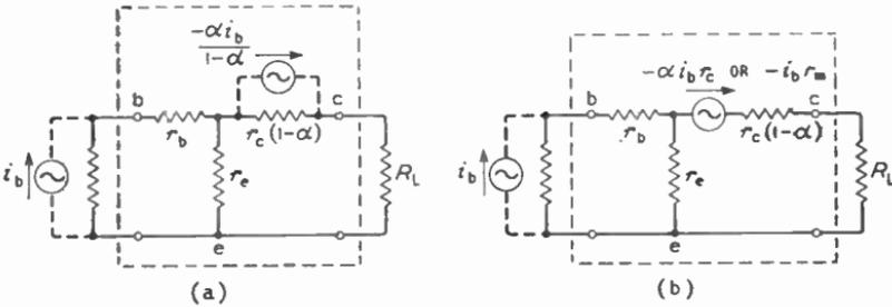
Fig. 22.6—Common-emitter T circuits corresponding to the common-base circuits of Fig. 22.5, using the same symbols
