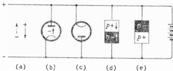
Fig. 10.7—Showing how in diodes the presence or absence of current depends on the presence or absence of the right kind of current-carriers
