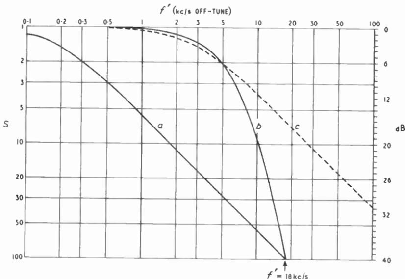
**Fig. 18.8**—Response curves of one ( $a$ ) and six ( $b$ ) tuned circuits on a basis of equal selectivity at 18 kc/s, showing how the six preserve sideband frequencies much better. Curve  $c$  refers to a single tuned circuit with its resonance flattened to give equal response at 5 kc/s off-tune
