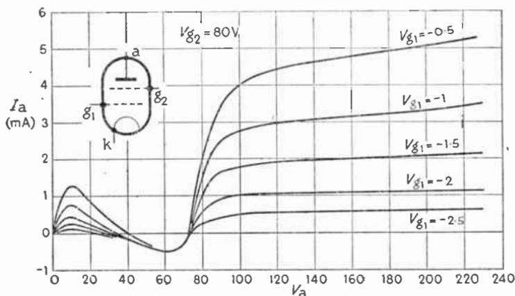
Fig. 17.7—Characteristic curves of a screened tetrode of the original type, which has now gone out of use
