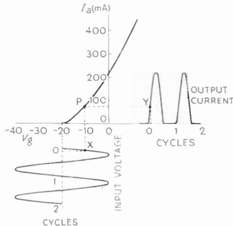
Fig. 13.1 — Illustrating "Class B" operation with the aid of a valve anode-current/grid-voltage characteristic curve
