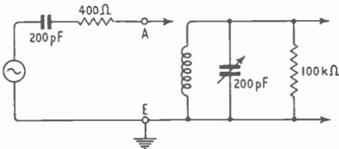
Fig. 17.11—A example of how connecting an aerial directly across the tuning circuit may have very bad effects. The components to the left of the A and E terminals are the circuit equivalent of the aerial
