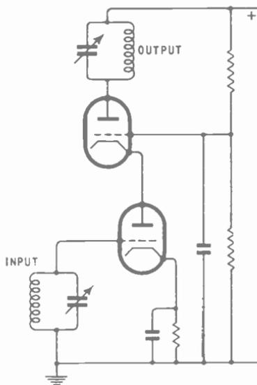
Fig. 19.10—Cascode amplifier circuit
