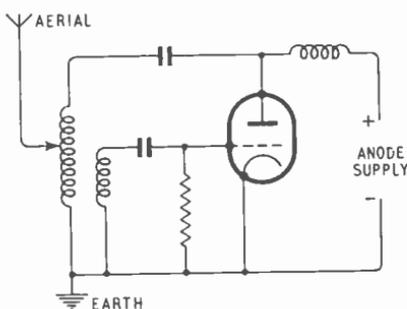
Fig. 13.3—Direct coupling of aerial to the tuned circuit of a self-oscillating sender. The other end is usually connected to earth
