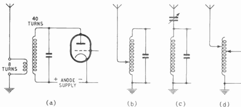
Fig. 13.10—Some of many varieties of method in coupling aerial to sender. *a* is the inductive coupling or r.f. transformer method, worked out in the text for a particular example; *b* is the aerial tapping or auto-transformer; *c* is the series capacitor method; and at *d* the valve is tapped down to reduce the effective load resistance
