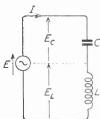
Fig. 8.1—Circuit consisting of an a.c. generator in series with capacitance and inductance
