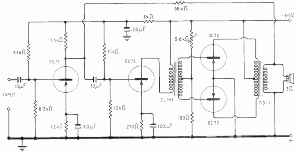
**Fig. 22.11**—Circuit diagram of a three-stage transistor a.f. amplifier, similar in configuration to a valve amplifier but requiring only a small fraction of the power supply. Junction transistors with common emitter are used for all stages. (Courtesy of Messrs. Mullard Ltd.)
