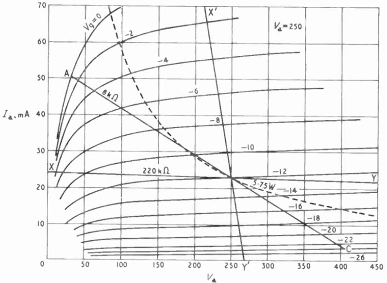
Fig. 20.14—Typical  $I_a$   $V_a$  curves for a small output pentode. The line AOC represents a usual load
