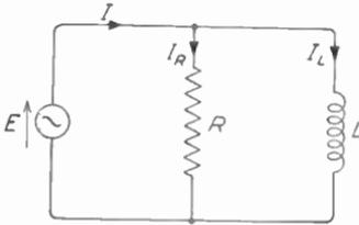
Fig. 7.5—As in Fig. 6.11, the branch currents are  $90^\circ$  out of phase with one another, the only difference being that the reactive current  $I_L$  is  $90^\circ$  later than  $I_R$
