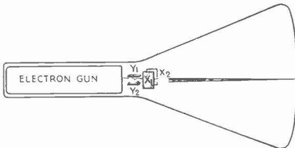
Fig. 21.3—Arrangement of deflector plates in a cathode-ray tube
