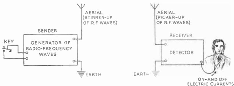
**Fig. 1.8—Elementary wireless telegraph.** Currents flow in the receiving headphones and cause sound whenever the sender is radiating waves
