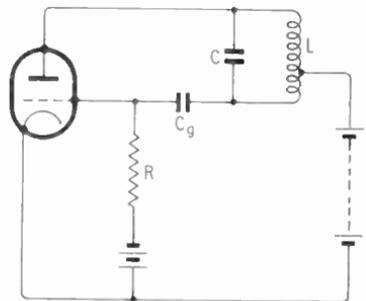
Fig. 12.6—The series-fed Hartley circuit, showing parallel-fed grid bias using a grid leak R and capacitor  $C_g$
