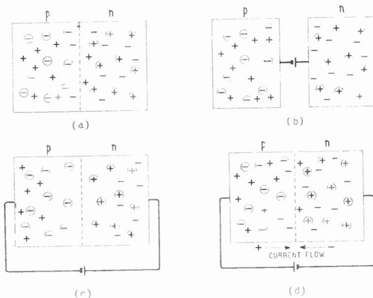
Fig. 10.6—Some mobile charges stray across an undefended frontier (*a*) causing an excess of negative on the *p* side and positive on the *n* side; this can be represented symbolically as at *b*. An external e.m.f. connected + to *n* (*c*) increases this p.d. against itself, sealing the circuit against current flow; but with + to *p* (*d*) it reduces or even removes the p.d. and current flows freely
