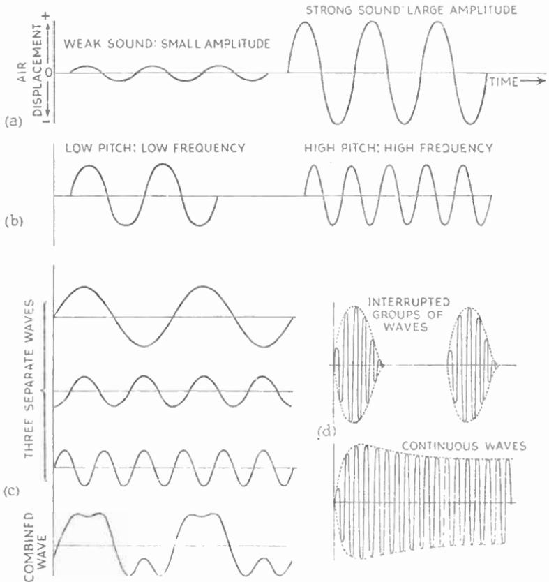
Fig. 1.2—Graphical representation of the four basic ways in which sound (or any other) waves can differ. (a) amplitude; (b) frequency; (c) waveform; and (d) envelope
