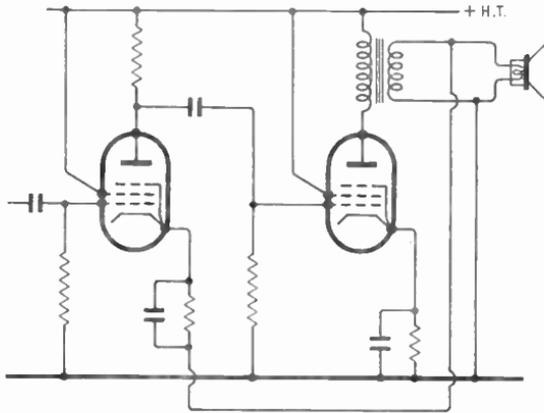
Fig. 20.17—In this negative feedback circuit the whole of the voltage across the loudspeaker is fed back to the last stage but one
