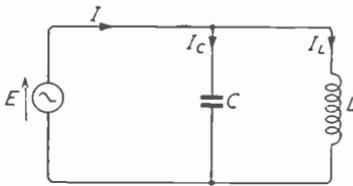
Fig. 8.8—Parallel resonant circuit, which may be compared with the series resonant circuit, Fig. 8.1
