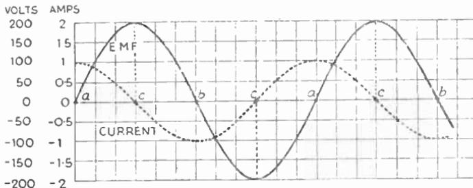
Fig. 6.4—E.m.f. and current diagram for Fig. 6.1, drawn to correspond with Fig. 5.2
