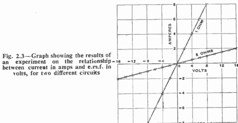
Fig. 2.3—Graph showing the results of an experiment on the relationship between current in amps and e.m.f. in volts, for two different circuits
