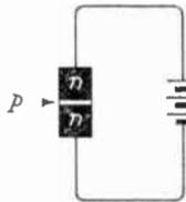
Fig. 10.11—A transistor triode consists of two semi-conductor diodes back-to-back. When it is connected like this, very little current can pass either way
