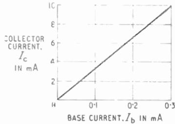
Fig. 10.15 — Collector-current/base-current characteristic of transistor connected as in Fig. 10.13
