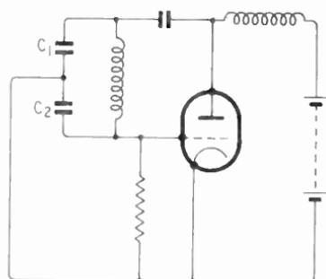
Fig. 12.8—Parallel-fed Colpitts circuit
