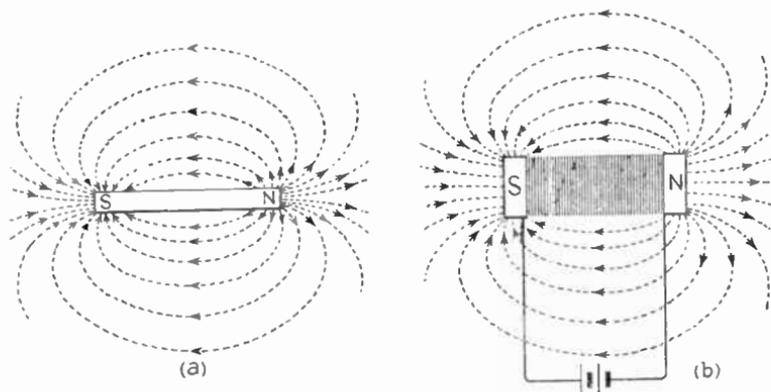
Fig. 4.1—The dotted lines indicate the direction and distribution of magnetic field around (a) a permanent bar magnet, and (b) a coil of wire carrying current
