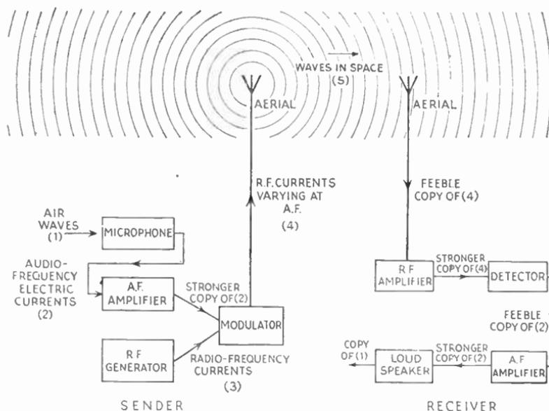
**Fig. 1.9—**The wireless telegraph of Fig. 1.8 converted into a wireless telephone by controlling the output of the sender by sound waves instead of just turning it on and off. In practice it is also generally necessary to use amplifiers where shown
