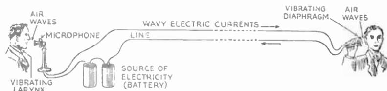
Fig. 1.7—A very simple form of one-way electric telephone, showing how the characteristics of the original air waves are duplicated in electric currents, which travel farther and quicker, and which are then transformed back into air waves to make them perceptible by the listener
