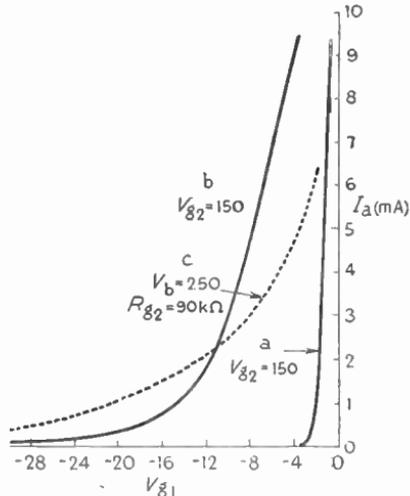
Fig. 19.19— $I_a/V_{g1}$  curves of (a) an ordinary screened pentode, (b) a variable-mu type, and (c) a variable-mu valve with  $g_2$  fed through a resistor so that  $V_{g2}$  rises as  $-V_{g1}$  is increased
