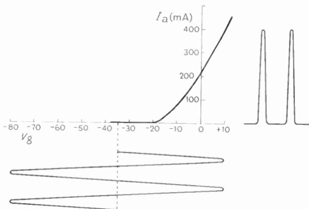
**Fig. 13.2—“ Class C ” operation.** Comparing this with Fig. 13.1, we see that the working grid bias (—35 V in this example) is considerably more than enough to cut off anode current, which flows during only part of the positive half-cycles of signal
