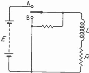
Fig. 4.8—Circuit used for studying the rise and fall of current in an inductive circuit
