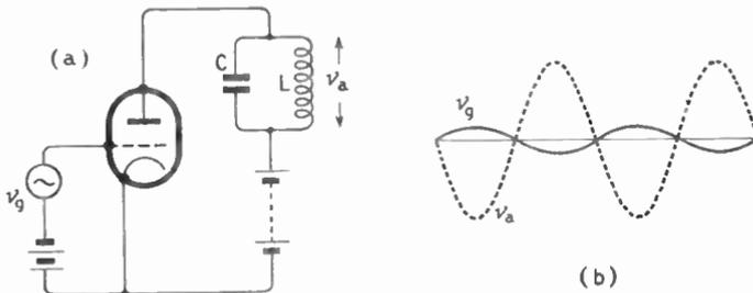
Fig. 12.4—Diagram *b* shows the relative amplitude and phase of grid and anode voltages when their frequency is the same as the natural frequency of the circuit LC
