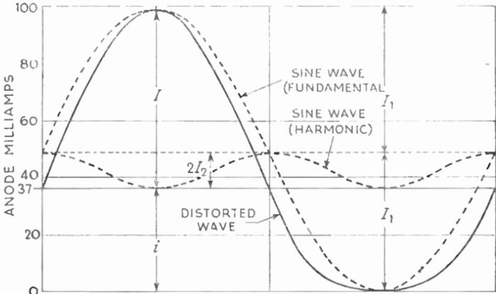
Fig. 20.11—Fig. 20.3 c again, with symbols added for convenience in deriving a formula for percentage second-harmonic distortion.  $I_1$  is the peak value of the fundamental current, and  $I_2$  of the harmonic;  $I$  is the peak current of the larger half-cycle of the distorted current, and  $i$  the smaller
