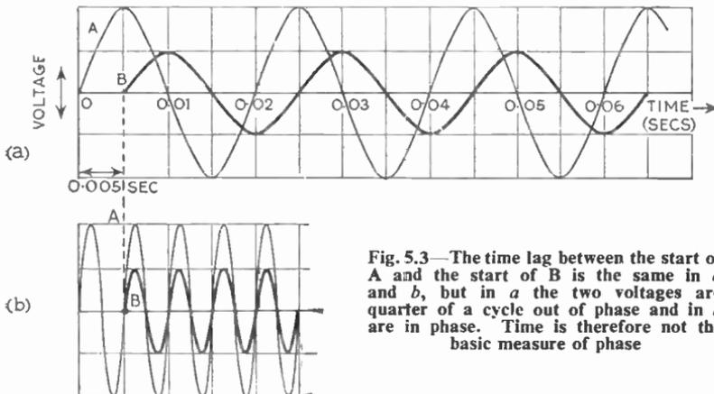
Fig. 5.3—The time lag between the start of A and the start of B is the same in *a* and *b*, but in *a* the two voltages are quarter of a cycle out of phase and in *b* are in phase. Time is therefore not the basic measure of phase
