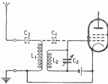
Fig. 17.12—Methods of adapting an aerial to the receiver
