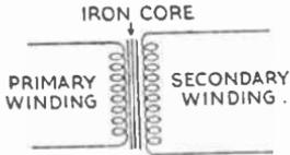
Fig. 4.10—How a transformer is represented in circuit diagrams
