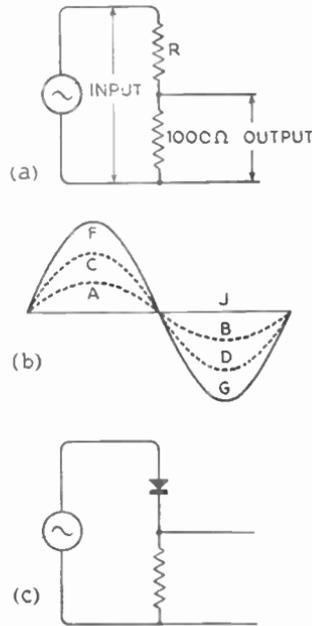
cycle, is, of course, nil when R is not a rectifier. Using the perfect rectifier, the average of the positive half is 64% of the maximum (p. 73), while the negative is, of course, nil; so the average rectified current taken over a whole cycle is 32% of the peak value. Using the rectifier with the graph COB, the negative half-cycle (B in Fig. 16.3b) cancels out half of the positive half (C), which is two-thirds of the input; so the rectified result is less than 11% of the peak input.
