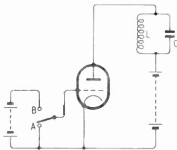
Fig. 12.1—Valve-operated device for setting up oscillations in the circuit LC
