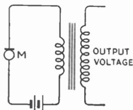
Fig. 13.9—How a carbon microphone (M) is connected to give an a.f. voltage
