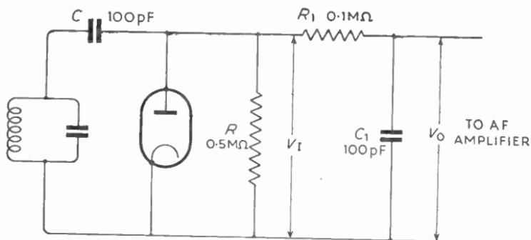
Fig. 16.10—To prevent the r.f. voltages left over after rectification being passed on to the a.f. amplifier, a simple filter,  $R_1$  and  $C_1$ , is commonly used. The component values shown are typical
