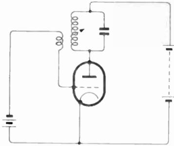
Fig. 12.5—The reaction-coil valve oscillator circuit
