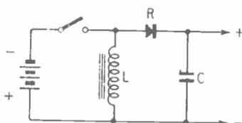
Fig. 23.7—Addition of rectifier to Fig. 23.6 to convert back to d.c.
