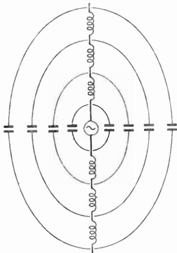
Fig. 15.3—Approximate representation of the distributed inductance and capacitance in the half-wavelength system of Fig. 15.2
