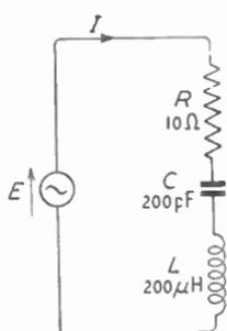
Fig. 8.4—The way the reactances in this circuit vary with the frequency of  $E$ , graphed in Fig. 8.5, leads to interesting conclusions regarding this type of circuit in general
