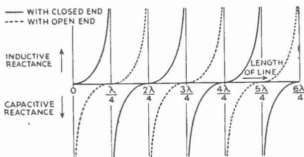
Fig. 14.8—Showing how the reactances of short-circuited and open-circuited lines vary with their length
