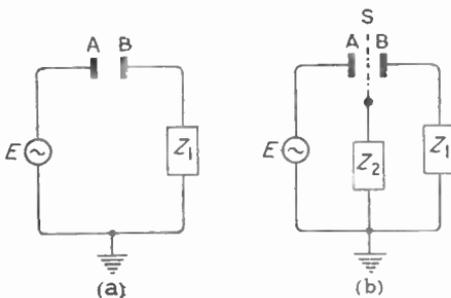
Fig. 17.6—Illustrating the theory of screening
