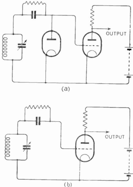
Fig. 16.9—If a diode detector (Fig. 16.8*c* variety) is connected straight to a triode amplifier (*a*), the grid-cathode path of the triode renders a separate diode unnecessary; this is what happens in the grid type of detector (*b*)
