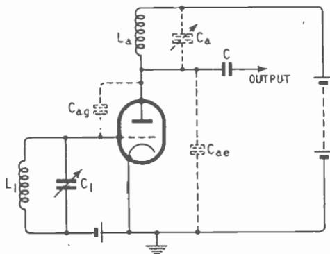
Fig. 17.4—The effect of  $C_{ae}$  in Fig. 17.2 can be overcome by substituting a tuned coupling for the resistance, but there is still trouble due to  $C_{ag}$
