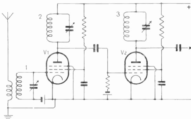
Fig. 17.13—Two-stage r.f. amplifier, using tuned-anode couplings
