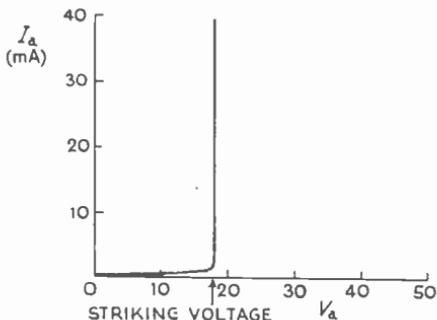
Fig. 21.6—Characteristic curve of a "soft" valve. When it is passing current the voltage across it is nearly constant, and  $r_a$  is therefore nil
