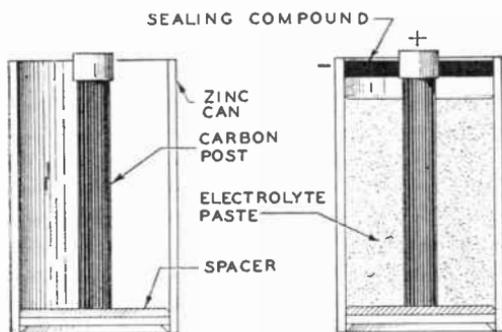
Fig. 7. Outer Shell of a Dry Cell
