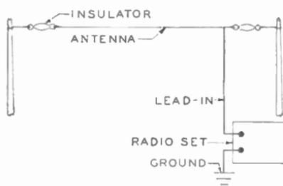
Fig. 1. Simple Antenna System
