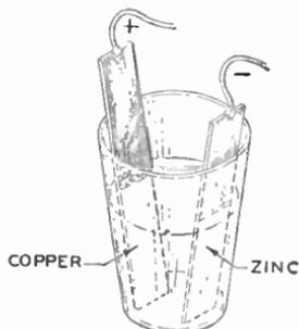
Fig. 5. Simple Voltaic Cell
