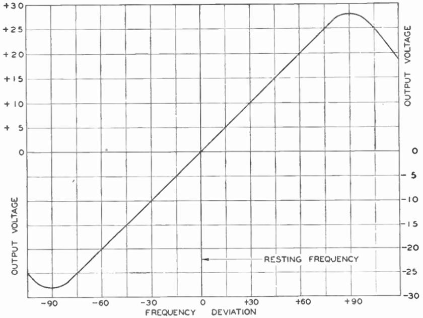
Fig. 7. Curve Showing Output Voltage Produced Due to Variation in Frequency of Signal
