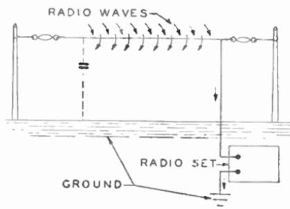
Fig. 3. Action of Radio Waves on Antenna
