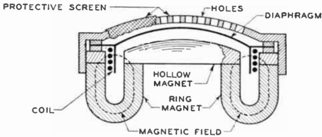
Fig. 7. Cross-Section of a Dynamic Type Microphone
