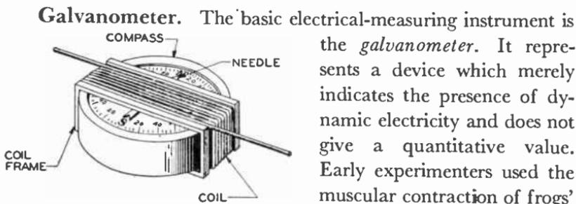
Fig. 1. A Tangent Galvanometer
