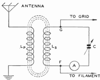
Fig. 2. Antenna Tuning Circuit
