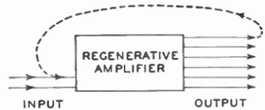
Fig. 2. Regenerative Amplifier. Portion of Output Returns to Input to Strengthen Original Input
