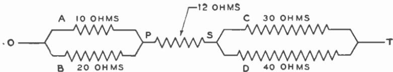
Fig. 7. Resistors Connected in Series-Parallel Circuit
