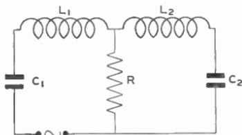
Fig. 5. Direct-Resistance Coupled Circuit
