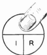
Fig. 14. How to Find the Voltage
