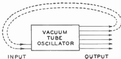
Fig. 3. Vacuum-Tube Oscillator. Sufficient Output Energy Returns to Grid Circuit to Avoid Additional Excitation from Outside Source
