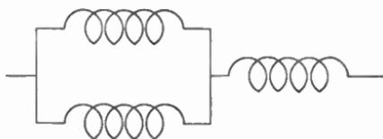
Fig. 6. Inductance Coils Connected in Series-Parallel
