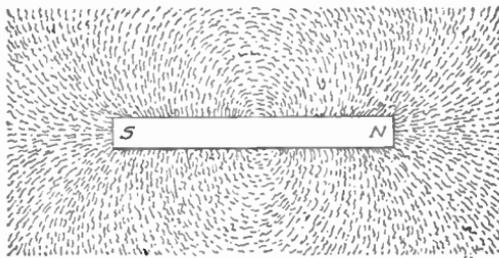
Fig. 6. Magnetic Field of a Bar Magnet
