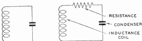
Fig. 1. Oscillatory Circuit
