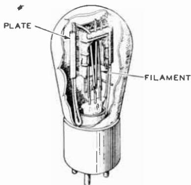
Fig. 1B. Diode or Two-Element Tube
