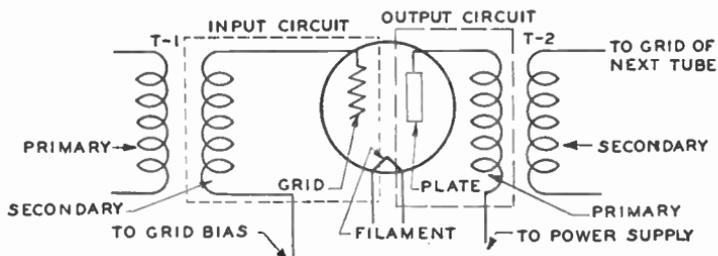
Fig. 1. Radio-Frequency Amplifier Circuit
