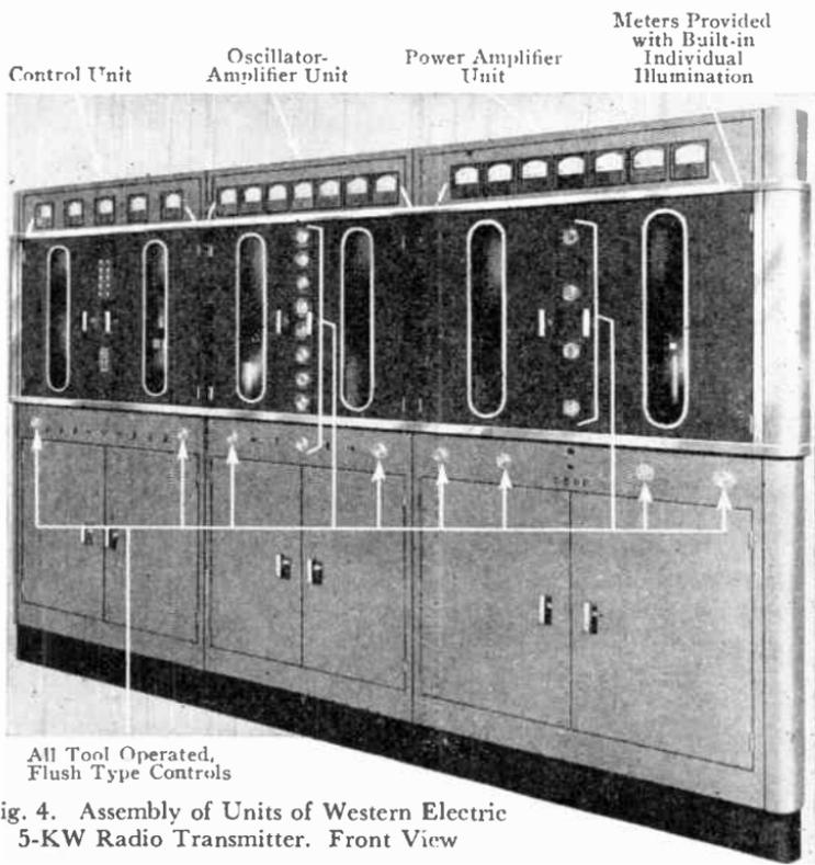
Fig. 4. Assembly of Units of Western Electric 5-KW Radio Transmitter. Front View
