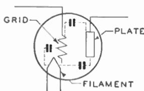
Fig. 10. Capacity Effect between the Different Tube Elements
