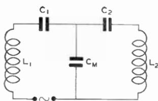
Fig. 4. Direct-Capacitively Coupled Circuit
