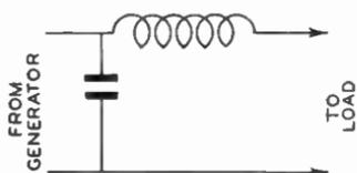
Fig. 13. Filter Which Passes Low Frequencies
