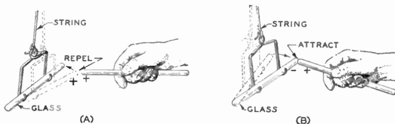
Fig. 3. Illustration Proving Law of Electrostatics
