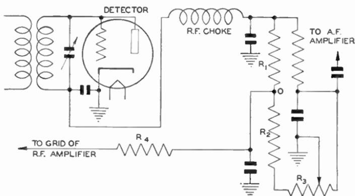
Fig. 12. Automatic Volume-Control Circuit
