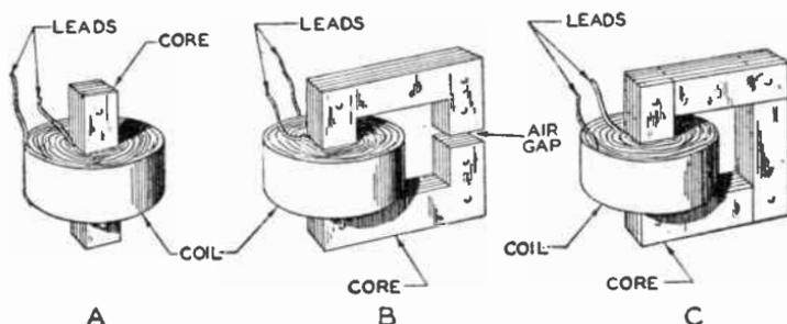
Fig. 7. Construction of Iron-Core Inductance or Choke Coil
