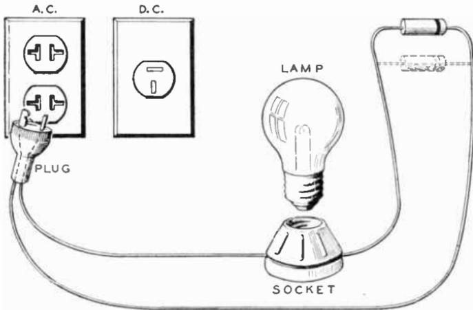
Fig. 7. Diagram of Condensers in Series with Lamp
