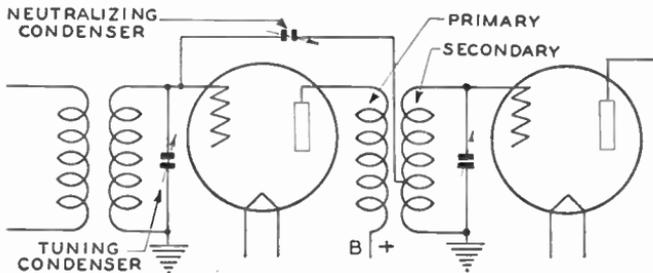
Fig. 4. Neurodyne Method of Controlling Feedback
