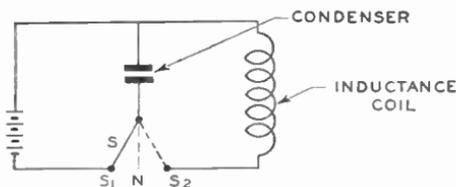
Fig. 2. Method of Charging and Discharging Condenser
