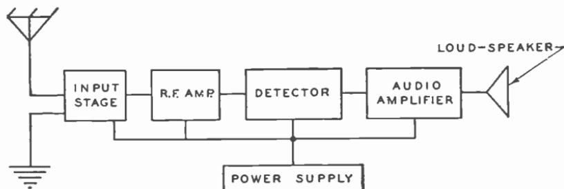
Fig. 1. Block Diagram of Units of Radio Receiver
