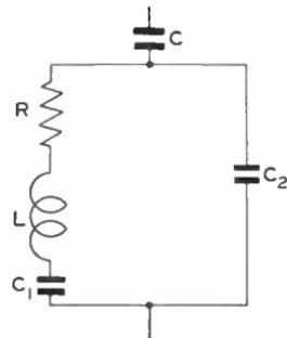
Fig. 10. Equivalent Circuit of a Quartz Crystal
