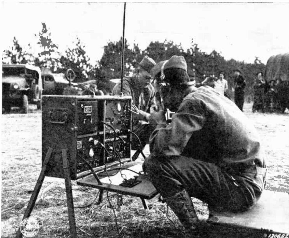
Portable Transmitter and Receiver which Can Be Operated with Phone and Key
