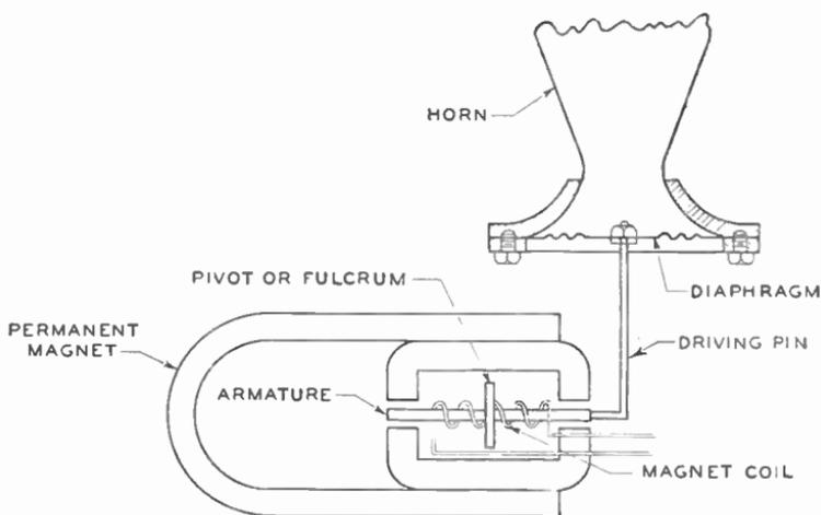
Fig. 3. Balanced-Armature Type of Speaker Unit
