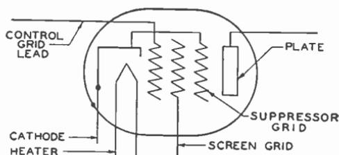
Fig. 13. The Symbol for a Pentode Tube
