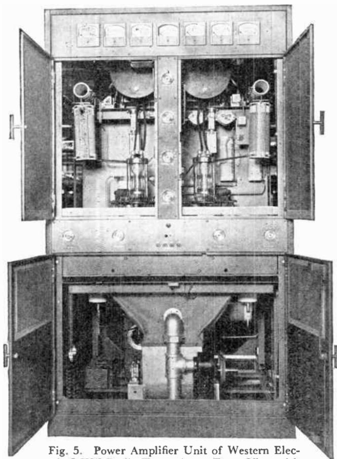
Fig. 5. Power Amplifier Unit of Western Electric 5-KW Radio Transmitter. Front View with Door Open
