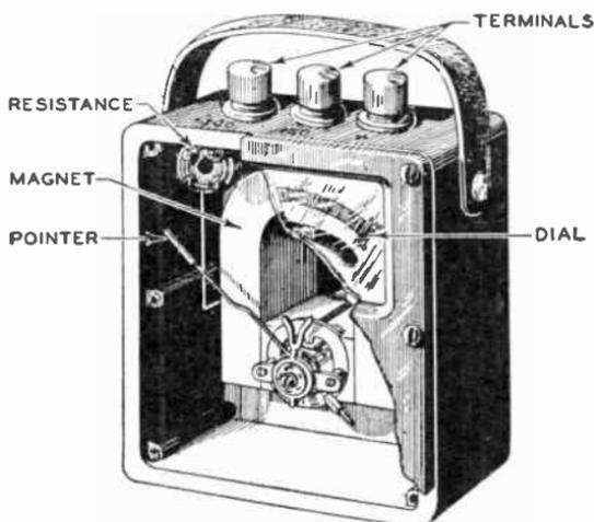
Fig. 2. Cutaway View of a Portable Type Direct-Current Voltmeter with Scales of 0 to 150 or 0 to 300 Volts
