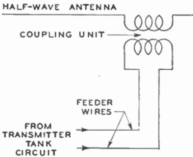
Fig. 5. Current Fed to Antenna by Tuned Feeders
