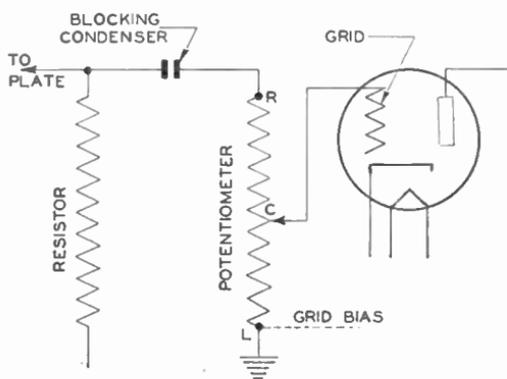
Fig. 10. Resistance-Coupled, Audio, Volume-Control Circuit
