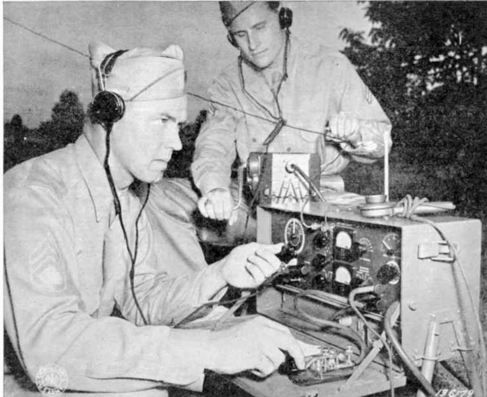
Radio Transmitter in Use in the Field. Man at Right Is Operating the Generator
