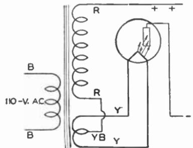
Fig. 2. Diagram of Half-Wave Rectifier Tube Circuit
