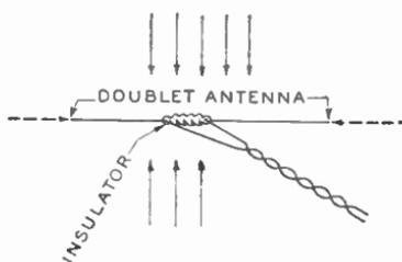
Fig. 4. Doublet Type of Antenna
