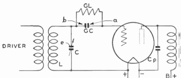
Fig. 6. Diagram of Grid-Leak, Condenser Detector Circuit
