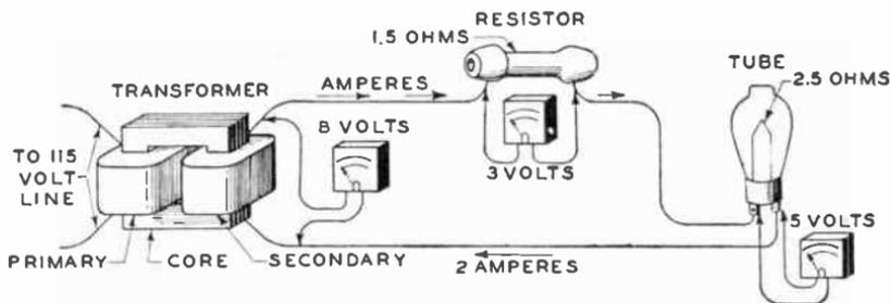
Fig. 15. Diagram Shows Circuit Consisting of Radio-Power Transformer, Resistor, and Tube
