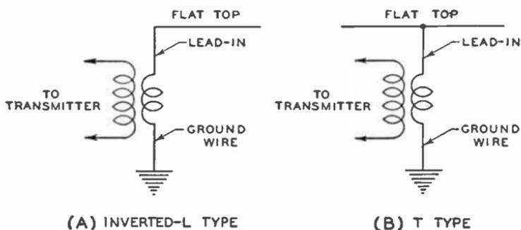
Fig. 1. Two Types of Marconi Transmitting Antennas
