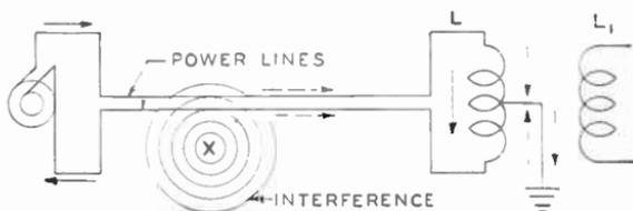
Fig. 7. Desired Current, Indicated by Full Arrows, Flows Around Complete Circuit Setting Up Magnetic Field Around Coil  $L$ . Interference Current Flows Through Coil  $L$  in Phase Opposition, Preventing Setting Up of Magnetic Field. Energy Appearing in  $L_1$  Will Be Due Only to Desired Current Flow in  $L$ .
