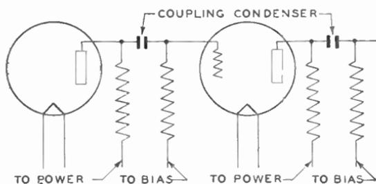
Fig. 12. A Resistance-Coupled Amplifier
