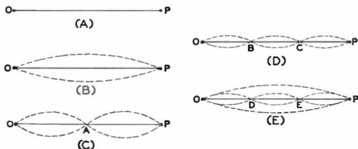
Fig. 6. Diagram Showing How Harmonics and Overtones Are Produced
