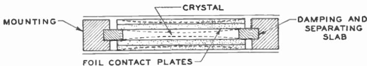
Fig. 6. Cross-Section of a Crystal Type Microphone
