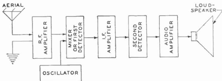
Fig. 1. Route of Radio Signal Through Superheterodyne Receiver
