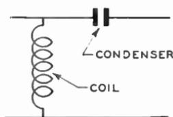
Fig. 14. Filter Which Passes High Frequencies
