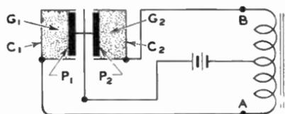
Fig. 3. Circuit Diagram of a Two-Button Carbon Microphone
