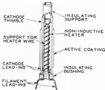
Fig. 9. Illustration Showing the Construction of Heater-Type Filament and Cathode
