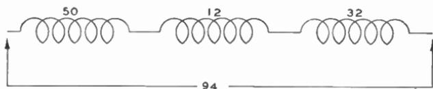
Fig. 4. Inductance Coils Connected in Series
