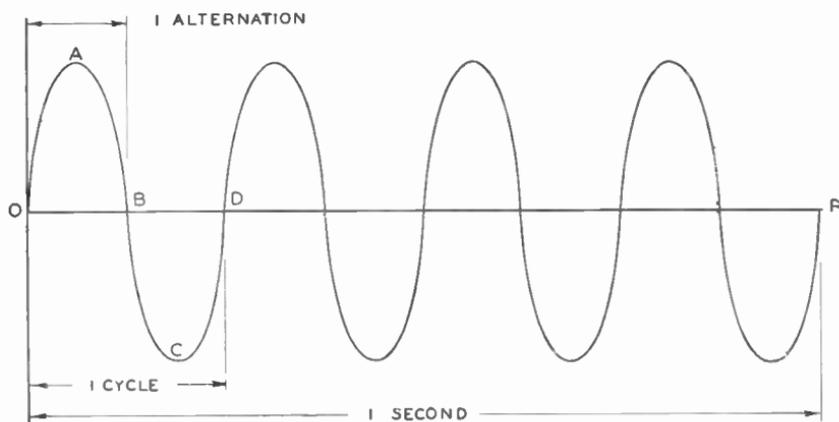
Fig. 2. Diagram Showing Four Cycles of Alternating Current
