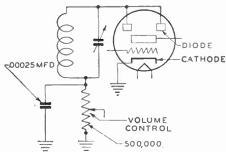
Fig. 6. Connections of Diode Section of 12SQ7
