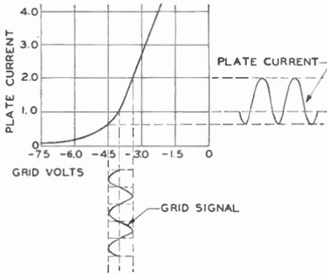
Fig. 6. Curves Showing Result of Changing the Grid Bias
