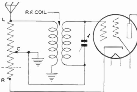
Fig. 8. Combination of Antenna and Grid-Bias Control
