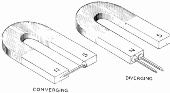
Fig. 4. Diagram Illustrating Laws of Attraction and Repulsion
