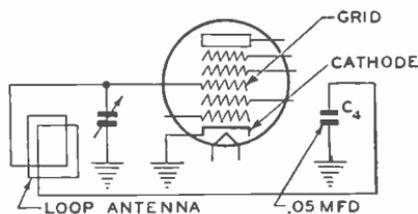
Fig. 3. Signal Input Circuit of Type 12SA7 Tube
