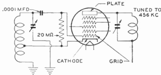
Fig. 4. Oscillator and Output Circuit of 12SA7 Tube
