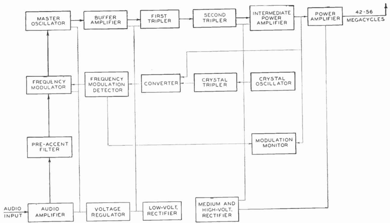
Fig. 4. Block Diagram of Frequency-Modulation Transmitter
