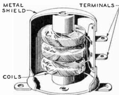
Fig. 4. Radio-Frequency Choke Coil
