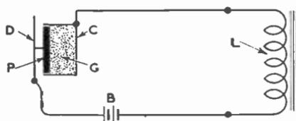
Fig. 1. Circuit for a Simple Carbon-Button Microphone
