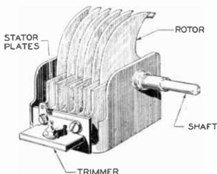
Fig. 8. Variable Condenser for Tuning Radio Circuits
