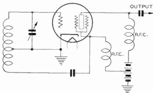
Fig. 12. Electron-Coupled Oscillator
