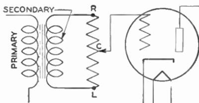
Fig. 11. Method of Connecting Volume-Control to Audio Transformer
