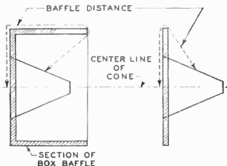
Fig. 5. Box- and Flat-Type Baffles
