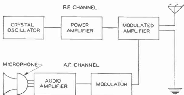
Fig. 2. Block Diagram of Radiotelephone Transmitter
