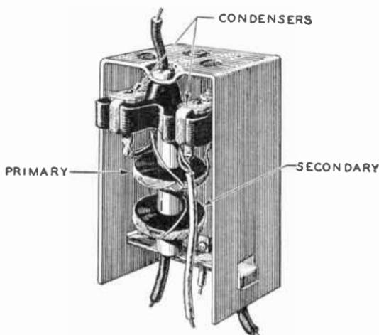
Fig. 7. Intermediate-Frequency Transformer
