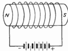
Fig. 5. An Electromagnet
