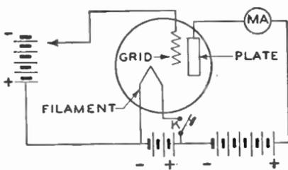
Fig. 6. Circuit Connection for Determining the Amplification Factor of Tube Circuit Connection Arranged for Varying the Grid Voltage
