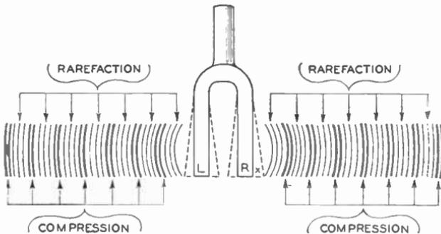
Fig. 3. Sound Waves from a Tuning Fork
