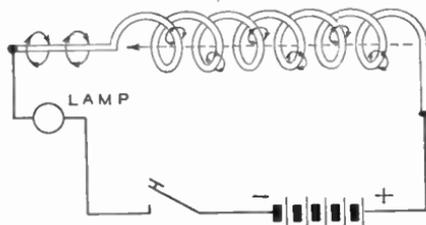
Fig. 15. Magnetic Fields around a Conductor and Coil
