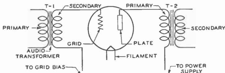
Fig. 2. Audio-Amplifier Circuit
