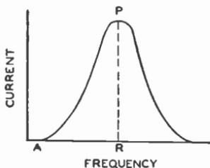
Fig. 8. Curve Showing Increase of Current as Resonant Frequency Is Increased
