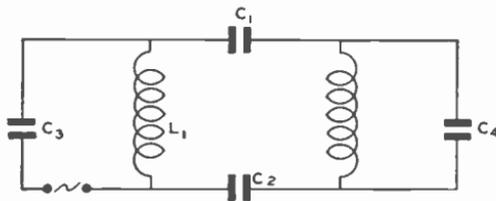
Fig. 7. Indirect-Capacitively Coupled Circuit
