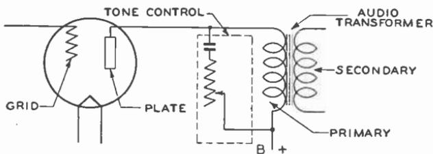
Fig. 13. Tone Control Connected Across Primary of Audio Transformer
