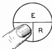
Fig. 12. How to Find the Current
