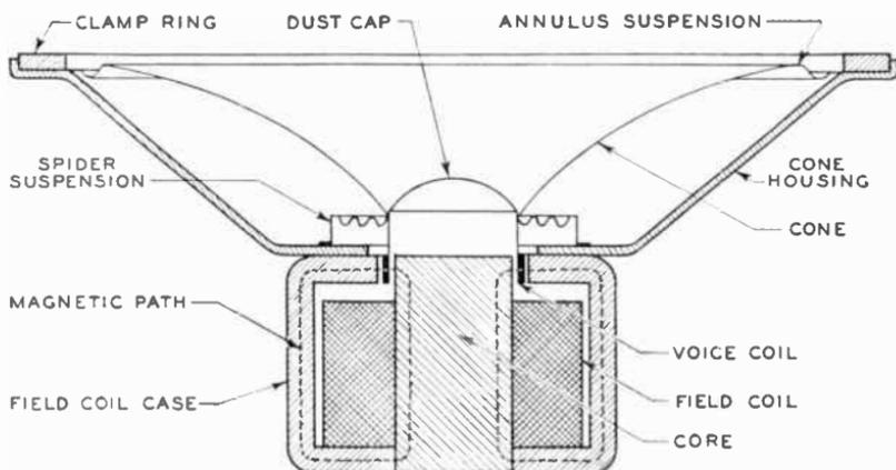
Fig. 4. Cross Section of Electrodynamic Speaker
