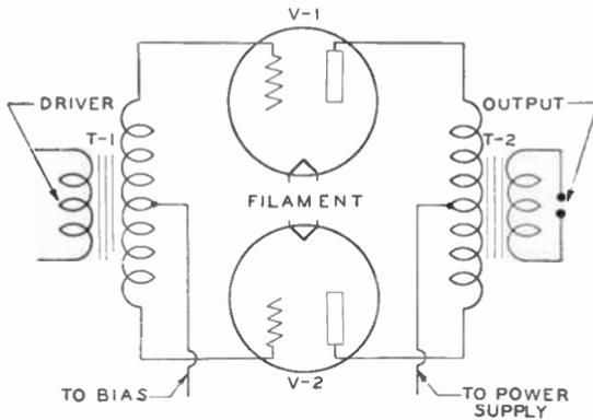
Fig. 9. Diagram Showing a Push-Pull Amplifier Stage
