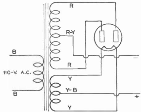
Fig. 5. Full-Wave Rectifier Tube Circuit
