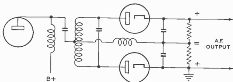
Fig. 6. Discriminator Stage of Frequency-Modulation Receiver
