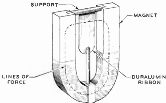
Fig. 8. Diagram Illustrating Principle of a Velocity Microphone
