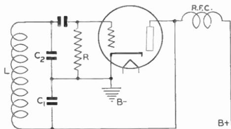
Fig. 7. Colpitts Oscillator Using Capacitive Feedback
