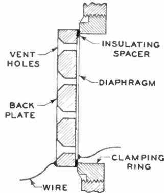
Fig. 4. Cross-Section of a Condenser Type Microphone
