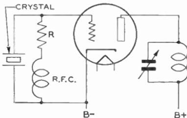
Fig. 9. Quartz-Crystal Oscillator
