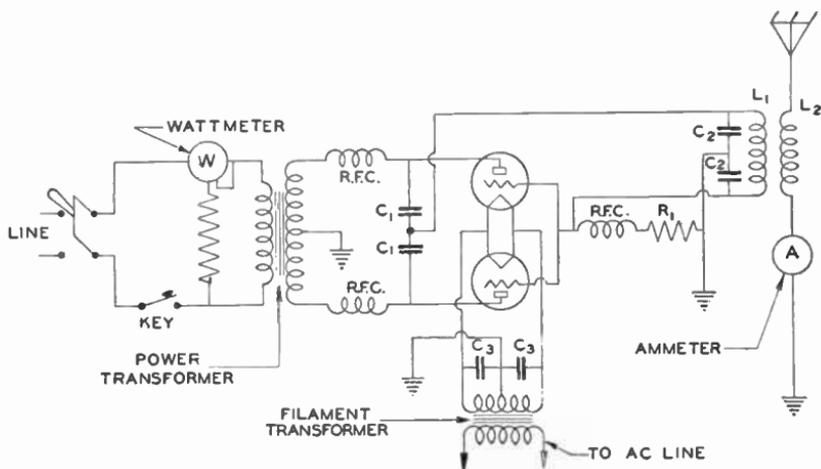
Fig. 3. Self-Rectifying Radiotelegraph Transmitter
