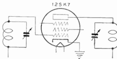
Fig. 5. Intermediate-Frequency Amplifier
