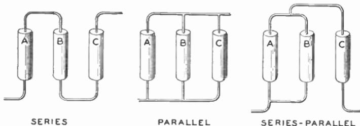
Fig. 16. Diagram Showing Difference between Series, Parallel, and Series-Parallel
