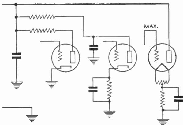
Fig. 8. Method of Using Individual Resistance Units to Obtain Different Voltages for Plate Circuits of Radio Set
