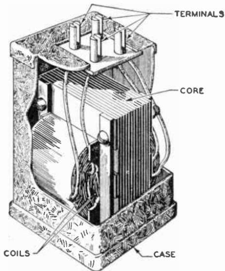
Fig. 7. Iron-Core Transformer
