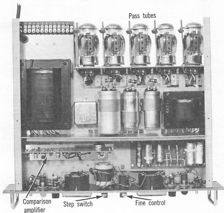
Fig. 5.6 Hybrid (HB) power supply design, employing stepped switch tracking.
