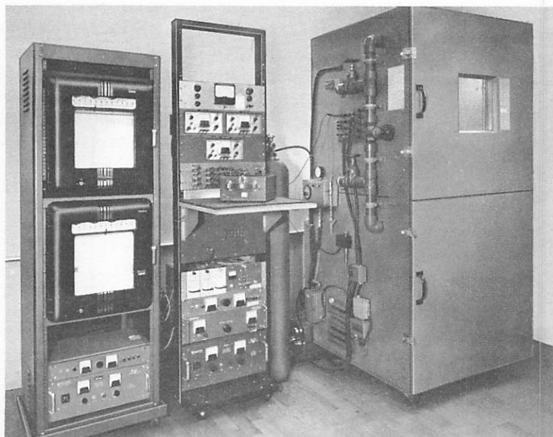
Fig. 8.7b 27 cubic foot temperature control chamber with refrigerated cooling. Recorders at the left are used to measure temperature performance of test samples in the chamber. A miniature air bath chamber with the same basic control mechanism is located under the shelf of the center rack and contains the standard and reference cells.
