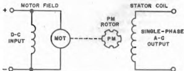
Simple Inverter with Permanent-Magnet Rotor; Single-Phase Output
