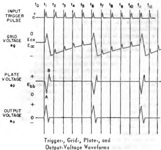
In the quiescent condition (with no trigger pulse applied), V1 is held at plate-current cutoff by the fixed negative bias taken from the voltage divider made up of resistors R1 and R3, and applied through grid resistor R2 and the grid winding of transformer T1 to the grid of V1 (time  $t_0$  on the waveform illustration).
