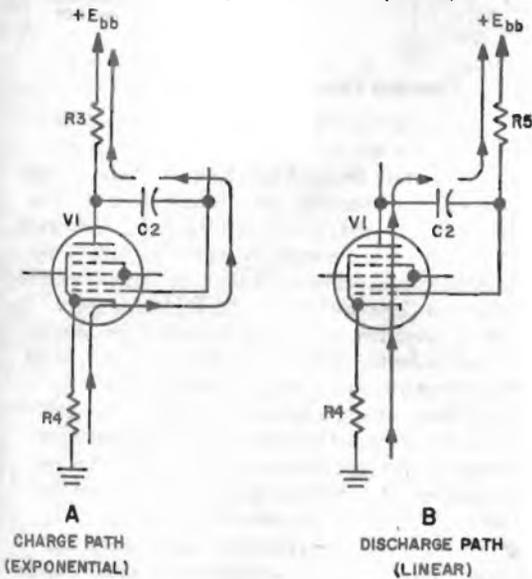
Charge and Discharge Paths for Capacitor C2
