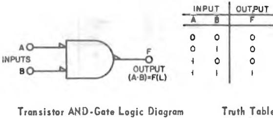
Transistor AND-Gate Logic Diagram Truth Table
