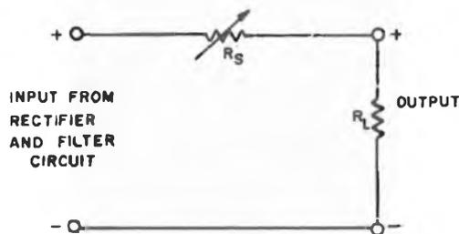
Simple Voltage-Regulator Circuit
