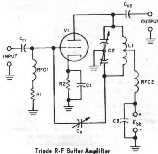
Capacitive input and output coupling are provided through  $C_{c1}$  and  $C_{c2}$ , respectively. Both fixed grid bias and pro-
