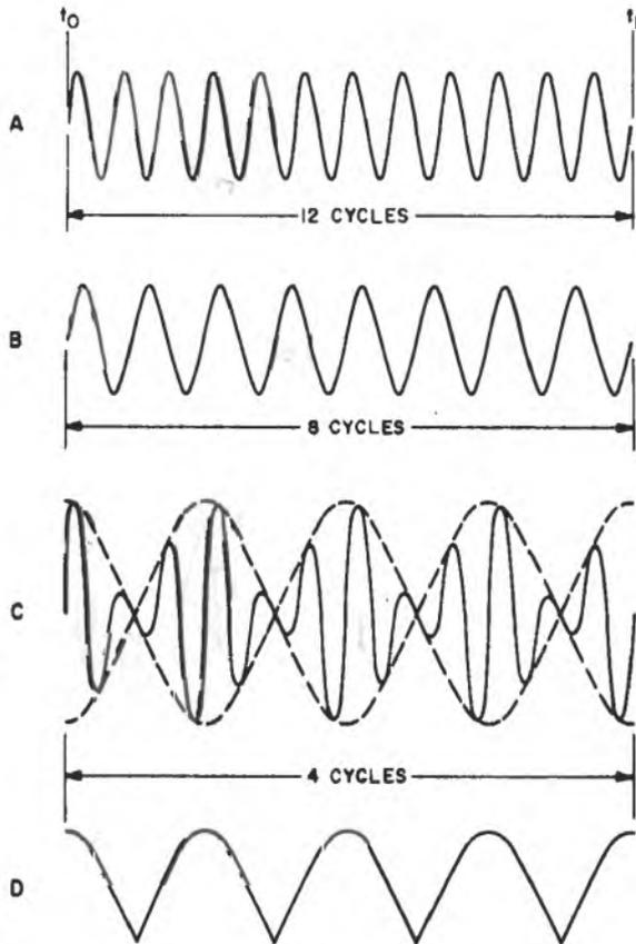
Heterodyning of Two Signals of Equal Amplitude With Resulting Distortion
