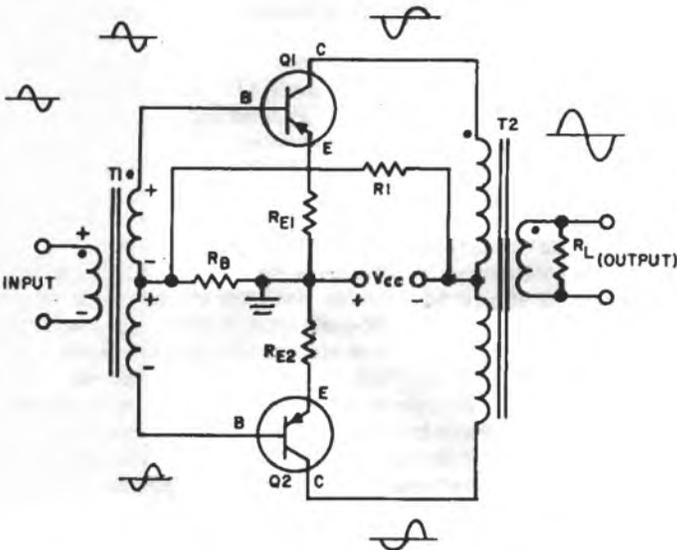
**Push-Pull Transformer-Coupled Transistor Power Amplifier**
