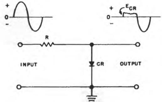
**Parallel-Diode Positive-Lobe Limiter**
