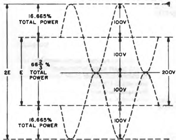
$$\text{PERCENT OF MODULATION} = \frac{E_{\text{MAX}} - E_{\text{MIN}}}{E_{\text{MAX}} + E_{\text{MIN}}} \times 100$$
