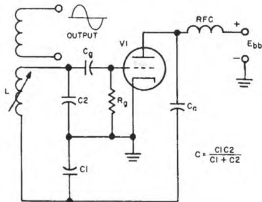
$$C = \frac{C_1 C_2}{C_1 + C_2}$$
