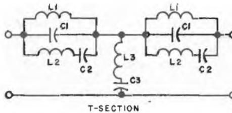
Shunt  $m$ -Derived Band-Elimination Filter
