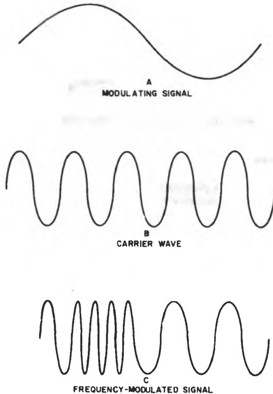
**Frequency Modulation Waveforms**
