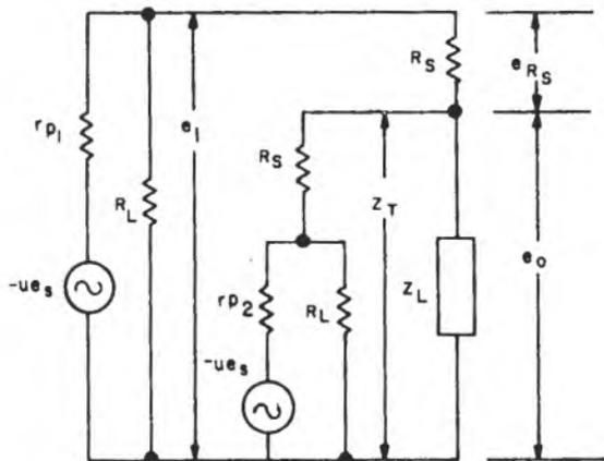
$$Z_T = \frac{\left( \frac{r_p R_L}{r_p + R_L} + R_s \right) Z_L}{\left( \frac{r_p R_L}{r_p + R_L} + R_s \right) + Z_L}$$
