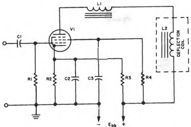
**Current (Electromagnetic) Deflection Amplifier Utilizing Square-Wave Input**
