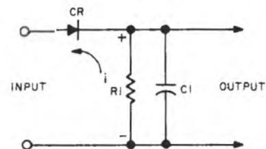
Voltage-Output Diode Detector
