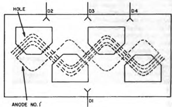
**Phasitron Anode Structure
