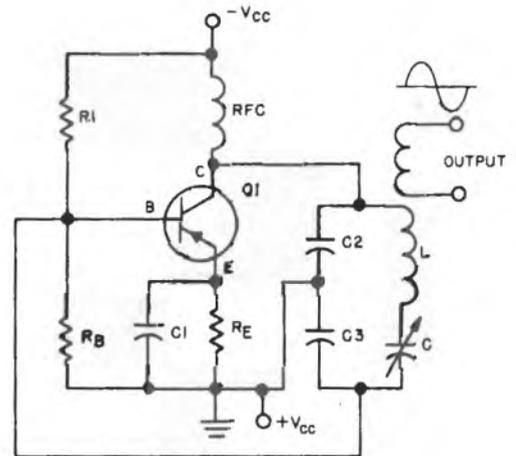
Shunt-Fed Clapp CE Oscillator
