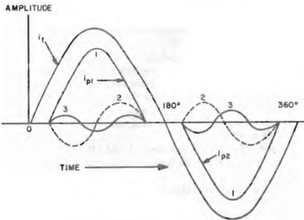
Tank Current versus Fundamental and Harmonic Plate Currents
