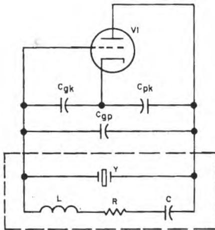
Ultraclon Equivalent Circuit
