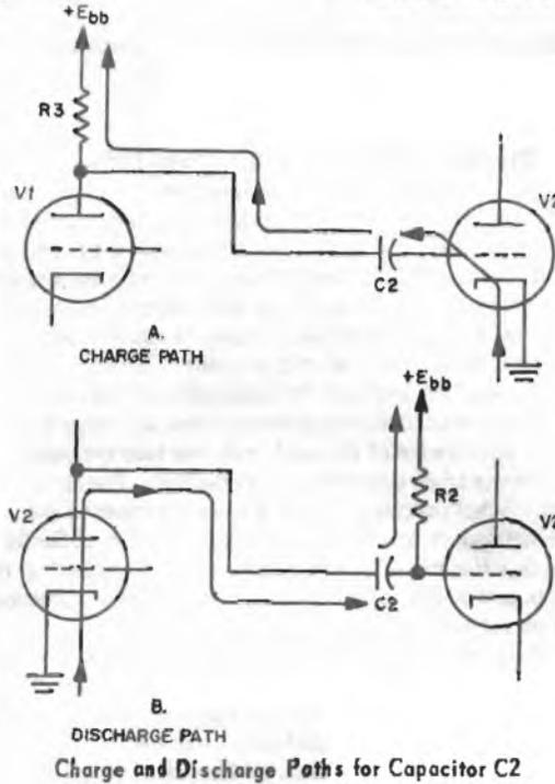
Charge and Discharge Paths for Capacitor C2
