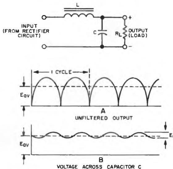
L-C Choke-Input Filter and Waveforms
