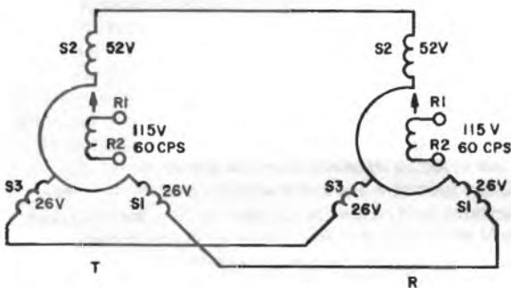
Synchro Transmitter-Receiver Circuit
