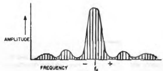
Typical Magnetron Spectrum
