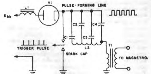
**Fixed Spark Gap Modulator Circuit**
