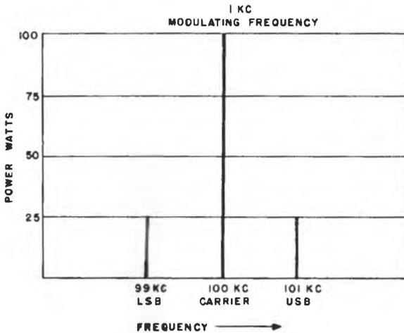
100% Modulated A-M Signal (100 Watt Carrier Power)
