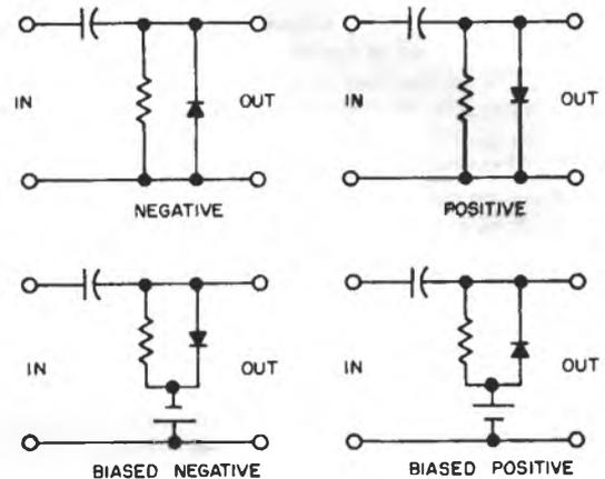
Types of Diode Clamping Circuits
