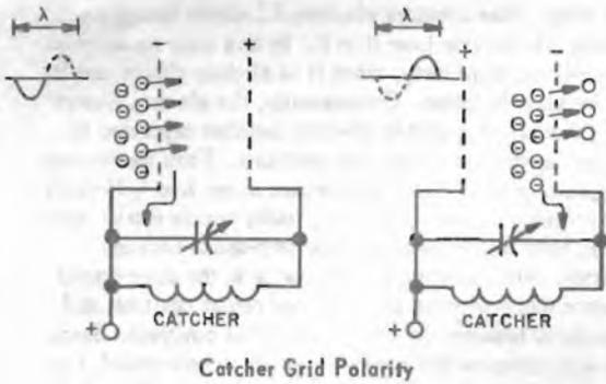
Since the second grid is also negative, it further slows down the electrons and again absorbs energy from them. Thus, in delivering energy to the tuned cavity connected to the catcher grids, the speed of the electrons is greatly reduced. After passing this second set of catcher grids the spent electrons are collected and removed from the tube by the positive collector plate.
