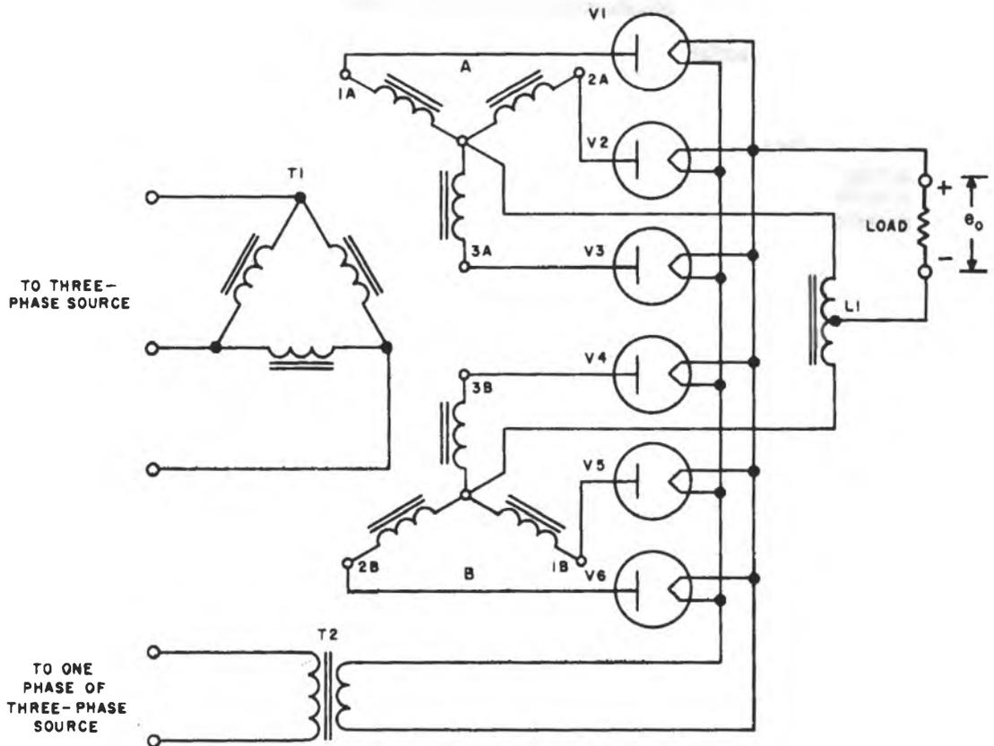
**Basic Three-Phase, Half-Wave (Double "Y" Secondary) Rectifier Circuit**
