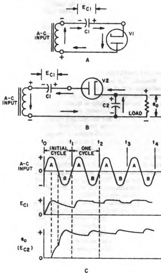
Typical Half-Wave Voltage-Doubler Circuit
