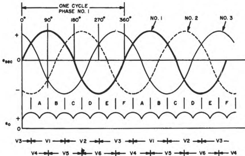
Simplified Circuit Schematics and Waveforms for
