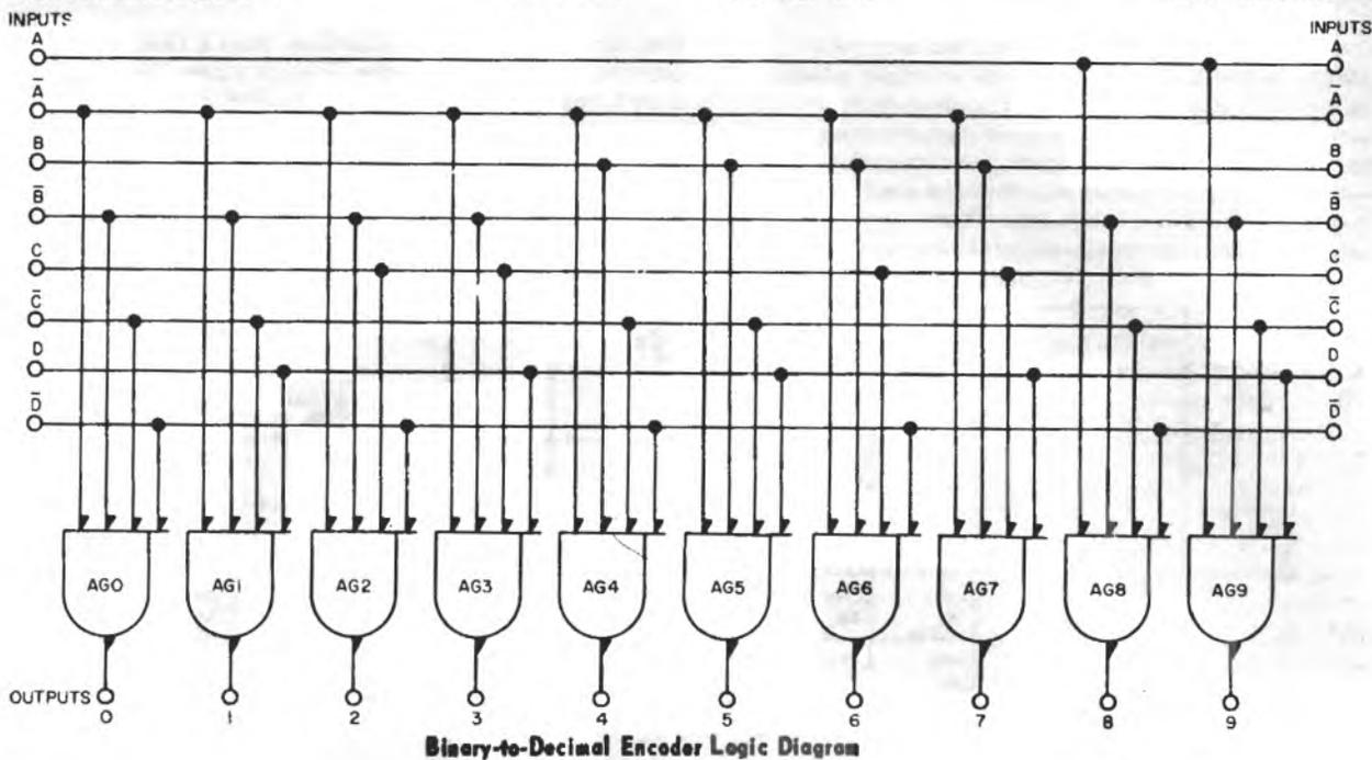
Examination of the logic diagram shows that 10-AND gates having 4-inputs and four diodes in each gate (AG0 through AG9) are used. The closed triangles indicate that positive logic is employed. Therefore, the inactive state (a logic 0) is represented by a relatively low voltage level (L), while the active state (a logic 1) is represented by a relatively high level (H).
