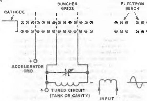
Electron Gun and Buncher Grids
