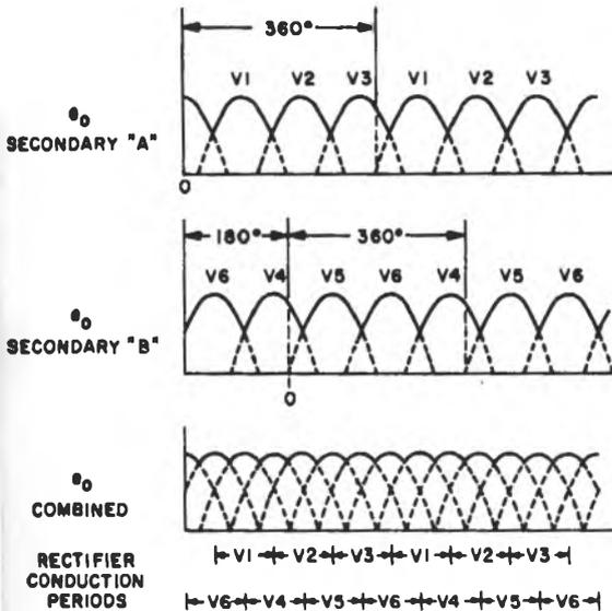
Waveforms for Three-Phase, Half-Wave
