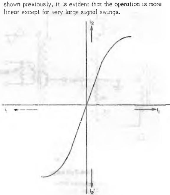
Composite Current Transfer Characteristic, Class AB Operation
