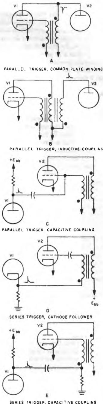
**Blocking-Oscillator Triggering Methods**
