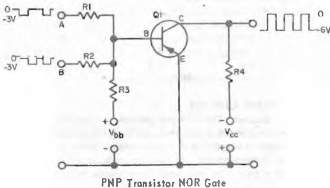
A positive (reverse) fixed bias is applied to the base to keep the transistor cut off in the inactive state. With no input applied, and reverse bias applied to the base and to the collector no conduction occurs, therefore, the collector and output voltage is approximately the same as the collector supply value. Since a negative "1" or high signal is re-
