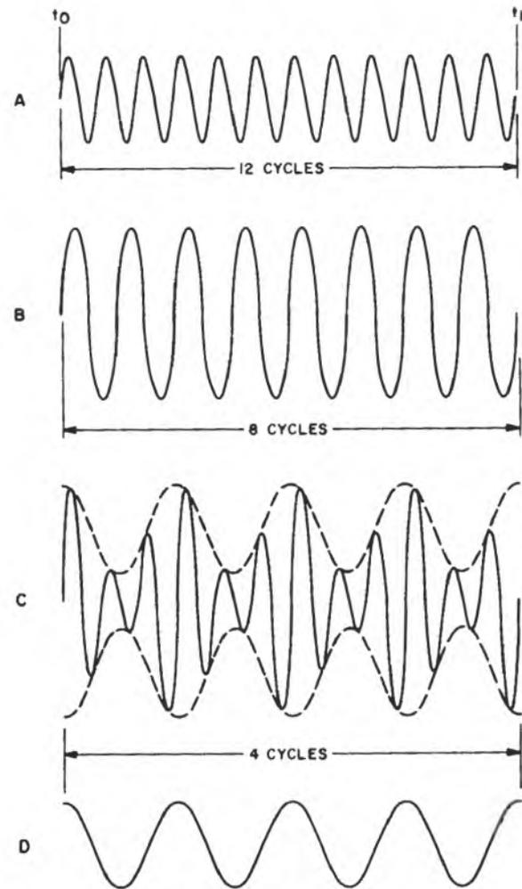
Heterodyning of Two Signals of Unequal Amplitude
