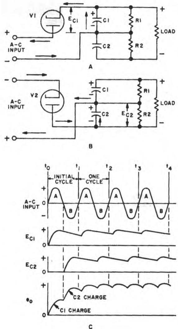
Typical Full-Wave Voltage-Doubler Circuit Operation and Waveforms
