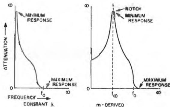
**Comparison of Filter Attenuation Characteristics**
