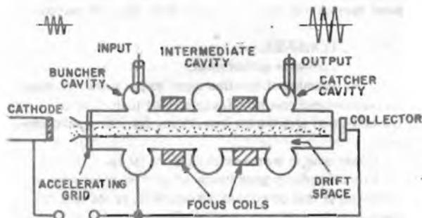
Simplified Klystron Multicavity Amplifier
