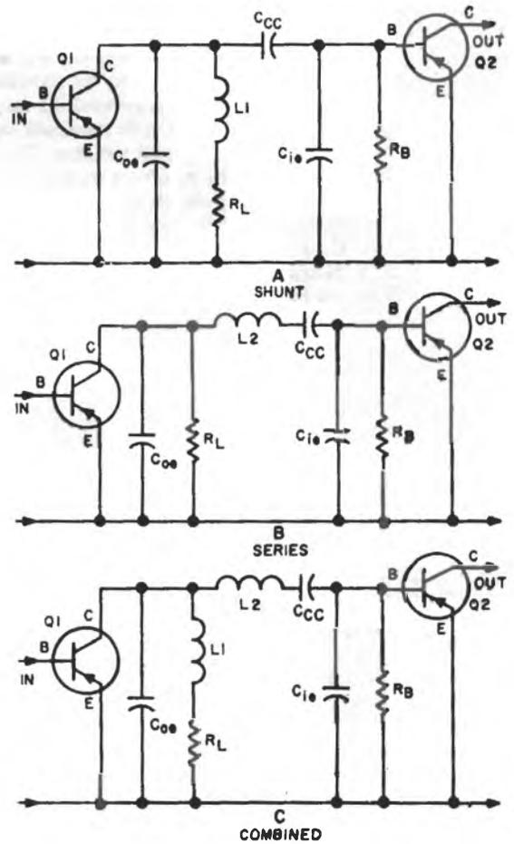
Figure 3-65. Shunt, Series, and Combined Peaking Circuits
