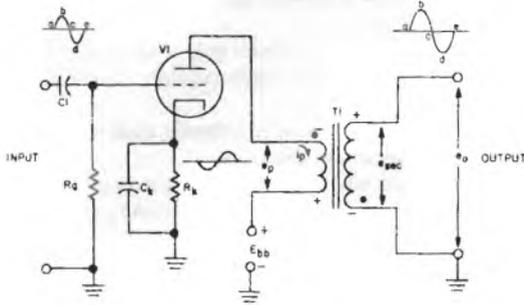
Typical Transformer-Coupled Audio Voltage Amplifier
