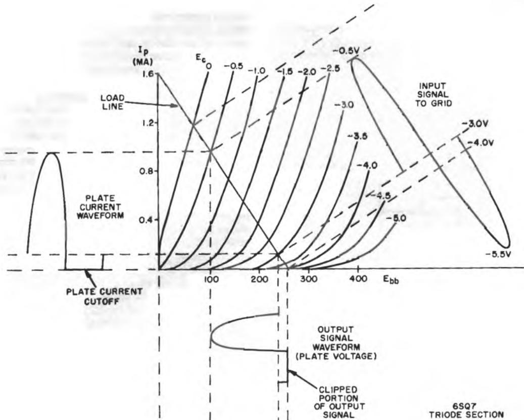
Operating Characteristics of a Typical Cutoff Limiter
