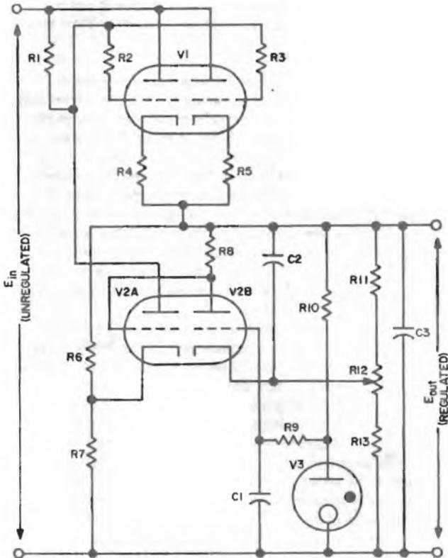
D-C Regulator Using Cascade Twin-Triode Amplifier
