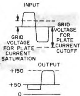
Typical Triode Saturation Limiter and Input-Output Waveforms
