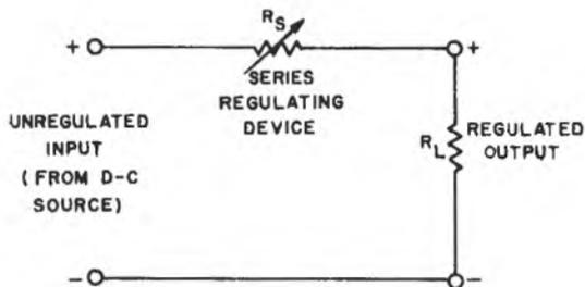
**Simple Series-Type Voltage-Regulator Circuit**
