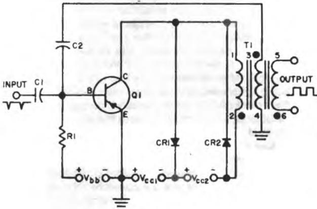
**Nonsaturating, Diode-Clamped Blocking Oscillator**
