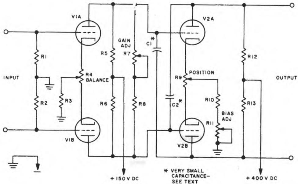
**Typical Two-Stage Push-Pull Direct-Coupled (D-C) Amplifier**
