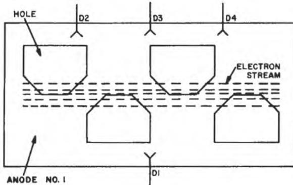
**Phasitron Anode Structure
