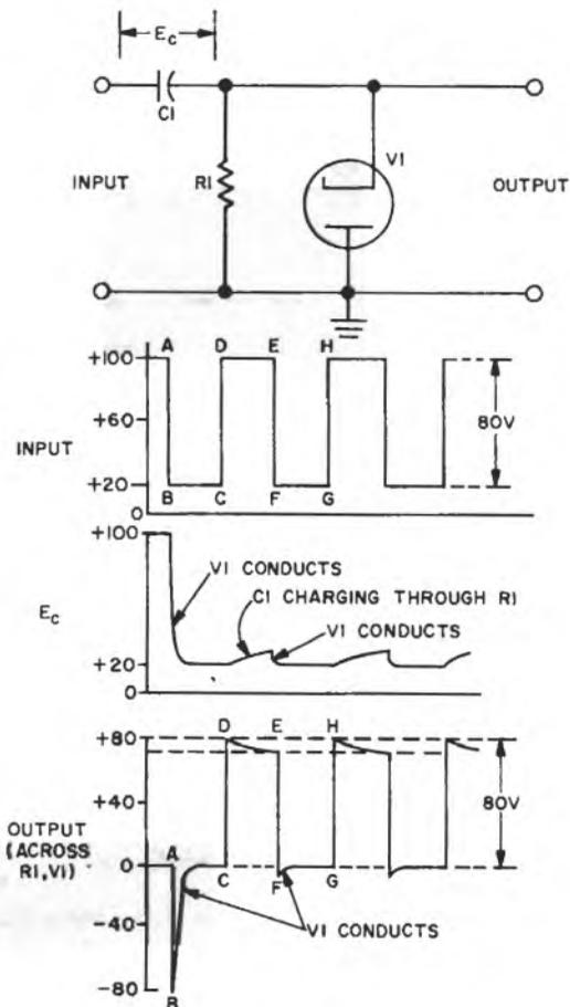
**Positive Diode Clamper Circuit and Waveforms**
