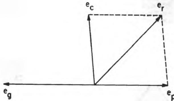
Vector Diagram Showing Effect of Modulation
