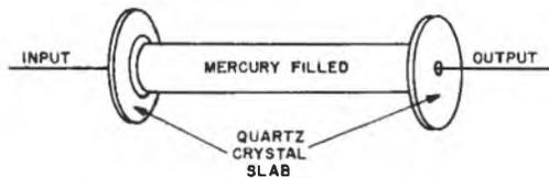
**Electromechanical (Acoustic) Delay Line**
