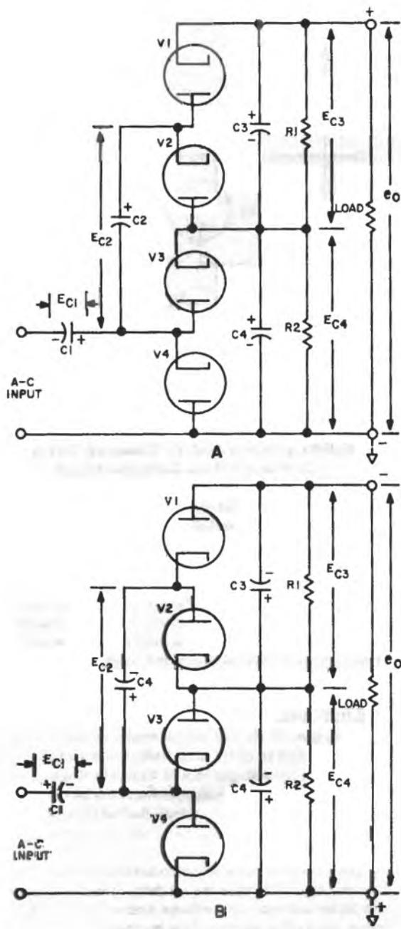
Basic Cascade Voltage-Quadrupler Circuits
