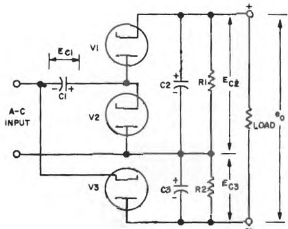
Basic Voltage-Tripler Circuit
