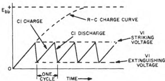
Output Voltage Waveform
