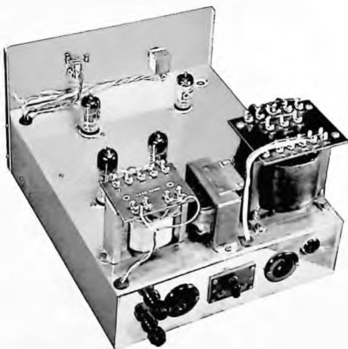
Fig. 33. Rear view of chassis fitted with Whiteley transformers.
