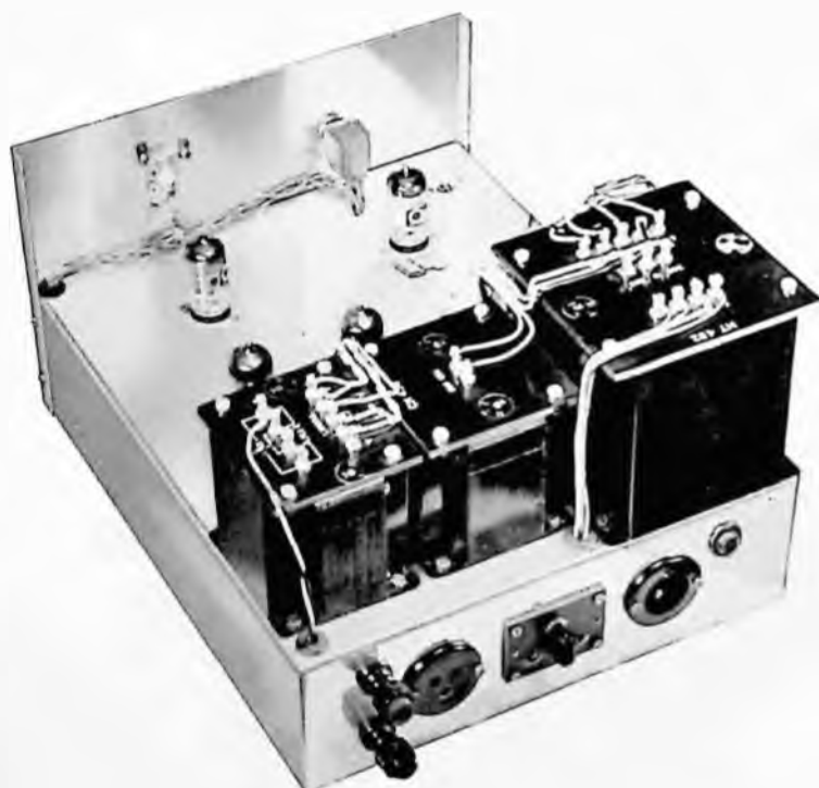
Fig. 31. Rear view of chassis fitted with Haddon transformers.
