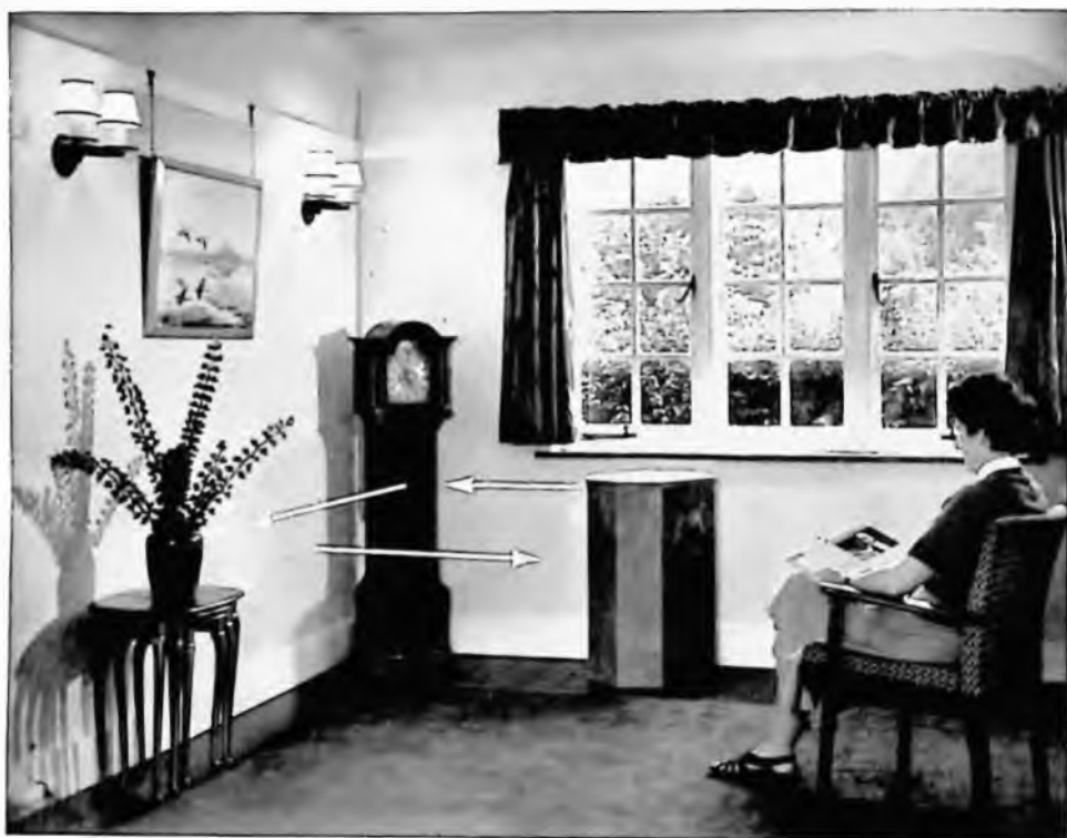
Fig. 5. The arrows show how the sound is reflected from wall to wall in order to widen the apparent source. Note that obstructions such as the clock have practically no effect ; it is not necessary for the corner to be absolutely bare.
