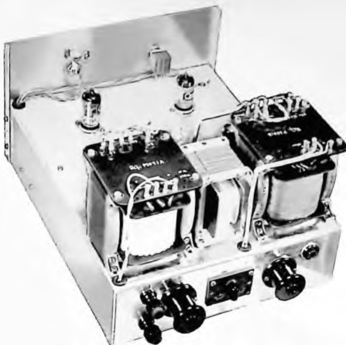
Fig. 32. Rear view of chassis fitted with Partridge transformers.
