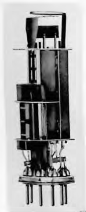
Fig. 4. The electrode system of the ECL86 triode-power pentode clearly showing the different lengths of the triode and the pentode sections. Note also the screening on the top of the triode section.
