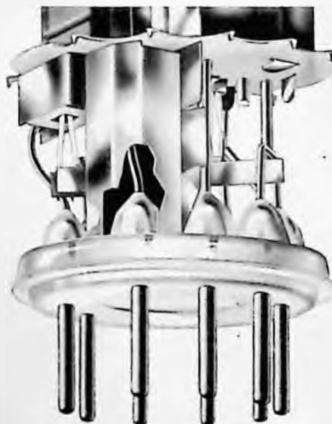
Fig. 5. Screening of the grid lead of the triode section.
