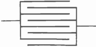
FIG. 1/II:22.—Construction of Condenser Plates.
