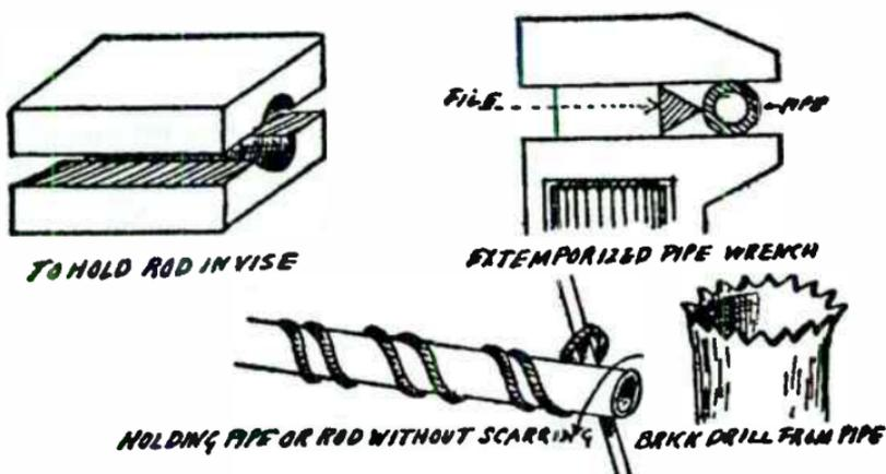
If you wish to hold a tube or rod in a vise, do not clamp it in the vise jaws. It will be impossible to hold it securely without scarring or flattening it, but by boring a hole a trifle smaller than the diameter of the pipe or rod through a wooden block and then sawing the block in two, you may clamp the pipe between the two sections of wood in the vise and hold it immovably without danger of injuring it.
