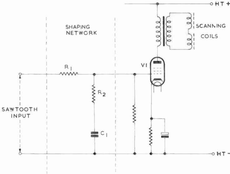
Fig. 133—Circuit in which linearity of field-scan is obtained by use of a shaping network at the input to the output valve
