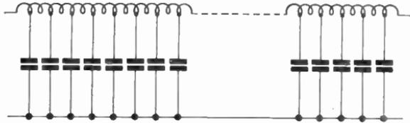
Fig. 76—The inductance and capacitance of a delay cable is distributed throughout its length
