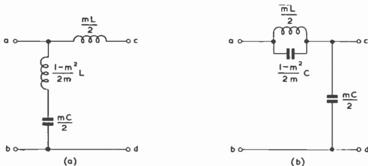
Fig. 86—Two basic forms of  $m$ -derived half-section
