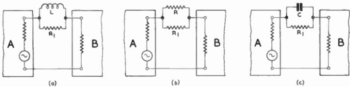
Fig. 114—In a variable equaliser the series element may be an inductor (a), a resistor (b) or a capacitor (c)
