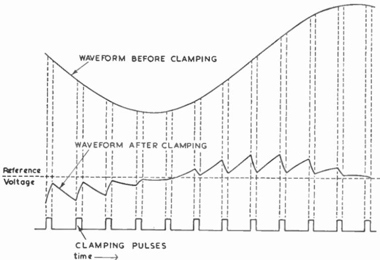
Fig. 54—Illustrating the action of a d.c. clamp
