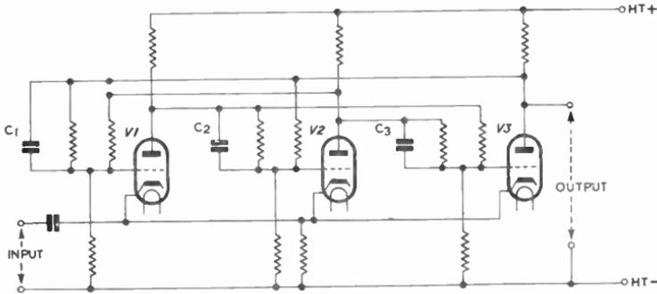
Fig. 7—Ring circuit for dividing by three
