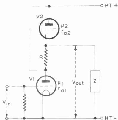
Fig. 155—Shunt-regulated amplifier with h.t. supply included
