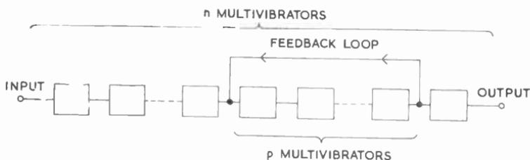
Fig. 16—General form of counter circuit with feedback
