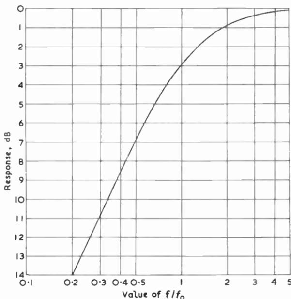
Fig. 101—Generalised frequency response for simple constant-resistance equaliser
