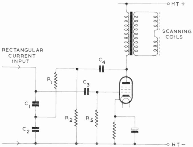
Fig. 137—Blumlein field output circuit
