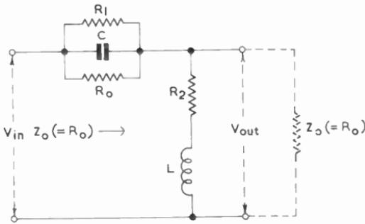
Fig. 102—Improved form of constant resistance L-section equaliser
