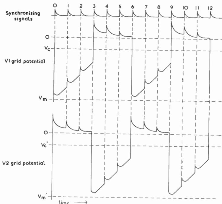
Fig. 32—Grid-potential waveforms for a symmetrical multivibrator with synchronising signals applied to both grids
