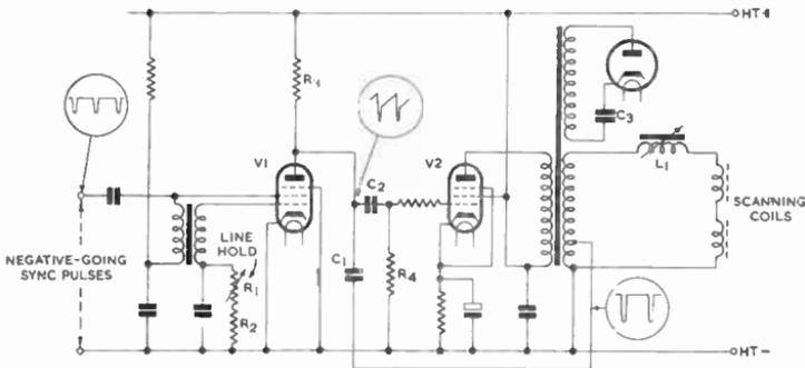
Fig. 146—Complete line oscillator and output stage incorporating an efficiency diode
