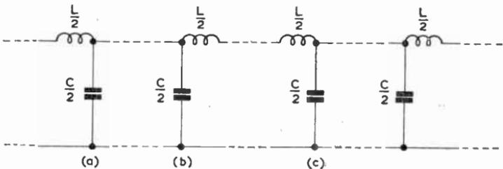
Fig. 77—Ladder network of inductance and capacitance with properties similar to those of a delay cable
