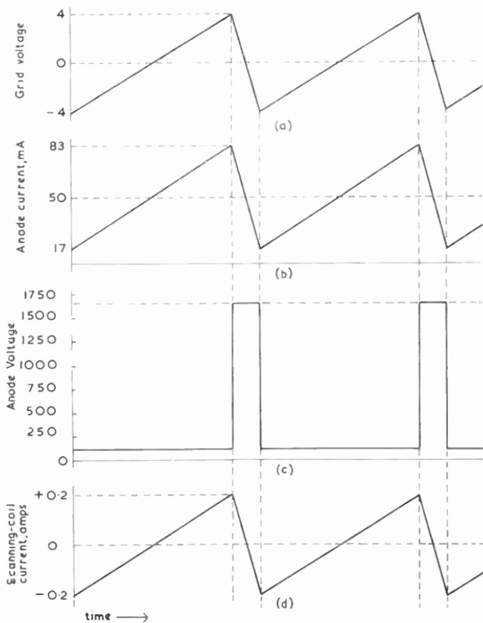
Fig. 139—Waveforms for ideal line output stage
