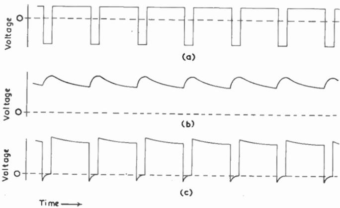
Fig. 46—A d.c. restorer with a finite discharge time constant, fed with waveform (a), adds a signal of form (b) to give an output of form (c)
