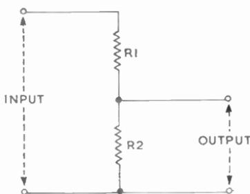
Fig. 63—A simple potential divider
