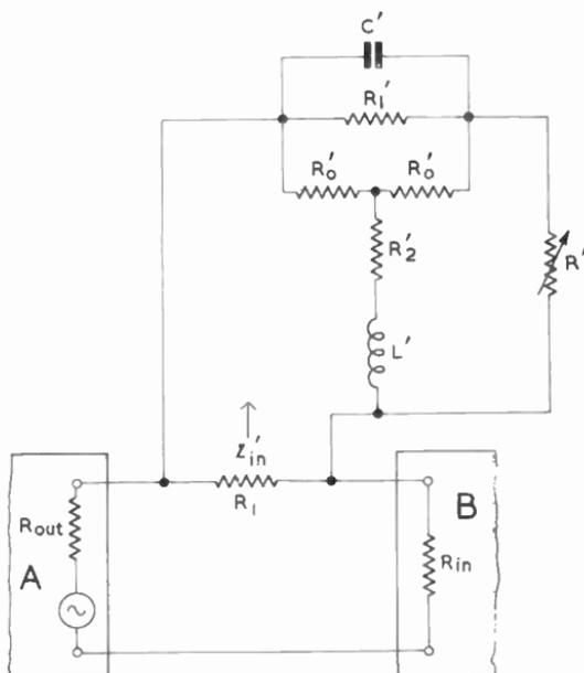
Fig. 116—Fundamental circuit of a Bode-type variable equaliser
