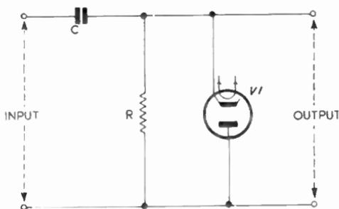
Fig. 44—Circuit of simplest type of d.c. restorer
