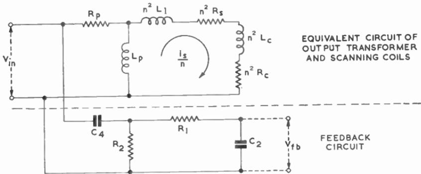
Fig. J.1—Blumlein circuit with output transformer replaced by equivalent network
