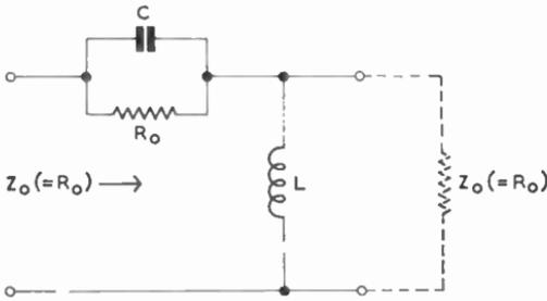
Fig. C.1—Simple constant-resistance equaliser
