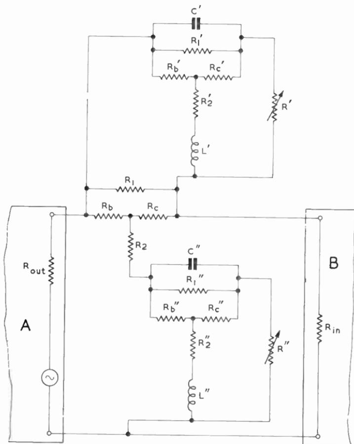
Fig. 120—Complete circuit of constant-resistance Bode-type variable equaliser
