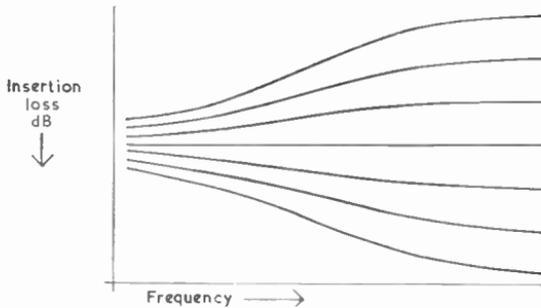
Fig. 112—Frequency responses obtainable from a variable equaliser
