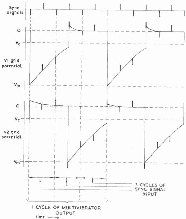
Fig. 34—Waveforms for a multivibrator in which sync signals are applied to the two grids in push-pull
