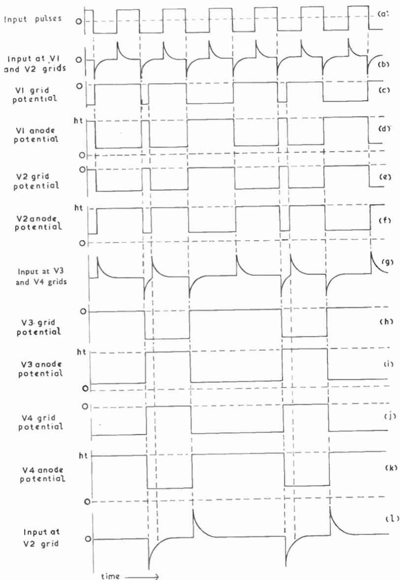
Fig. 15—Waveforms for the binary counter of Fig. 14
