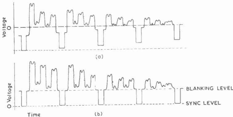
Fig. 42—A video signal with varying sync level is shown at (a) and the waveform after d.c. restoration at (b)
