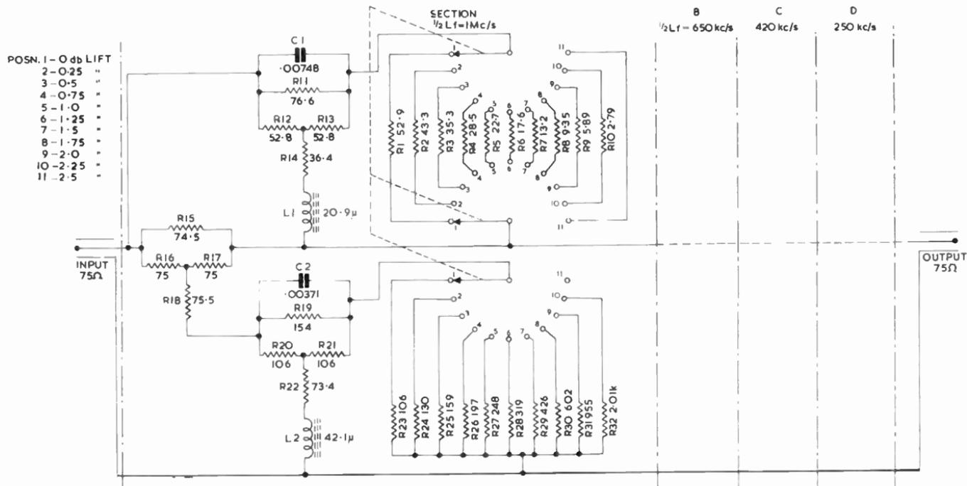
Fig. 121—Illustrating the component values in one section of a constant-resistance Bode-type variable equaliser
