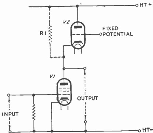
Fig. 67—Simplified circuit diagram of a gamma corrector employing the non-linearity of a triode  $I_a-V_g$  characteristic
