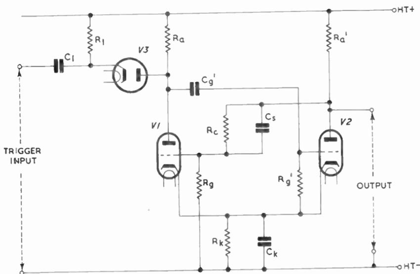
Fig. 22—A monostable multivibrator used as frequency divider
