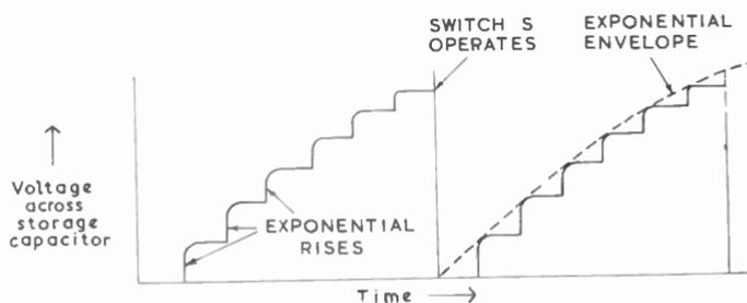
Fig. 2—Waveform across storage capacitor in step counter
