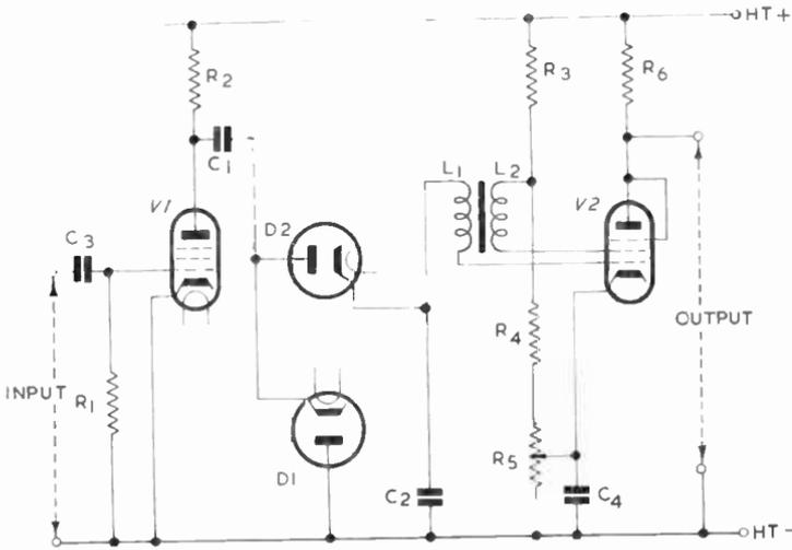
Fig. 6—A step divider using a blocking-oscillator switch
