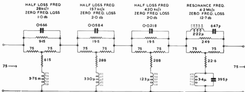
Fig. 110—Typical complete video constant-resistance equaliser
