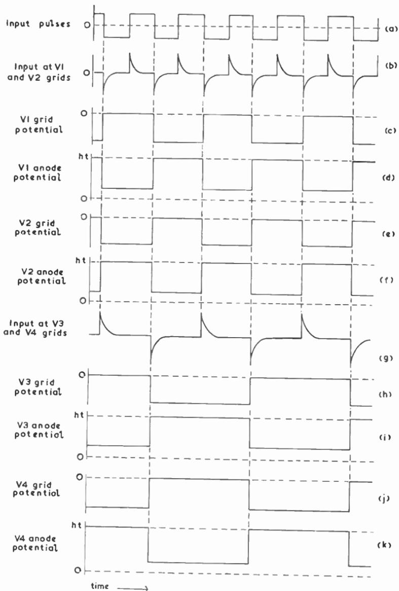
Fig. 13—Waveforms for the binary counter of Fig. 12
