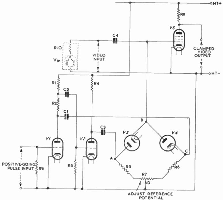
Fig. 55—An alternative circuit for a d.c. clamp
