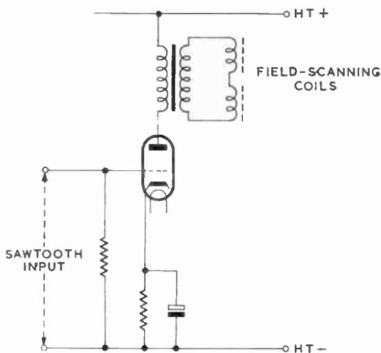
Fig. 126—Basic circuit for transformer-coupled field scanning output stage
