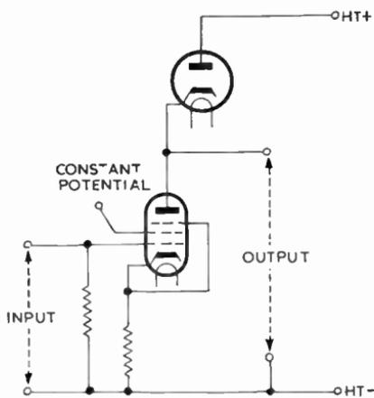
Fig. 66—Simple gamma corrector using a pentode as constant-current source
