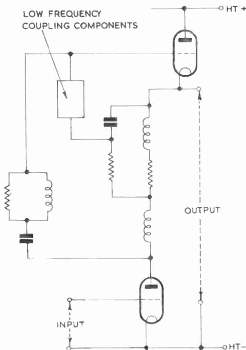
Fig. 158—A complex network used to compensate a shunt-regulated amplifier with two similar valves, feeding a capacitor  $C$ , it is shown in Appendix L that if
