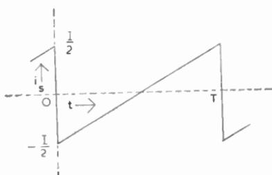
Fig. 129—Ideal sawtooth waveform required in scanning coils
