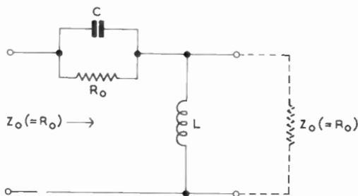
Fig. 100—Simple constant-resistance equaliser circuit
