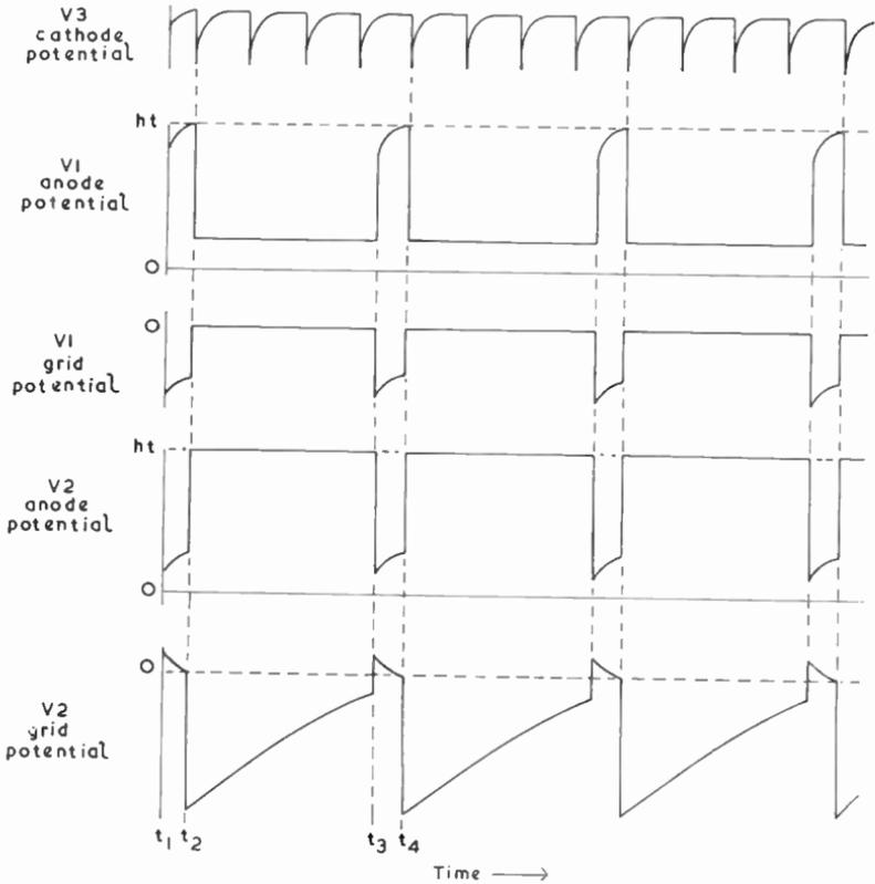
Fig. 23—Waveforms for the frequency divider of Fig. 22
