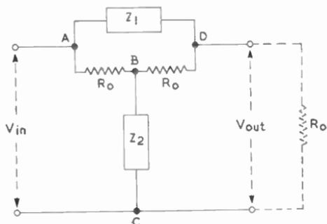
Fig. 99—Bridged-T network obtained by connecting a resistor  $R_0$  between terminals B and D in Fig. 96
