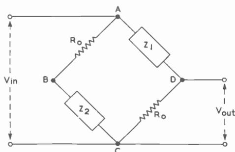
Fig. 96—Input and output connection used when the bridge circuit is employed as an equaliser
