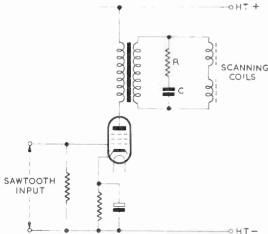
Fig. 143—Improved circuit of simple line output stage
