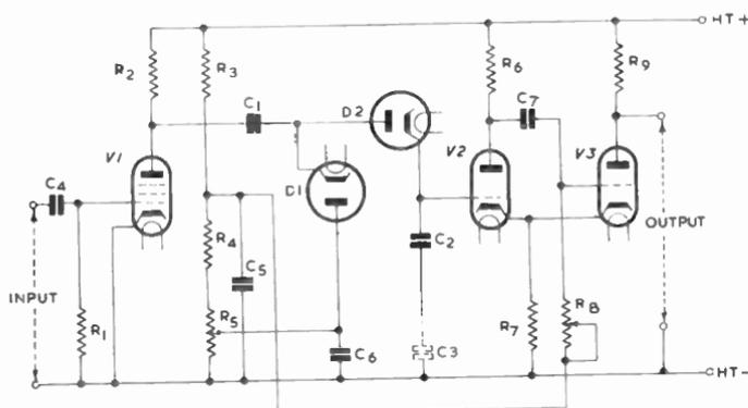
Fig. 4—Step divider using a multivibrator switch
