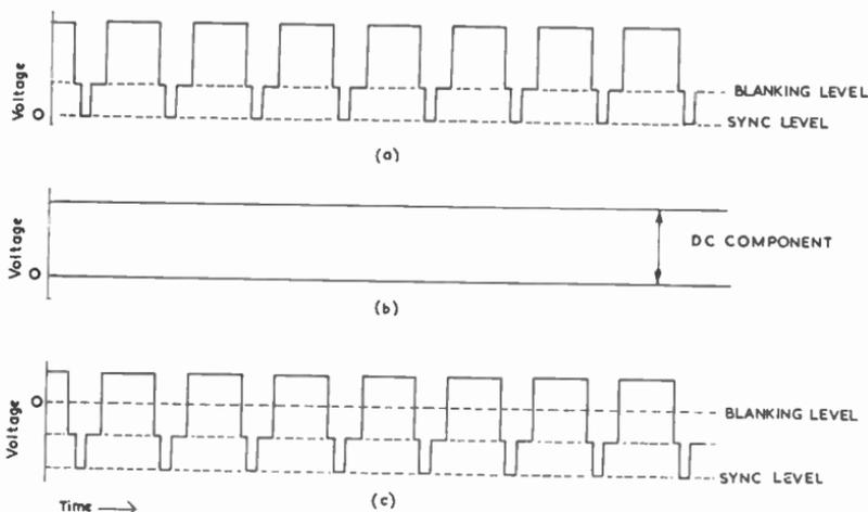
Fig. 39—A video signal for a white scene is shown at (a); its d.c. and a.c. components are shown at (b) and (c)
