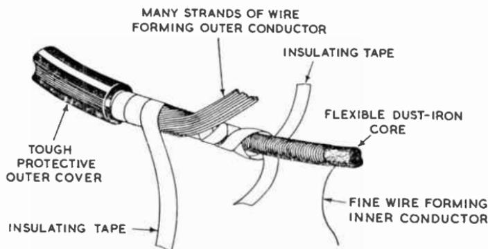
Fig. 75—Construction of a delay cable
