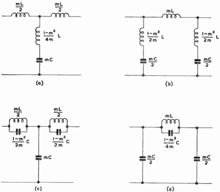
Fig. 84—Four basic types of  $m$ -derived section
