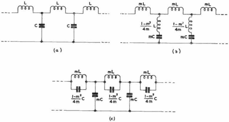
Fig. 83—Part of a recurrent network is shown at (a), one  $m$ -derived equivalent at (b) and a second  $m$ -derived equivalent at (c)
