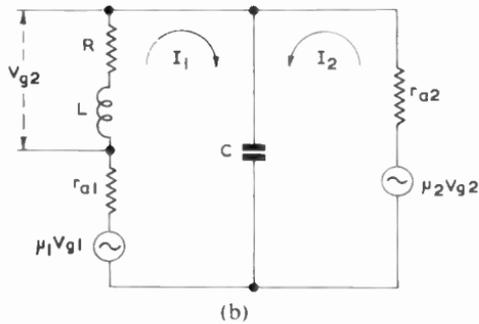
Fig. L.1—An inductance-compensated shunt-regulated amplifier is shown in simplified form at (a) and its equivalent circuit at (b)
