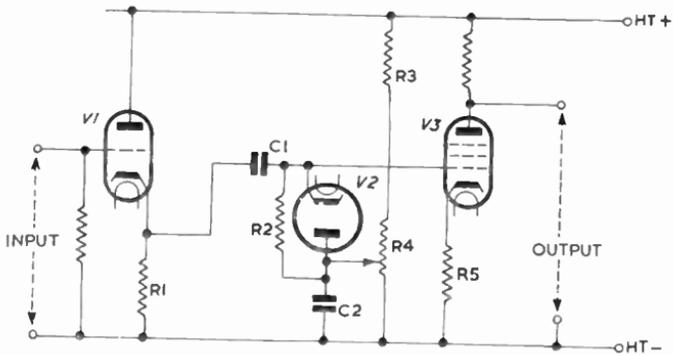
Fig. 49—Circuit diagram of a d.c. restorer with provision for adjusting sync level of output
