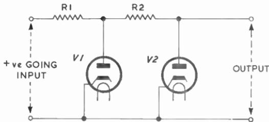
Fig. 65—Circuit of a gamma corrector using two diodes
