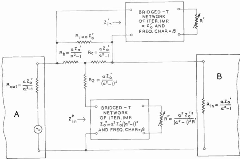
Fig. 119—Final form of constant-resistance Bode-type variable equaliser
