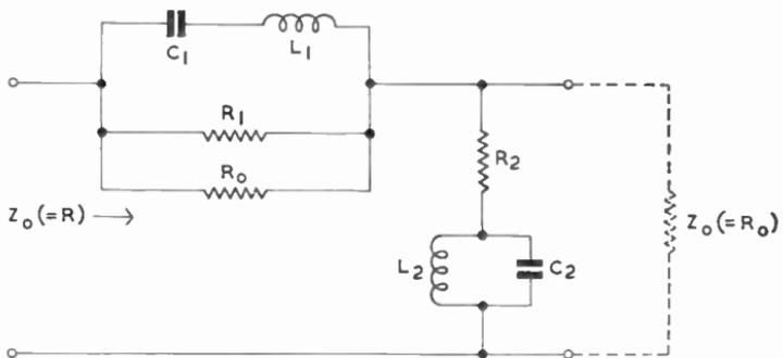
Fig. E.1—Resonant constant-resistance equaliser
