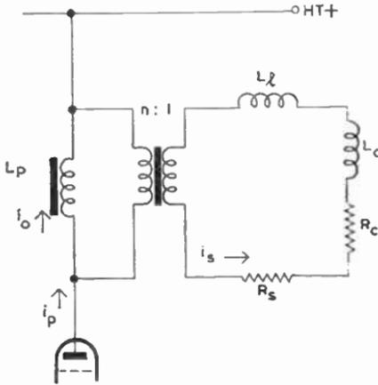
Fig. 127—Equivalent circuit of field output stage
