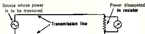
FIG. 8.21. A transmission line power meter.
