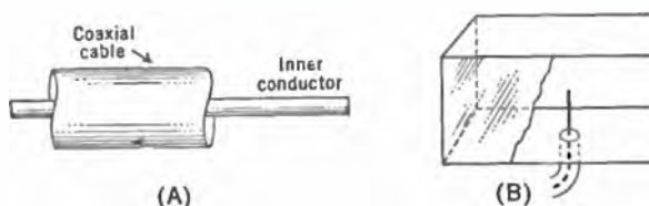
FIG. 6.14. (A) Extended inner conductor acts as capacitive coupler to electric field in cavity resonators and wave guides. (B) Actual position in resonator.
