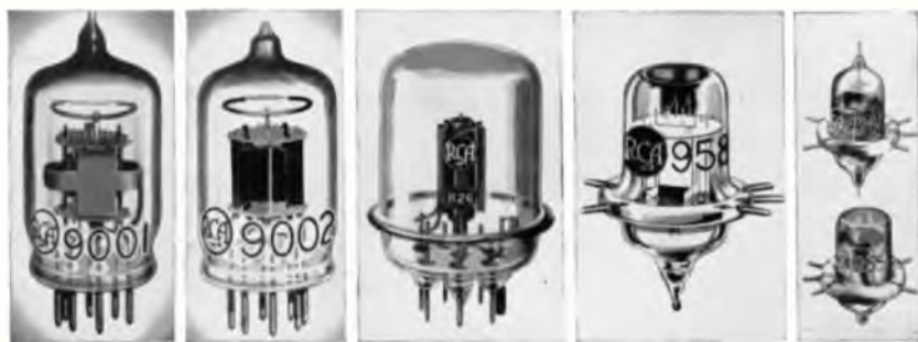
Fig. 1.2. Number of different tubes that have been designed for ultra-high frequency applications.
