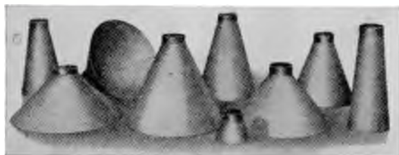
FIG. 7.20. Various electromagnetic horns that were used in tests.
