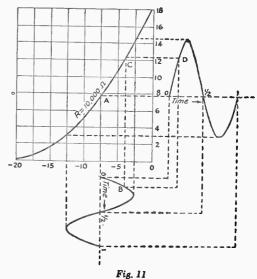
veloped across the load resistor. This a.c. voltage is the useful output of the tube. The maximum drop in the resistor occurs when the plate current is maximum, corresponding to the most positive value of instantaneous grid voltage, and the mini-
