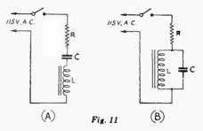
**Procedure:** Connect the choke coil,  $0.1-\mu$ fd. condenser and the 1000-ohm resistor in series as shown in Fig. 11-A. Read the voltages across the resistance, capacity, inductance, and across the condenser and inductance in series. Substitute the 2000, 5000 and 10,000-ohm resistances one
