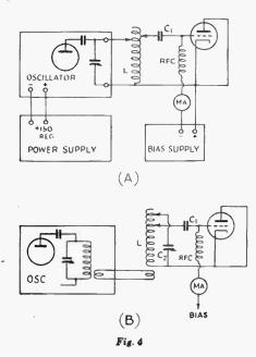
may be used without affecting the results of the experiment. *RFC* is a 2.5-millihenry choke coil and  $C_2$  is one of the tuning condensers (250  $\mu\mu$ fd.) on the circuit board. The tube used in the experiment should be a 6J5 or 6C5.
