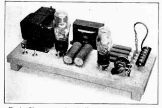
Fig. 4 — The power supply unit. Mounting of parts closely follows the circuit diagram of Fig. 3. The baseboard is  $6 \times 14$  inches. Voltage divider taps are machine screws projecting through the baseboard just to the left of the terminal strip. The variable section of the divider is mounted on a metal bracket at the right front.
