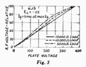
11). If the modulation characteristic is not linear, the envelope of the modulated wave will not be a true reproduction of the audio-frequency voltage applied to the plate circuit of the modulated amplifier, hence distortion will be introduced in
