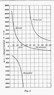
increase in capacity, with the difference in the reactance at the old and new settings equalling 100 ohms. Thus with series tuning the condenser capacity must be increased when the line is capacitive and decreased when the line is inductive, the opposite of the case when parallel tuning is used.
