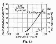
bias of 64 volts and the plate current and output are cut off at 82 volts. The peak modulating voltage required for 100 per cent modulation therefore is 82 - 64 = 18 volts. The modulation peak will occur at 64 - 18 = 46 volts, which is
