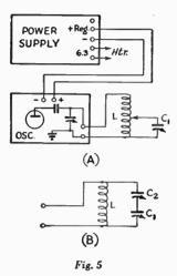
Oscillator plate voltage may be taken from the regulated tap, using a VR-105-30 regulator tube. However, voltage regulation is not essential, so that the plate voltage can be taken from one of the divider taps on the power supply, keeping the voltage at about 100 volts or less.
