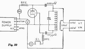
tively high, but decreases with increasing gridleak resistance. The grid bias — product of grid current by grid-leak resistance — shows comparatively little variation, indicating the selfregulating properties of the oscillator in this respect; that is, the grid current regulates itself so as to develop about the same bias over a wide range of grid resistance.
