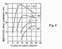
of negative grid bias, 25, 50, 75 and 100 volts. In all four cases the oscillator plate was tapped on the coil at the 25th turn. At the highest bias, 100 volts, the grid current is just reaching maximum with 30 turns in the grid circuit; that is, a step-up
