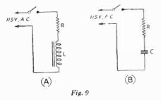
**Procedure:** Connect the 1000-ohm resistor in series with the inductance as shown in Fig. 9-A. Measure the voltage across the resistor and that across the inductance. Repeat with the other resistors substituted. A typical tabulation of readings will be as follows:
