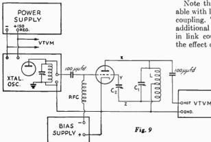
Q of the secondary circuit, the constants of the primary circuit being fixed. With a fixed value of load resistance, represented by the grid circuit of the tube, the Q of the circuit depends on the L/Cratio and/or the ratio of turns in the tuned circuit to turns in the load (grid-cathode) circuit. Using 35 turns in the tuned circuit, maximum output is
