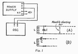
"vernier" or slow motion type if possible, to facilitate accurate setting. The coil L should be mounted close to the condenser so that the shortest possible leads can be used to connect the **two**.
