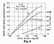
total voltage swing required from the modulator for 100 per cent modulation. Half of 45 volts, or 22.5 volts, is the peak value of the modulating voltage on one side of its axis, and since the minimum instantaneous grid bias must not be
