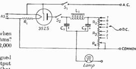
Fig. 2 - Circuit diagram of the transformerless power supply.
