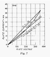
tortion in such a system because of the variation, with plate voltage, of the load resistance represented by the Class-C amplifier plate circuit. The effect of such variation on the modulator operation was described in the preceding experiment.
