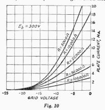
**zero** current there is no voltage drop in the load resistor. As in the case of the diode which was the subject of Exp. 21, increasing the value of load resistance has the effect of straightening out the curve, so that the curves taken with high values of load show less bending than curves with no load or small values of load resistance.
