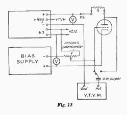
to the selected value (300 in this illustration) with plate current flowing (push-button closed). Shift the v.t.v.n. to the plate circuit and measure the a.c. output voltage, keeping the push-button closed. Repeat for various values of plate load resistance, using two resistors in series to make up values intermediate to those available in the single units. The results of a typical set of measurements are given below, for 2 volts r.m.s. applied to the grid:
