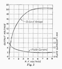
of a 25,000-ohm cathode resistor. The by-pass condenser in this case is  $0.01 \ \mu fd.$ , but somewhat smaller or larger values may be used. The measuring procedure is the same as with the grid-leak detector. In this case the plate current is quite
