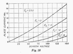
affected by the plate voltage so long as it is appreciably higher than the screen voltage. Vary the screen voltage in small enough steps so that smooth curves can be plotted from the data. Do this for several values of grid-bias voltage. Typical experimental curves obtained by this method are shown in Fig. 18, taken on a 6J7. These curves have essentially the same nature as the explanation of the operation of the screen-grid tube given above.
