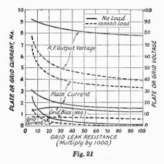
When the circuit is loaded the plate current shows a pronounced increase. This is partly because the load reduces the Q of the tuned circuit, thus lowering its parallel impedance and hence
