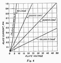
which will give current intervals of about 1 milliampere so that enough points will be secured to give a smooth curve when the points are plotted. In the case of the 6H6 tube, using one plate and cathode only, one-volt intervals are suitable. Proceed similarly when the load resistance is inserted in the circuit; in this case larger voltage intervals (5-volt steps, for instance) can be used.
