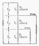
the voltage drops, indicated as E1, E2 and E3 on the diagram, across these three resistors. I1 is the current through R1, I2 is the current through  $R_2$ , and  $I_3$  is the current through  $R_3$ . The current through I1 is not known, but I2 is equal to the sum of I1 and the 5-ma. load current taken from the tap between R1 and R2, while R3 is the sum of I2 and the 8-ma. load current taken from the tap between R2 and R3. In equation form.
