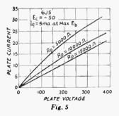
voltage is decreased one tap at a time on the power supply. When the run is complete, repeat the procedure with the grid current set to 3 ma., and then repeat once more with the grid current set at 1 ma. with the amplifier operating at the highest plate voltage. Plotting the plate voltageplate current data should give a set of curves resembling those of Fig. 6, taken on a 6J5 in such an experimental set-up. Increasing the amount of excitation, as measured by the d.c. grid current,
