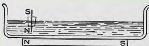
Fig. 8. Direct Proof that Magnetic Lines of Force are Curved.
