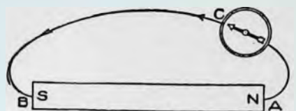
Fig. 7. Direction of Magnetic Lines of Force,
