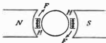
FIG. 1.—Moving-coil galvanometer.
