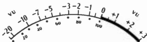
FIG. 14a.—"A" scale for VU meter.
