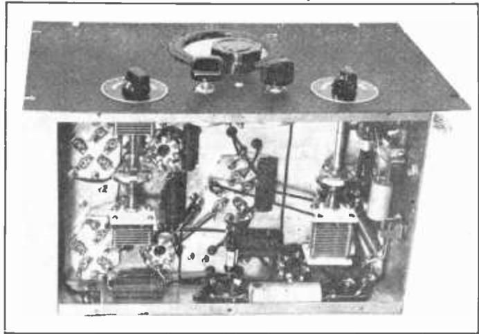
Figure 10. SHOWING FRONT PANEL AND UNDER-SIDE OF CHASSIS. Most of the "works" are under the chassis. The two ganged r.f. and mixer tuning condensers are visible in this photograph, as is the oscillator band-setting condenser.
