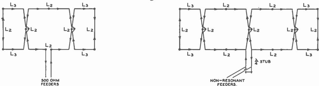
HORIZONTALLY POLARIZED BROADSIDE BARRAGE ANTENNAS
