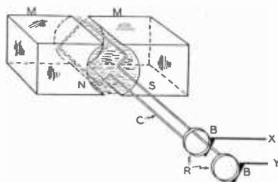
Figure 14. Schematic representation of the simplest form of the alternator.
