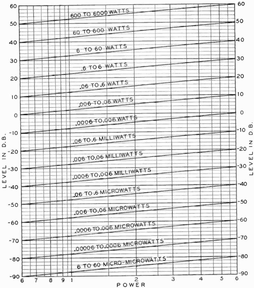
*Based on .006 watts at zero level.*
