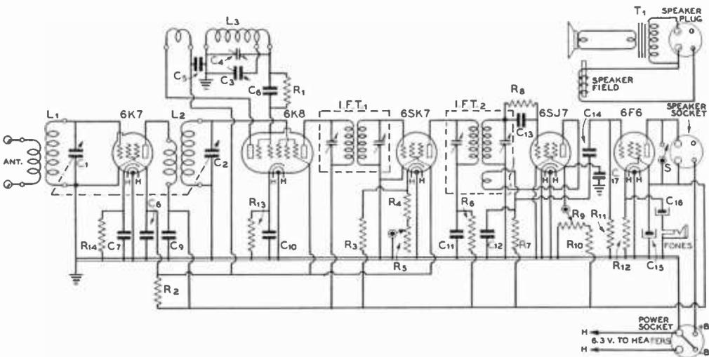
Figure 11. GENERAL WIRING DIAGRAM OF THE 5-TUBE SUPER.
