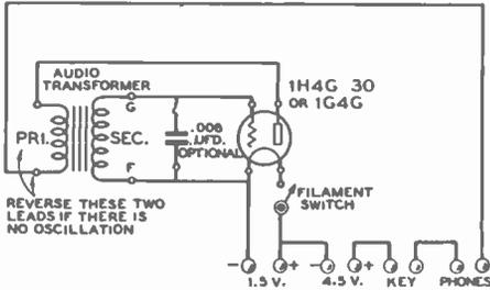
Figure 8. SIMPLEST TYPE V.T. CODE PRACTICE OSCILLATOR.
