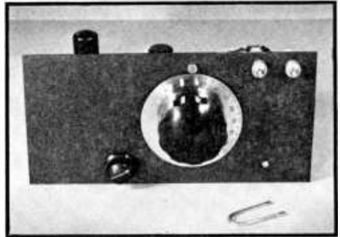
Figure 3. SIMPLE RECEIVER FOR USE BETWEEN 112 AND 350 MC.
