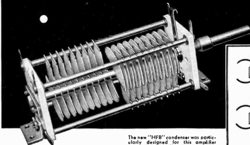
The new "HFB" condenser was particularly designed for this amplifier circuit. The "HFB" in this circuit permits the use of higher plate voltages for a given condenser plate spacing.
