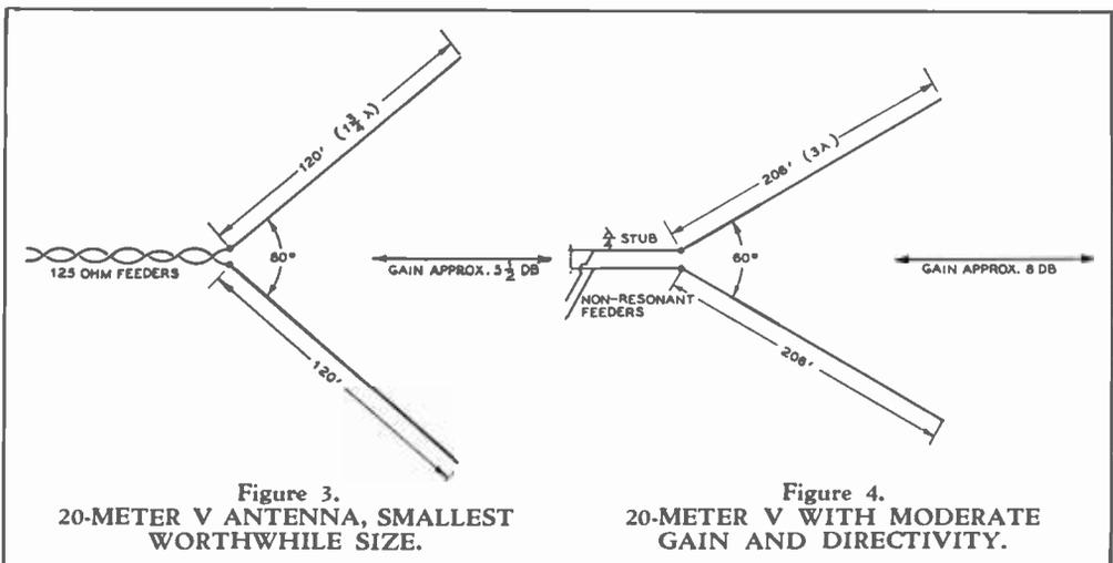
Figure 3. 20-METER V ANTENNA, SMALLEST WORTHWHILE SIZE.
