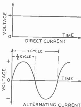
Figure 13. Graphical comparison of unidirectional or direct current and alternating current.
