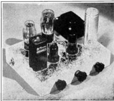
Figure 17. THE SELF-EXCITED 50-KC. SUBSTANDARD.
