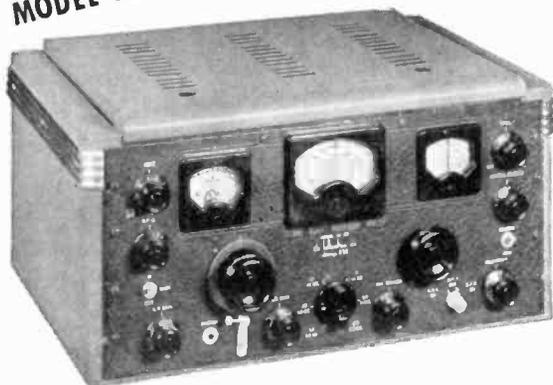
**H**ALLICRAFTERS Super Sky rider, Model SX-28A, covers the busiest part of the radio spectrum—standard broadcast band, international short wave broadcast bands, long distance radio telegraph frequencies, and all the other vital services operating between 550 kilocycles and 42 megacycles. Designed primarily as a top flight communications receiver the SX-28A incorporates every feature which long experience has shown to be desirable in equipment of this type.
