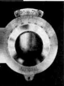
The four-inch N Dial has an engine divided scale and vernier. The vernier is flush with the scale. The planetary drive has a ratio of 5 to 1, and is contained within the body of the dial. 2, 3, 4 or 5 scale. Fits 1/4" shaft. Specify scale.
