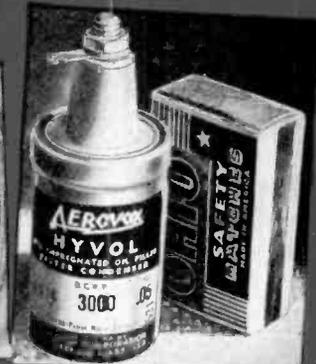
The war made Aerovox more space-conscious than ever. Type 14 miniature oil-filled transmitting capacitor is typical Single pillar terminal. Grounded case. Ring mounting. 3000 v. There's also Type 12 with two pillar terminals and ribbed cover. 2000 to 7500 v. D.C.W. Here's high-voltage insurance in minimum bulk and at popular prices.
