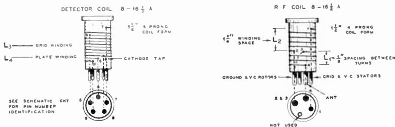
Figure 12—8 to 16 $\frac{1}{2}$ -Meter Coil Construction for Continuous Coverage T.R.F. Receiver.
