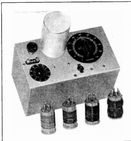
Figure 19—All-Wave Test Signal Generator in Aluminum Shield Can. The coil is also shielded with a large coil-shield can, as shown.
