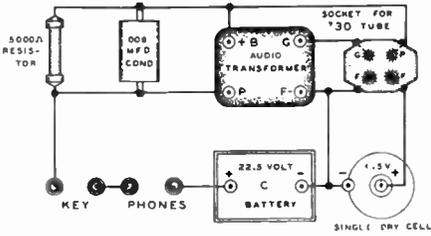
**Figure 4—Pictorial Wiring Diagram of Code Practice Oscillator Shown Schematically in Figure 3.**
