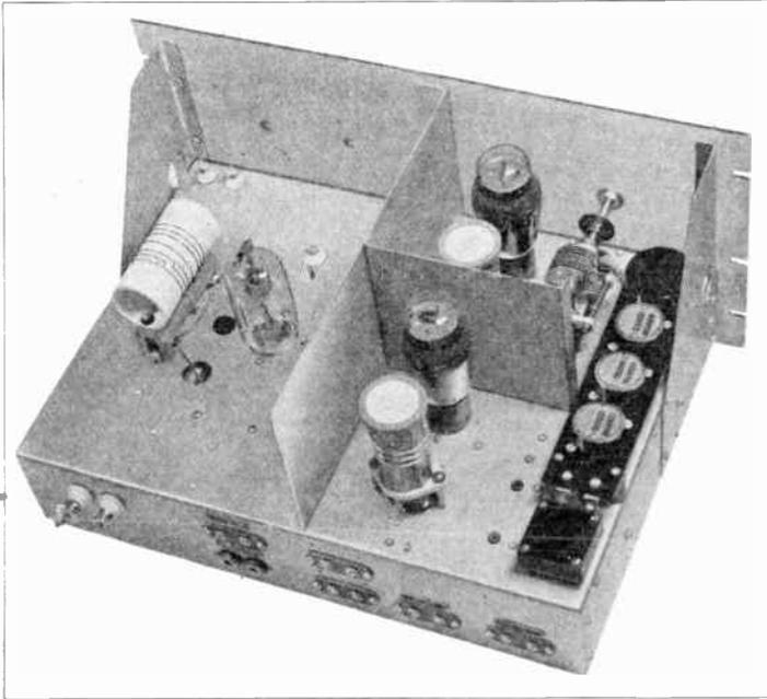
**Figure 19**—The exciter unit uses a 35-T, driven either directly by a 6L6-G harmonic oscillator or by a 6L6-G doubler. Most of the components are mounted on the under side of the sub-chassis (see figure 21). This unit can be used as a low power transmitter, plate modulated by the 2A3 driver stage to give about 35 watts of carrier until time or finances permit completion of the 250 watt amplifier and associated modulator.
