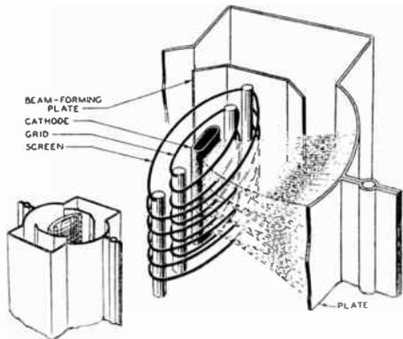
Figure 8—Internal Structure of Beam Power Tube
