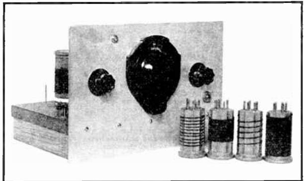
**Figure 6—Front View of Receiver. Coils for All-Band Operation are to the Right.**
