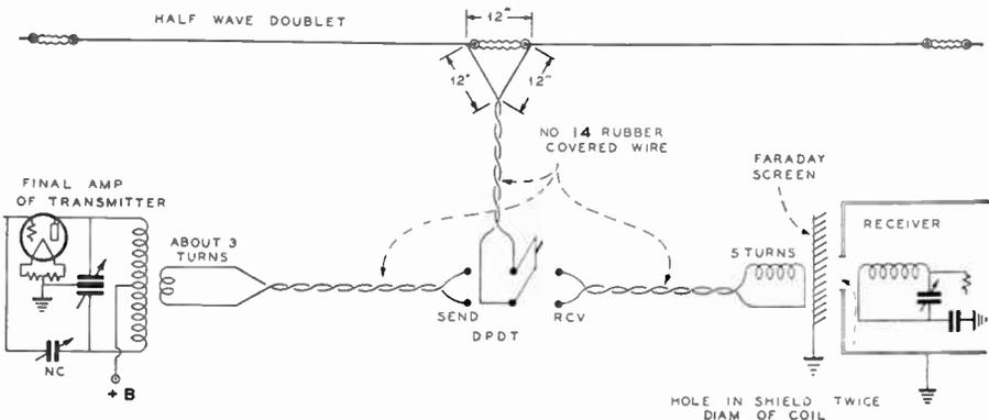
Figure 27—One-Band Doublet Antenna With Twisted-Pair Feeders for Transmitting and Receiving.
