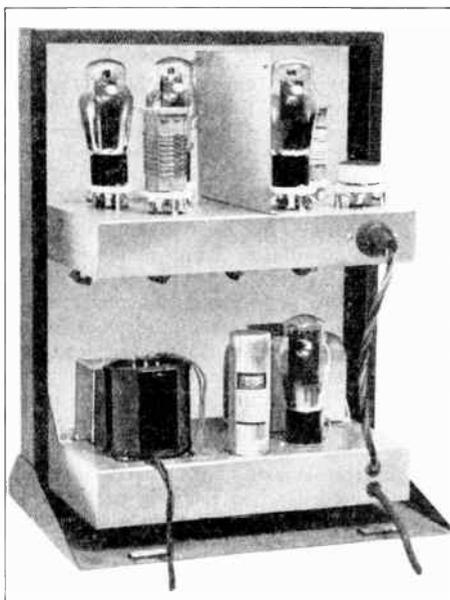
Figure 7—The Complete 6L6G Transmitter or High-Power Exciter, with Power Supply on the Lower Chassis. Five-Band Operation is Secured, with High Output for Either Direct Connection to an Antenna or Feeder System or as a Driver for a Medium Power R. F. Amplifier.
