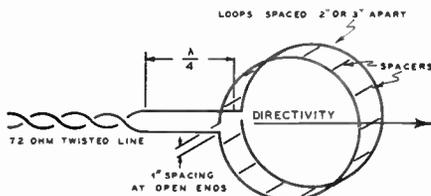
Figure 94—Reinartz Rotary Beam with Twisted-Pair Feeder and Stub.
