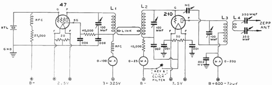
**Figure 22—Complete Circuit Diagram of 47 Oscillator link coupled to 210 amplifier stage. One or two turns of wire are wound around coils L1 and L2 to form the coupling loop. The two loops are connected through a twisted-pair feed line, made with hook-up wire.**
