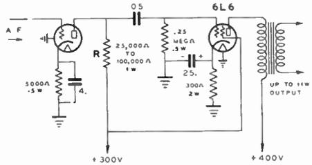
6L6 Audio Amplifier with 6F5 Driver. Low Values of "R" Tend to Generate Out-of-Phase 2nd Harmonic Which Cancels Distortion of 6L6 as Single-Tube Audio Amplifier
