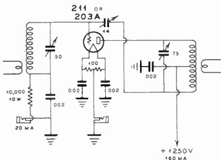
Figure 15—Circuit for 211 Amplifier Pictured in Figure 14.
