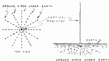
Figure 5—Ground System For Vertical Radiator.
