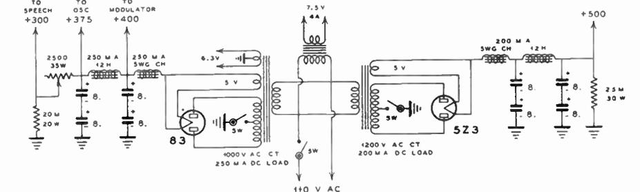
**Figure 5—Two Power Supplies Provide All Necessary Power for the Transmitter.**
