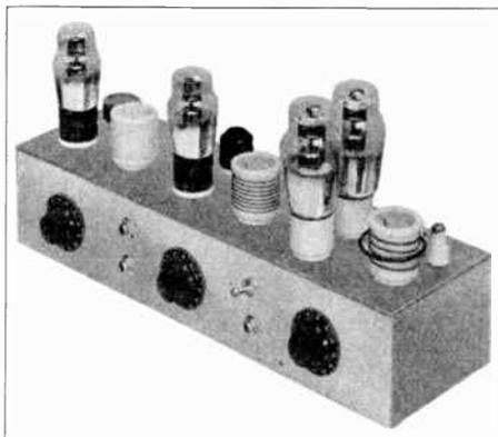
**Figure 25—Illustrating Physical Layout of Parts in the "Bi-Push" Exciter**
