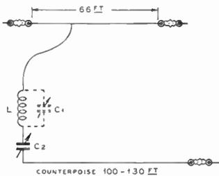
Figure 29—40-Meter Single-Wire-Fed Hertz for 160-Meter Operation. If "L" has sufficient turns, C1 is not required. "L" is coupled to the plate tank circuit.
