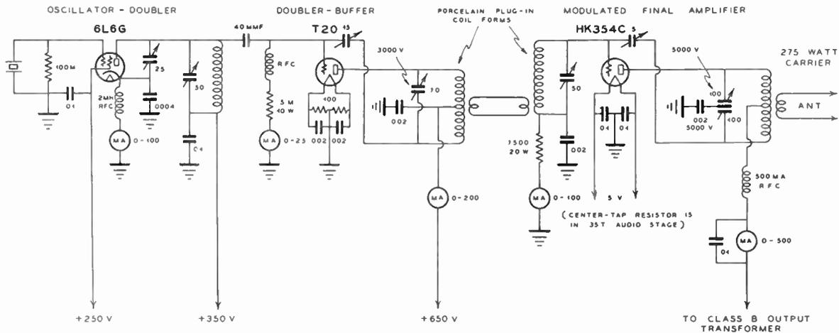
**Figure 9—Schematic diagram of the radio frequency portion of the 400-watt phone transmitter.**
