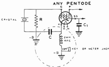
HIGH OUTPUT PENTODE CRYSTAL OSCILLATOR WITH REGENERATIVE FEATURE AS DEVELOPED BY JONES
