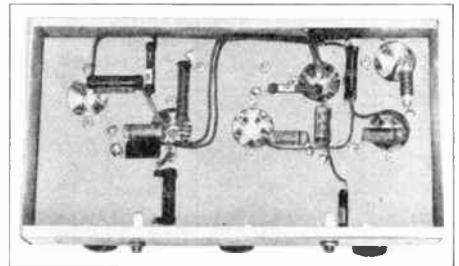
**Figure 21—Showing Construction of the 6A6-6L6 Five Band Exciter, Top and Bottom Views**
