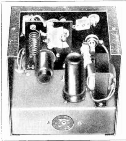
Figure 27—Interior View, showing Coil and Condenser Support, Also Horizontal Mounting of 6C5.
