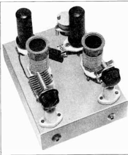
Figure 19—The Two Tube, 10 to 160 Meter 15-Watt Exciter
