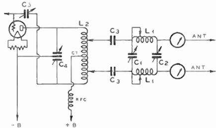
**Figure 37**—Two-Wire Line from Single-Ended Amplifier. Split-Stator Tuning and Series Feed.
