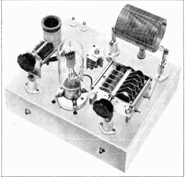
This amplifier can be driven by a 6L6G amplifier or doubler which delivers an output of 15 watts or more.
