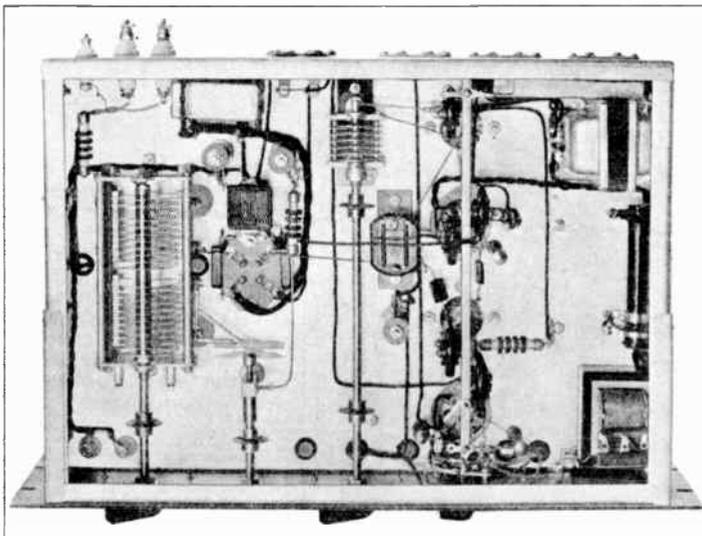
Figure 21—Underneath view of the exciter unit, showing placement of components. Extension shafts allow the various condensers to be placed closer to their associated circuits.
