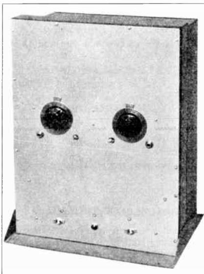
Figure 6—Front View of Housing for a Small Transmitter or High-Power Exciter. The Two Dial Lights for Tuning are Clearly Seen Between the Tuning Dials. These Dial Lights Obviate the Need of a Milliammeter.
