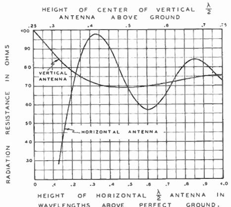
**Figure 3—Effect of Height on the Radiation Resistance of a Dipole**
