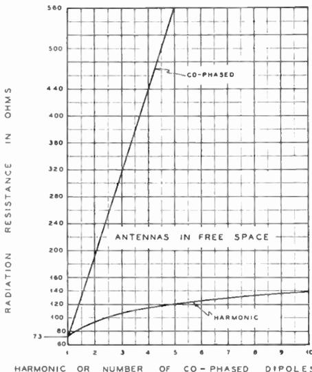
**Figure 45—Radiation resistance (at a voltage node) versus harmonic or co-phased elements**
