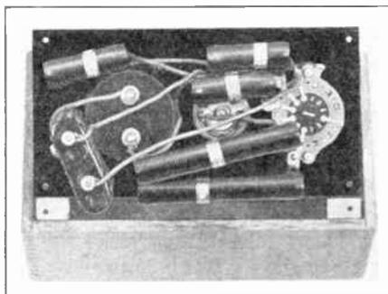
**Figure 16—Interior View of Ohmmeter, Showing Battery, Rotary Switch and Ohmite Resistors.**
