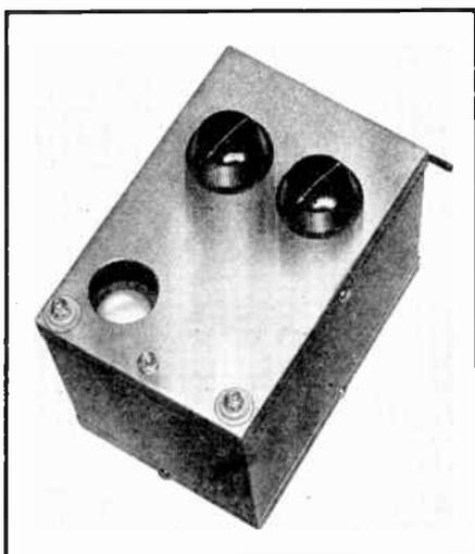
**Figure 28—Exterior View of 913 Oscilloscope.**
