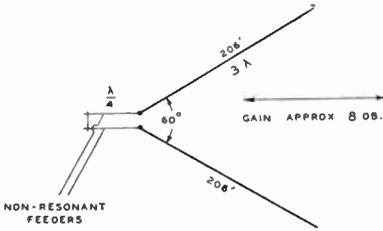
**Figure 86—20 Meter "V" with Moderate Gain and Directivity, Best Suited for General Amateur Use**
