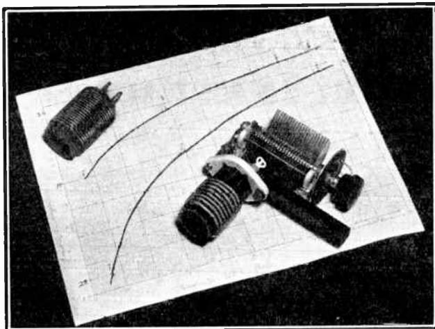
**Figure 3—Simple Absorption Type Wavemeter, Useful for Identifying Harmonics**
