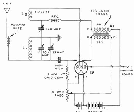
Figure 3—Schematic circuit diagram of the one-tube receiver. L1 is the secondary, or grid coil. L2 is the "tickler," or regeneration coil.
