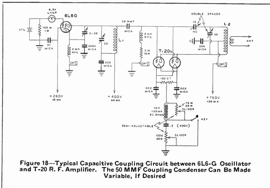
Figure 18—Typical Capacitive Coupling Circuit between 6L6-G Oscillator and T-20 R. F. Amplifier. The 50 MMF Coupling Condenser Can Be Made Variable, If Desired
