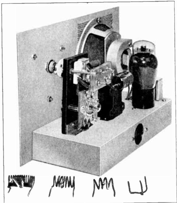
**Figure 23—One-to-Ten-Meter Super-regenerative Receiver with Loudspeaker Output. A feature of this receiver is the almost complete absence of connecting leads. Note arrangement and assembly of tube socket and coil holder. In the foreground are the coils for 1-,  $2\frac{1}{2}$ - and 5-meter operation.**
