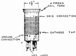
Each coil has three connections: top, bottom, and cathode-tap. These connections are made to three of the coil prongs; the wires must be soldered into the prongs.
