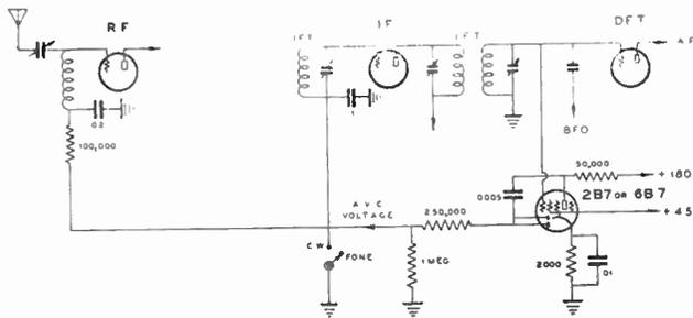
**Figure 10—Automatic volume control is a distinct advantage when the receiver is used for phone reception. It automatically compensates for signal fading. Briefly, the carrier signal strength causes a control voltage to vary in proportion to the actual carrier intensity.**
