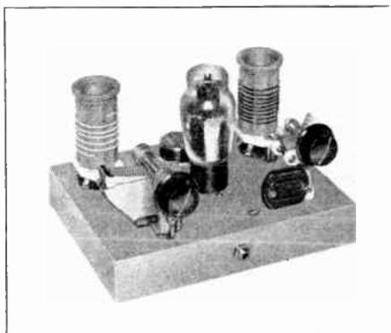
**Figure 7—6L6G Tritet Oscillator for Operation on Both Fundamental Frequency and Second Harmonic**
