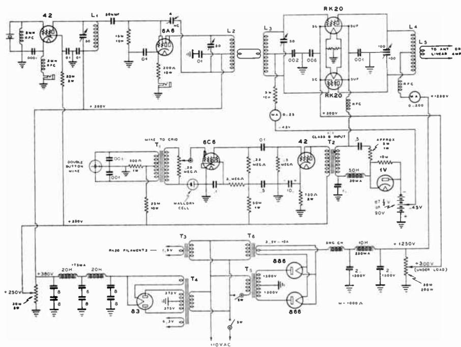
SUPPRESSOR MODULATED - CONTROLLED CARRIER PHONE
