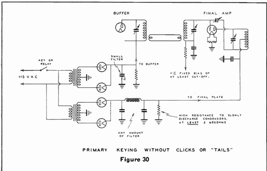
filter has no appreciable time lag, and will not add tails to the dots and dashes, but it does provide sufficient time lag for key click elimination. The small amount of filter will not introduce a.c. hum modulation into the output of the final amplifier, because the latter is operated in class-C, under saturated grid conditions. A moderate a.c. ripple in the grid excitation will not introduce hum in the output circuit under this operating condition.
