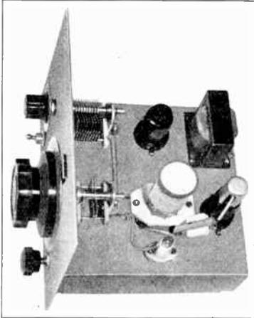
**Figure 8**—Metal tube version of the receiver. The circuit is the same, though the mechanical layout is slightly different. It is built on a metal chassis instead of a wood baseboard.
