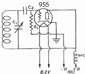
**Figure 11—RCA 955—Circuit Diagram and Suggested Layout.**
