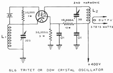
The Same Circuit Is Also Suitable for 41, 42, 2A5 89 and 6F6 Tubes
