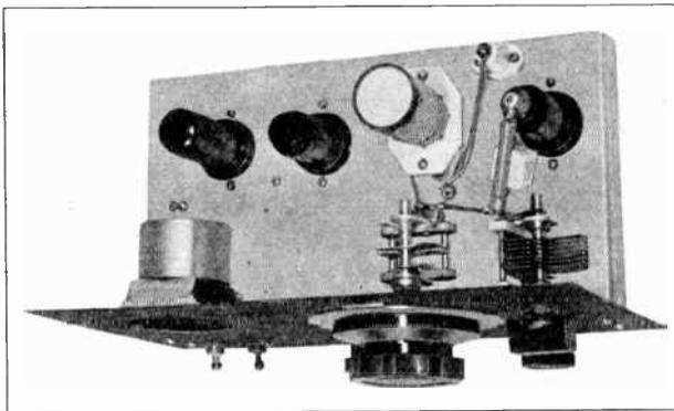
**Figure 10**—Interior of the receiver illustrated in figure 9. The permanent magnet, dynamic loudspeaker at the extreme left gives ample volume for enjoyable room reception of both code and voice signals.
