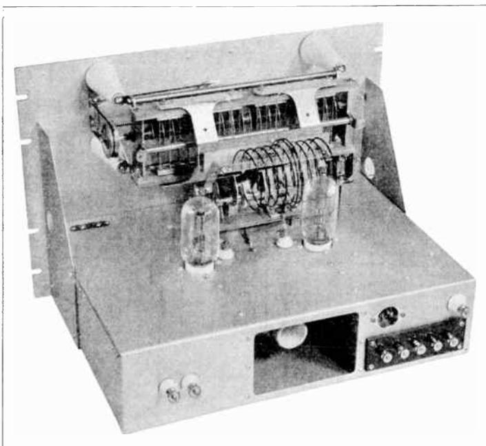
Figure 22—The 250-Watt 35-T Amplifier. This stage is either plate modulated or used to drive the high-power modulated amplifier. The plate tuning condenser is mounted parallel with the front panel to allow shorter leads, and is driven by cord and pulleys.
