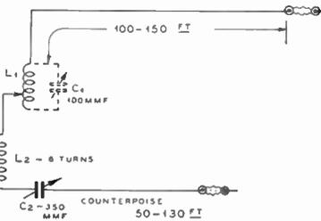
Figure 30—System for Loading Any Antenna for 160-Meter Operation.
