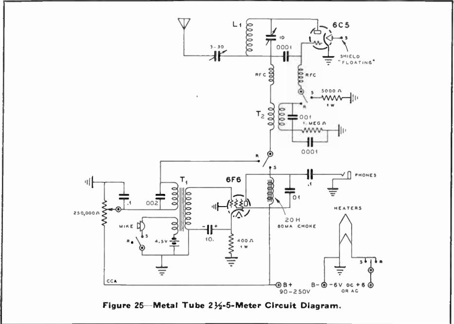
**Figure 25—Metal Tube 2½-5-Meter Circuit Diagram.**
