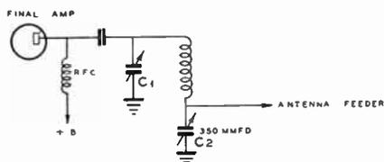
**Figure 39—Simplified Pi Antenna Coupling System.** The 350- $\mu$ mfd. condenser is an ordinary receiving type variable condenser.
