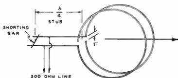
Figure 95—Reinartz Rotary Beam Antenna with Spaced Feeder and Stub.
