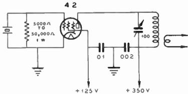
Figure 2—Pentode Crystal Oscillator with Type '42 Tube
