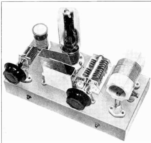
Figure 14—The “Old Reliable” Type 211 or 203A Triode is Still Widely Used by Amateurs. The Amplifier Design is Ideal for Such Tubes. The Larger-Than-Usual Neutralizing Condenser is Easily Made from Aluminum, Bent as Shown in the Photograph, with One of the Sections Attached Directly to the Stator of the Plate - Tuning Condenser. Note How Well the Parts Lend Themselves to Symmetry in This Design.
