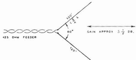
Figure 84—20 Meter "V" Antenna, Smallest Worthwhile Size
