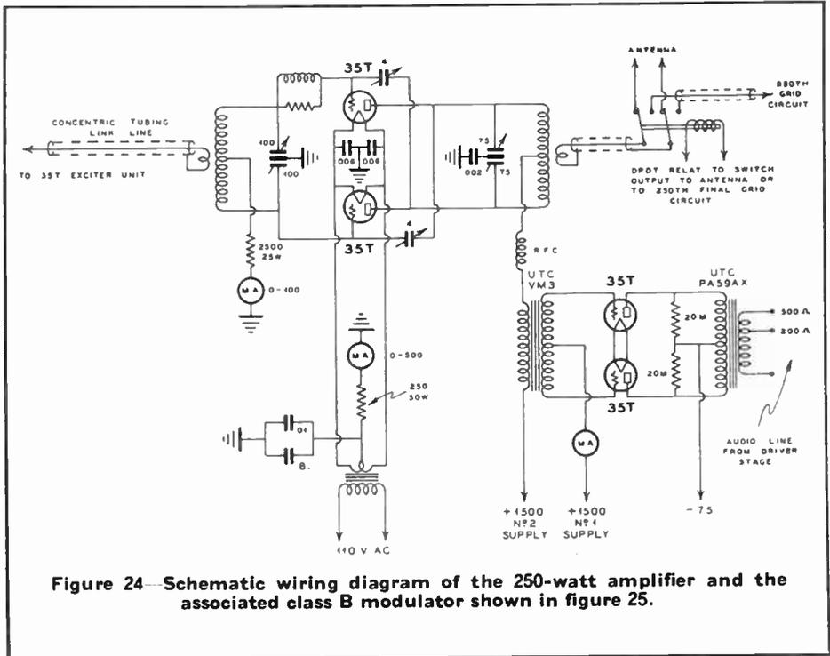
**Figure 24—Schematic wiring diagram of the 250-watt amplifier and the associated class B modulator shown in figure 25.**
