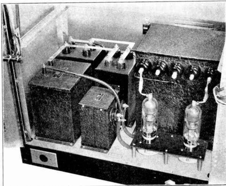
Figure 37—High voltage, high power plate supply referred to in figure 36.
