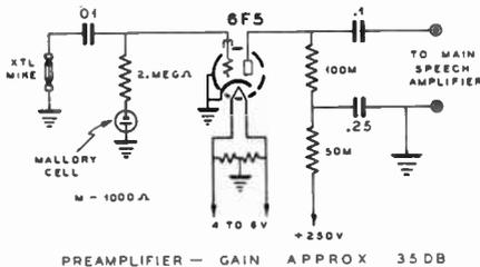
**Figure 7—This pre-amplifier can be used with an inductive microphone by changing the resistance network in the input to a transformer of the correct design. If the pre-amplifier is far removed from the main speech amplifier, a plate-to-500-ohm-line transformer should be connected in the output, with a corresponding 500 ohm-to-grid transformer at the speech amplifier.**
