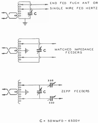
**Figure 43—Link Coupling from Final Amplifier to Tuned-Antenna Circuits.**
