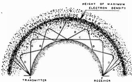
Figure 1—Reflection of Radio Waves from the Kennelly-Heaviside Layer Around the Earth
