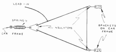
**Figure 110—Triangular Antenna**
