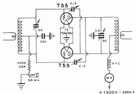
**Figure 29—Push-Pull 300-Watt Amplifier with T-55 Tubes.**
