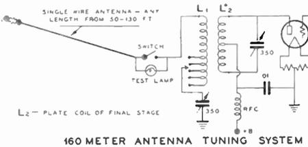
**Figure 35**—The circuit shows a tuning lamp in series with the antenna and a shorting switch for bridging the lamp after the antenna is tuned. Another method is to wrap a turn or two of the lead-in wire around a 2-turn loop connected to the lamp. The former system is best adapted for low power, the latter for medium or high power.
