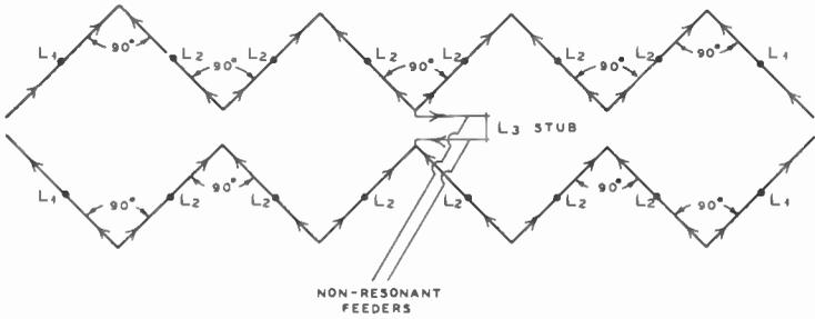
CHIREIX-MESNY ARRAY — VERTICALLY POLARIZED — GAIN APPROX 8 DB.
