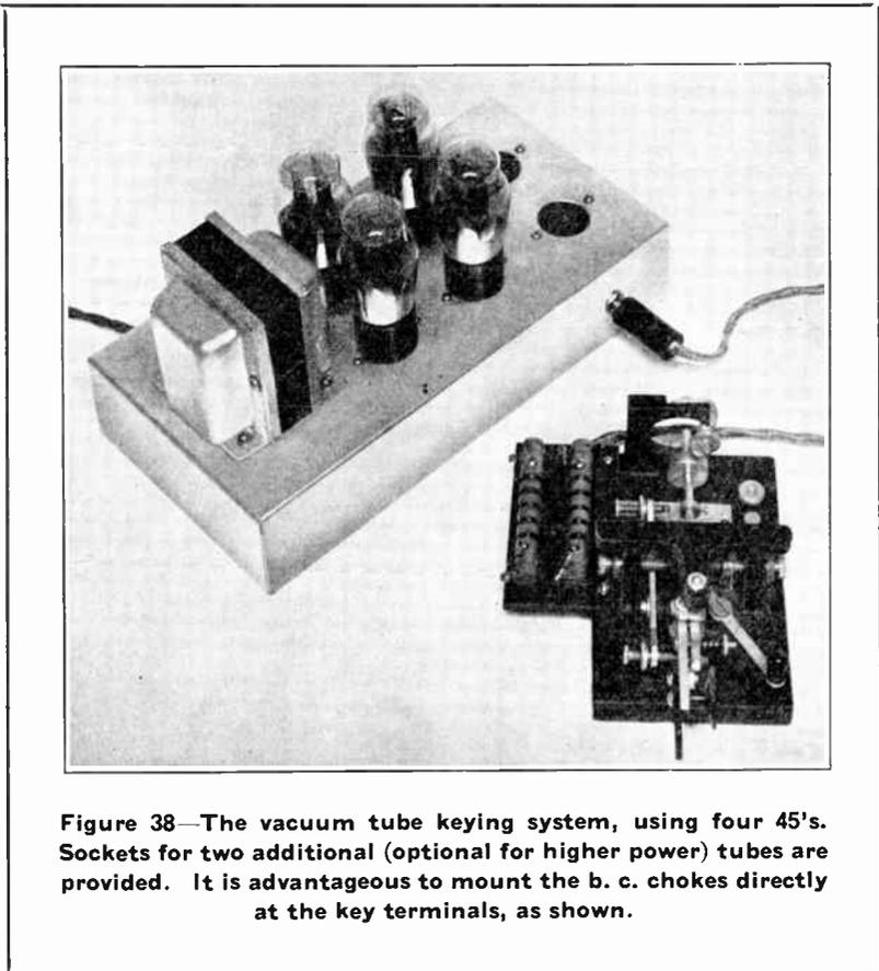
which is shunted from grid to filament, and the values of the two high resistances in series with the grid and power supply leads. R.f. chokes can be connected in series with the key directly at the key terminals, to prevent the minute spark at the key contacts from causing interference in nearby broadcast receivers. These r.f. chokes are of the conventional b.c. type. There is no danger of shock to the operator when this keying circuit is used.
