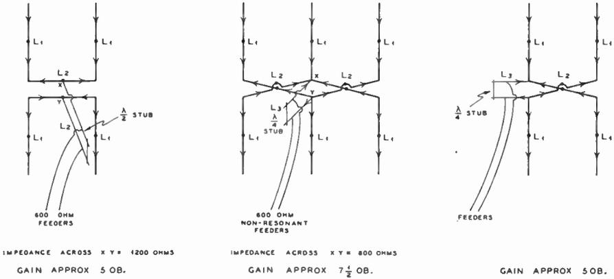
STACKED DIPOLE ANTENNAS — BROADSIDE RADIATION
