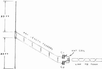
Figure 17—20- and 40-Meter Vertical Antenna with Zepp. Feeders. C1-C2 Are .00025  $\mu$ f. Condensers.
