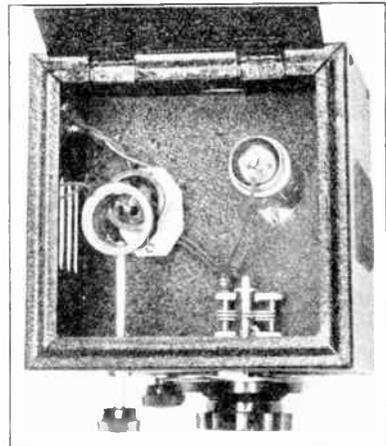
**Figure 21—Regenerative Pre-Selector with Noise Balancing Antenna Circuit and Variable Antenna Coupling.**
