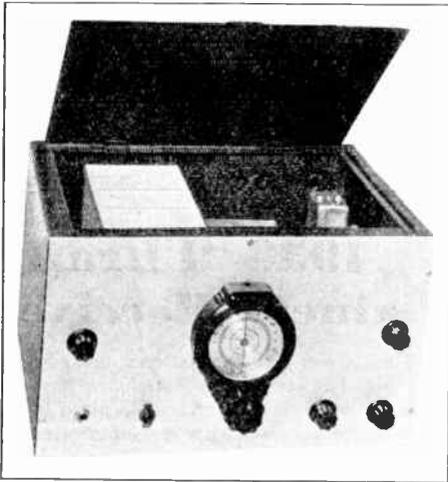
Figure 15—The 1938 "Ultra Gainer" receiver, showing fully enclosed coil shield compartment and front panel layout.
