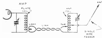
Figure 10—Alternate Method of Coupling Single-Wire Fed Antenna by Tapping the Link Line Directly to the Antenna Coil. The Lower End of the Antenna Coil Should be Grounded.
