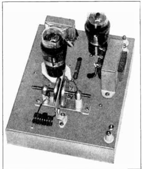
Figure 41—Stabilized U.H.F. Oscillator, diagrammed in figure 42. Note center plate between adjustable rotors of a standard, small size neutralizing-type condenser. It is of importance that the components be placed precisely as shown.
