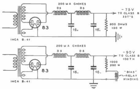
Figure 27—Showing bias supply for the 35-T modulator (above) and the bias supply for the 100-TH modulator (below).
