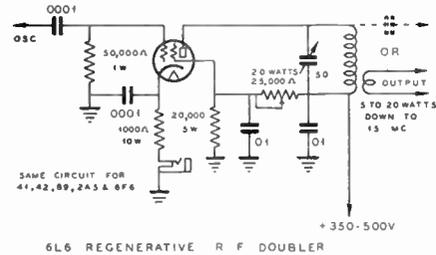
Circuit also Suitable for Other Tubes, Such as 41 42, 2A5, 89 and 6F6
