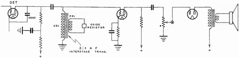
Figure 22—Oxide Rectifier Noise Silencer Circuit for Loud Speaker.
