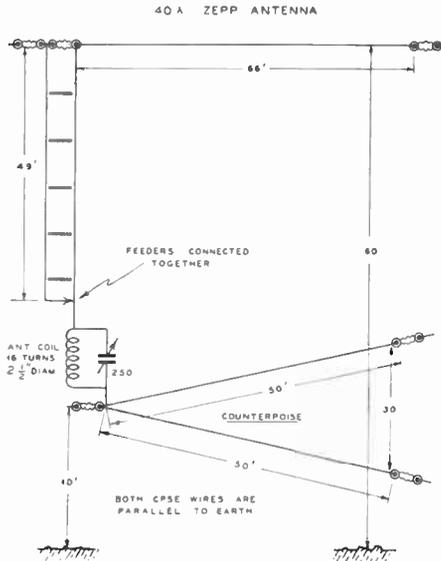
Figure 28—160 Meter Operation From a 40-Meter Zeppe. Where space is limited, the 40-meter zeppe-fed Hertz antenna illustrated above will give satisfactory operation on 160 meters. The zeppe feeders are connected together at the station end and attached to one side of the tuning condenser and coil, as shown in the diagram. The remaining ends of the coil and condenser connect to the counterpoise.
