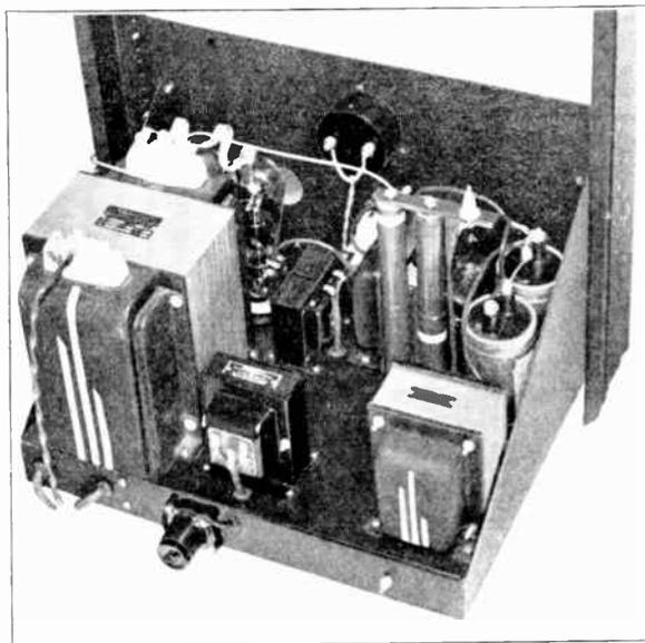
Figure 35—A laboratory type power supply which makes provision for various heater and plate voltages, with socket plugs for cable connections to any device under test. Some components are secured directly to the front panel, the others on a sub-deck. A variable resistor allows fine voltage adjustment over a wide range.
