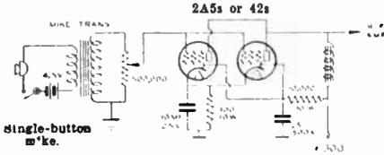
**Figure 3—10-Watt Amplifier for Use with a Single-Button Microphone.**
