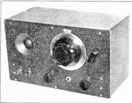
**Figure 9**—Another modification of the simple regenerative receiver. A miniature loud-speaker and conventional pentode power audio stage have been added. A 7 x 12 x 7 in. metal cabinet houses the complete receiver.
