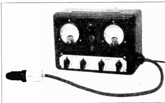
Figure 9—Front View of the Peak V. T. Voltmeter
