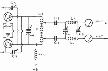
**Figure 38**—Coupling a Two-Wire Line to a Push-Pull Final Amplifier. Single-Wire Line Out of a Push-Pull Final Through a PI Network is Not Recommended.
