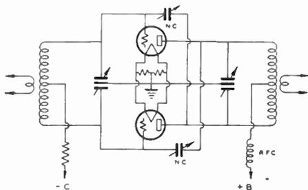
**Figure 10—Push-pull r.f. amplifier stage**
