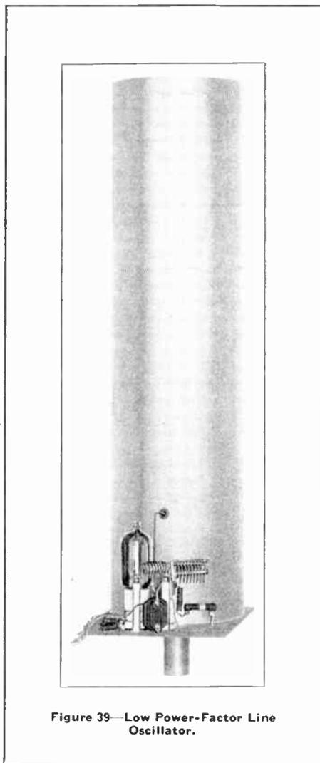
Figure 39—Low Power-Factor Line Oscillator.
