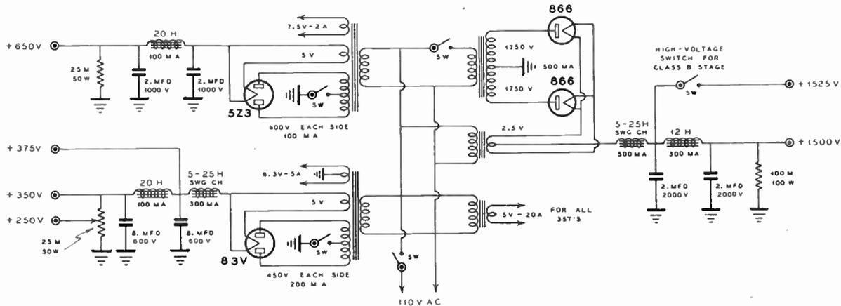
Figure 11—Low, medium, and high voltage power supplies for the medium power radiophone.
