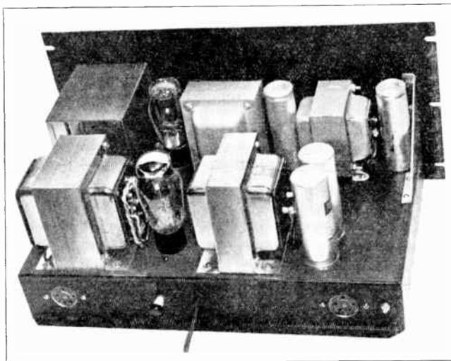
**Figure 33—Dual-power supply for crystal oscillator, buffer-doubler and speech amplifier service. The unit closest to the front panel delivers from 350 to 400 volts, the other is a 600-volt supply for a buffer stage. Bleeder resistors are under the chassis. Wafer sockets are for plug-in terminals and cords.**
