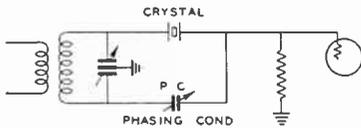
Figure 14—Typical Crystal Filter Circuit.
