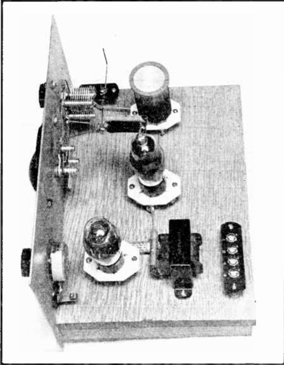
**Figure 5—Looking Into the Receiver. The Various Parts Should be Mounted Exactly as Shown.**
