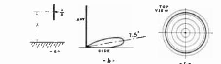
**Figure 6—Horizontal Half-Wave Antenna Radiation Patterns.**
