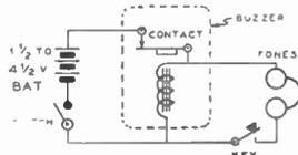
Figure 1—The Simplest Code Practice Set—a Key, Buzzer, Battery and Headphones. The Buzzer Operates Continuously, but Signals are Heard in the Headphones Only When the Key is Depressed.
