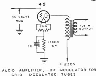
**AUDIO AMPLIFIER, - OR MODULATOR FOR GRID MODULATED TUBES**
