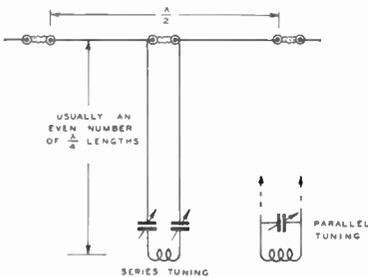
Figure 16—Center-Fed Zepp. Antenna.
