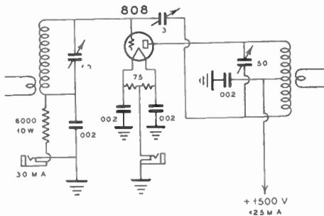
**Figure 15—Circuit of Amplifier Pictured in Figure 12.**
