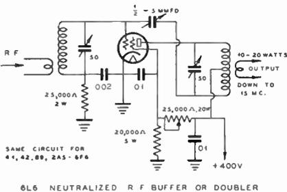
41, 42, 2A5, 89 or 6F6 Tubes Can Be Used in Same Circuit
