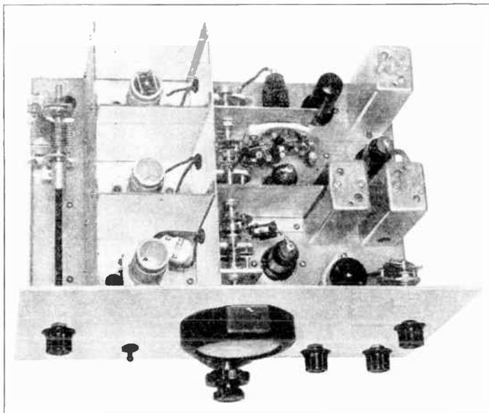
**Figure 16—**Illustrating assembly of the new "Ultra Gainer," showing antenna noise suppressor, shielded coil compartment (cover removed to show coils) and ganged condenser arrangement.
