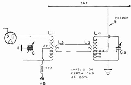
Figure 9—Single Wire Feeder Coupling to Final Amplifier.
