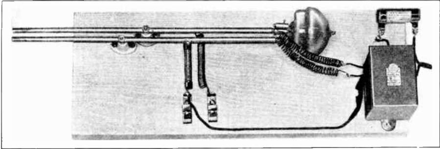
Figure 14—W.E.-316A  $\frac{3}{4}$ -Meter Oscillator.
