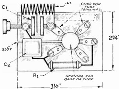
**Figure 12—Plan view of transmitter.**
