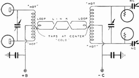
**Figure 21—Link coupling between push-pull stages**
