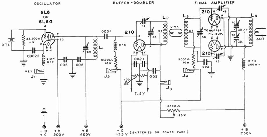
Figure 11—Circuit Diagram of R. F. Portion of 210 C. W. Transmitter.
