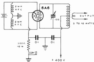
Figure 3—Dual-Triode 6A6 (or 53) High-Output Push-Pull Oscillator
