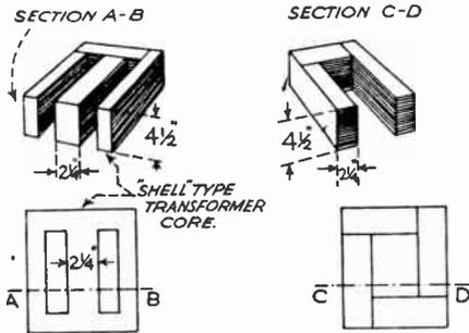
Figure 41—Types of Transformer Cores.
