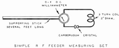
Figure 14—Simple Circuit Diagram of Device Illustrated in Figure 13.
