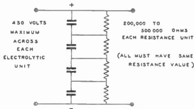
**Figure 13—Electrolytic condensers connected in series plus to minus, with 500,000-ohm, 1-watt, resistor connected across each condenser in order to equalize the leakage and to prevent excessive strain on any one section of condenser.**
