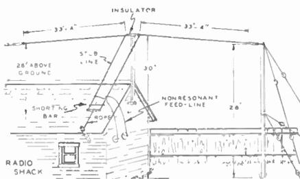
20METER DIRECTIVE ANTENNA - (2 HALF-WAVE SECTIONS)
