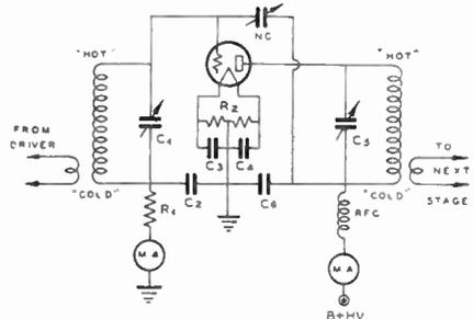
Figure 20—Link coupling between single-ended stages
