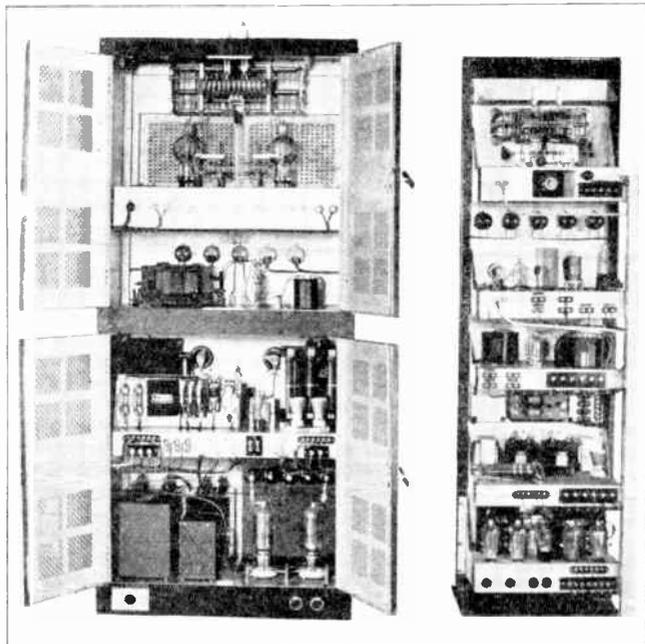
the deck of each amplifier in order to prevent excessive voltage drop in the connecting leads to the tube sockets. The neutralizing condenser for the 35T is adjusted from the front panel by means of an extension shaft.
