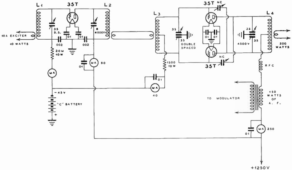
**Figure 44—General Wiring Diagram of the 5 and 10 Meter 200 Watt Unit. It Can Be Driven by Any 10 Watt 10 Meter Exciter**
