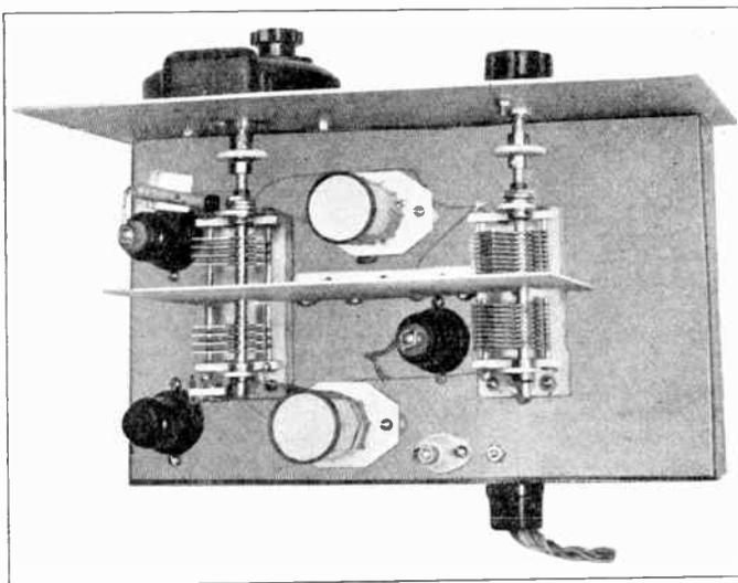
**Figure 14—Interior view of the t.r.f. amateur type receiver. The receiver should preferably be housed in a metal container in order to reduce hum pickup.**
