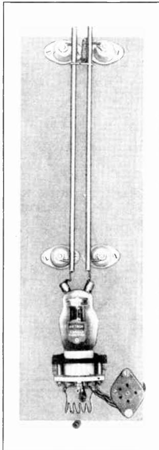
Figure 19—Raytheon RK-34  $2\frac{1}{2}$ -Meter Oscillator.
