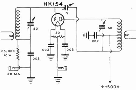
Figure 27—HK-154 Amplifier. It Will Supply 200 Watts Output for C. W. Operation. Figure 26 Shows the Mechanical Design.
