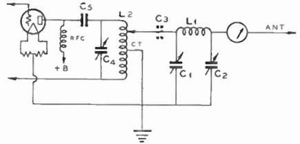
**Figure 36**—Single-Wire Feed Line—Single Section Plate Tuning Condenser—Shunt Feed.  $C_1$  and  $C_2$  in All Circuits Are .00035  $\mu$ fd.
