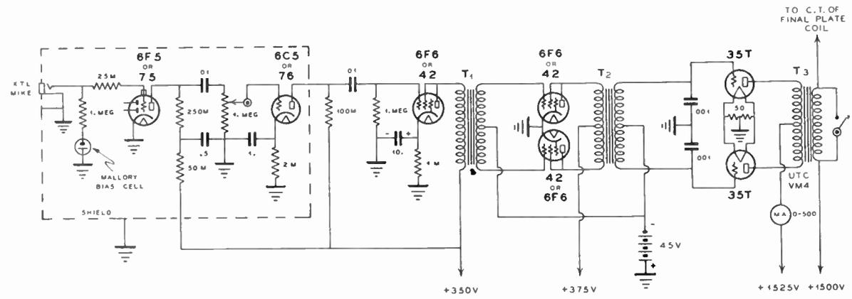
Figure 10—Audio channel and modulator for the HK-354C radiophone transmitter.
