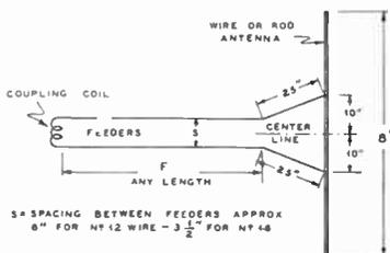
**Figure 96—5-Meter Matched Impedance Antenna**
