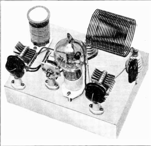
Figure 18—Standard Low-Cost Parts are Used in This Amplifier. The Tube is an RK - 35 Triode. Double-Spaced 50  $\mu\text{fd}$ . Midget Variable Condensers Tune Both the Grid and Plate Circuits. Neutralizing Condenser is a Standard 4- $\mu\text{fd}$ ·Wide-Spaced Midget. When Mounted Behind a Metal Relay-Rack Panel, Condenser Shafts Should be Fitted with Insulated Couplings.
