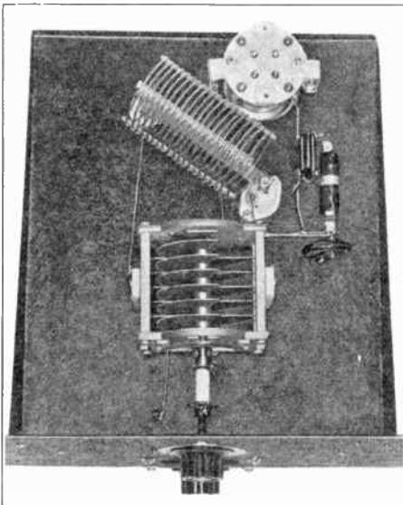
Figure 36—Under-Subpanel View of 1-Kw. R.F. Amplifier, Showing Grid Coil and Tuning Condenser, Method of Socket Mounting and Arrangement of Resistor and Bypass Condensers.
