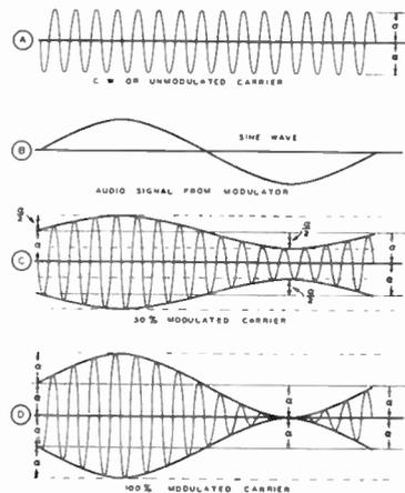
Figure 1—Graphical representation of four types of wave form, illustrating the difference between an unmodulated carrier, audio sine wave, 50 per cent modulated carrier, and 100 per cent modulated carrier.
