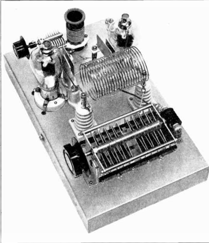
**Figure 28—Push-Pull R. F. Amplifier with Taylor T-55 Triodes. Home-Built Neutralizing Condensers are Mounted on Stand-off Insulators, the Assembly Being Clearly Shown in the Photograph. The Grid Coil and Grid-Tuning Condensers are at the Extreme Left. Symmetrical Layout of Parts is All-Important in Amplifier Design. The Amplifier Illustrated Above Adapts Itself to Numerous Types of Tubes, Such as T-55s, 35T's, 808's, RK-35's, etc.**
