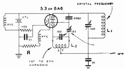
Figure 5—Jones Regenerative Exciter for all-band operation. R-50,000 ohms
