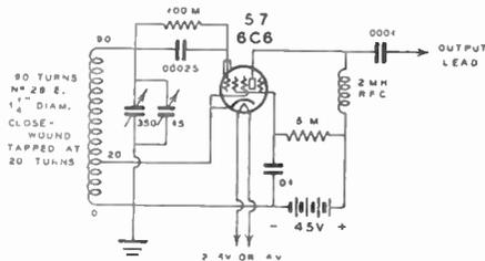
**Figure 24—With Heater Type Tubes, Battery Plate Supply is Still Good for Stability.**
