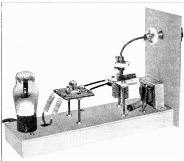
Figure 22—Practical Micro-Wave Receiver with Acorn Triode Detector and '76 Audio Stage. This design must be rigidly adhered to, and all specifications closely followed.
