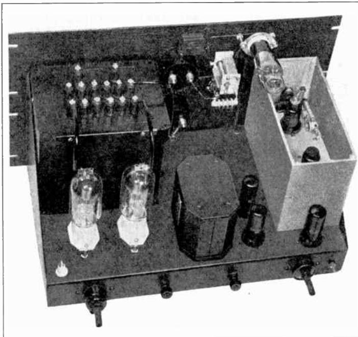
**Figure 14** — Speech amplifier for crystal microphone, and 35-T modulator unit. The first two stages of the speech amplifier are housed in a grounded metal box. The over-modulation indicator components are fastened directly to the front panel.
