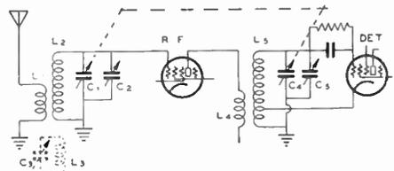
Figure 7—R. F. Amplifier and Regenerative Detector Circuit
