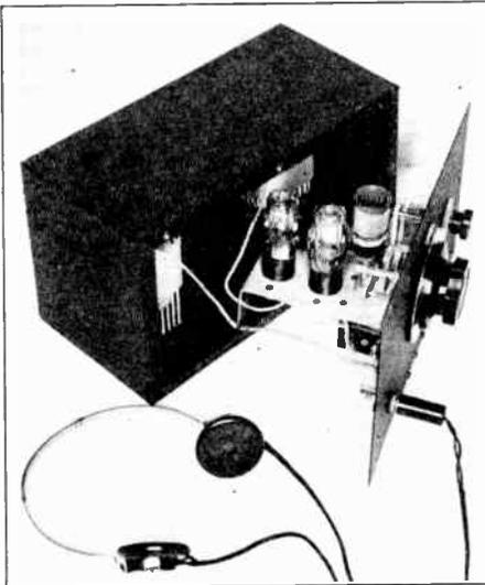
Figure 26—Illustrating Construction of the C. W. Monitor.
