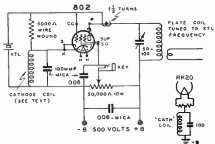
Figure 12—Reinartz 802 Oscillator Circuit
