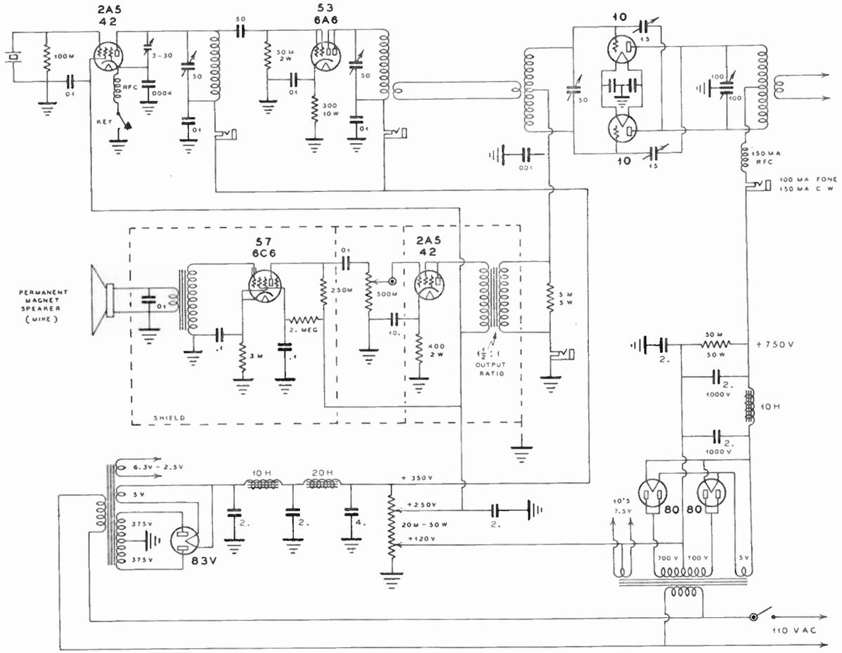
and the 7.5-volt filament center-tap lead to the proper point on the bleeder resistor of the 350-volt power supply. This positive 120-volt bias is obtained under normal load conditions by adjustment of the slider on the bleeder resistor. This positive bias on the filaments of the type-10 tubes provides a *negative* bias of 120 volts to the grids of the 10's. The bias is approximately  $1\frac{1}{2}$  times cutoff.
