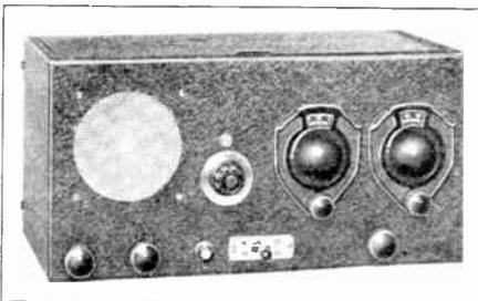
**Figure 33—Front View of High-Output 6A6 Transmitter-Receiver.**
