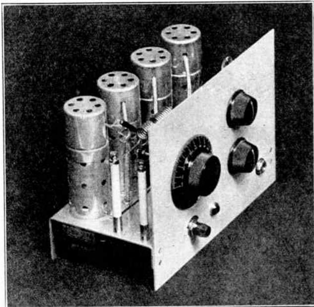
Figure 28—The Complete 5-Meter R-C Coupled Superheterodyne.
