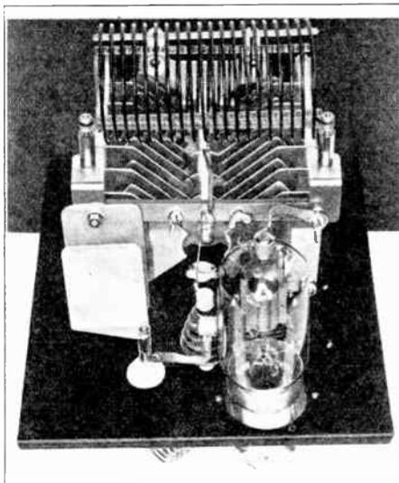
Figure 35—1-Kw. R. F. Amplifier with HK-354D Gammatron and New Atkins-Brown "Propeller-Type," Split-Stator Tuning Condenser. Note Extremely Short Connecting Leads.
