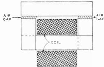
Figure 42—Two types of choke coil construction. The air-gap is approximately  $1/32$  inch.
