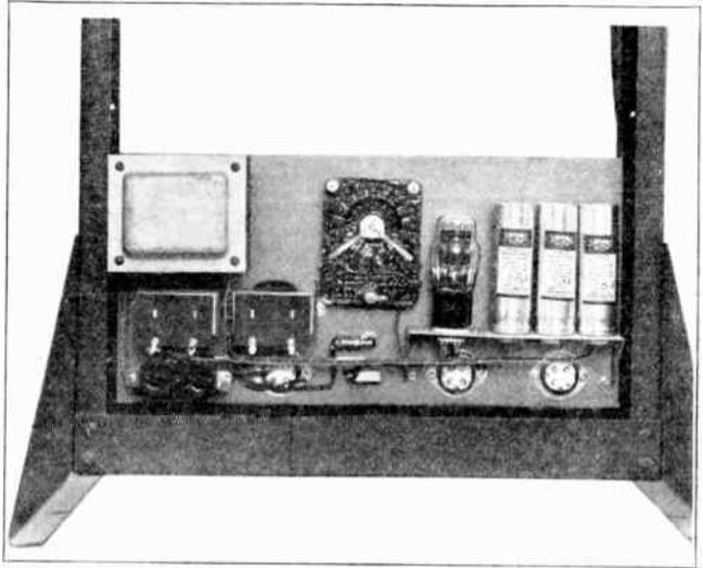
Figure 36—This unit, and the one illustrated in figure 37, are referred to in the W6LVS transmitter description in the radiotelephone construction chapter of this handbook. Figure 36 shows the relay-switching control unit, bias supply, bleeder resistors and filament supply transformers for a high power modulator. Figure 37 shows the high-power plate supply system for this same transmitter. A "pole pig" transformer, re-encased and re-impregnated, is shown at the far right in figure 37.
