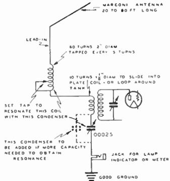
Figure 31—Loading System for Short Marconi Antenna for Boats, Aeroplanes, Etc.
