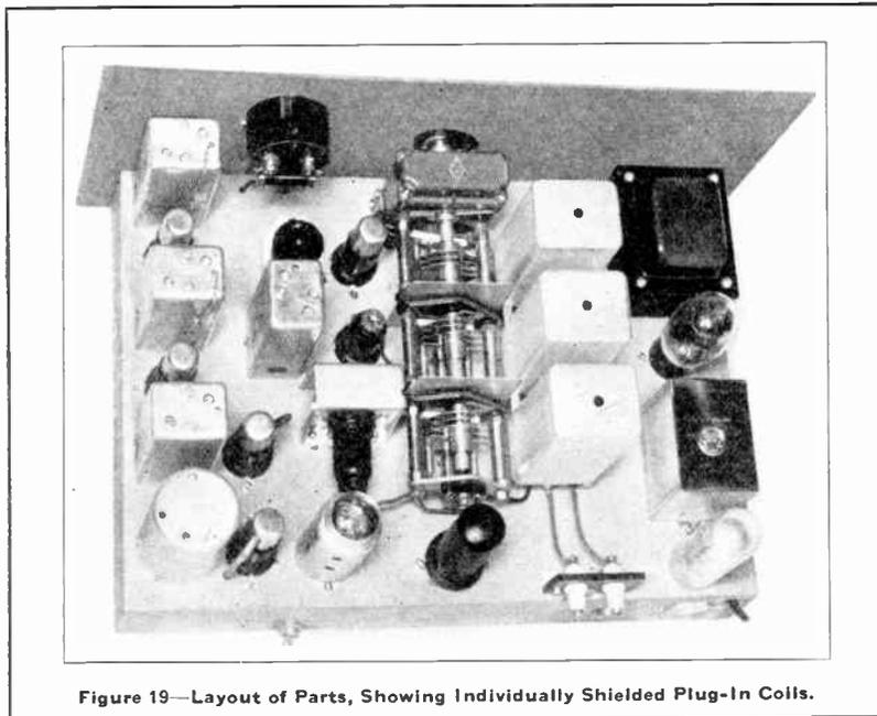
Figure 19—Layout of Parts, Showing Individually Shielded Plug-In Coils.
