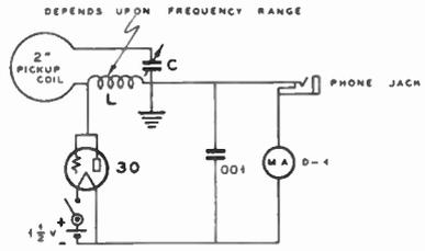
**WAVEMETER WITH DIODE INDICATOR**
