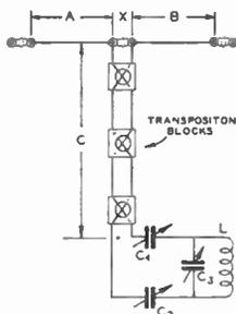
Figure 108—Noise-Reducing Shortwave Doublet Feeder System with Transposition Blocks.
