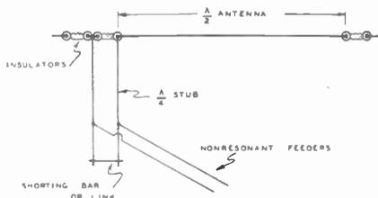
**Figure 18—Half-Wave Antenna with Quarter-Wave Matching Stub.**
