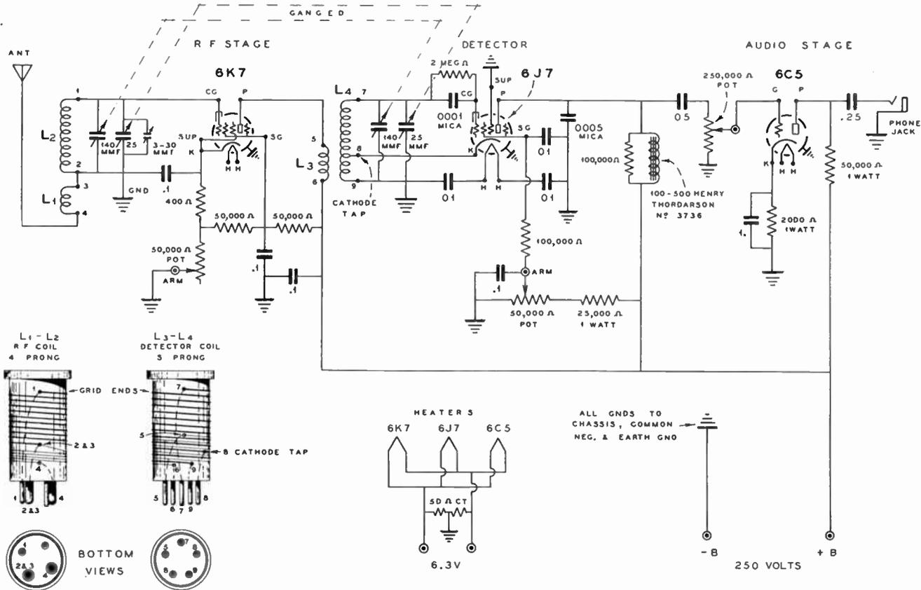
Figure 13—General Wiring Diagram and Coil Construction.
