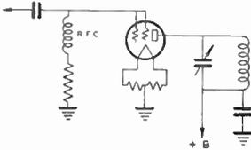
Figure 2—Simple doubler circuit with type 46 Tube
