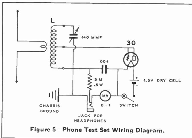
**Figure 5—Phone Test Set Wiring Diagram.**
