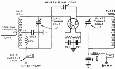
Figure 7—Grid neutralizing with series feed
