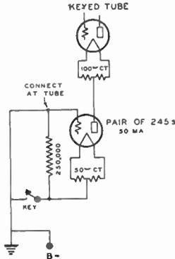
**Figure 36**—Vacuum Tube Keying. The circuit shows one of the more simple vacuum tube keying circuits. Some current flows through the key and this system sometimes produces clicks when the key is opened. Both filament transformers must be insulated from each other and also from ground. This circuit will not completely cut off the plate current to the keyed stage, but will reduce it to a very small value.
