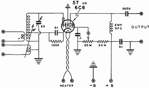
**Figure 22—Wiring Diagram of the Regenerative Preselector.**
