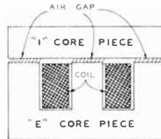
Figure 43—The air-gap can be filled with non-magnetic material, such as brass, bakelite, etc.
