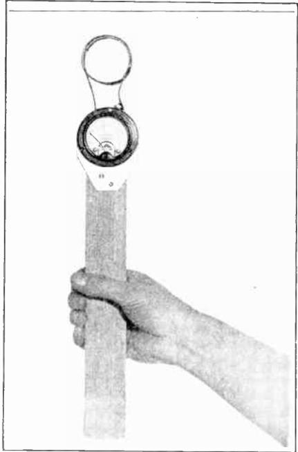
Figure 13—"Standing Wave Detector" and Field Strength Meter. The Device Is Moved Along the Feeder or Antenna, Held Close to the Wire in the Same Relative Position. A Variation of Current Denotes Standing Waves.
