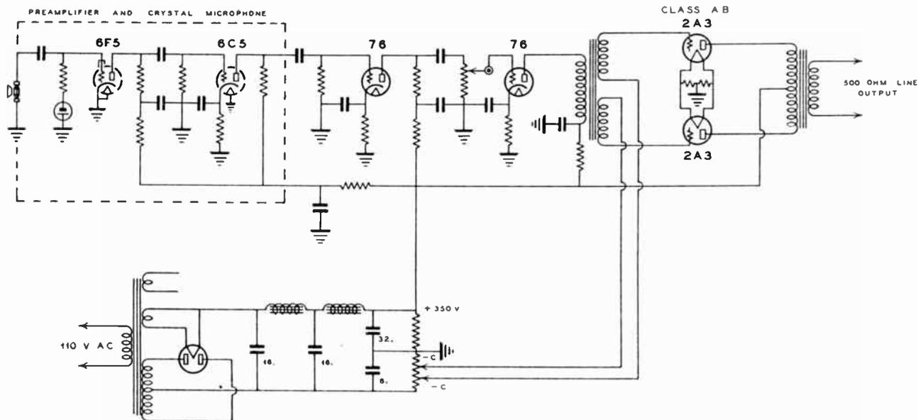
Figure 18—The Speech Amplifier-Driver Unit. It is used to drive either the medium or high power modulator. The first two stages (shown dotted) are built in a pre-amplifier can, on which the microphone is mounted. Coupling condenser and resistor values are conventional; those not familiar with them can find them elsewhere in this chapter.
