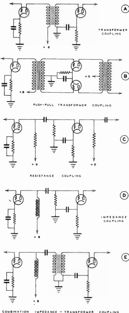
Figure 4—Five Common Methods of A.F. Interstage Coupling.
