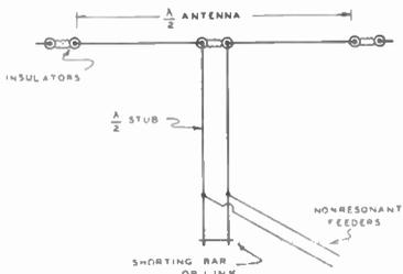
**Figure 19—Center-Fed Half-Wave Antenna with Half-Wave Matching Stub.**
