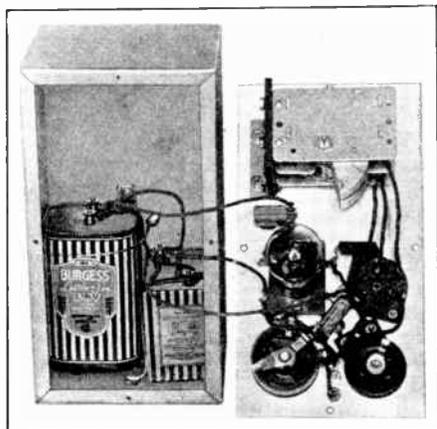
Figure 18—Interior View of All-Wave Test Signal Generator, Showing Type 30 Tube, Dry Cells, Condensers and Resistors.
