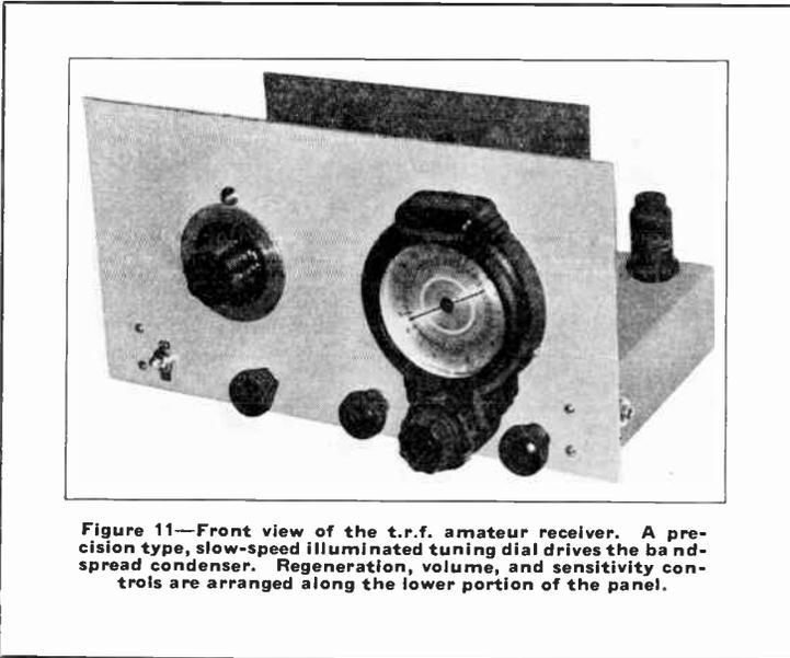
Figure 11—Front view of the t.r.f. amateur receiver. A precision type, slow-speed illuminated tuning dial drives the band-spread condenser. Regeneration, volume, and sensitivity controls are arranged along the lower portion of the panel.
