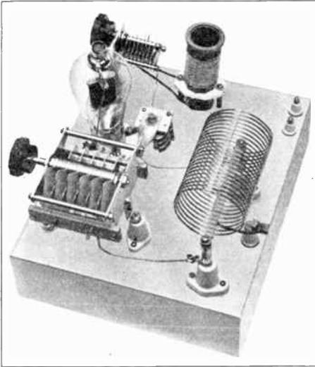
**Figure 20—Single-Ended R. F. Amplifier with Taylor T-55, or Similar Triode. This Amplifier is Suitable for Buffer Service. It Will Drive a 1-Kilowatt Amplifier for C. W. Operation.**
