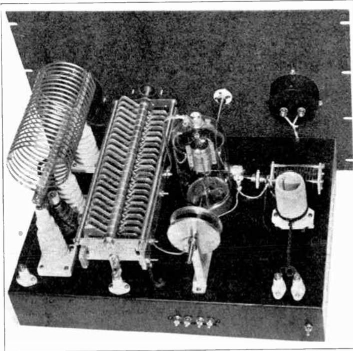
**Figure 13** — The modulated final amplifier uses an HK-354C running class C. The grid tuning condenser is mounted parallel to the front panel; a flexible cable connects it to the dial on the front panel.
