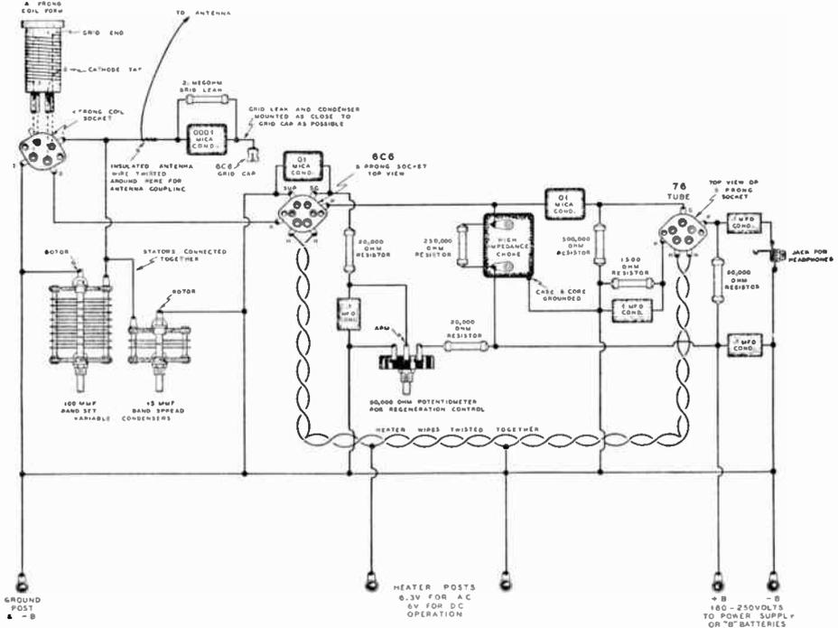
Figure 7—Schematic and Pictorial Circuit Diagrams of the Standard "Gainer" Regenerative Receiver.
