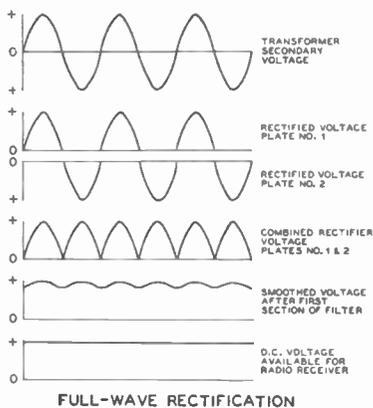
Figure 1—Showing effects of rectification and filtering of an AC current.
