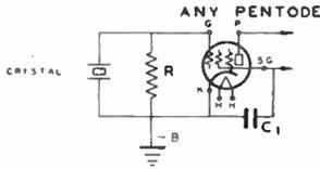
CONVENTIONAL LOW OUTPUT PENTODE CRYSTAL OSCILLATOR WITH GRIDLEAK BIAS RESISTOR
