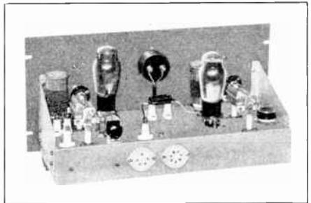
**Figure 9—6L6G Exciter and 210 Buffer-Doubler.**
