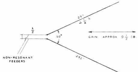
Figure 85—More Directive "V" Than Shown above, with More Efficient Method of Feed. Dimensions are for 20 Meters
