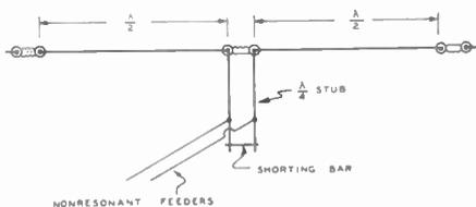
**Figure 21—Two Half-Wave Sections in Phase with Quarter-Wave Stub.**
