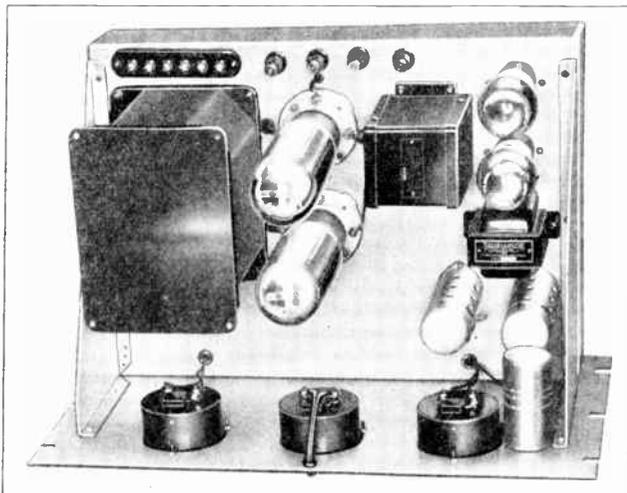
Figure 1—Relay Rack and Chassis for Mounting Heavy Modulator Components.
