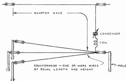
Figure 4—Typical Counterpoise System with Loading Coil and Series Tuning Condenser
