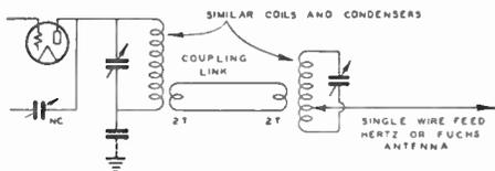
**Figure 41—Link Coupling for End-Fed or Single-Wire Feeders.**
