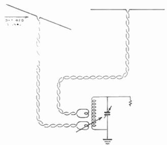
**Figure 92—Directive Doublet Receiving Antenna System.**
