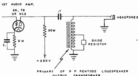
**Figure 21—Automatic Noise Limiter Circuit.**
