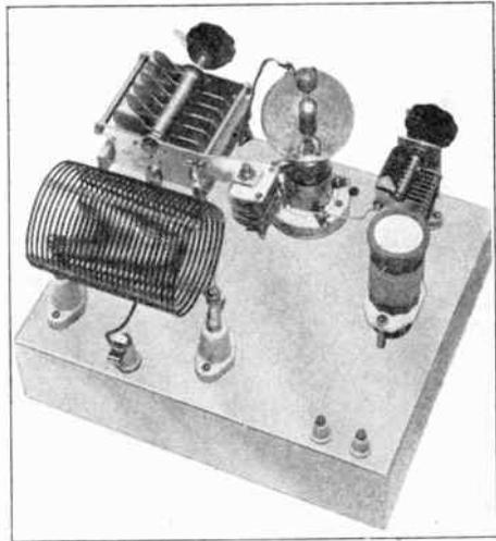
**Figure 12—RCA-808 Tantalum Plate Triode in a Simple, Effective R. F. Amplifier Unit.**
