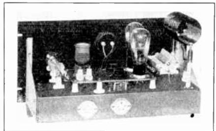
**Figure 10—Final Amplifier with Two 210 Tubes in Push-Pull. The Tubes, Grid Coil and Neutralizing Condensers are Mounted on a Separate Masonite "Deck," Supported on Small Insulators.**
