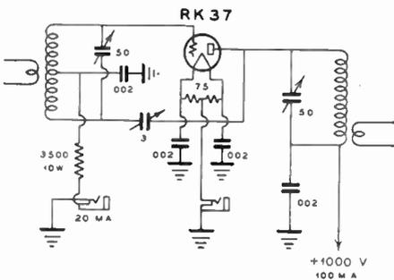
Figure 19—RK-37 Amplifier Circuit for the Unit Shown in Figure 18.
