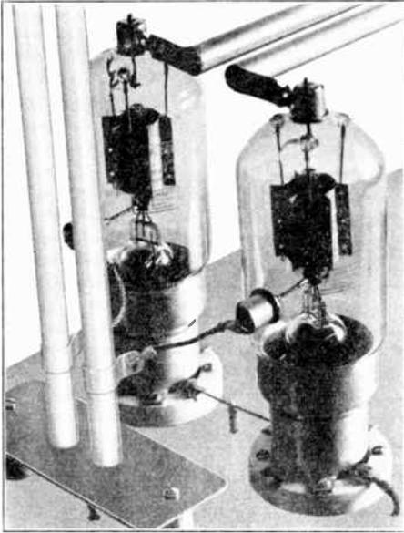
**Figure 36—Parallel Rod U.H.F. Oscillator with HK-354C Gammatrons in Push-Pull. The circuit diagram is shown in figure 37.**
