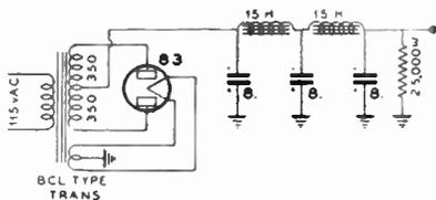
**Figure 29**—Here is a Bias Pack which uses a medium-to-high resistance bleeder. Voltage regulation is usually unimportant in biasing a class A modulator and very little bleeder is used.
