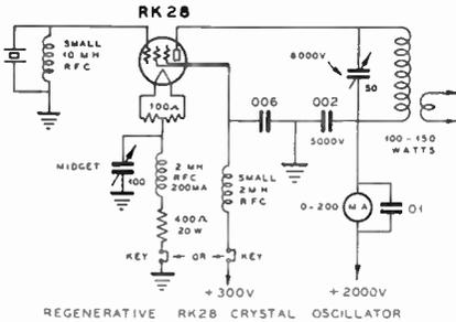
Figure 26—RK-28 Oscillator 100 to 150 Watts Output on 80 Meters
