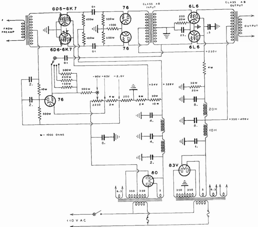
Figure 37—The gain of this amplifier varies inversely with the input signal.
