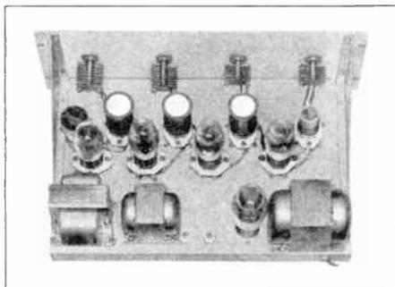
Figure 15—Top View of 6-Band Exciter. 5 to 160 Meter Operation
