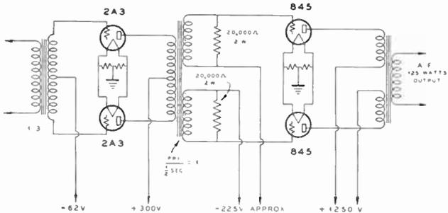
**125-Watt Output Modulator with 845's in Push-Pull with Provision for Balancing Plate Current**
