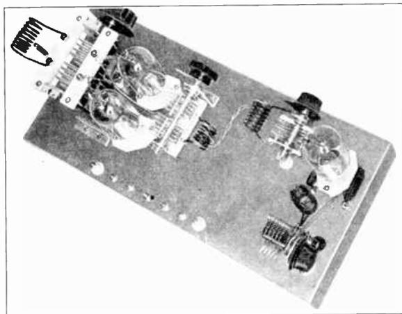
Figure 43—An ultra-efficient buffer-doubler and final r.f. amplifier for 5- and 10-meter operation. The illustration shows a complete group of 5-meter coils in their respective positions. The r.f. plate choke in the final stage is mounted closely to the center tap of the plate coil. Neutralizing condensers for the push-pull 35T stage are barely visible in the photograph; they are mounted directly under the final plate tuning condenser, close to the 35T's and the condenser terminals.
