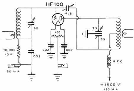
Figure 25—HF-100 Triode Amplifier. Figure 24 Shows Its Mechanical Construction.
