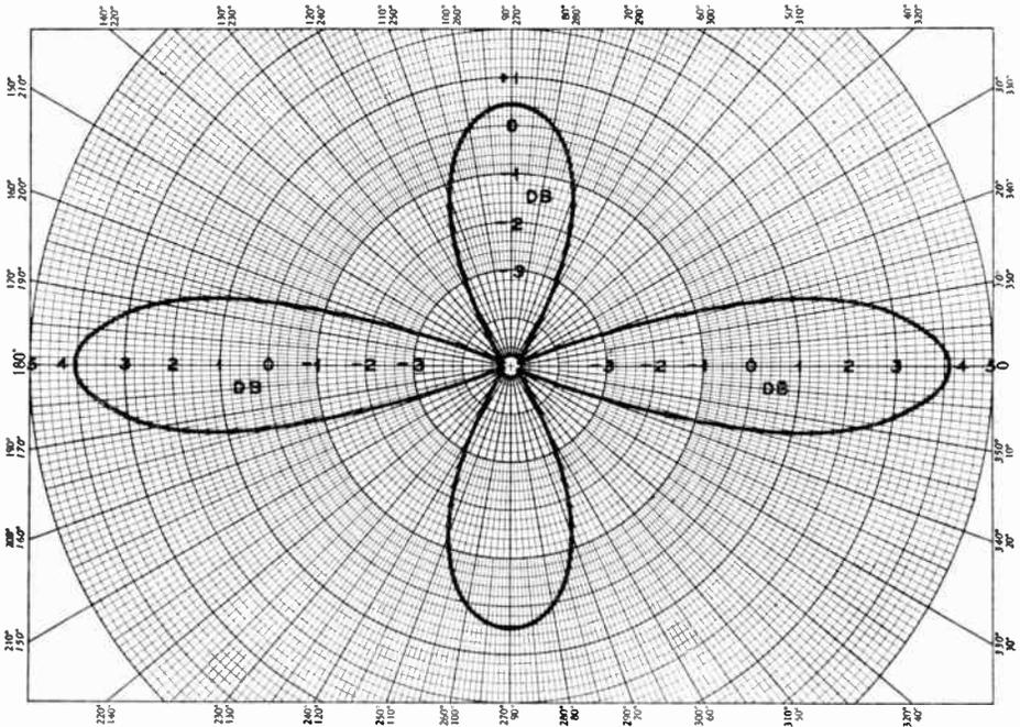
**RADIATION PATTERN IN A HORIZONTAL PLANE OF A "V" ANTENNA  $L = 1\lambda$   $\delta = 110^\circ$  ANGLE**
