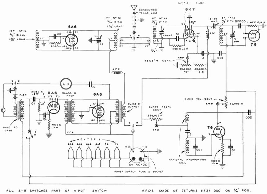
Figure 34—Complete Circuit Diagram of High-Output 6A6 Transmitter-Receiver.
