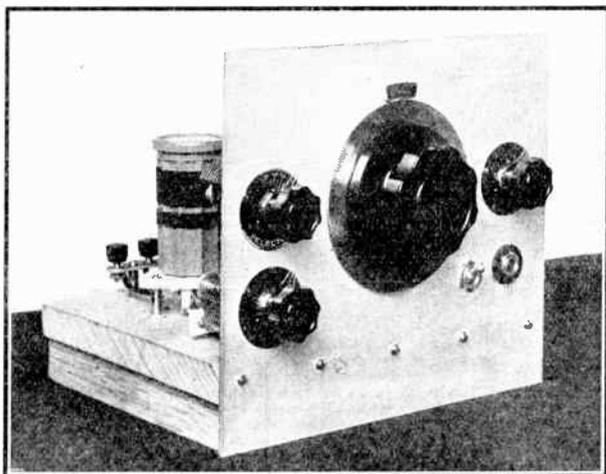
**Figure 1—Dual Triode Regenerative Receiver, wood baseboard model described in detail in the text. Components should preferably be mounted as shown here and in figure 2.**
