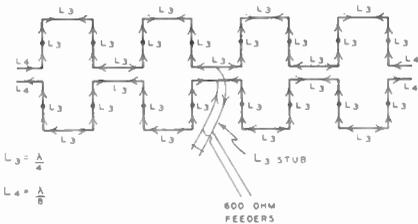
MODIFIED BRUCE ANTENNA WITH VERY EFFICIENT FEEDER SYSTEM AND DOUBLE ROW OF BRUCE ELEMENTS.
