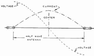
SHOWING HOW STANDING WAVES EXIST ON A RESONANT ANTENNA
