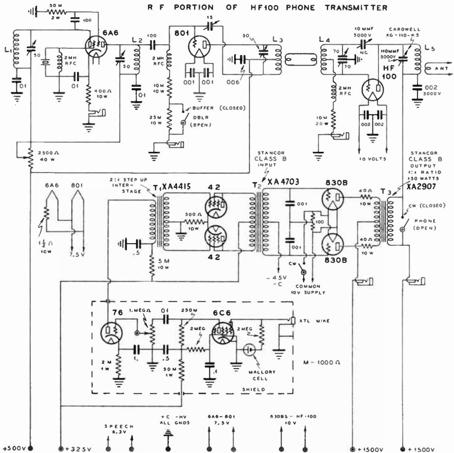
**Figure 11—Speech Amplifier and Modulator for 175-Watt Class C R.F. Amplifier.**
