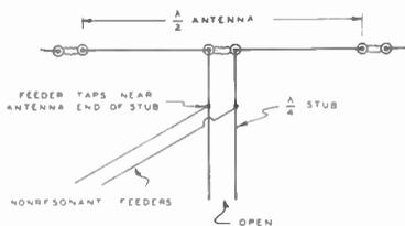
**Figure 20—Center-Fed Half-Wave Antenna with Stub Line Cut to Exact Length Without Shorting Bar.**
