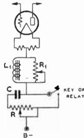
Straight center-tap keying as shown in figure 35 never should be used, because this circuit produces extremely bad key clicks. The key click filter in figure 34 always can be connected into the center-tap lead as an external unit. A more effective key click filter for the center-tap lead is made possible through the use of vacuum tubes. A simple vacuum tube keying circuit is shown in figure 36.
