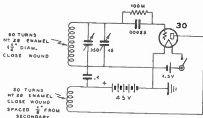
**Figure 23—Calibration Oscillator for Battery Operation.**
