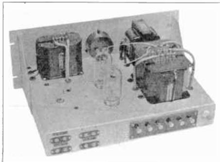
Figure 25—The 35-T class B modulator unit.
