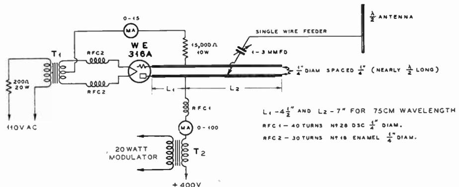
Figure 15—W.E.-316A  $\frac{3}{4}$ -Meter Oscillator Circuit.
