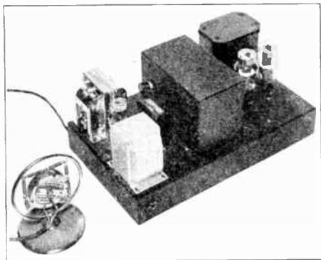
**Figure 8—Speech channel, power supply and modulator for the 160 meter phone transmitter. It delivers 35 watts of audio power, sufficient to modulate over 70 watts input to the parallel 210 final amplifier.**
