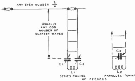
Figure 15—Zepp. Antenna System and Feeder Tuning.
