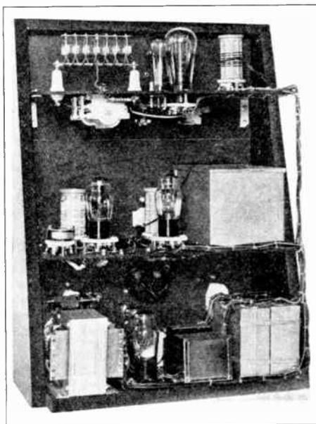
**Figure 3—The continued popularity of the type 10 tube prompted the design of this grid-modulated transmitter. It will deliver a 30-35 watt carrier on phone, more on c.w. on the lower frequency bands.**
