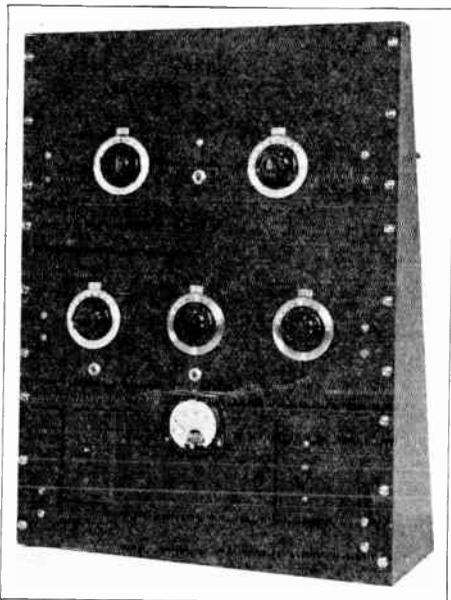
**Figure 2**—Front view of the inexpensive grid-modulated radiotelephone transmitter. It uses wall type on-off switches to control the power supplies. The Masonite panels are mounted on a wood rack. The two end pieces are ripped from one board by means of a single diagonal cut. Crackle paint gives both rack and panels the appearance of metal.
