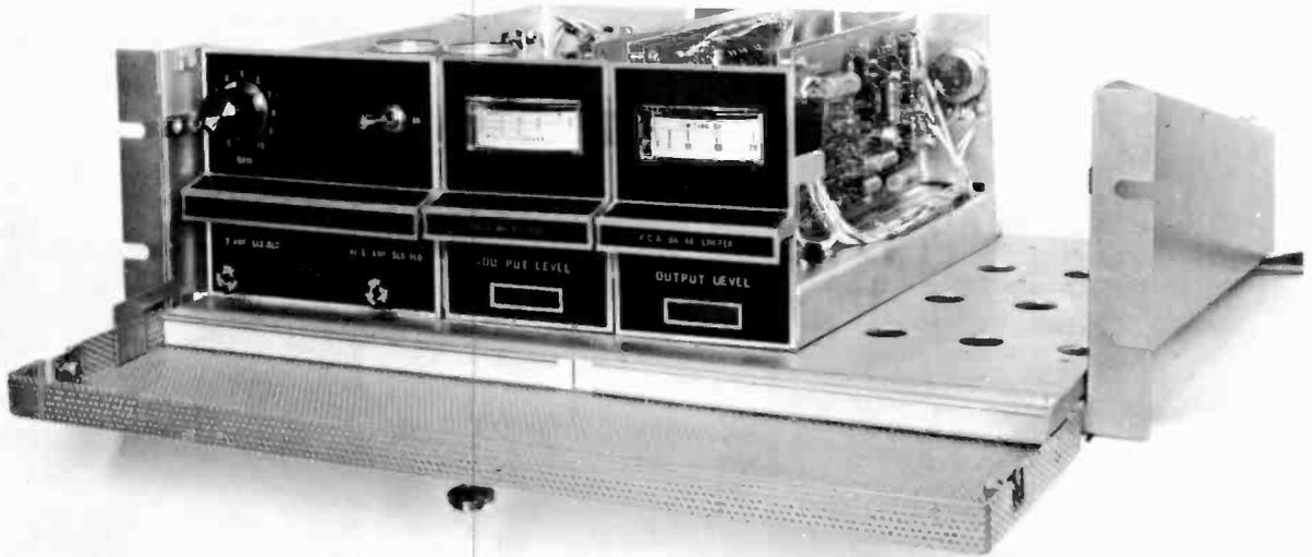
Fig. 10-13. Program amplifier shown with AGC and limiter units in a rack-mounting shelf.
