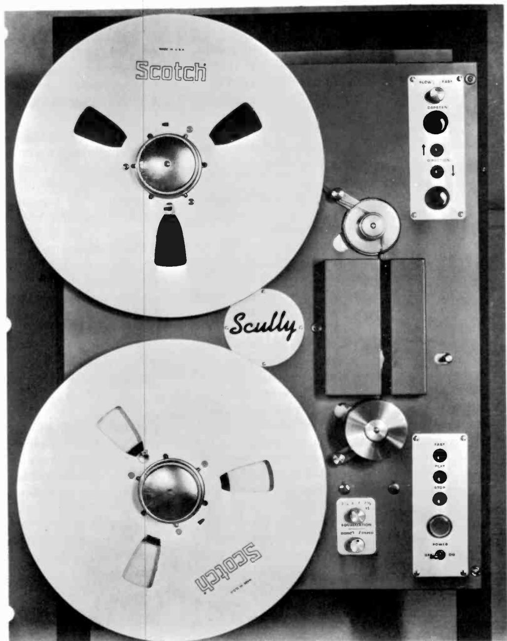
Fig. 11-7. Reel-to-reel mono or stereo tape playback unit.
