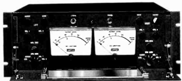
Fig. 10-15. Dual peak-limiting amplifier designed for stereo or dual monaural operation.
