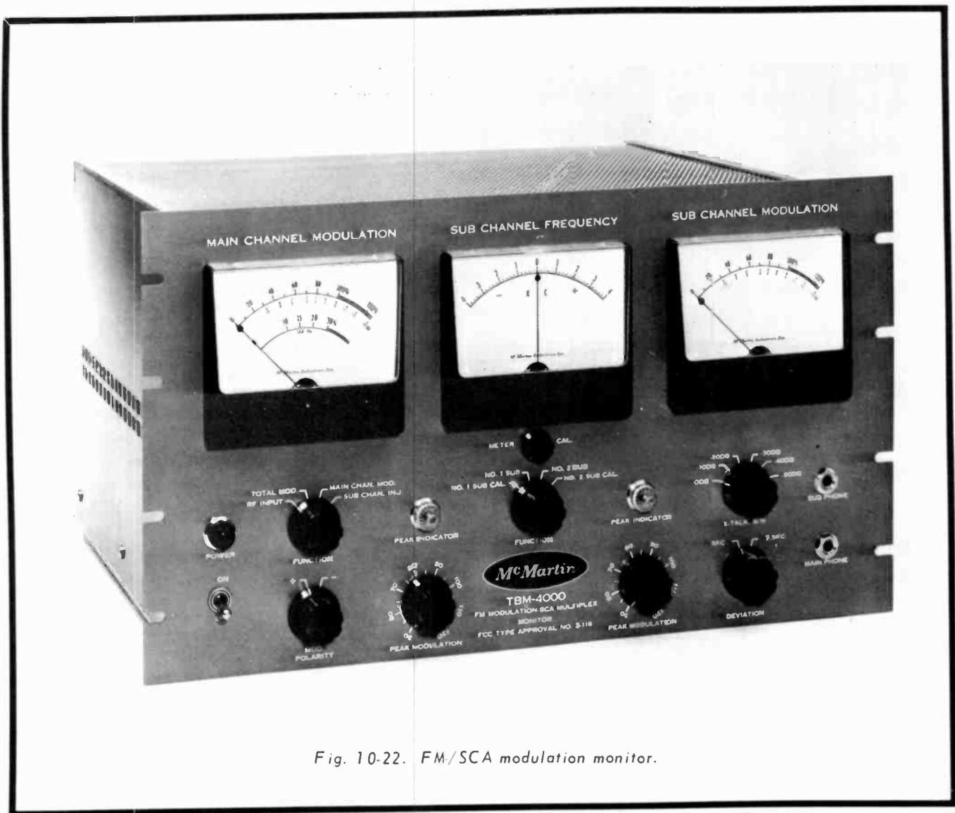
Fig. 10-22. FM/SCA modulation monitor.
