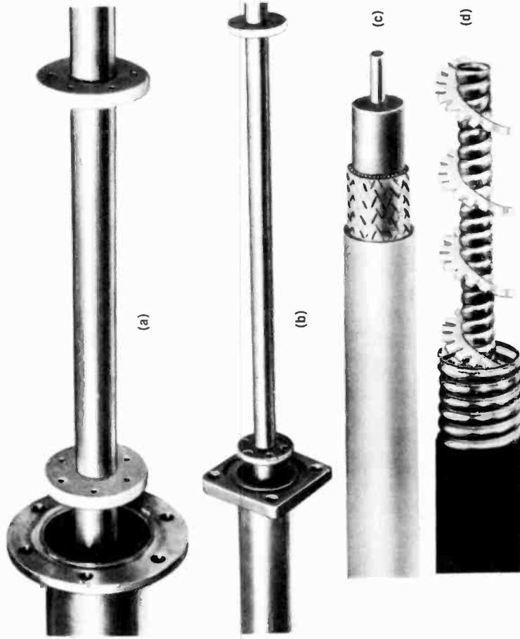
Fig. 8-15. Types of transmission line: Rigid 3 1/8-inch copper (a), rigid 1 5/8-inch copper (b), flexible RG cable (c) and flexible Heliac cable (d).
