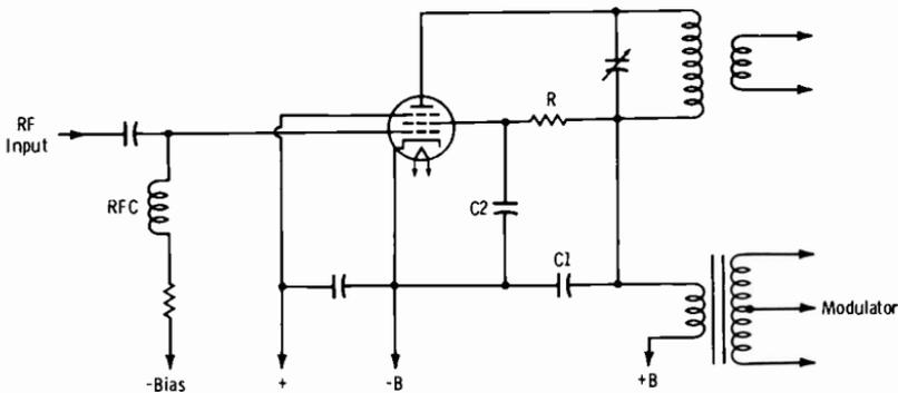
Fig. 9-28. Plate-screen modulation of rf pentode.
