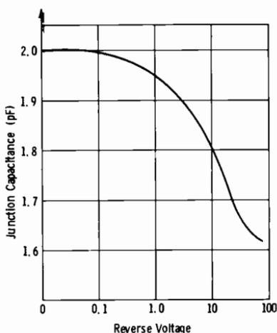
(A) Typical small-signal diode.
