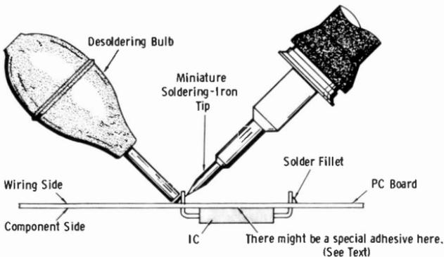
**Fig. 13-14. Method for desoldering components.**
