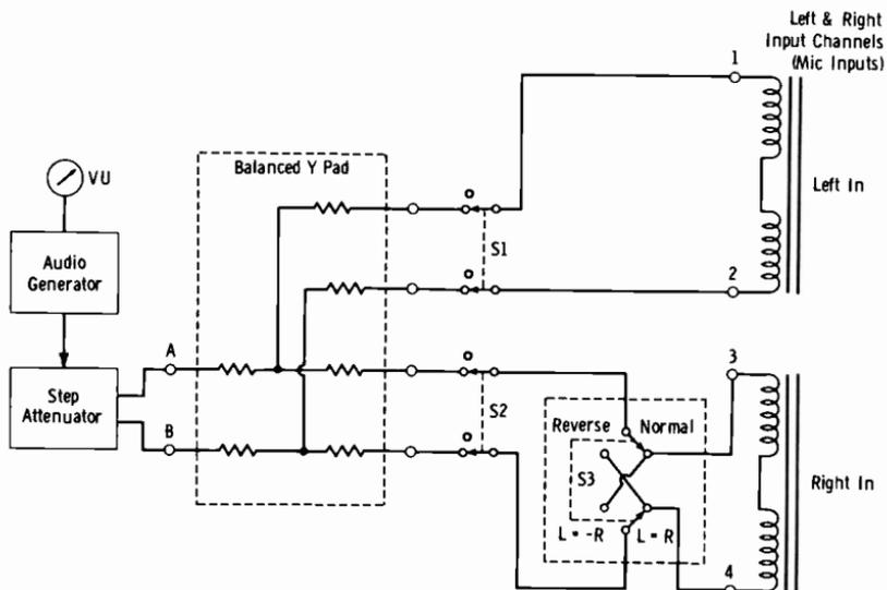
Fig. 14-26. Studio setup for stereo measurements.
