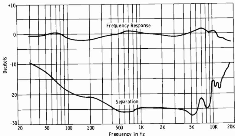
**Fig. 13-6. Typical frequency response and channel separation of GE VR-22 series cartridge.**
