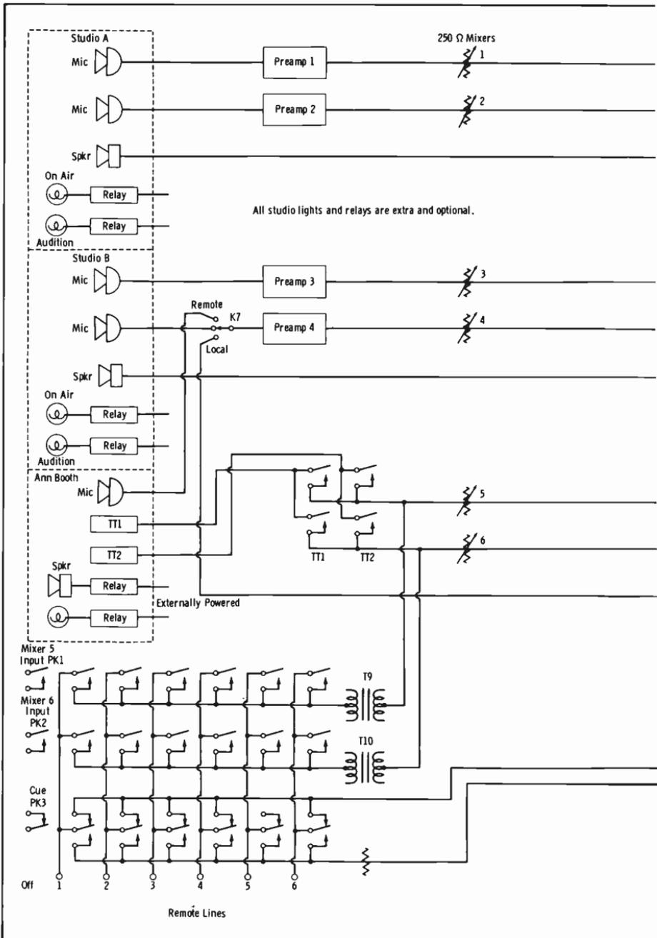
Fig. 11-36. Block diagram
