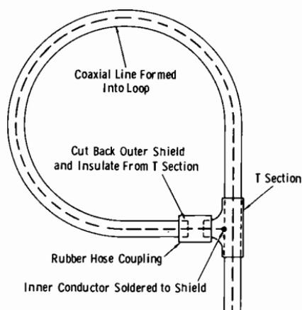
Fig. 9-18. A nonresonant pickup loop.
