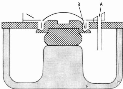
**Fig. 4-7. Means of damping (A) and compensation for mass reactance (B) at high frequencies.**
