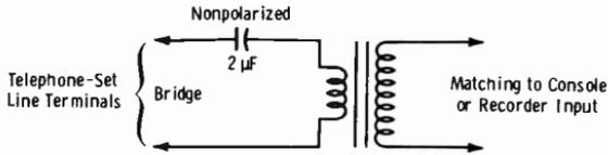
**Fig. 8-17. Direct connection to telephone-set line terminals.**
