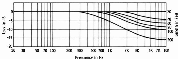
Fig. 4-2. Signal loss versus cable length (high-impedance input).
