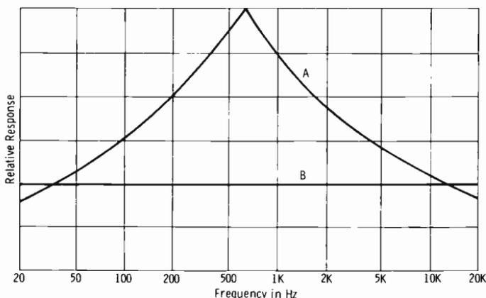
**Fig. 4-6. Dynamic-microphone response curves.**
