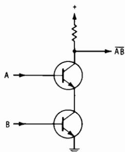
Fig. 3-37. Direct-coupled-transistor-logic NAND circuit.
