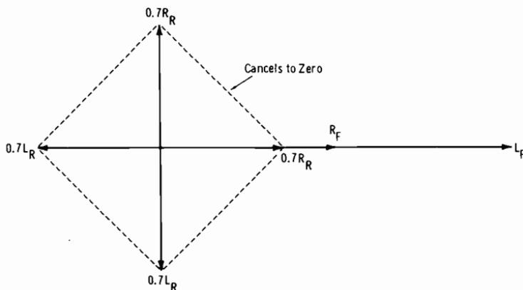
**Fig. 7-9. Encoder output when  $L_F = R_F = L_R = R_R$ .**
