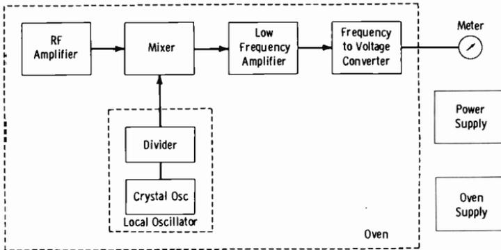
Fig. 9-40. Metron Model 510 analog a-m frequency monitor.
