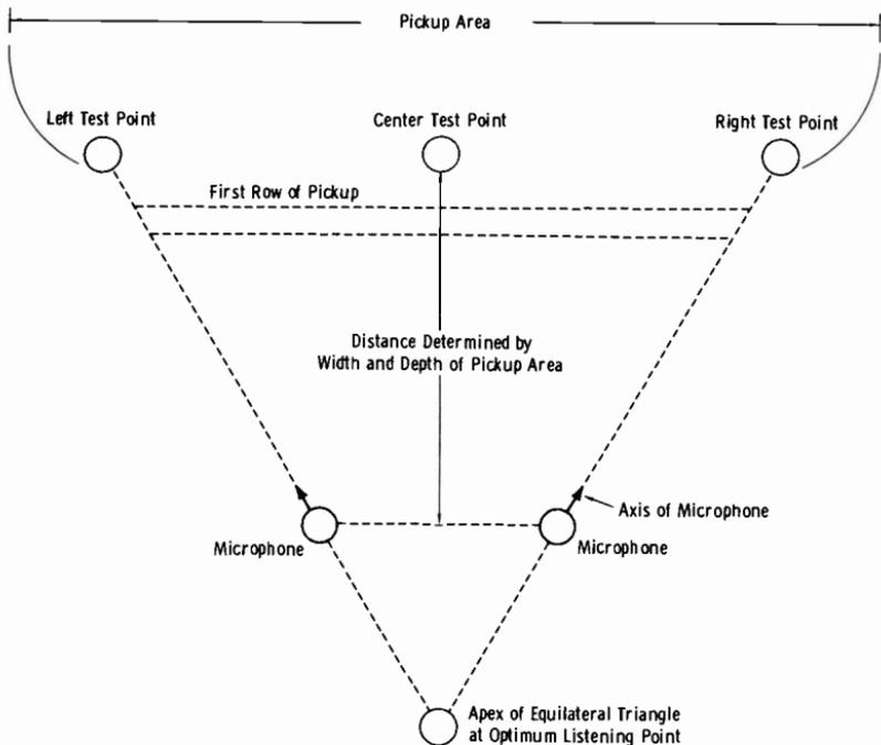
Fig. 11-29. Basic arrangement for stereo pickup.
