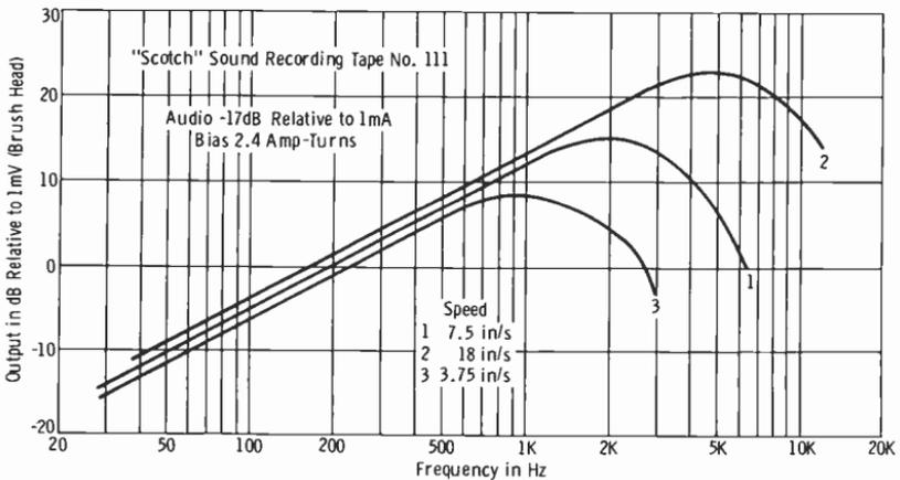
Fig. 4-30. Effect of tape speed on frequency response.
