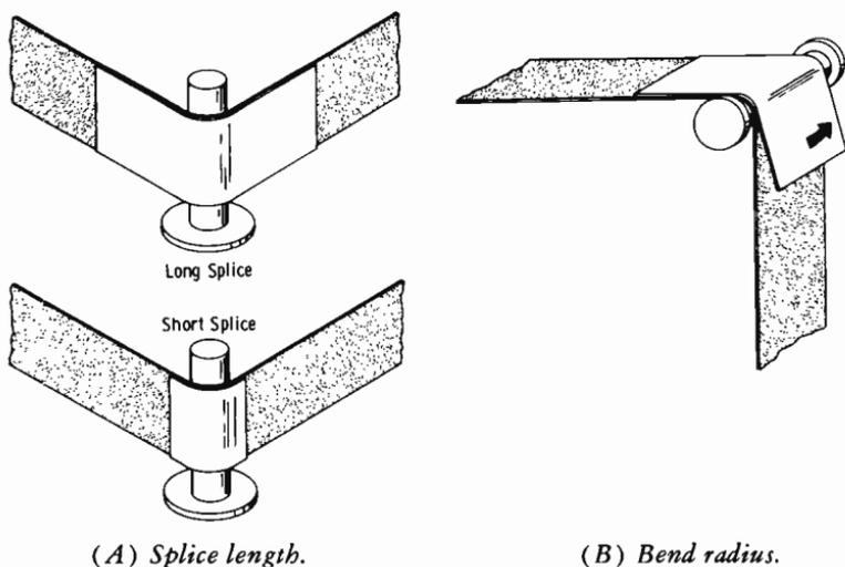
Fig. 13-24. Splice length and bend radius.
