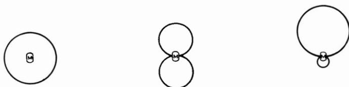
(A) *Nondirectional.*      (B) *Bidirectional*      (C) *Unidirectional.*
