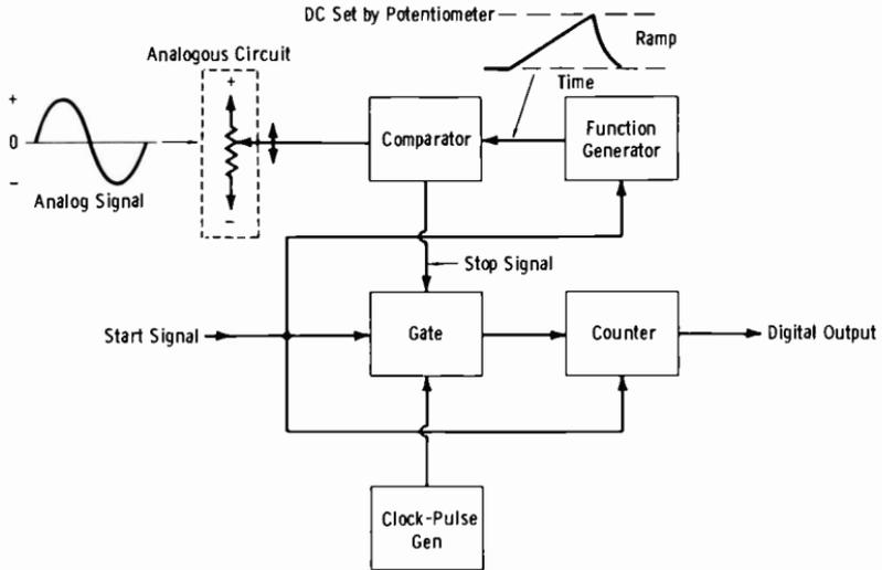
Fig. 3-59. Comparison method of analog-to-digital conversion.
