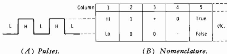
Fig. 3-41. Pulse nomenclature for logic systems.
