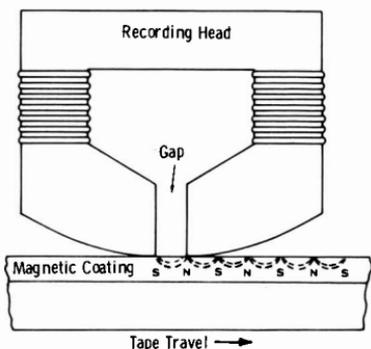
(A) Magnetizing action of recording head.
