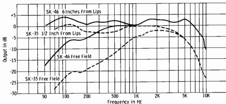
Fig. 4-10. Frequency response of SK-35 and SK-46 microphones.
