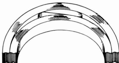
Care must be taken not to raise the reel too high, because this creates too much downward pressure on the tape edge after the lid has been fastened in place. Before the lid is fastened in place, put the cartridge in a tape player that has its head cover removed to allow the lid to be secured in place while the reel is in motion. Observe the reel motion carefully to make sure that while the lid is being secured no binding is produced between the wire guides and the edge of the tape.
