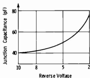
(B) Variable-capacitance diode.
