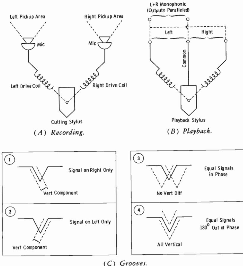
Fig. 4-22. Principles of stereo disc recording.
