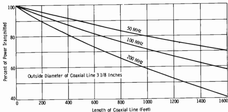
transmitted by coaxial cables.
