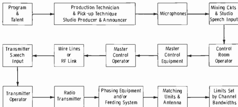
Fig. 6-1. Links in the chain involved in putting a program on the air.
