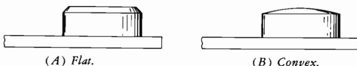
Fig. 14-36. Relay-contact shapes.
