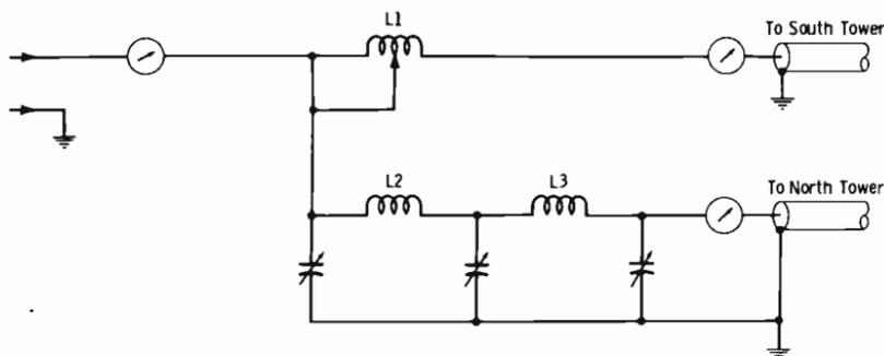
(C) Equivalent circuit for directional operation.
