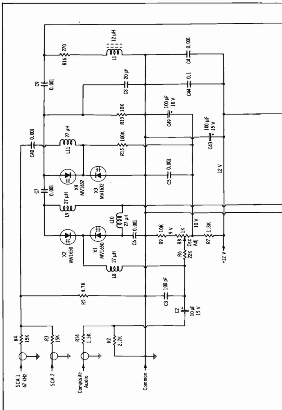
Fig. 10-36. Modulated oscillator
