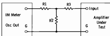
(B) Meter connected through isolating and matching pad.
