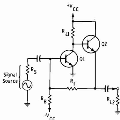
Fig. 3-4. Diagram of a feedback pair.
