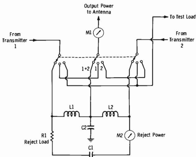
Fig. 9-38. Simplified diagram of combiner network.
