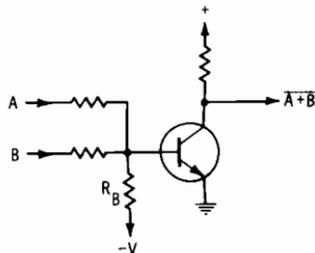
Fig. 3-40. Resistor-transistor-logic NOR circuit.
