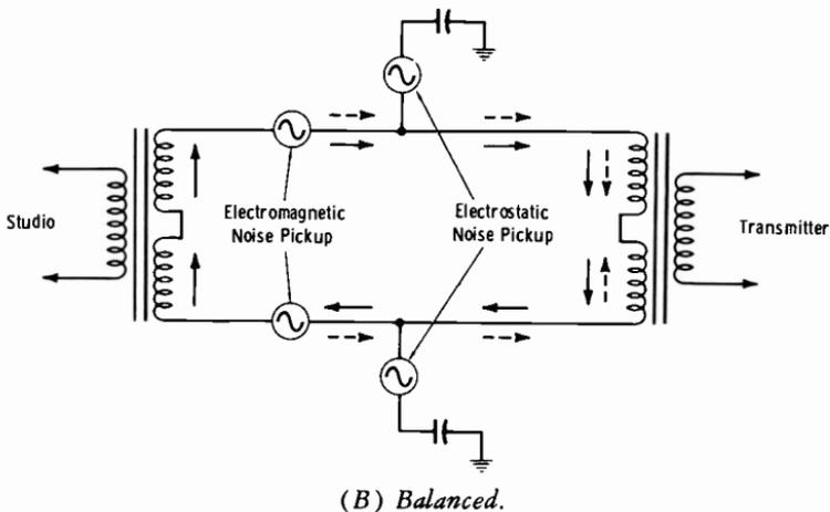
**Fig. 12-2. Remote telephone lines.**
