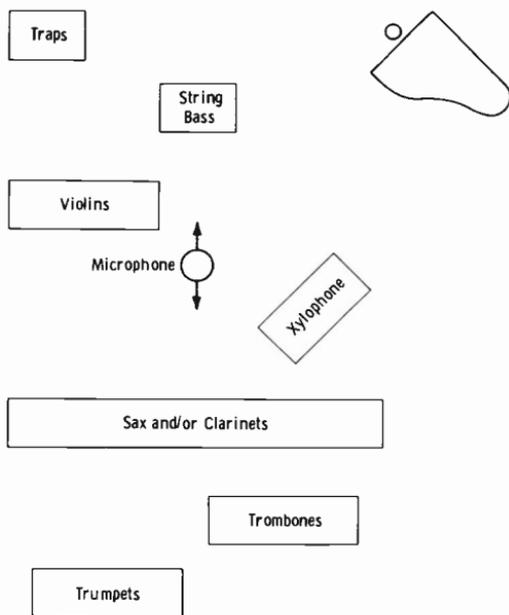
**Fig. 11-18. Small-orchestra pickup with bidirectional microphone.**
