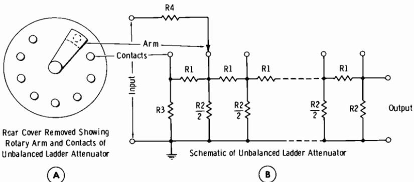
Fig. 6-10. Principles of unbalanced ladder attenuator.
