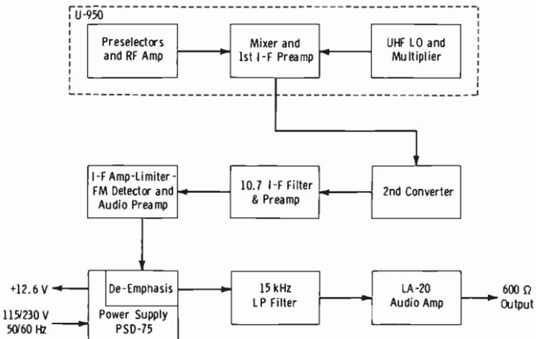
Fig. 8-26. Block diagram of stl receiver.
