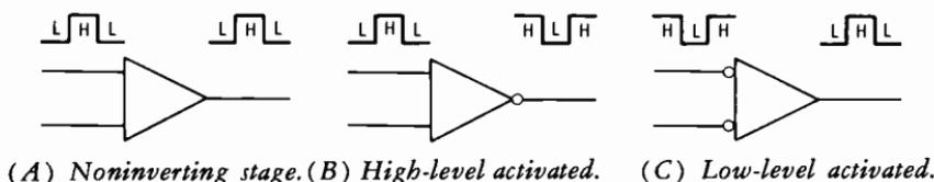
Fig. 3-44. Inversion in logic stages.
