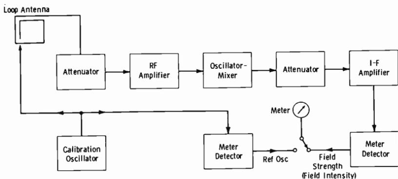
**Fig. 14-9. Block diagram of a field-strength meter.**
