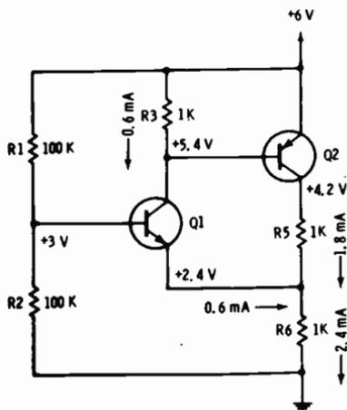
Fig. B-1. Dc equivalent of Fig. 3-69.
