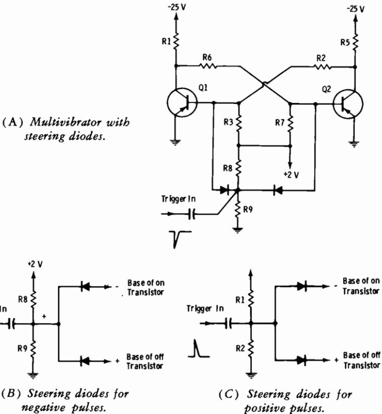
Fig. 3-61. Fundamentals of pulse steering.
