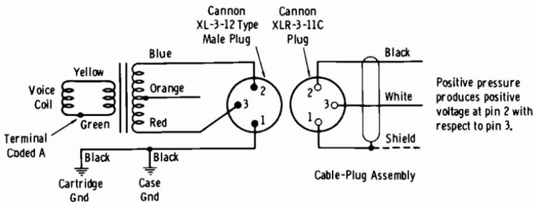
(B) *Shure Model SM 58.***Fig. 7-6. Examples of microphone wiring.**
