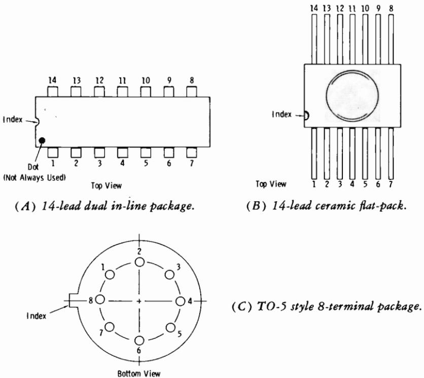
**Fig. 13-12. Basic integrated-circuit packages and terminal arrangements.**
