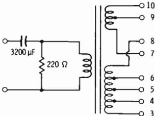
**Fig. 6-46. Typical monitor-amplifier output transformer.**
