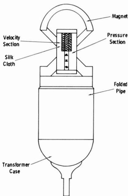
**Fig. 4-16. Unidirectional microphone.**
