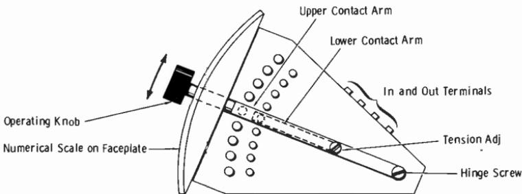
Fig. 6-16. Side view of typical vertical attenuator.
