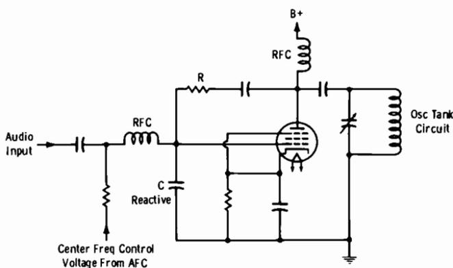
(A) *Simulated variable inductance.*
