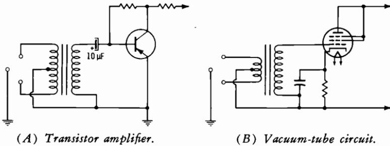
Fig. 4-3. Microphone input circuits.
