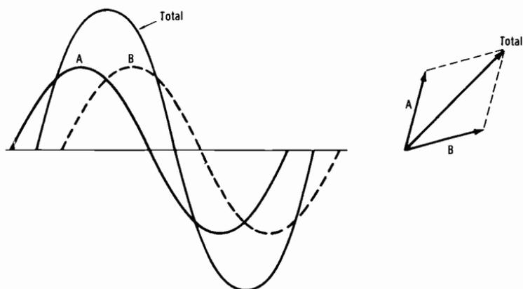
(A) *Small phase difference.*
