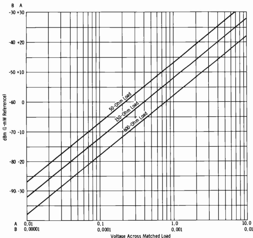
Fig. 2-12. Relationship of dBm and load voltage.
