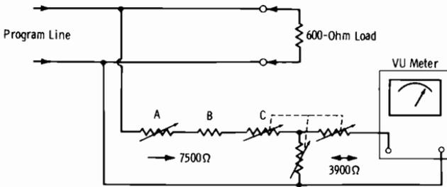
Fig. 2-13. External circuit of standard VU meter.
