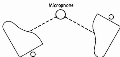
the microphone. The temperament of the pianists must, of course, be considered and the lead piano given prominence by moving the microphone closer to that piano if the accompanist is "heavier fisted." The above procedure for bass and treble balance must be followed by moving not the microphone, but the piano itself.
