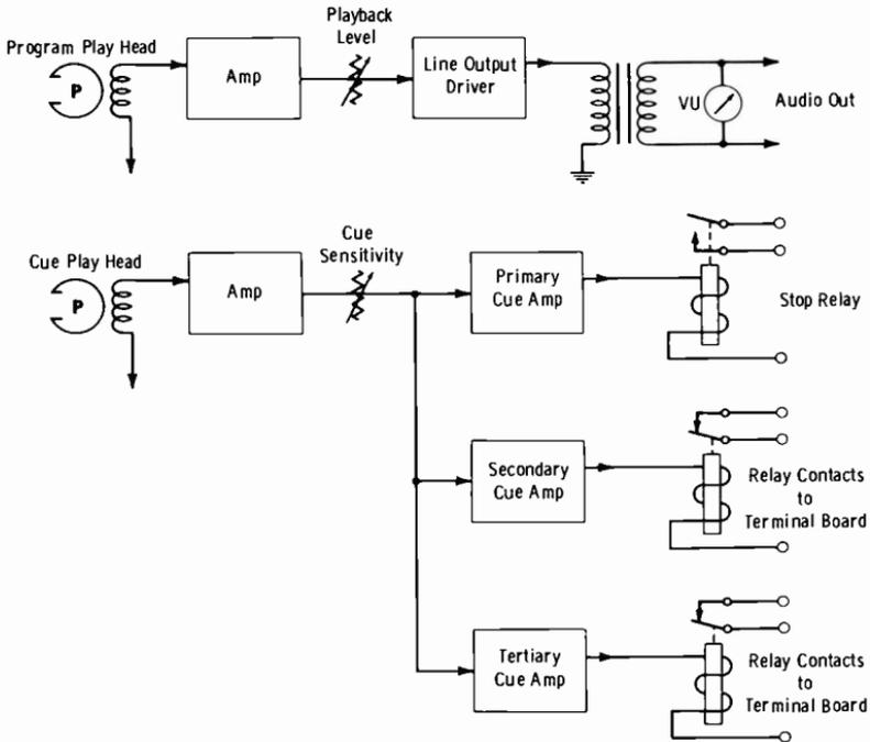
Fig. 5-12. Typical playback electronics in tape cartridge system.
