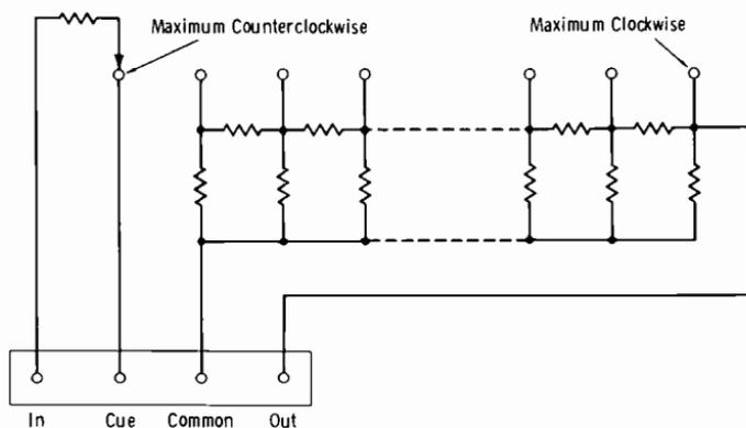
Fig. 6-11. Unbalanced ladder attenuator with cueing position.
