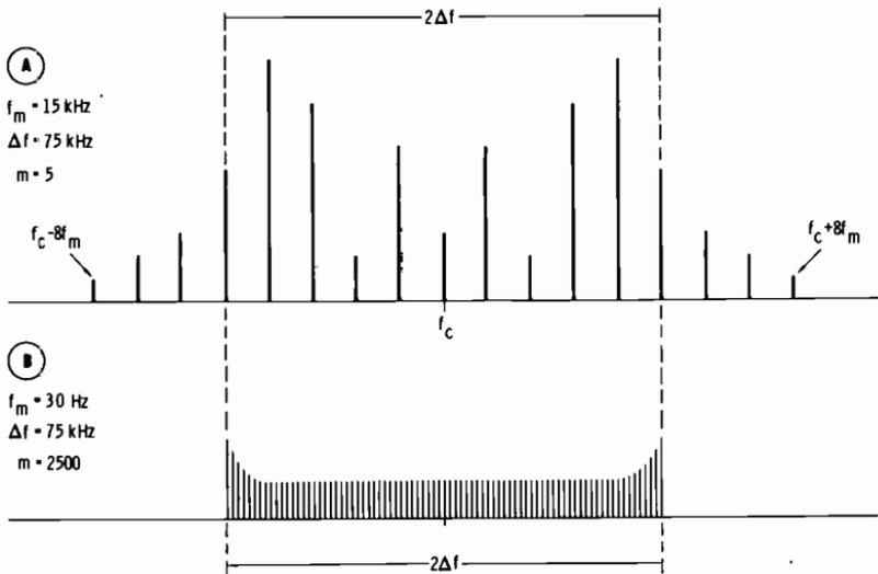
Fig. 10-14. Spectrum analysis of fm signals.
