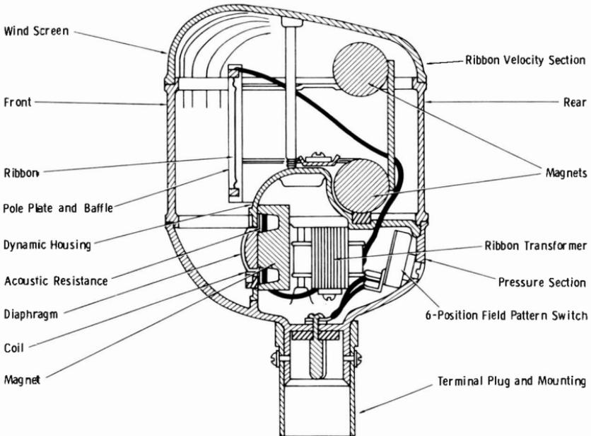
**Fig. 4-14. Construction of cardioid microphone.**
