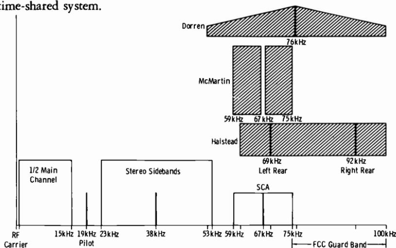
Fig. 7-22. Three proposed carrier multiplexing systems.
