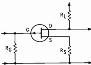
(B) *P-channel.***Fig. 3-15. Amplifier circuits using FETs.**
