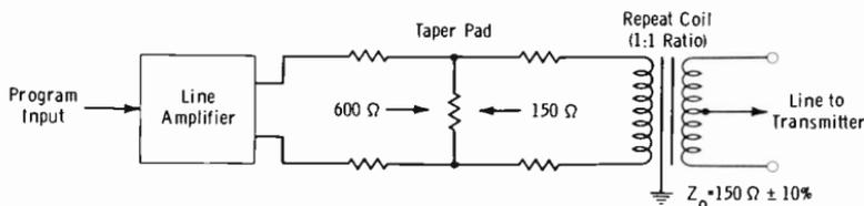
Fig. 6-5. Use of taper pad for feeding 150-ohm line from 600-ohm source.
