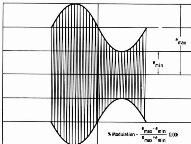
**Fig. 9-34. Measurement of percent modulation.**
