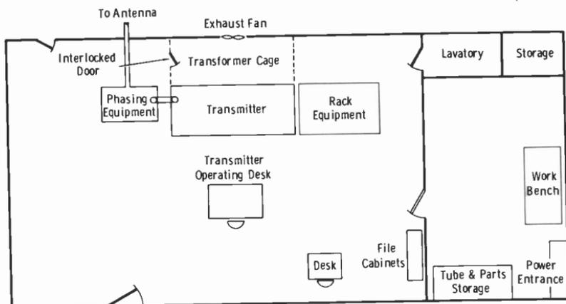
**Fig. 1-4. Example of transmitter equipment layout.**
