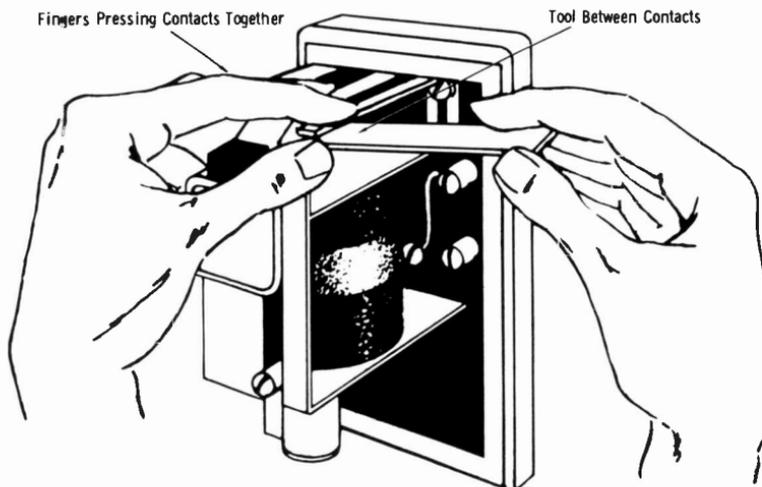
**Fig. 14-35.** Method of cleaning hard-alloy relay contacts.
