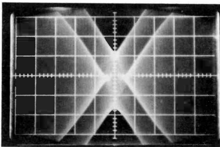
(B) Time base of  $50 \mu\text{s}/\text{cm}$ , correct phase.
