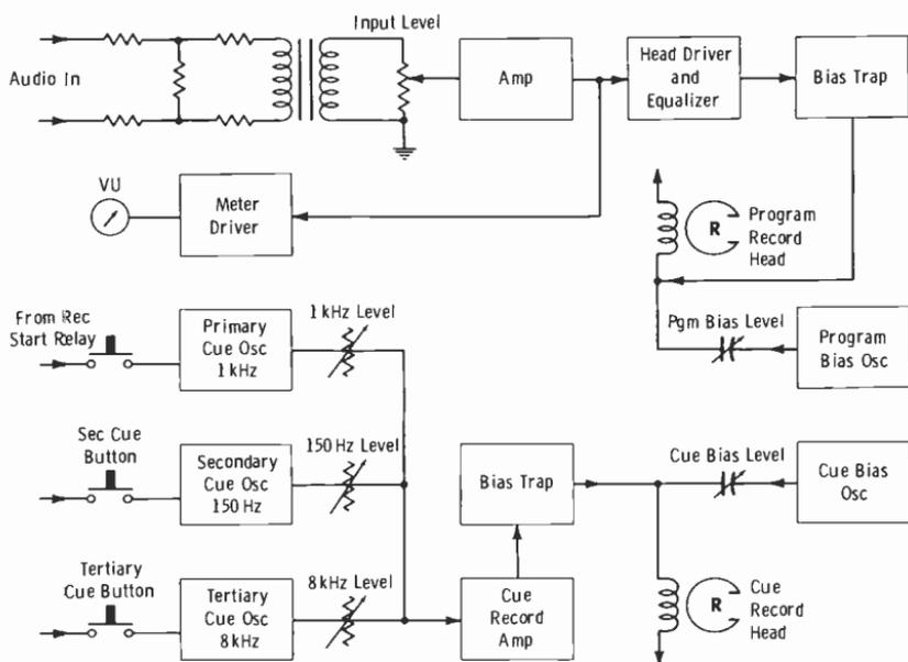
Fig. 5-11. Typical recording electronics of tape cartridge system.
