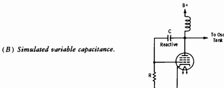
(B) *Simulated variable capacitance.***Fig. 10-17. Fundamental reactance-tube circuits.**
