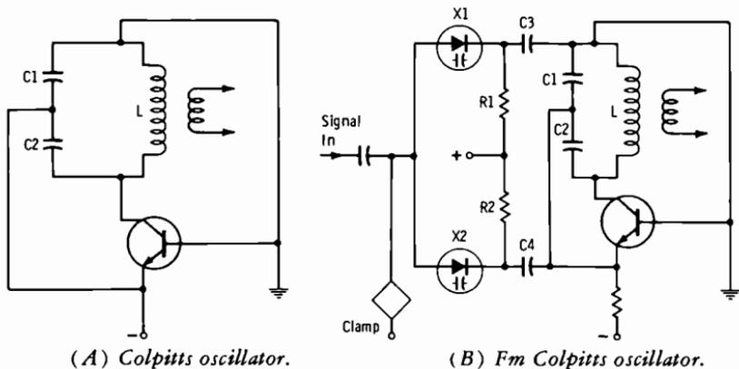
Fig. 10-21. Use of voltage-variable-capacitance diodes for direct fm.
