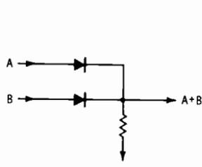
Fig. 3-35. Diode-logic OR circuit.
