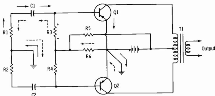
(A) *Input resistors.*
