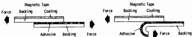
(A) *Shear adhesion (creep).*
