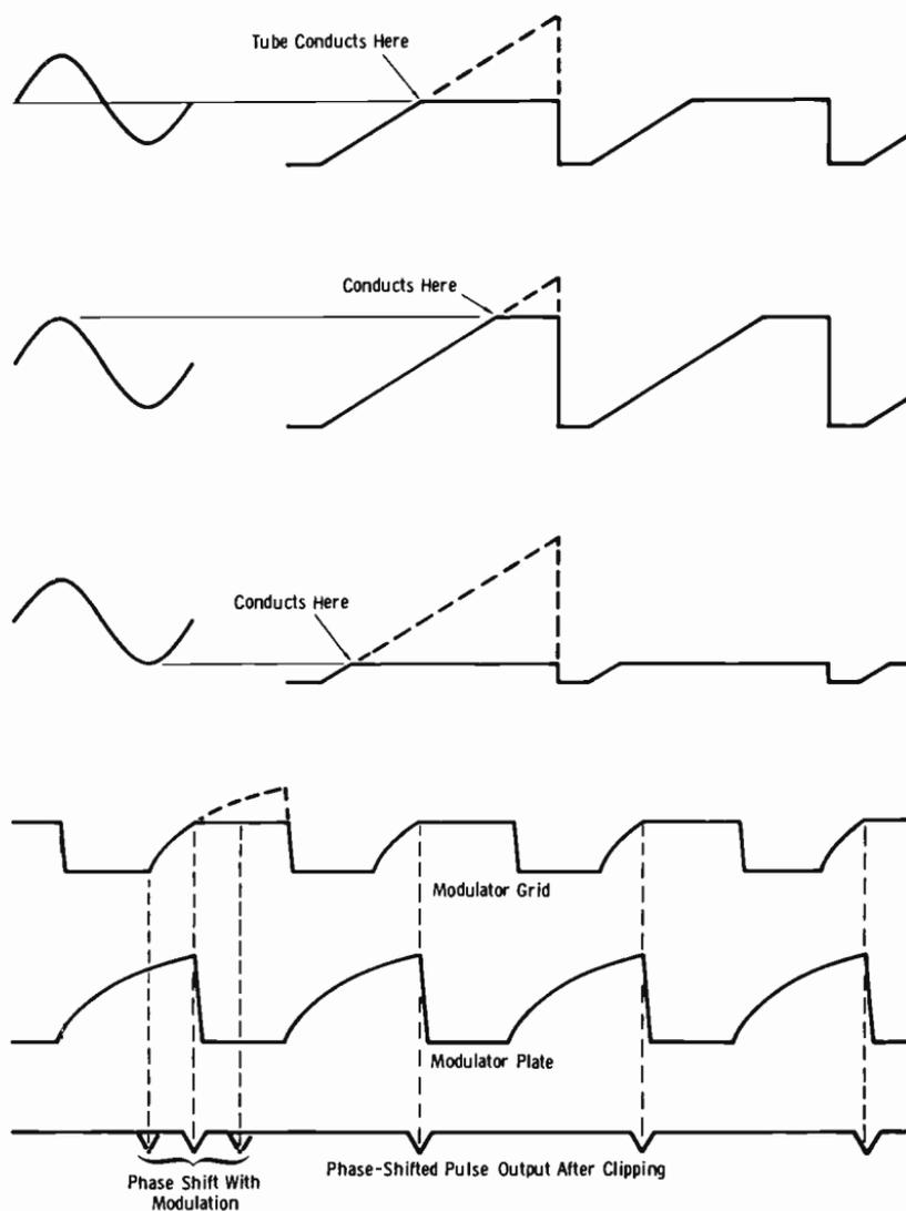
**Fig. 10-16. Modulated sawtooth waveforms.**
