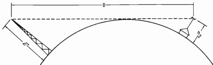
Fig. 10-2. Calculation of line-of-sight distance.
