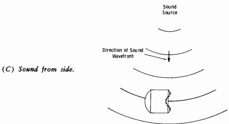
**Fig. 4-11. Action of pressure microphone.**
