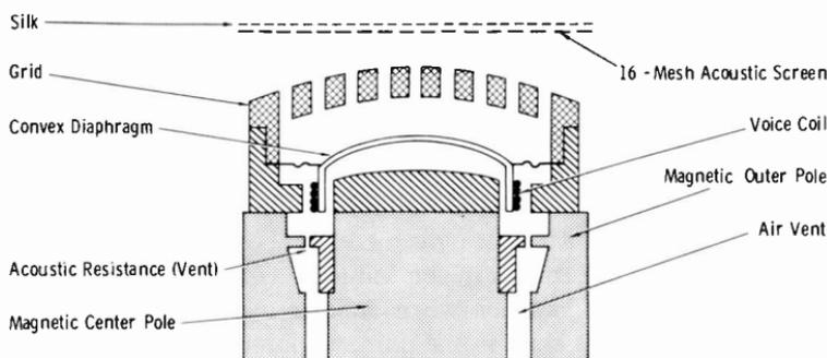
Fig. 4-5. Basic diagram of moving-coil microphone.
