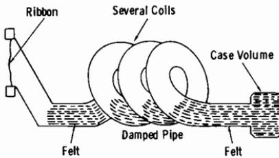
**Fig. 4-15. Infinite impedance for producing unidirectional characteristics.**
