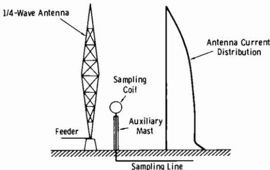
(B) Coil mounted on auxiliary mast.
