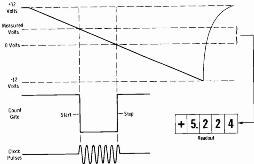
Fig. 3-22. Time-to-voltage conversion for digital voltmeter readout.
