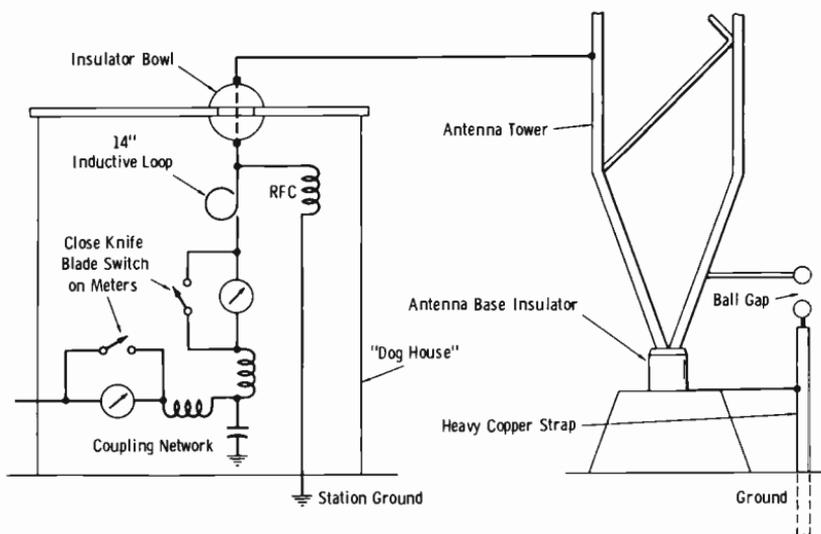
Fig. 9-14. Lightning protection for a-m tower.
