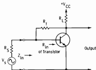
$$A_i = \frac{R_f}{R_L} \quad (\text{Eq. 3-15})$$
