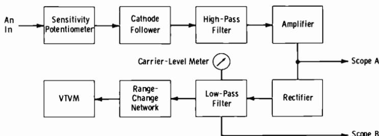
(B) *Analyzer section.*
