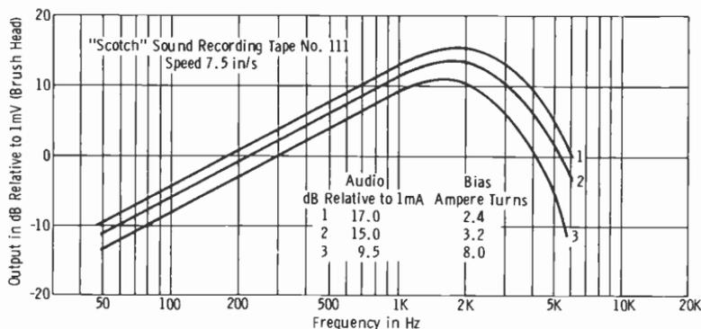
Fig. 4-29. Effect of bias on frequency response.
