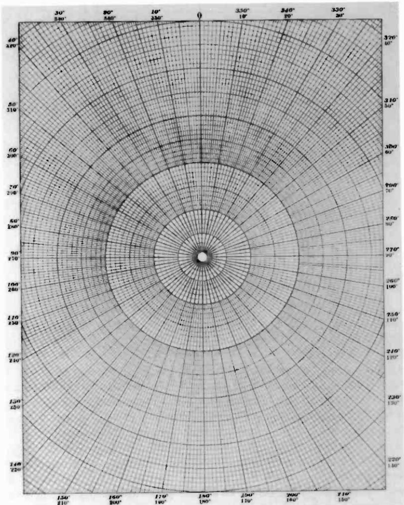
Fig. 2-21. Example of polar-coordinate paper.
