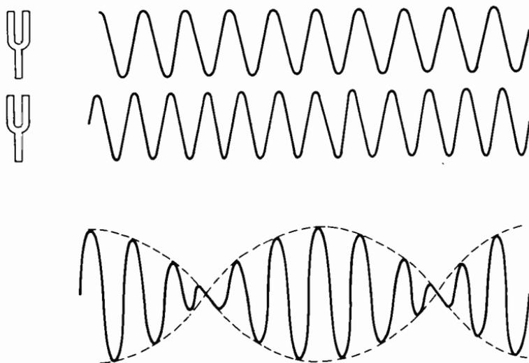
Fig. 11-3. Beat note produced from two fundamental frequencies.
