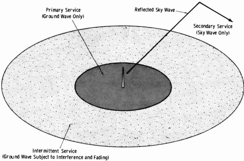
**Fig. 9-5. Service areas of an a-m broadcast station.**
