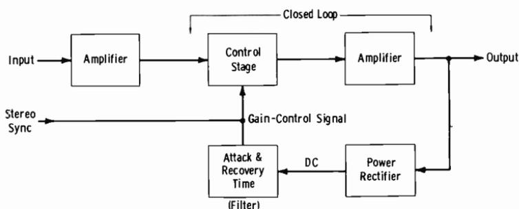
(A) *Limiter amplifier.*
