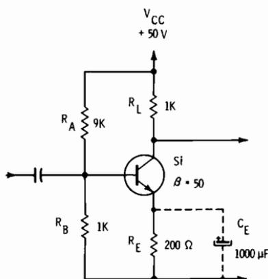
Since the emitter voltage is +4.4 volts, the emitter current (from Ohm's law) must be:
