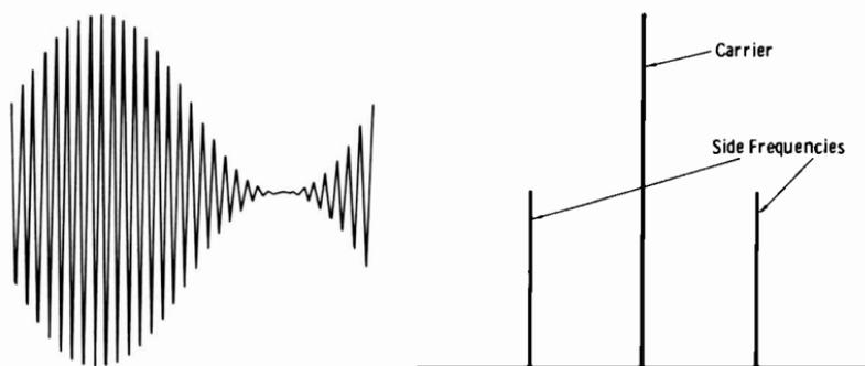
(A) *Modulated 100%.*
