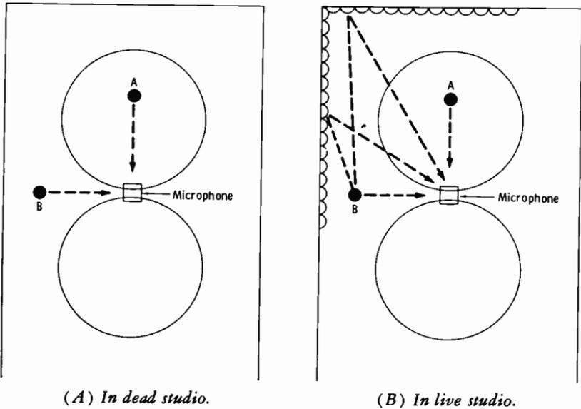
**Fig. 11-10. Response patterns for a bidirectional microphone.**
