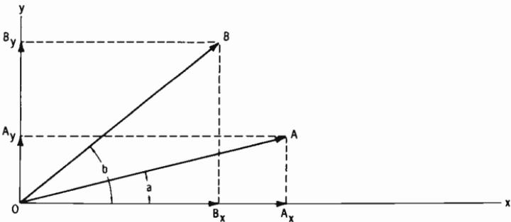
(B) Components along x and y axes.
