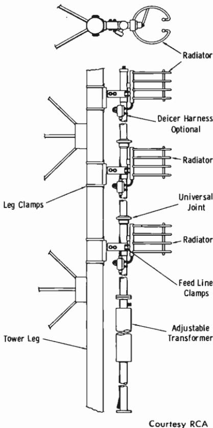
**Fig. 10-4. Three-bay fm antenna side-mounted on tower.**
