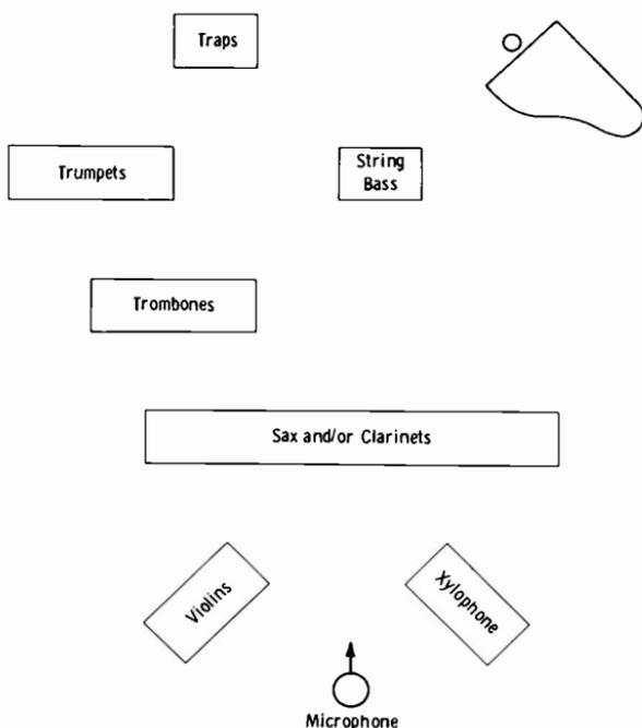
**Fig. 11-17. Arrangement for small-orchestra pickup.**
