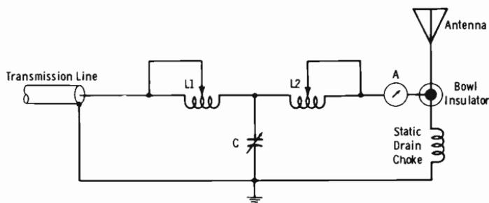
Fig. 9-13. Single-antenna tuning unit.
