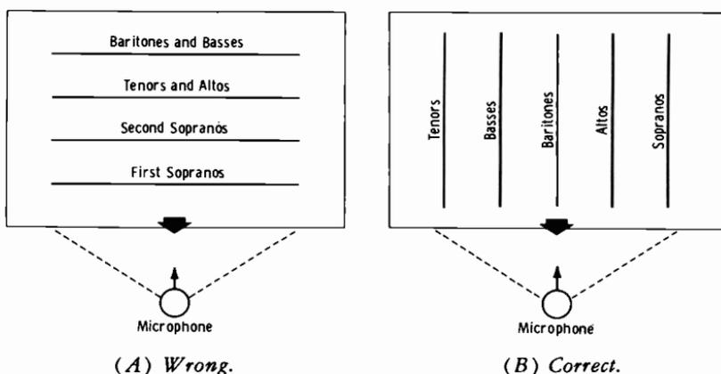
Fig. 11-21. Arrangement for choral pickups.
