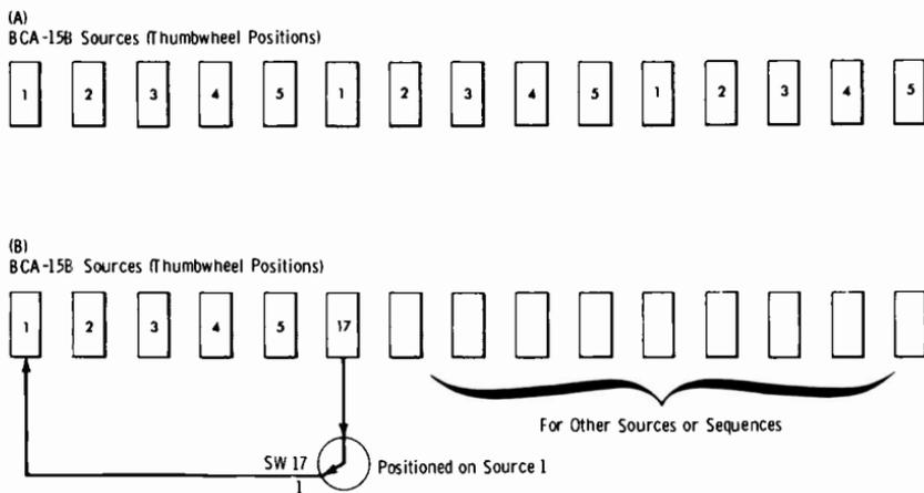
Both A and B continue to repeat a 5-source sequence, but 20-position recycling switch in B uses only six thumbwheel positions.
