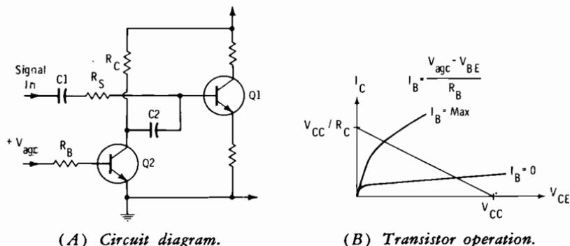
Fig. 6-41. Variable impedance with transistor.
