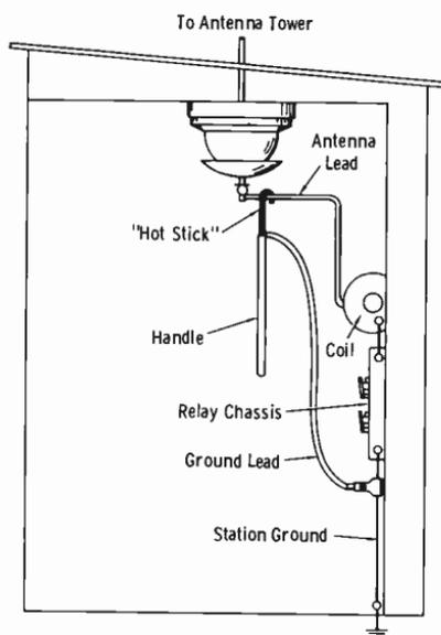
**Fig. 14-37. Safety device for grounding high-voltage points.**
