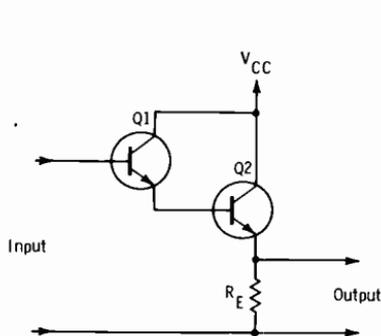
**Fig. 3-11. Darlington circuit.**
