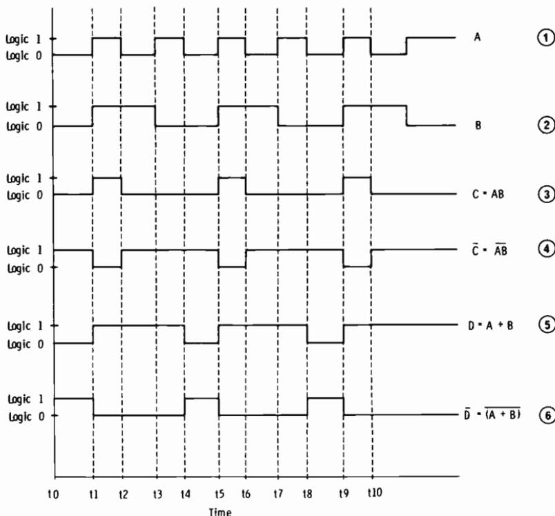
**Fig. 13-11. Timing diagram.**
