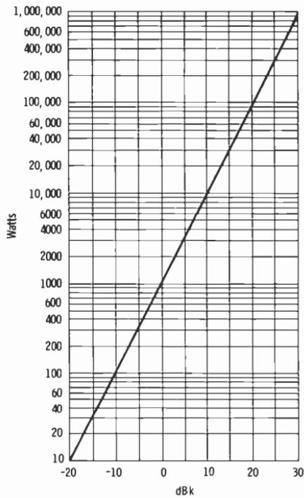
mission-line attenuation, and antenna gain. For example, assume that the transmitter power output is 10 kW, the transmission-line efficiency (for type, frequency, and length of line required) is 79 percent, and the antenna power gain is 3.2. Note that if the conventional computation of erp is made, it is necessary to take 79 percent of 10,000 and then multiply by 3.2 to obtain the erp (25,280 watts). However, the computation can be carried out as follows:
