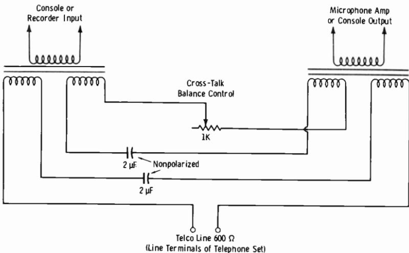
**Fig. 8-18. Hybrid circuit for two-way communication.**
