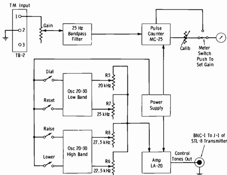
Fig. 8-29. Block diagram of remote-control studio unit.
