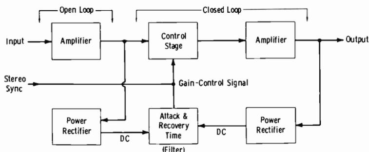
(B) *Agc amplifier.***Fig. 6-37. Audio level-control devices.**
