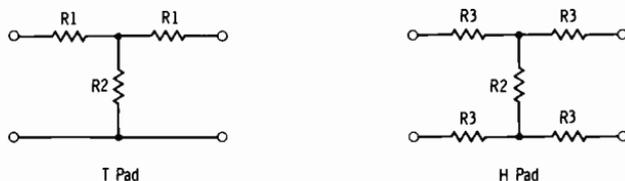
For case where  $Z_{in} = Z_{out} = 600$  ohms. For other than 600 ohms (but equal impedances), multiply all resistance values by factor  $Z_x/600$  (0.40 for 250 ohms, 0.25 for 150 ohms, 0.083 for 50 ohms).
