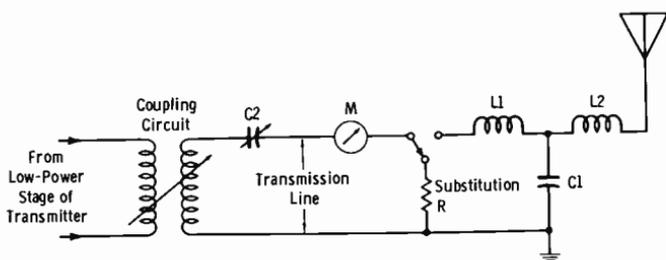
Fig. 14-7. Substitution method for adjusting antenna system.
