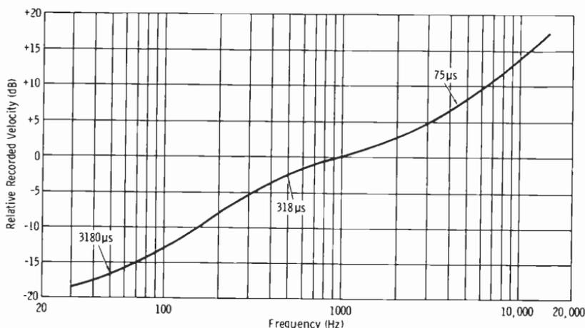
Fig. 6-31. EIA standard lateral disc-recording characteristic.
