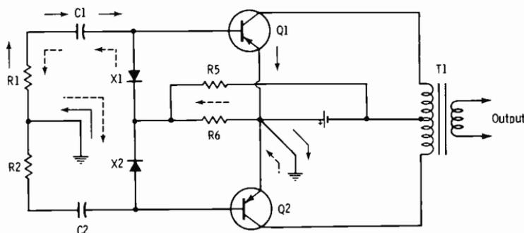
(B) *Input diodes.***Fig. 3-19. Class-B amplifier with RC input coupling.**
