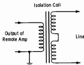
Fig. 12-3. Isolation-coil circuit.
