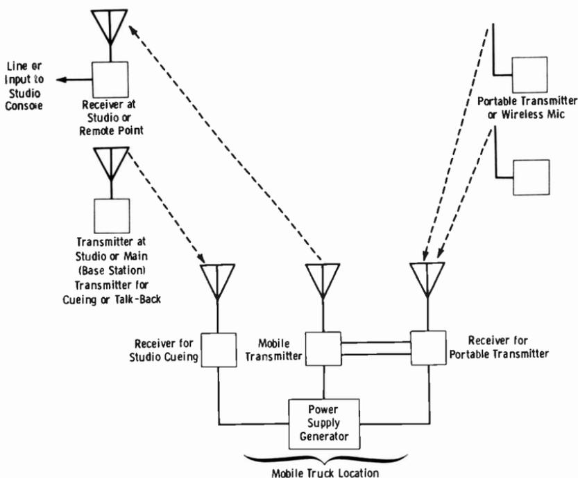
**Fig. 8-10. Block diagram of remote-relay system.**
