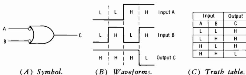
Fig. 3-45. OR gate with phase inversion.
