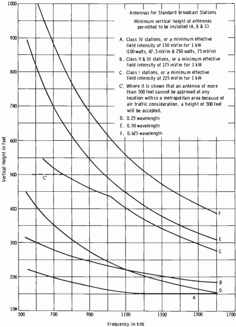
**Fig. 9-8. FCC antenna requirements for a-m stations.**
