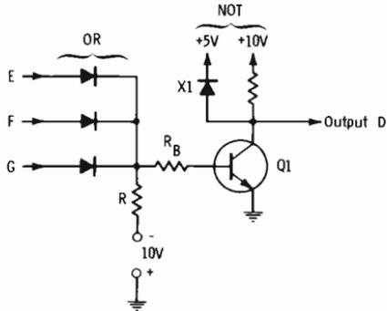
**Fig. 3-52. Logic circuits for transmitter high voltage.**
