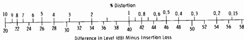
Fig. 13-18. Chart for converting decibels to percent distortion.
