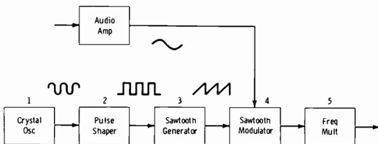
Fig. 10-15. Block diagram of pm exciter.
