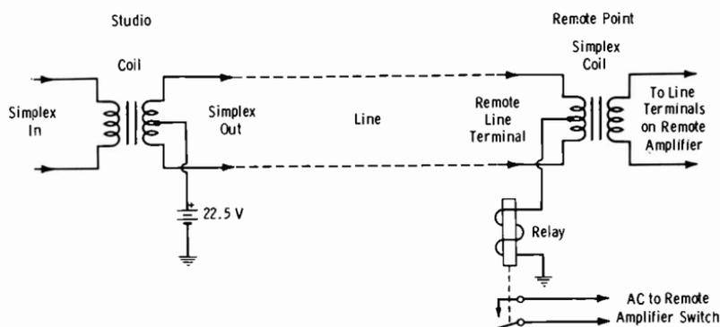
Fig. 8-14. Simplex circuit for control of remote amplifier.
