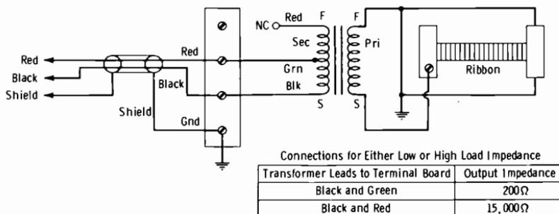
Fig. 13-2. Schematic diagram of a typical microphone.
