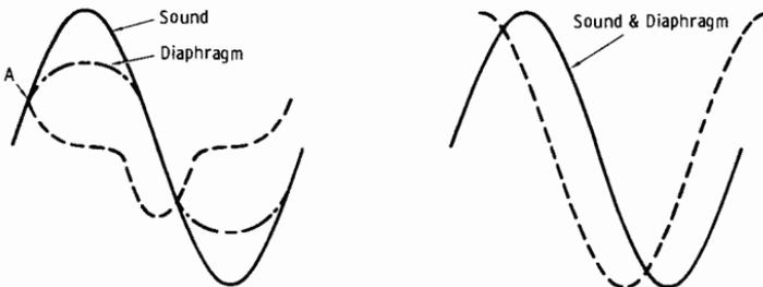
(A) Action under excessive pressure. (B) Action with normal loading.
