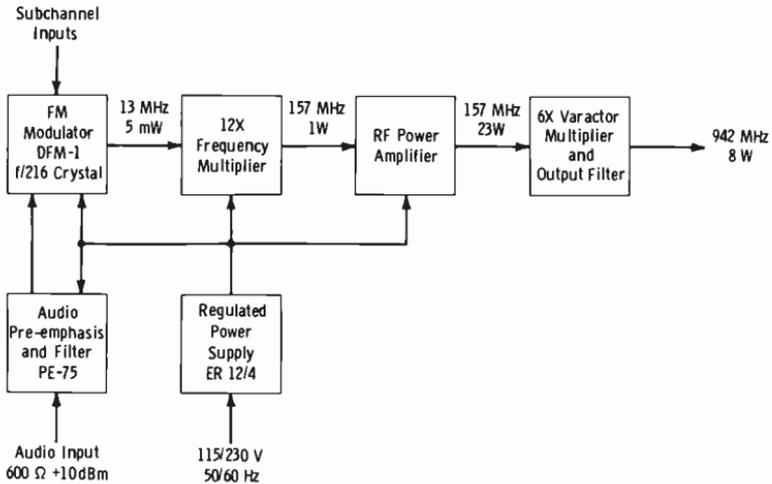
Fig. 8-25. Block diagram of stl transmitter.
