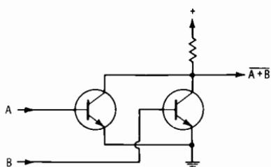
Fig. 3-38. Direct-coupled-transistor-logic NOR circuit.
