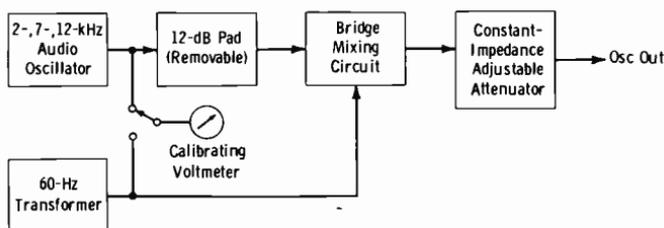
(A) *Signal-generating section.*
