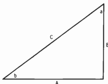
Fig. 2-6. Terminology applicable to trigonometric functions.
