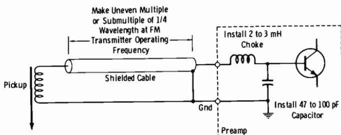
**Fig. 13-8. Precautions to minimize fm-to-am rectification in vicinity of strong rf field from transmitter.**
