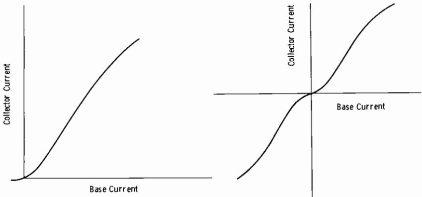
(B) Single transfer characteristic. (C) Combined transfer characteristic.
