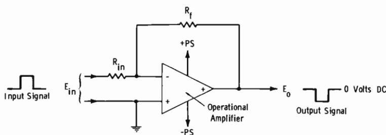
(A) *Inverting input referenced to ground.*
