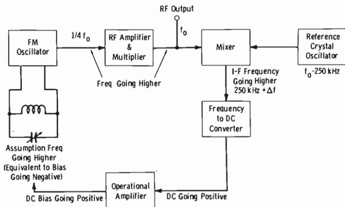
(B) Block diagram of afc loop.
