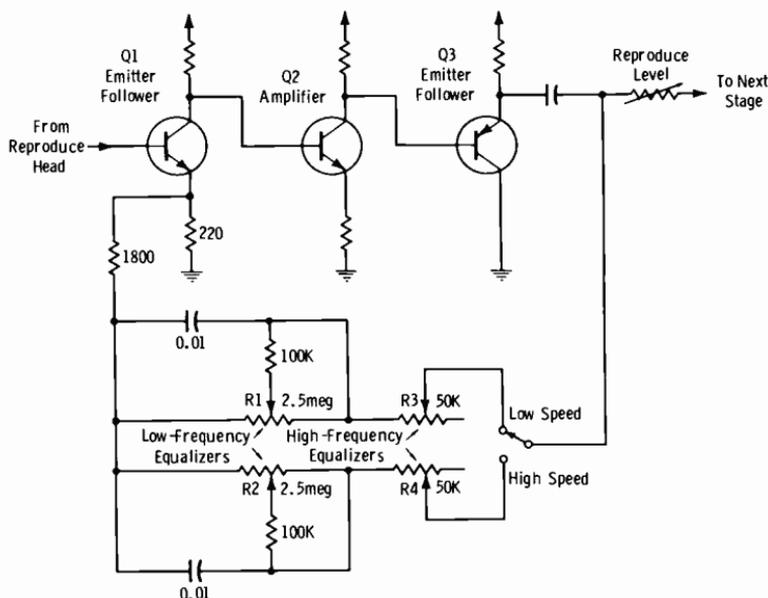
Fig. 5-4. Simplified diagram of typical post-equalization circuitry.
