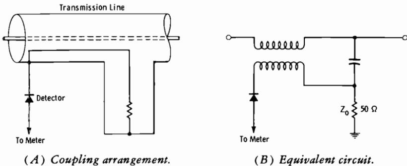
Fig. 10-27. Principle of directional coupler.
