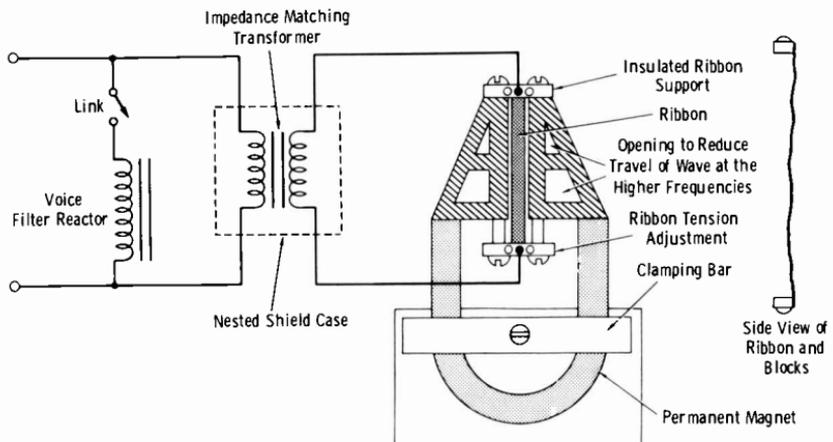
Fig. 4-8. Fundamental construction of ribbon microphone.
