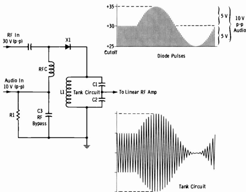
Fig. 9-29. Basic diode modulator.
