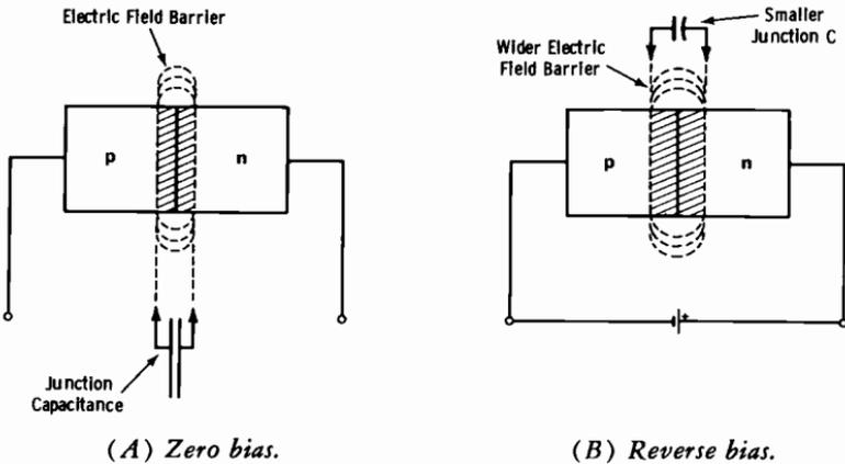
Fig. 10-18. Voltage-variable-capacitance diode.
