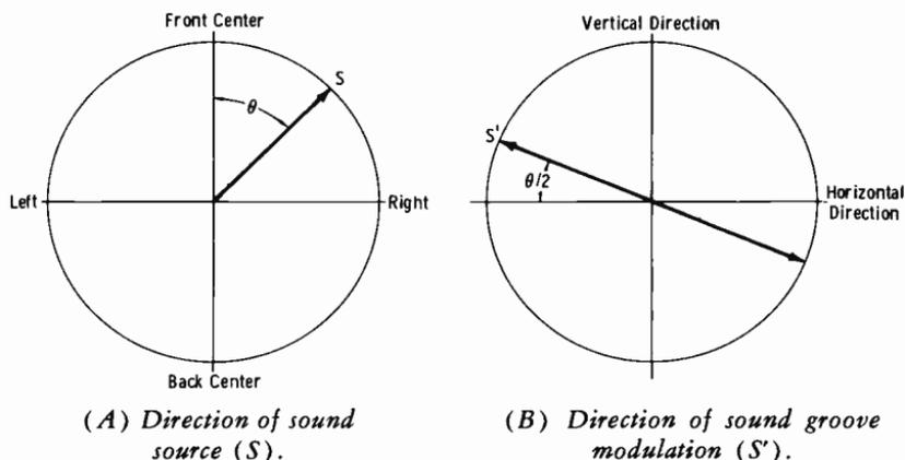
**Fig. 7-10. Directions of sound source and sound groove modulation.**
