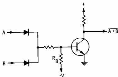
Fig. 3-39. Diode-transistor-logic NOR circuit.
