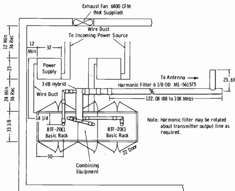
Fig. 10-26. Physical layout of BTF-40E1 transmitter.
