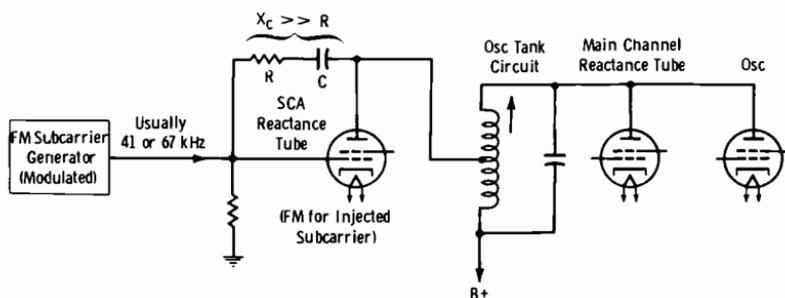
Fig. 10-28. Main-channel and SCA modulation of oscillator.
