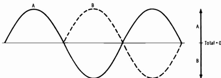
(B) *180° phase difference.***Fig. 11-7. Two harmonic motions of the same frequency.**
