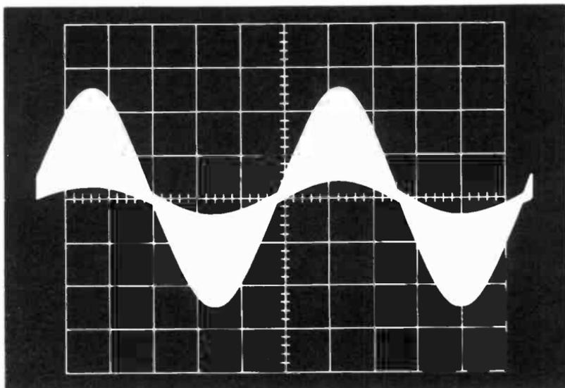
(D) Detected main-channel output where  $L - R$  channel lacks sufficient gain.
