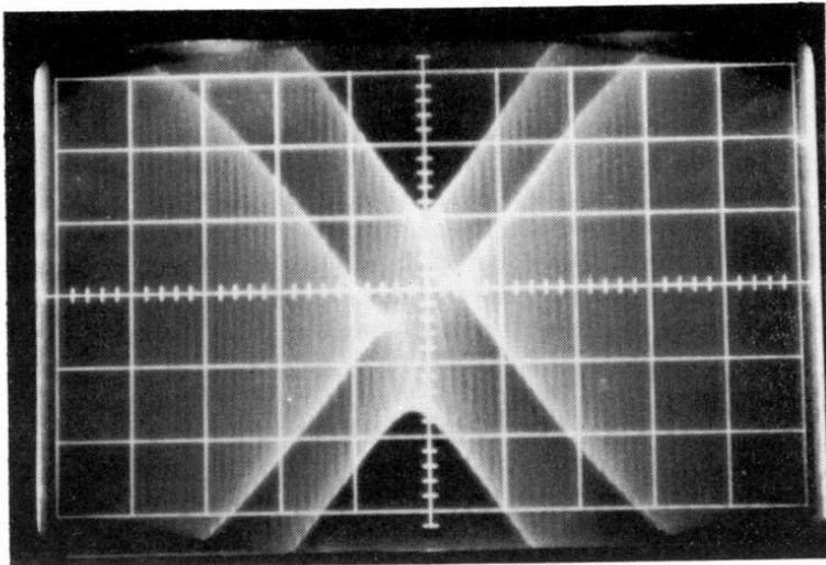
(C) Time base of  $50 \mu\text{s}/\text{cm}$ , incorrect phase.
