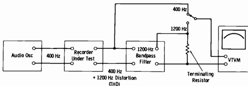
Fig. 13-17. Method of measuring third-harmonic distortion.
