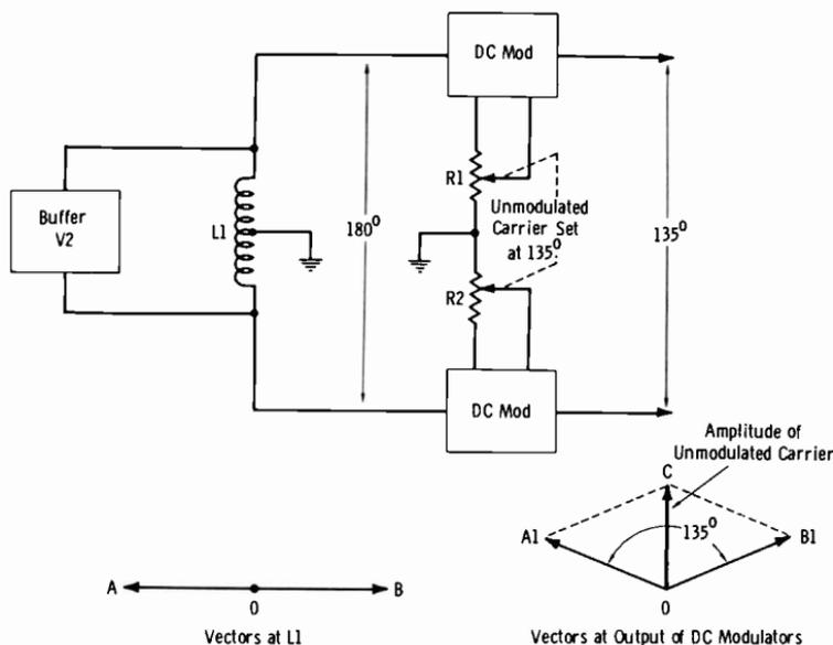
**Fig. 9-31. Principle of carrier phase set.**
