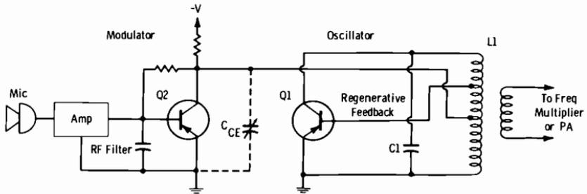
Fig. 8-12. Basic frequency-modulated oscillator.
