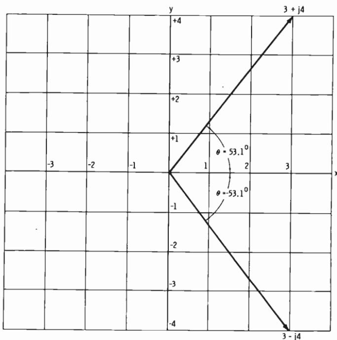
Fig. 2-10. Two vectors in rectangular form.
