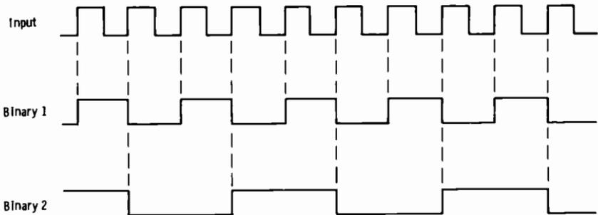
Fig. 3-63. Waveforms of binary circuits.
