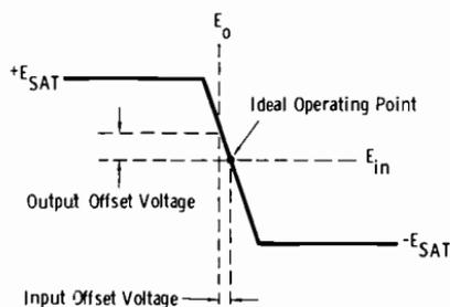
Note: Not to Scale, Since Supply Voltages ( $E_{SAT}$ ) May Be, for Example, + and -10 Volts, While Offset Voltage Is Normally in Millivolts
