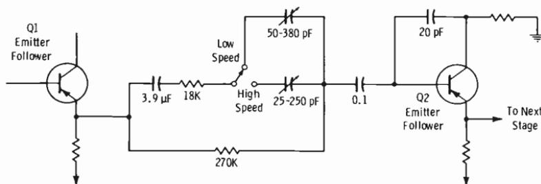
Fig. 5-3. Typical pre-equalization in two-speed tape system.
