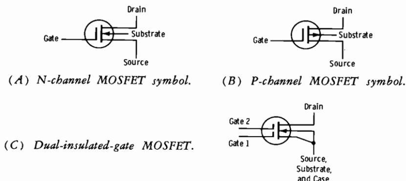
Fig. 3-16. Schematic symbols for MOSFETs.
