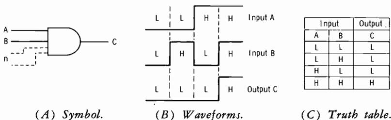
Fig. 3-42. Coincidence (AND) gate.
