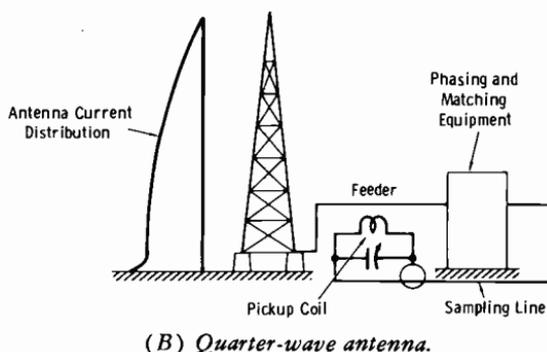
**Fig. 9-19. Antenna current distributions.**
