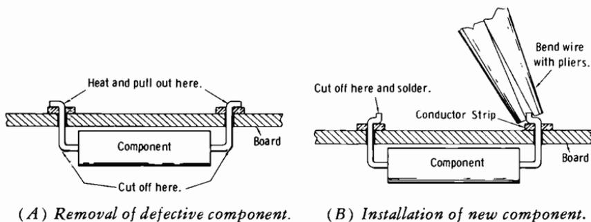
**Fig. 13-10. Replacement of component in printed circuit.**
