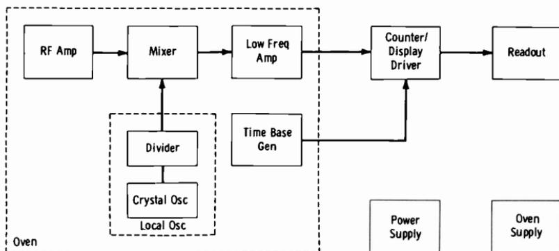
Fig. 9-41. Metron Model 520 digital a-m frequency monitor.
