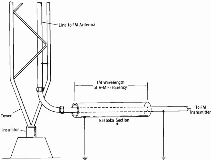
Fig. 9-22. Bazooka used in attaching fm line to a-m tower.
