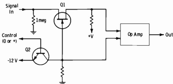
Fig. 6-26. Attenuators using FETs.
