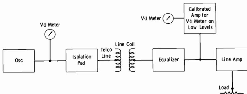
Fig. 8-15. Block diagram of line equalization.
