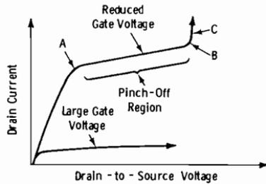
to provide a control element analogous to the grid of a vacuum tube. The FET also has a *source* (analogous to the cathode) and a *drain* (analogous to the plate). Note that the gate receives a voltage which is the reverse bias necessary to control majority-carrier current in the *channel*.
