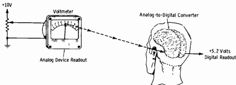
Fig. 3-21. Familiar example of analog-to-digital conversion.
