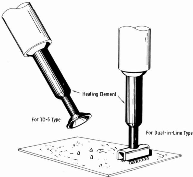
**Fig. 13-13. Desoldering tools for integrated circuits.**
