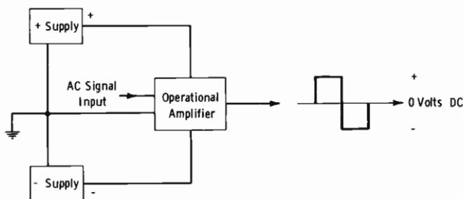
(B) *Method of obtaining dc ground at output.***Fig. 3-54. Fundamentals of operational amplifier.**
