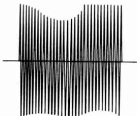
(E) *Push-pull stage with overloaded single-ended driver stage.*
