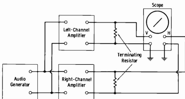
(B) Arrangement for phase-shift measurement.
