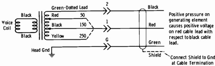
(A) *E-V Model 666.*
