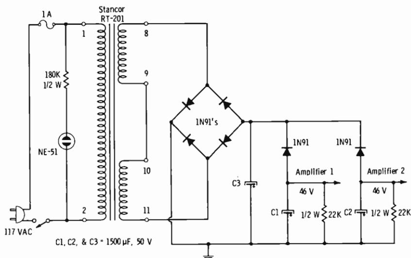
(B) Power-supply schematic.
