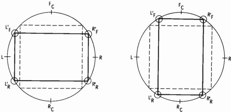
(A) Angle less than  $22.5^\circ$ .(B) Angle greater than  $22.5^\circ$ .**Fig. 7-17. Reproduced sound field simulation when angle  $\theta$  is not  $22.5^\circ$ .**
