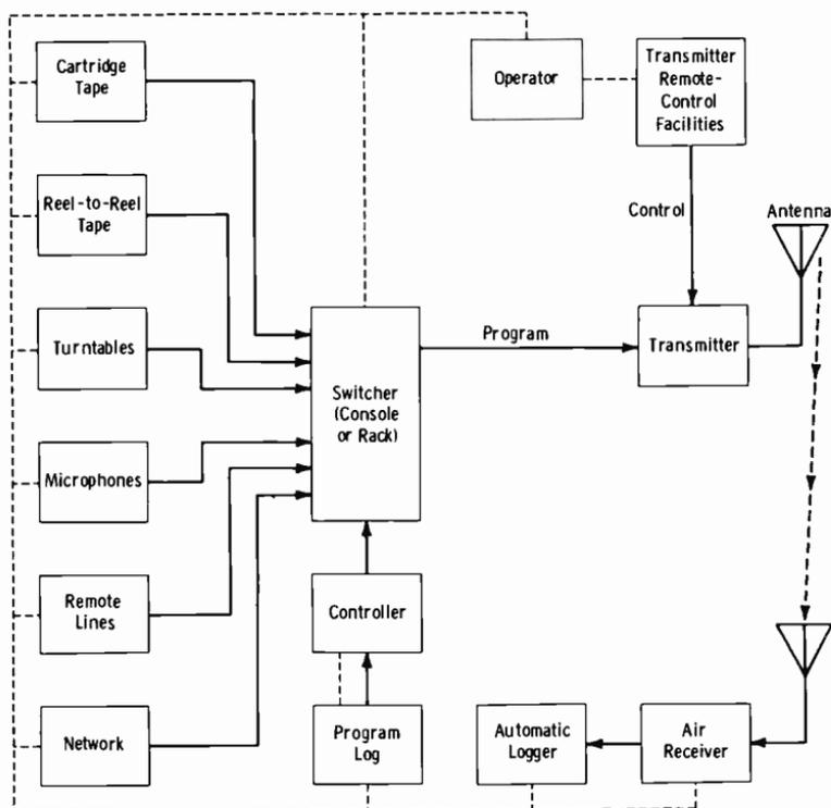
Fig. 7-27. Basic technical automation facility.
