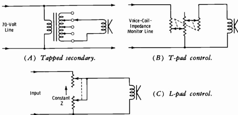
Fig. 6-49. Control of volume of individual speakers.
