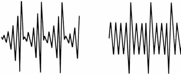
Fig. 11-6. Waveforms of two male voices intoning the same vowel.
