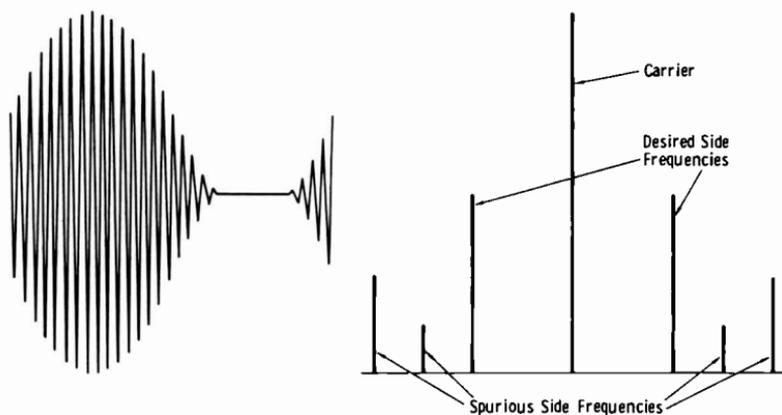
(B) *Overmodulated.***Fig. 9-35. Sidebands of amplitude-modulated carrier.**
