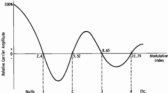
Fig. 14-30. Variation of carrier amplitude with modulation index.
