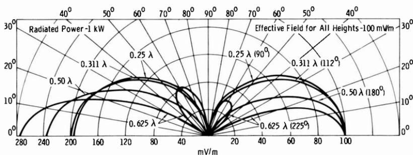
Vertical Radiation Patterns for Different Heights of Vertical Wire Antennas
