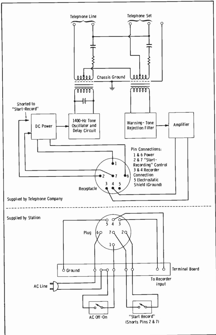
Fig. 8-16. Typical recorder-connector arrangement.
