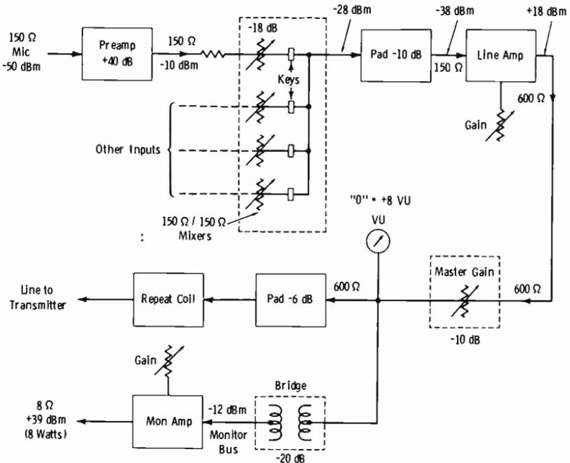
Fig. 6-35. Typical broadcast audio circuit.
