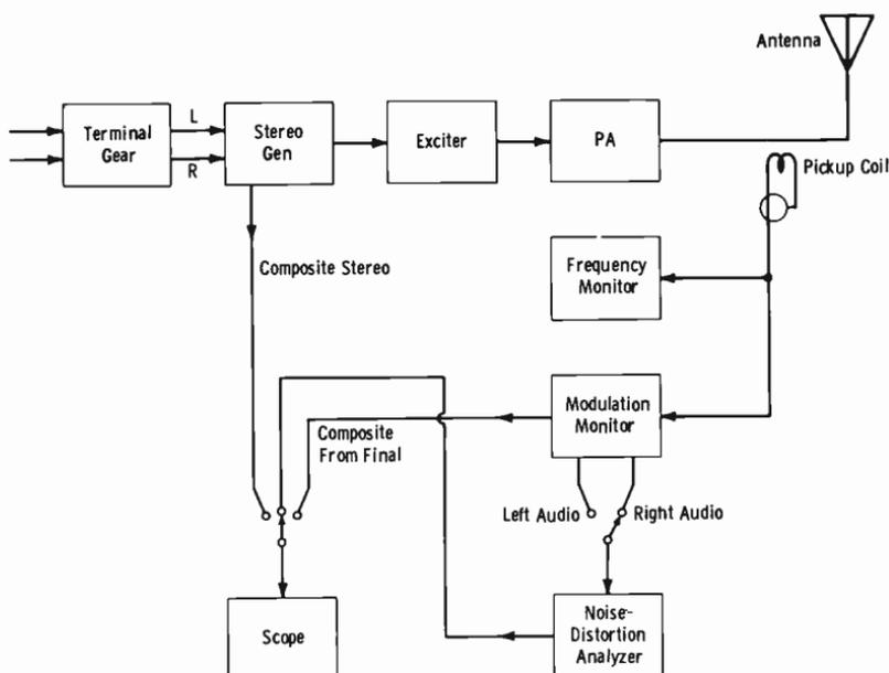
Fig. 14-27. Transmitter setup for stereo measurements.
