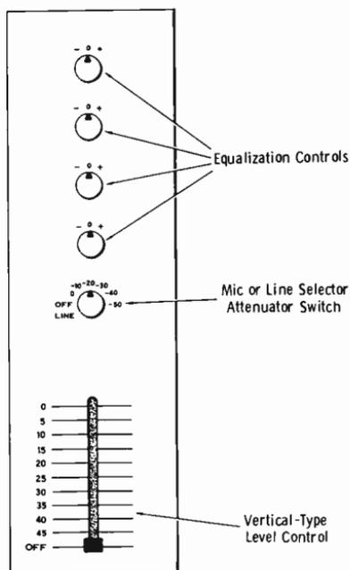
illustrates a typical control-panel module for an individual channel in such a system. Quite often these modules are of the plug-in variety for maximum versatility of application in custom consoles. These may be used with or without echo equipment, which has wide application in special productions (Chapter 11).
