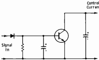
Fig. 6-38. Power rectifier circuit diagram.
