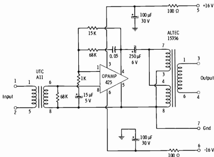
Fig. 7-4. Circuit of line amplifier.
