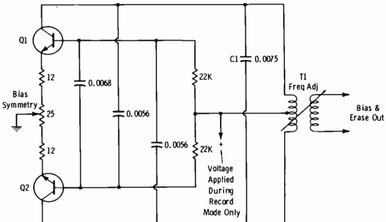
Fig. 5-7. Typical erase and bias oscillator.
