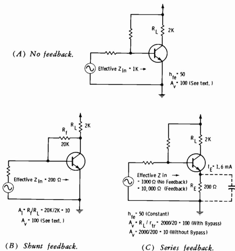
Fig. 3-5. Comparison of shunt and series feedback.
