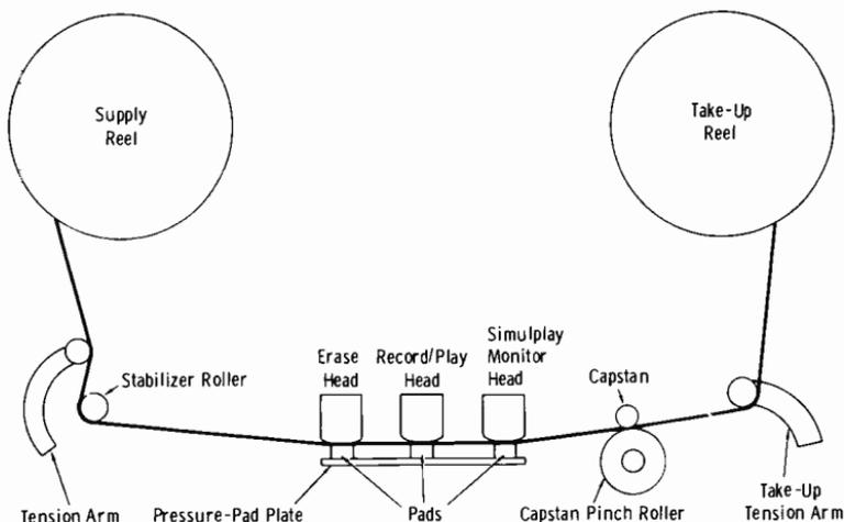
Note: Pressure pads are not used in many late model recorders. The head assembly is moved downward by a solenoid to make contact with the tape during recording or playback. In fast wind or rewind, the head assembly is moved upward away from the tape, as in the stop position.
