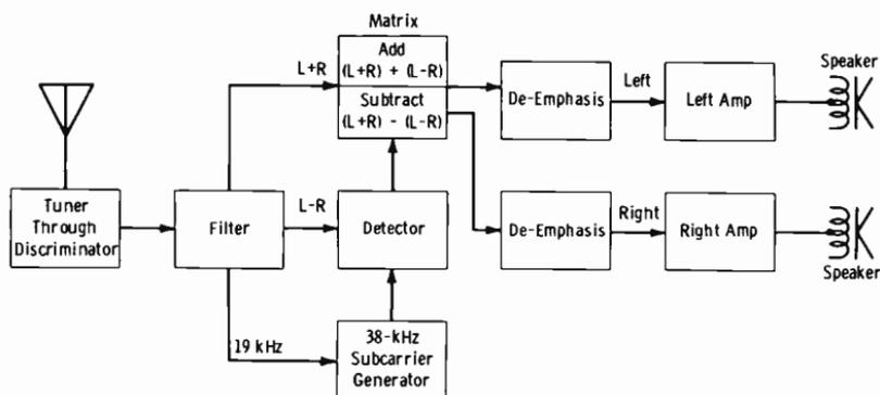
Fig. 10-32. Block diagram of stereo receiver.
