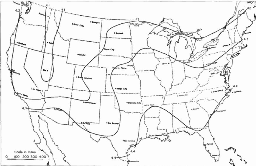
FIG. 17. August values of 300-mile propagation path absorption loss (in db) to be exceeded 1 per cent of the time for a frequency of 10 Gc/s.
