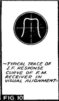
~ TYPICAL TRACE OF I.F. RESPONSE CURVE OF F.M. RECEIVER IN VISUAL ALIGNMENT ~
