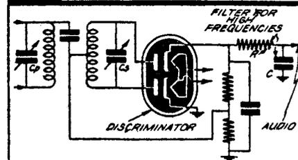
FIG. 21 ~POSITION OF HIGH-FREQUENCY ATTENUATING FILTER IN DISCRIMINATOR-AUDIO CIRCUIT. REDUCTION IN R OR C VALUES WILL INCREASE HIGH-FREQUENCY RESPONSE~
