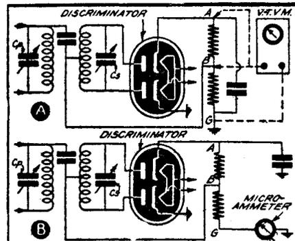
FIG. 20 ~METHOD OF CONNECTING INDICATOR FOR DISCRIMINATOR ALIGNMENT~
