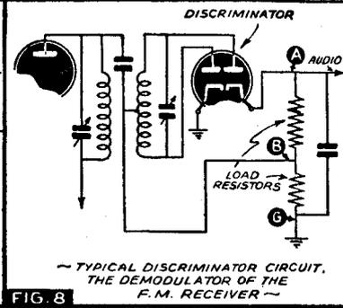
~ TYPICAL DISCRIMINATOR CIRCUIT, THE DEMODULATOR OF THE F.M. RECEIVER ~
