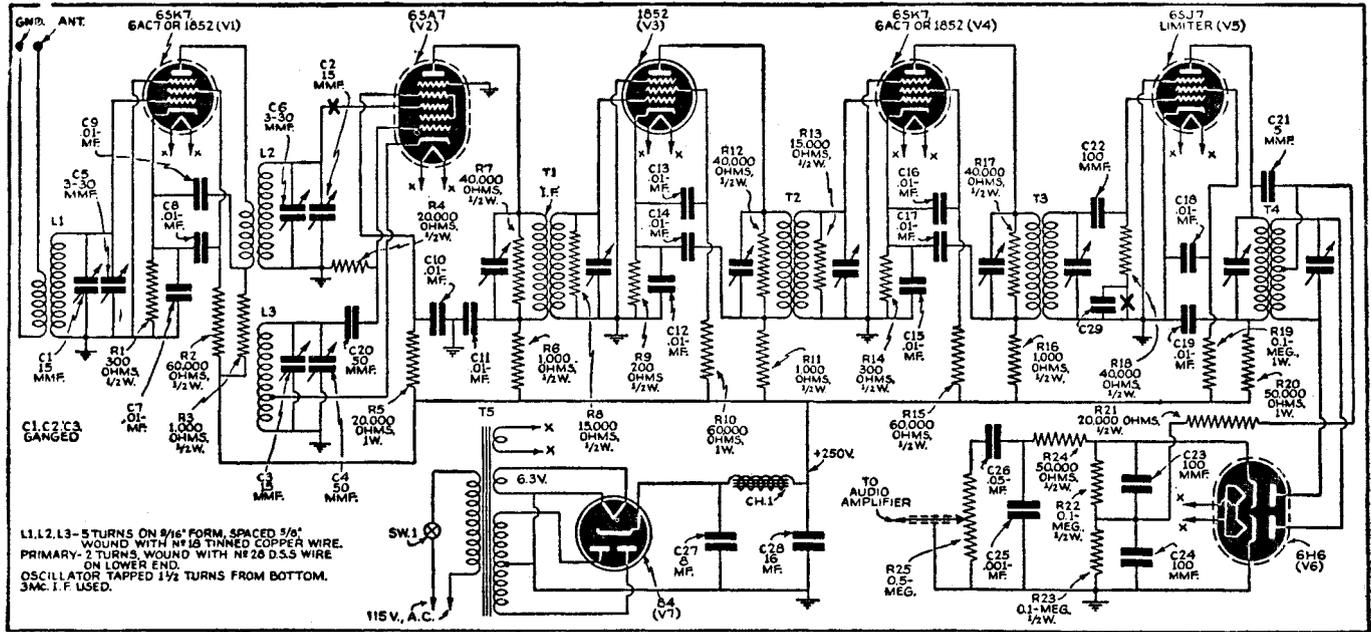
L1, L2, L3 - 5 TURNS ON #16 FORM, SPACED 5/8" WOUND WITH #18 TINNED COPPER WIRE. PRIMARY - 2 TURNS WOUND WITH #26 D.S.S WIRE ON LOWER END. OSCILLATOR TAPPED 1/2 TURNS FROM BOTTOM. 3MC. I.F. USED.
