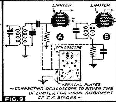
~ CONNECTING OSCILLOSCOPE TO EITHER TYPE OF LIMITER FOR VISUAL ALIGNMENT OF I.F. STAGES ~
