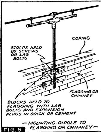
Fortunately, the current and voltage distribution on a half-wave doublet or dipole antenna, which is the most effective and popular type employed for F.M. reception, is such that the voltage at the center of the dipole is theoretically zero. This is shown at Fig. 1. For this reason, and since the 2 sections of the antenna are generally supported at the center, it is not absolutely essential that extremely-low-loss insulators or supports be used for this purpose.
