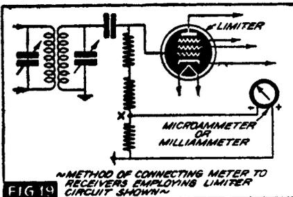
FIG. 19 ~METHOD OF CONNECTING METER TO RECEIVERS EMPLOYING LIMITER CIRCUIT SHOWN~
