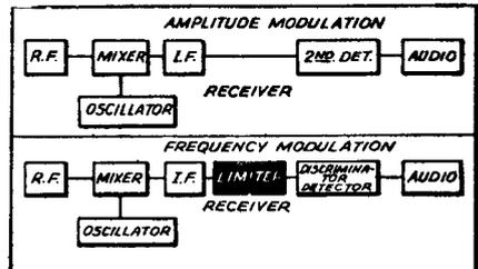
FIG. 1 ~ SIMPLIFIED BLOCK DIAGRAMS SHOWING SEQUENCE OF A.M. AND FM RECEIVER STAGES ~
