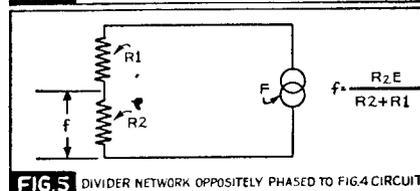
FIG. 5 DIVIDER NETWORK OPPOSITELY PHASED TO FIG. 4 CIRCUIT
