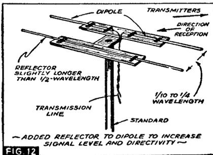
obtain the requisite rigidity, only wire of a heavy gauge, either No. 10 or No. 12, should be used, supported by low-loss insulators. The transmission line must be run at right-angles to the dipole for at least a  $\frac{1}{4}$ -wavelength, at least 5 feet, before any bends in the line are made.
