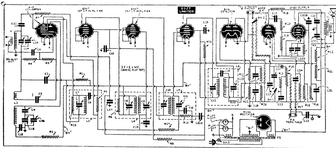
Schematic circuit of the G.E. HM-80 table-model frequency-modulated receiver
