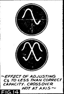
~ EFFECT OF ADJUSTING  $C_s$  TO LESS THAN CORRECT CAPACITY. CROSSOVER NOT AT AXIS ~
