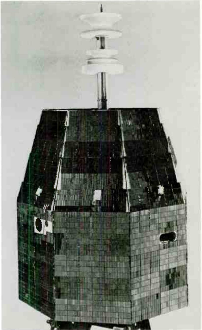
Fig. 1-6. The Relay satellite weighed 169 pounds—less than the first Sputnik (courtesy NASA).
