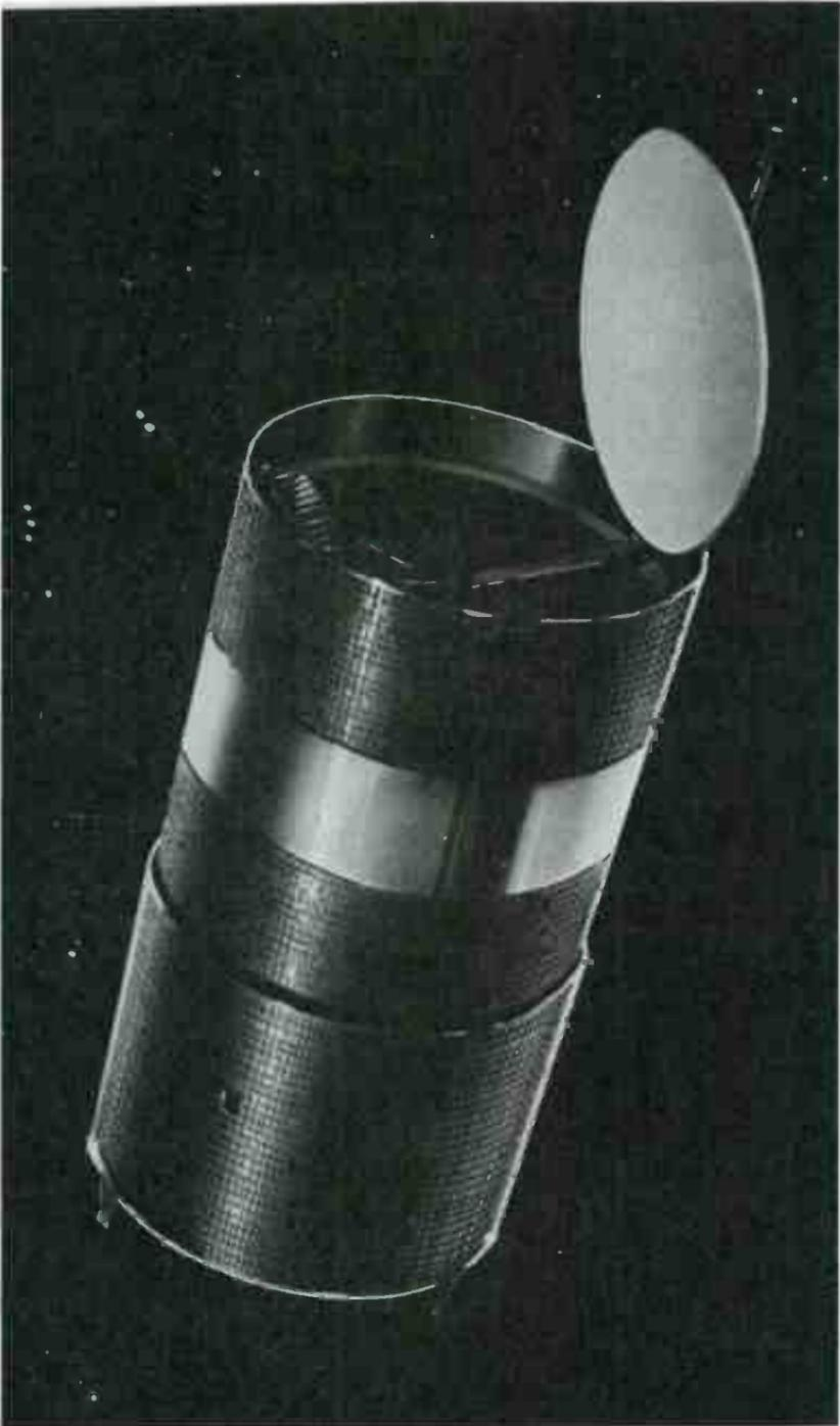
Fig. 9-1. Westar IV has the capacity to handle 24 channels of television simultaneously.
