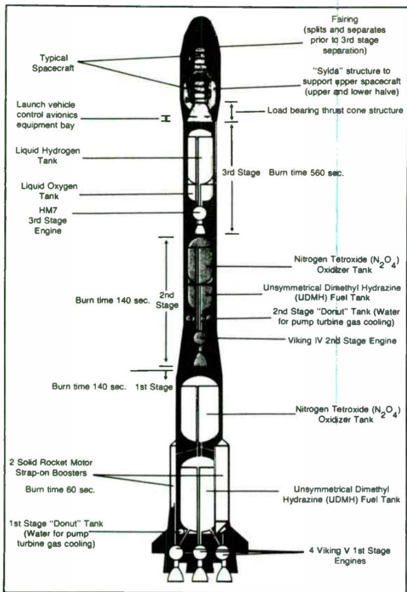
Fig. 1-21. The European Ariane is a competitor for the space shuttle for launching communications satellites (courtesy GTE).
