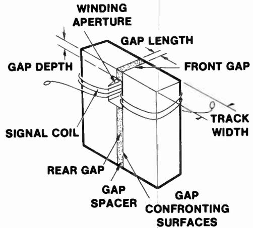
Figure 38 Typical Video Head Core
