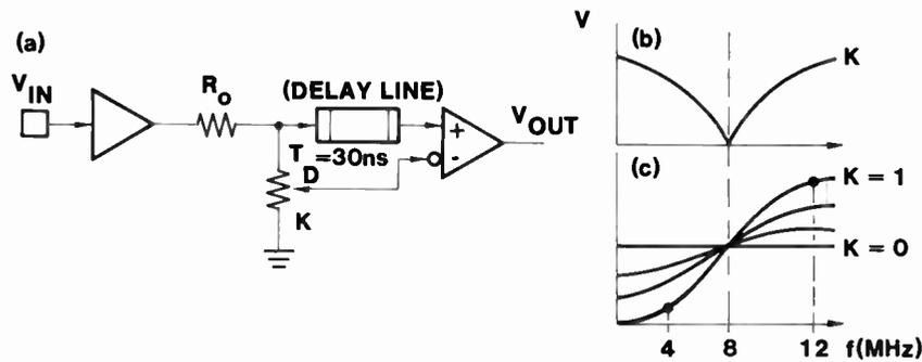
**Fig. 79 Aperture Correction by Cosine Equalizer - Single Delay Line Method**
