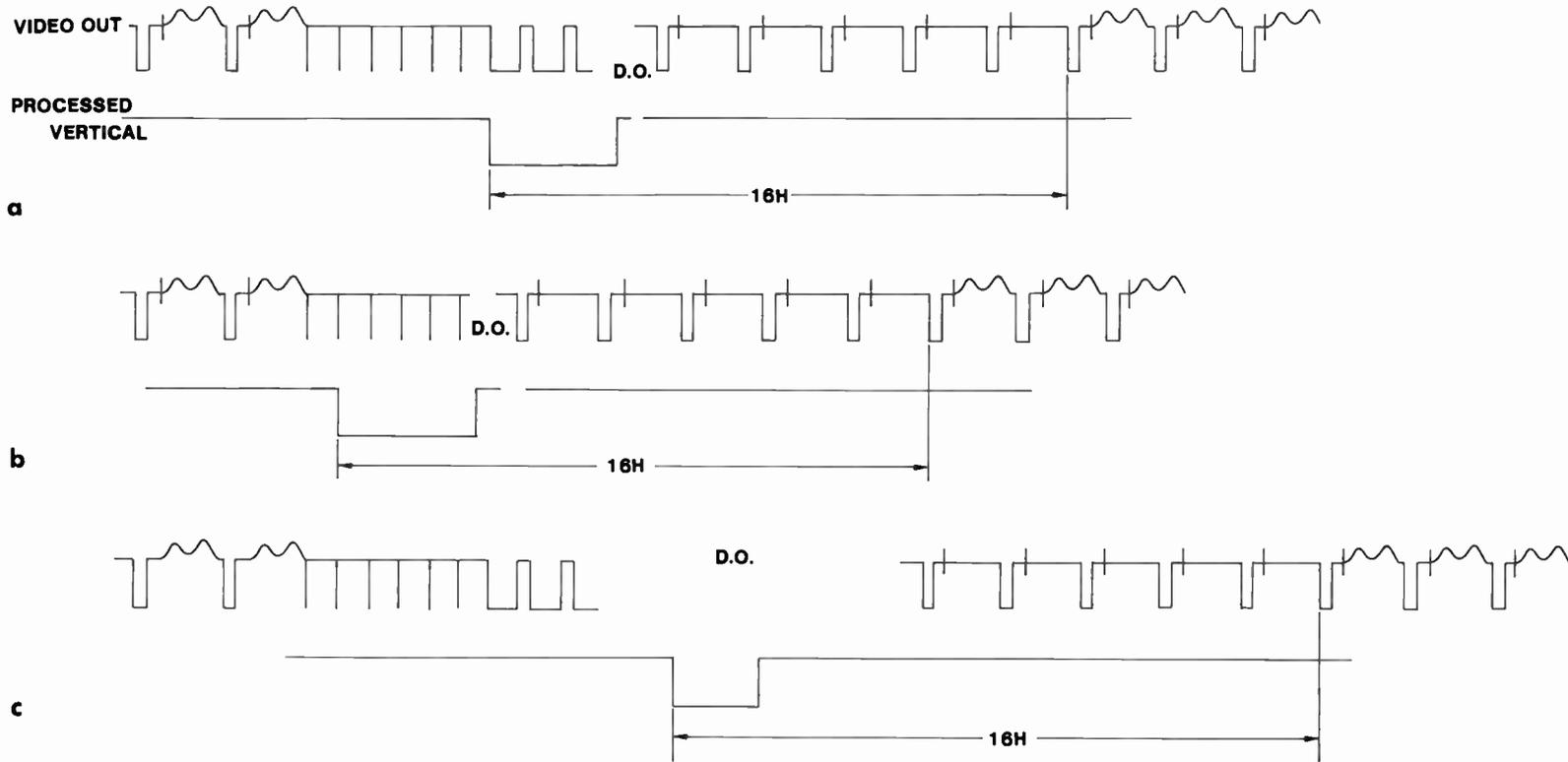
Fig. 142 Processed Vertical Output for Various Playback Conditions - 525 Line Format
