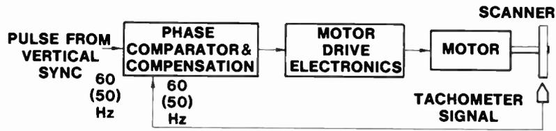
Fig. 111 Type C VTR Scanner Servo
