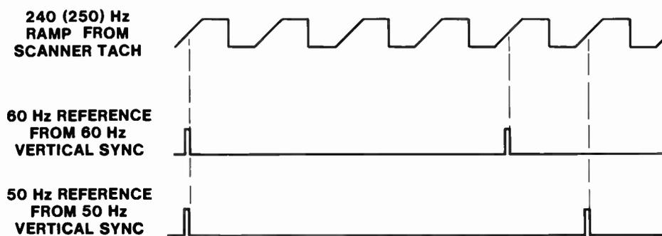
Fig. 110 Phase Comparison by Sample and Hold Circuit
