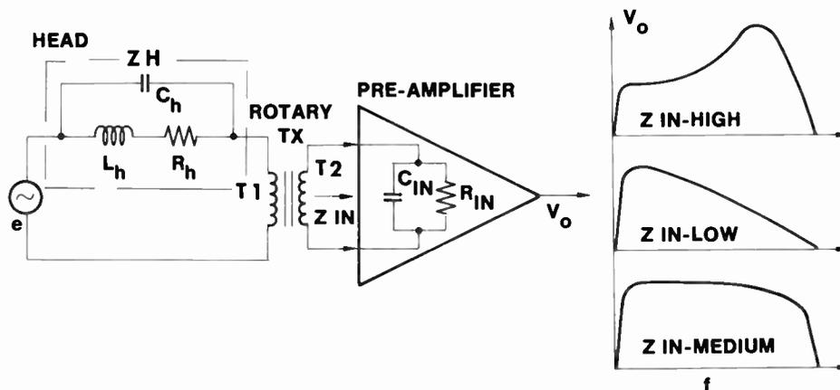
Fig. 78 Response as Function of Pre-Amp Input Impedance
