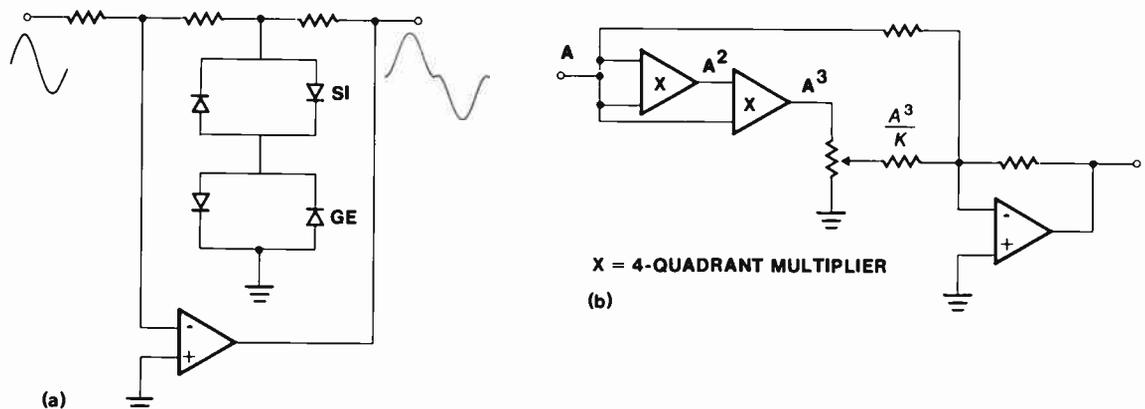
Fig. 153 Methods for Generating Odd-Order Harmonics
