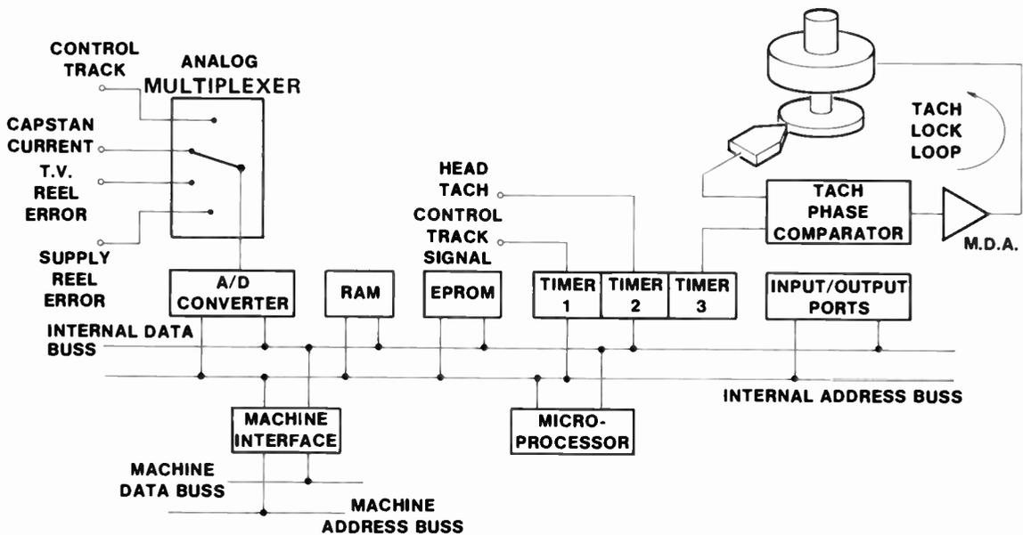
Fig. 144 Basic Configuration of Microprocessor - Controlled Servo Control System
