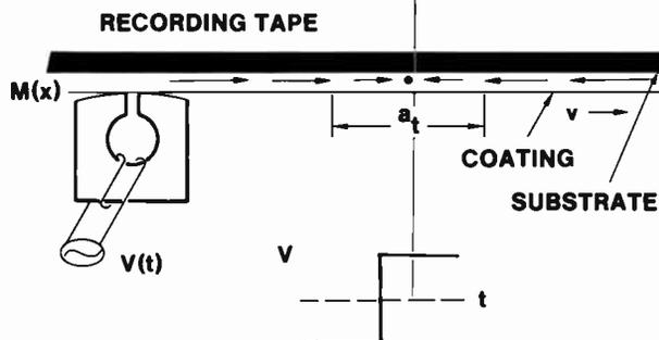
Fig. 8 Resultant Magnetization From a Step Change in Head Voltage
