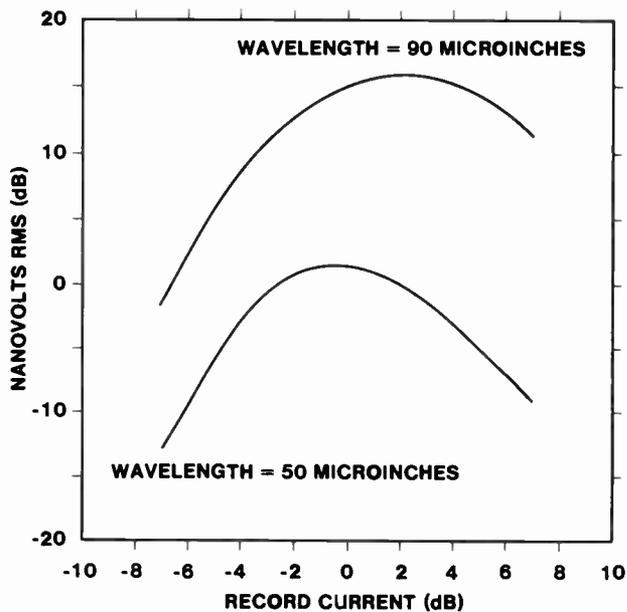
Fig. 11 Reproduce Voltage vs Record Current for Typical Video Tape
