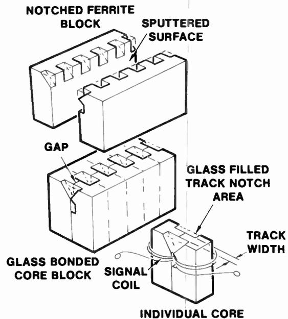
**Fig. 57 Narrow Track Ferrite Head Fabrication**
