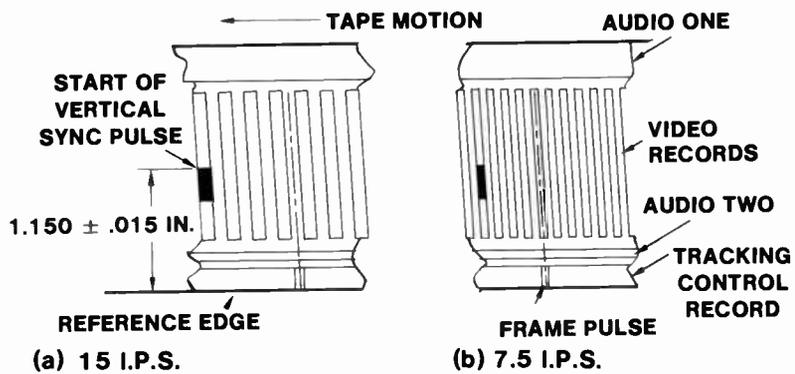
Fig. 108 Quadruplex 525/60 Format
