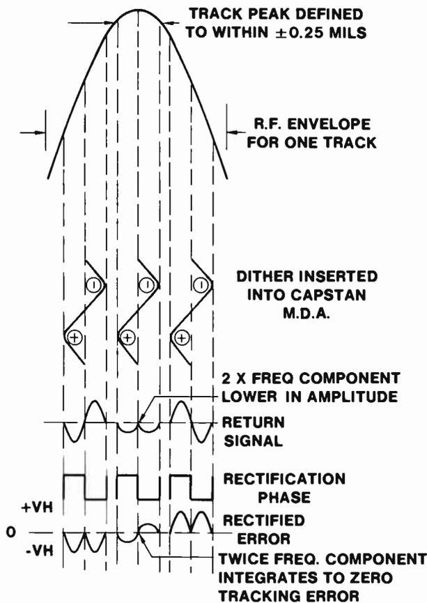
Fig. 127 Operation of Synchronous Detector
