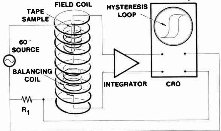
Fig. 33 Loop Tracer
