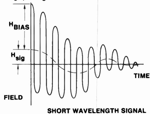
Fig. 12 Signal Field History for a.c. Bias and Recording
