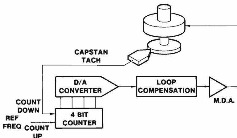
Fig. 147 Wide Range Phase Comparator for Tach Lock Loop
