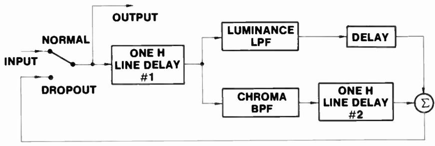
Fig. 90 Comb Filter-Based D.O.C.
