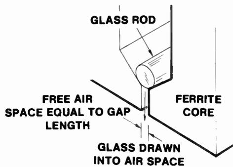
**Fig. 56 Capillary Bonding Technique for Ferrite Heads**
