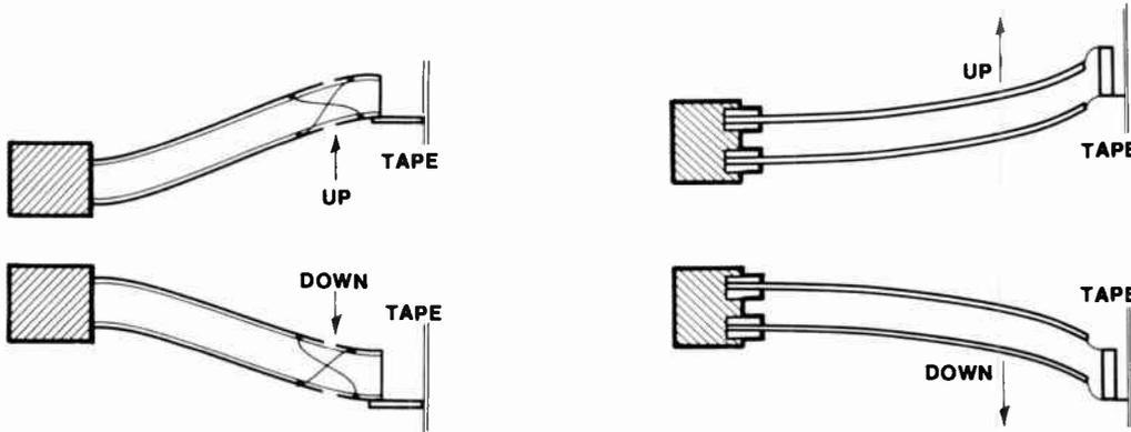
**Fig. 135 Zenith Error Correction by Deflector Re-curling**
