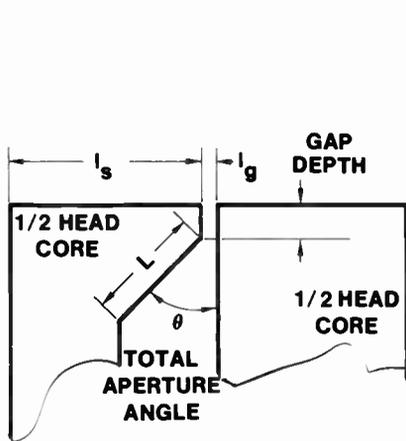
Figure 42 Aperture Angle
