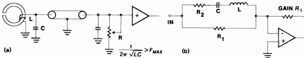
Fig. 148 Resonance Used to Correct for  $\sin \frac{X}{X}$  Loss
