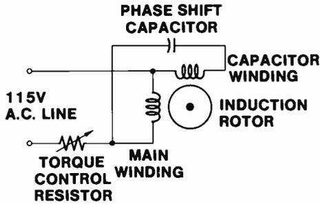
Fig. 107 A.C. Torque Motor Reel Drive Circuit
