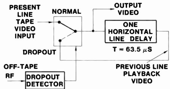
Fig. 87 Simple Monochrome Previous-Line D.O.C.
