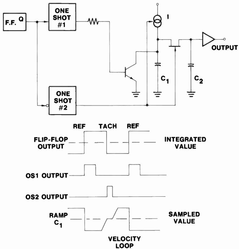
Fig. 117 Removal of Clocking Signals by Clamping
