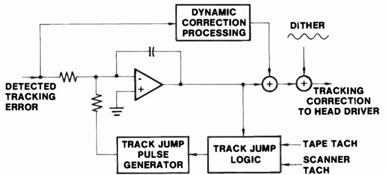
Fig. 141 Error Signal Processing Based on Head Deflection Information
