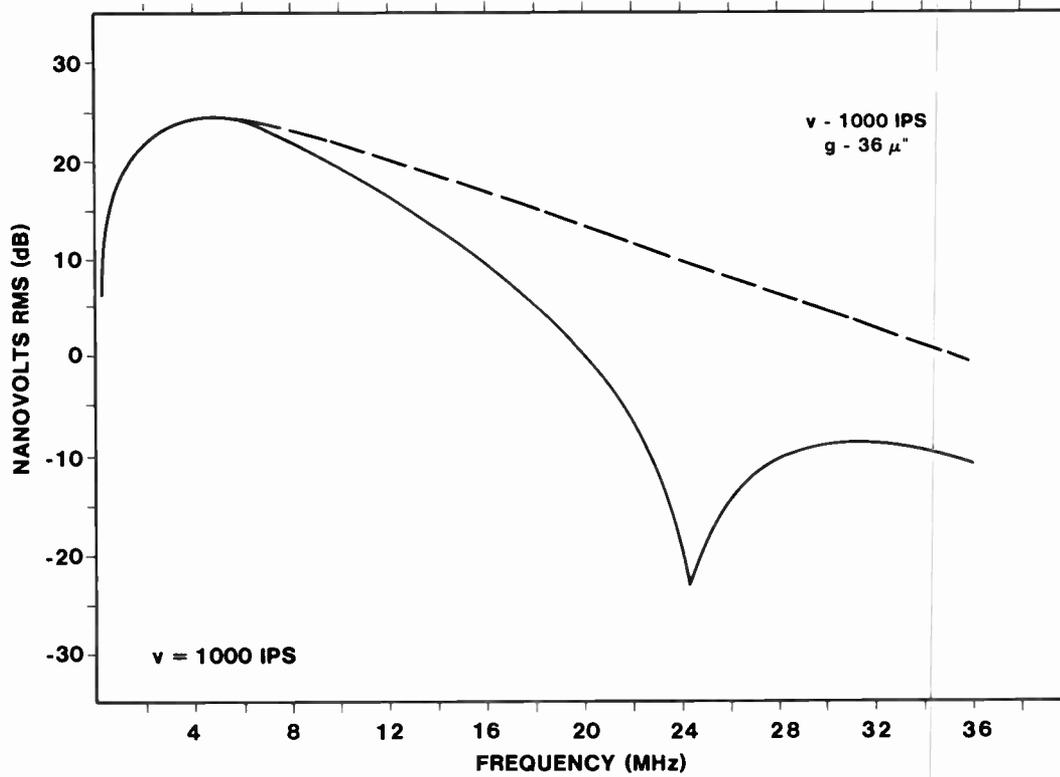
Fig. 16 Voltage Spectrum for Typical Video Tape
