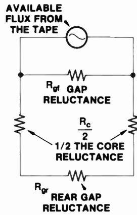
Figure 40 Electrical Analog of Playback Head
