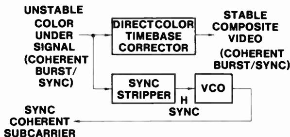
Fig. 95 Time Base Correction of Color-Under Signals by Direct Color TBC
