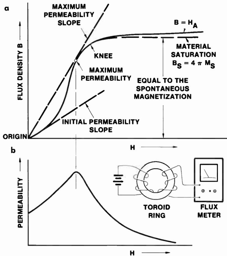
Fig. 25a Initial B-H Curve
