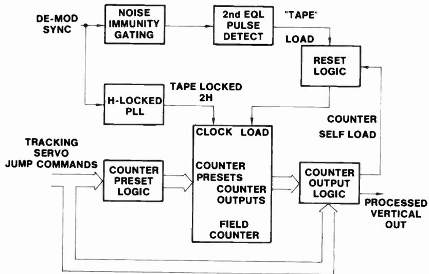
Fig. 143 Processed Vertical Generator
