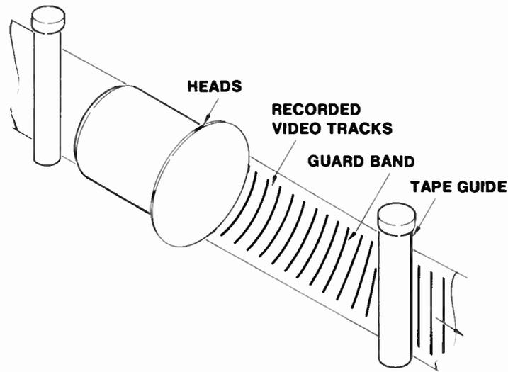
Fig. 60 Transverse Scan Configuration
