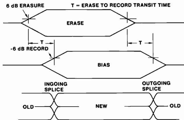
**Fig. 154 Controlled Onset and Decay of Bias and Erase for Editing**
