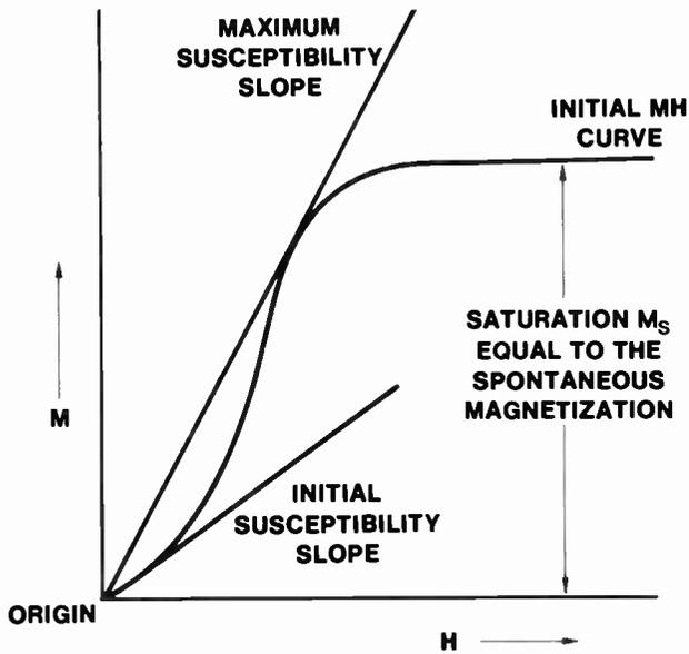
Fig. 30 Initial M-H Curve
