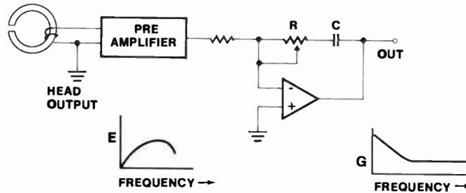
Fig. 149 Typical Reproduce Equalizer
