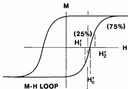
Fig. 9 M-H Hysteresis Loop for a Typical Tape
