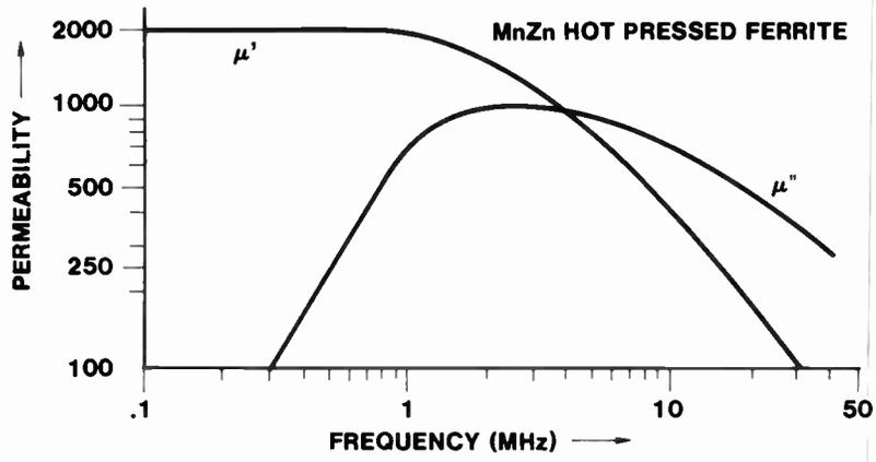
Fig. 45 Permeability vs. Frequency for Hot Pressed Ferrite
