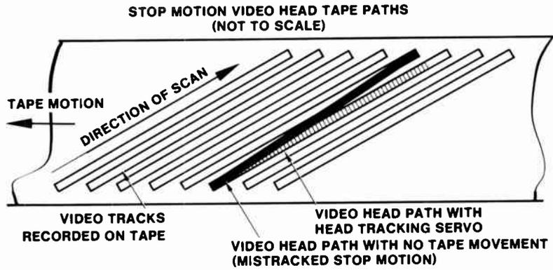
**Fig. 128 Head Tracking Geometry**
