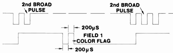
Fig. 113 b) Helical Control Track Record Waveform
