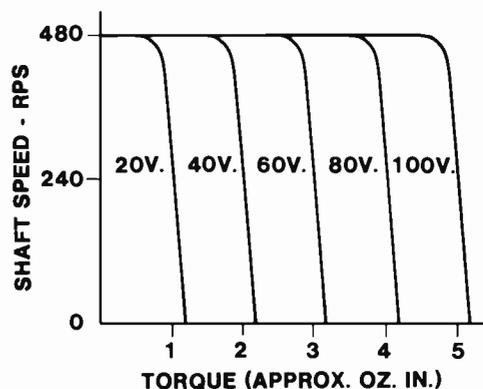
Fig. 106 Hysteresis Motor Operating Below Synchronous Speed
