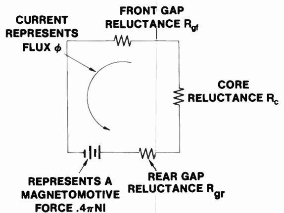
Fig. 39b Electrical Analog
