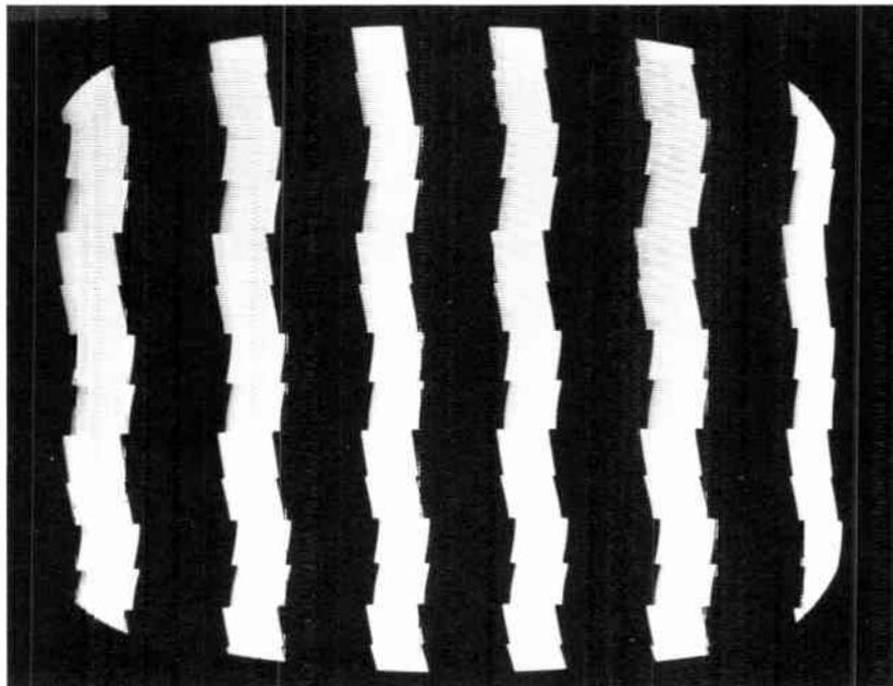
**Fig. 101 Effect of Quadrature Errors on a Reproduced Picture**
