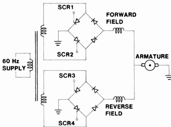
**Fig. 122 SCR Controlled Reel Motor**
