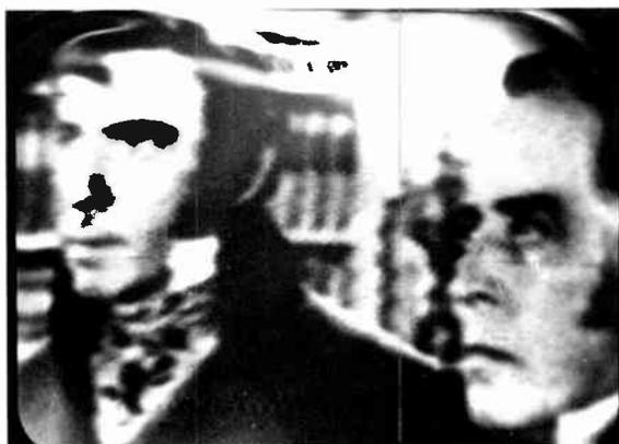
**Fig. 3** By March 1955 the Ampex team had corrected many of the playback problems by introducing an FM signal. The comparative improvement in this picture encouraged Ampex to support the video project with time and money commitments.
