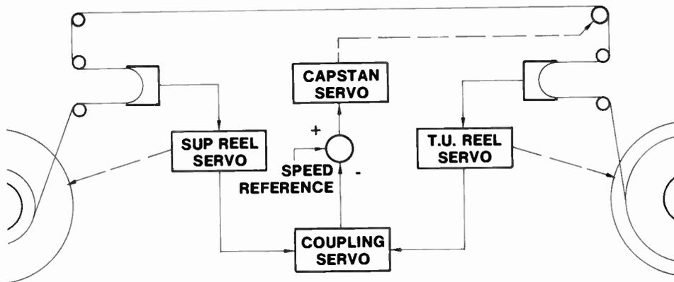
Fig. 125 Reel-to-Capstan Coupling Servo
