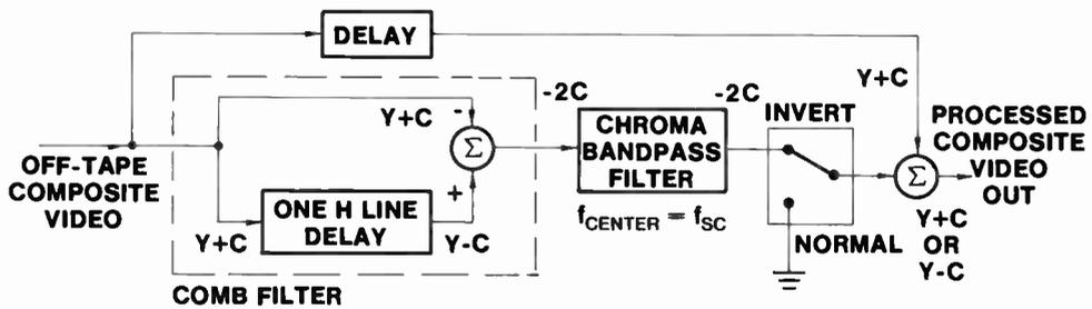
Fig. 92 Comb Filter Based Chroma Processor (NTSC)
