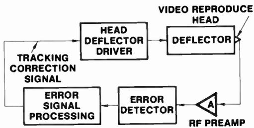
**Fig. 130 Head Tracking Servo**
