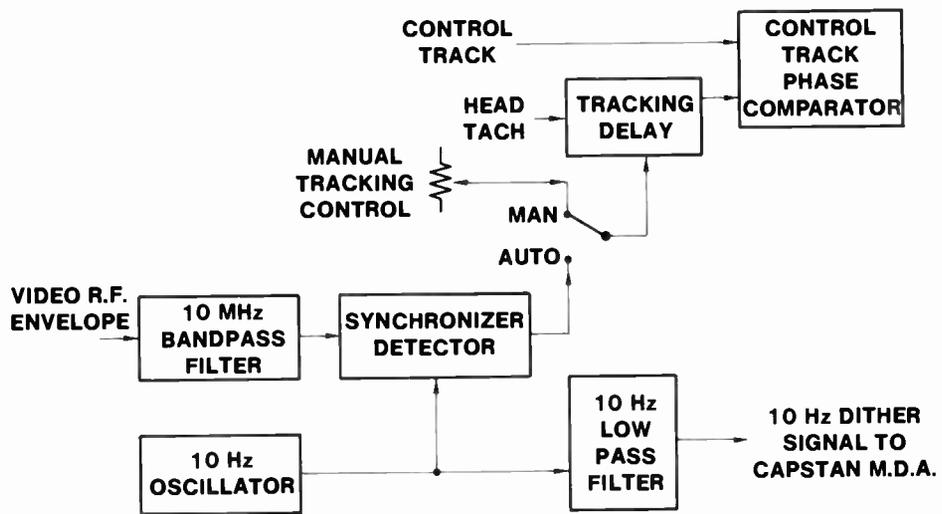
Fig. 126 Block Diagram of Autotracking System
