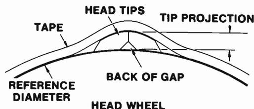
Fig. 99b Head-Tip-Tape Engagement Detail
