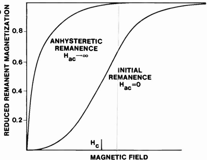
Fig. 13 Comparison of Sensitivities of a.c. Bias and Direct Recording
