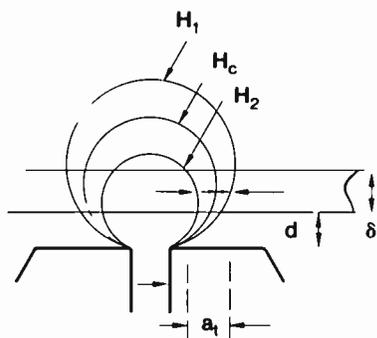
**Fig. 10 Head Field contours Showing Recording Zone in Tape**
