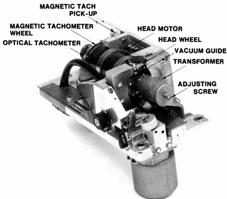
Fig. 96 Ampex Mk XV Video Head Wheel Panel
