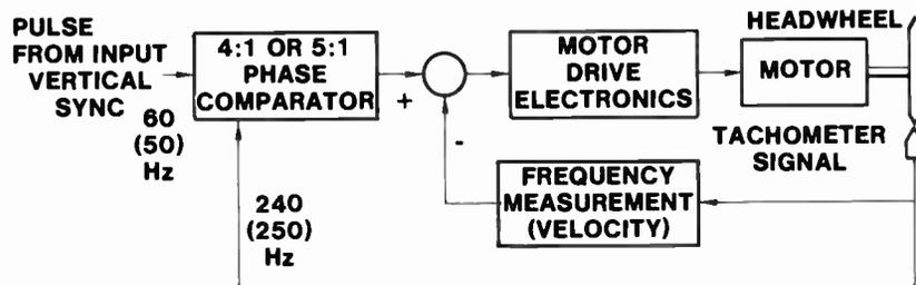
Fig. 109 Record Mode Head Wheel Servo
