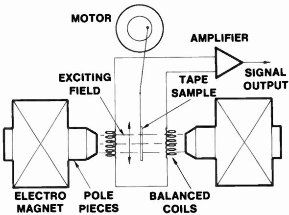
Fig. 32 Vibrating Sample Magnetometer
