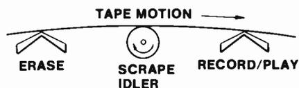
Fig. 155 Inertial Damping of Scrape Flutter
