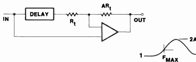
Fig. 151 Delay-Line Equalizer
