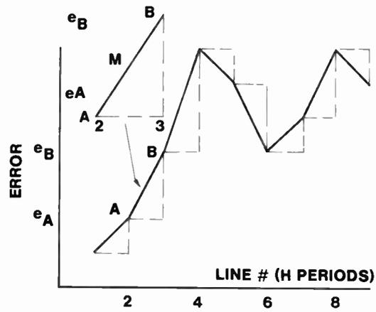
Fig. 85 First Order Interpolation of Velocity Error
