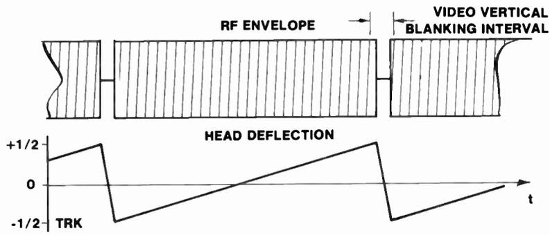
Fig. 138 Playback Envelope in Still Field Mode
