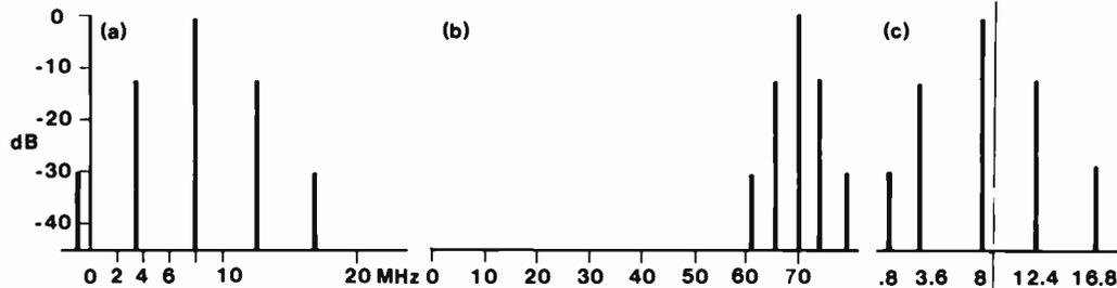
Fig. 68 FM Signal Spectra
