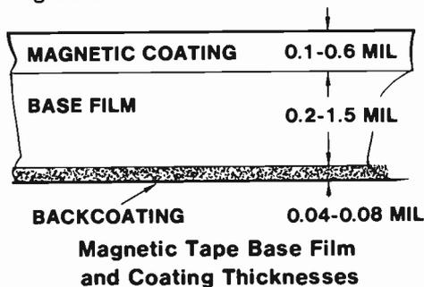
**Backcoating** Backcoatings are used primarily in the most demanding tapes, such as professional and some consumer video, professional audio, instrumentation and data products, where special winding and handling characteristics are required. This coating contains a conductive pigment, usually carbon black, which reduces buildup of
