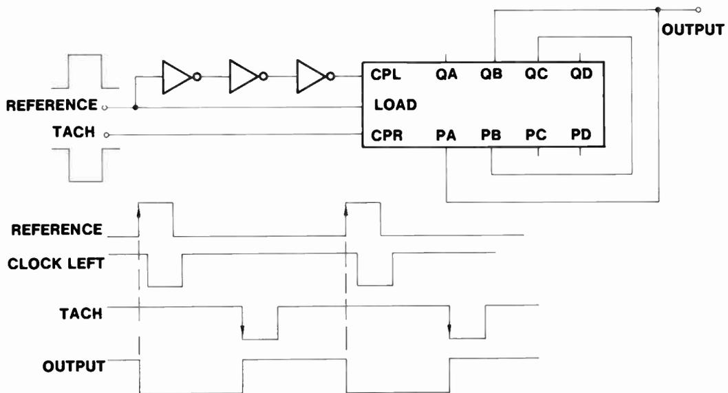
Fig. 116 Digital Phase Comparator
