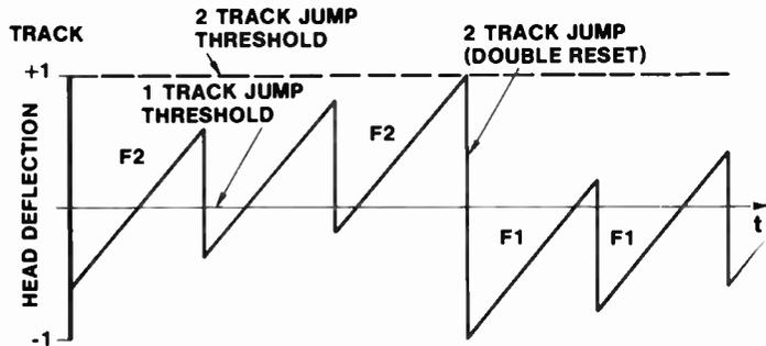
Fig. 140 Error Processing Output for 1/5 Speed Reverse Mode
