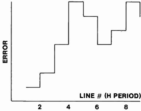
Fig. 84 Line-by-Line Error Profile (Zero Order)
