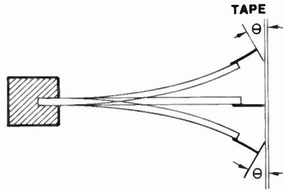
**Fig. 134 Head to Tape Angle as a Result of Deflection**
