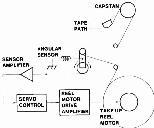
**Fig. 120 Closed Loop Servo Using Tension Arm**
