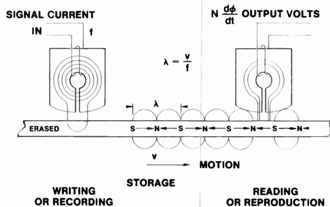
**Fig. 7 Fundamental Recording and Reproduction Process**
