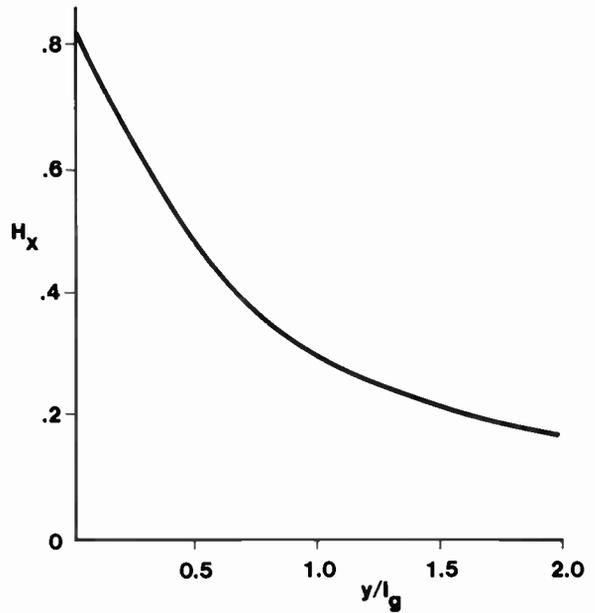
Fig. 49 Longitudinal Field vs. Recording Depth to Gap Length Ratio
