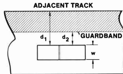
**Fig. 152b Dimensions for Reproduce Crosstalk Calculation**
