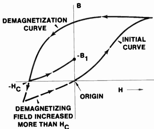
Fig. 36 Demagnetization Curve
