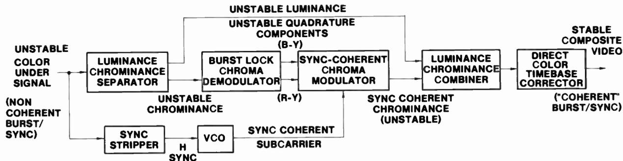
Fig. 94 Interactive Timebase Correction of Color-Under Signals (One Wire Operation)
