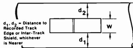
**Fig. 152a Dimensions for Fringing Gain Calculation**
