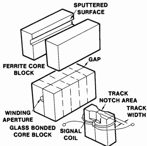
**Fig. 55 Wide Track Ferrite Head Fabrication**
