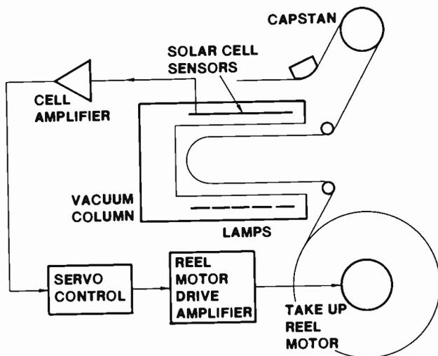
**Fig. 119 Closed Loop Servo Using Vacuum Column**
