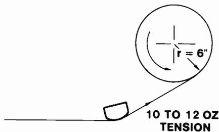
Fig. 118 Torque as a Function of Radius
