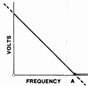
Fig. 74 Straight Line Equalizer Limitations
