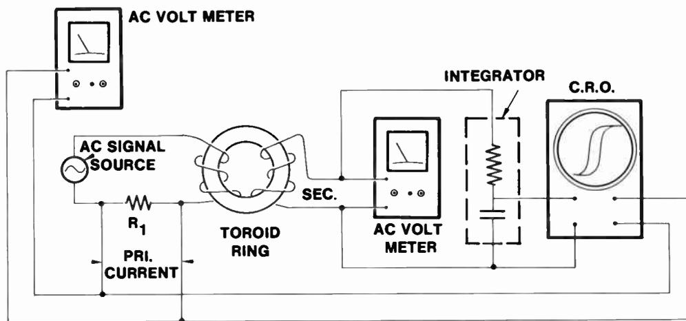
Fig. 28 Measurement of Permeability and B-H Loop for Soft Materials
