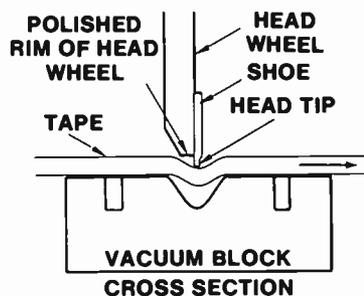
Fig. 99a Cross Section of Vacuum Guide
