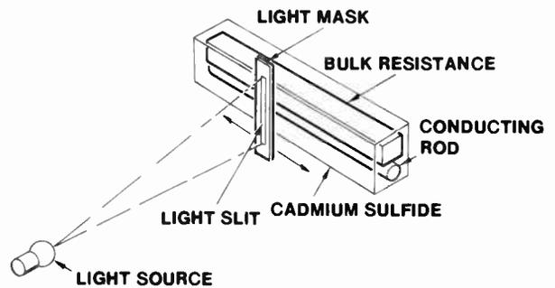
**Fig. 121 Cadmium Sulphide Photo Pot Sensor**
