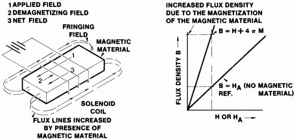
Fig. 24 Increase in Flux with Magnetic Core Material
