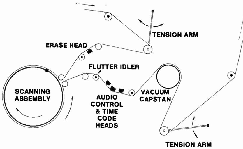
Fig. 103 Advanced Type C Format Transport
