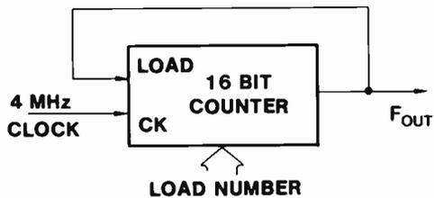
Fig. 145 Counter Loading Method
