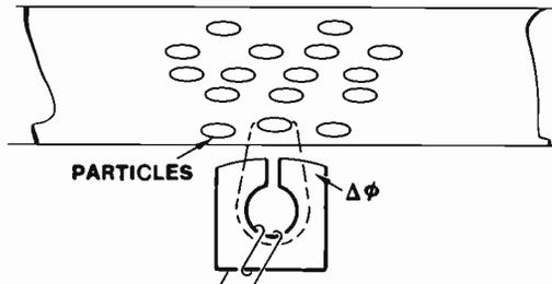
Fig. 18 Flux Contribution From Each Particle as a Source of Noise
