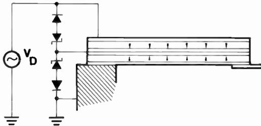
Fig. 133 Deflector Drive Using Zener Diodes
