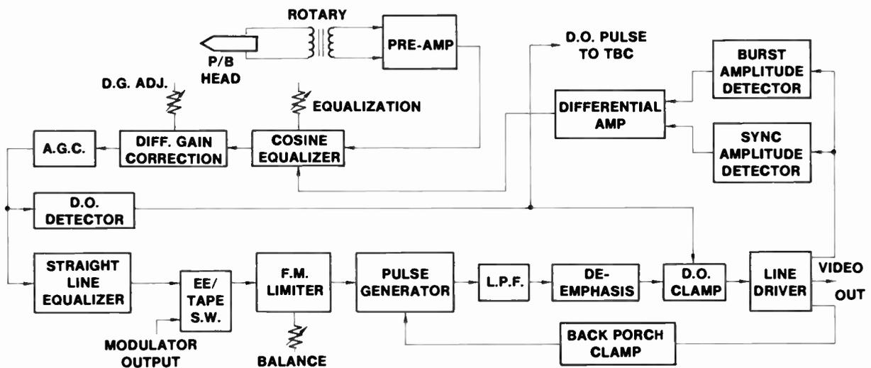
Figure 77 Single Head Playback System
