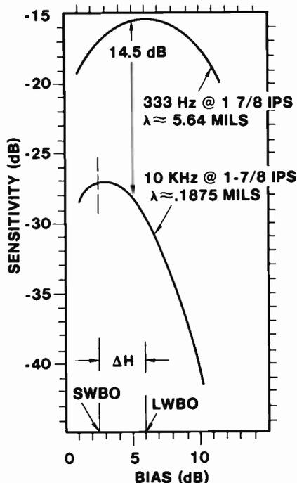
Fig. 14 Low Level Output Sensitivity of a.c. Bias for a Long and Short Audio Cassette
