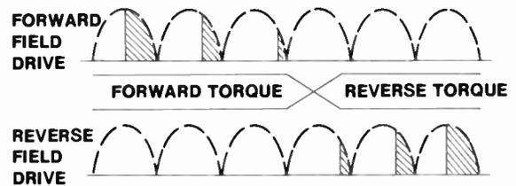
**Fig. 123 SCR Controlled Reel Motor Waveforms**
