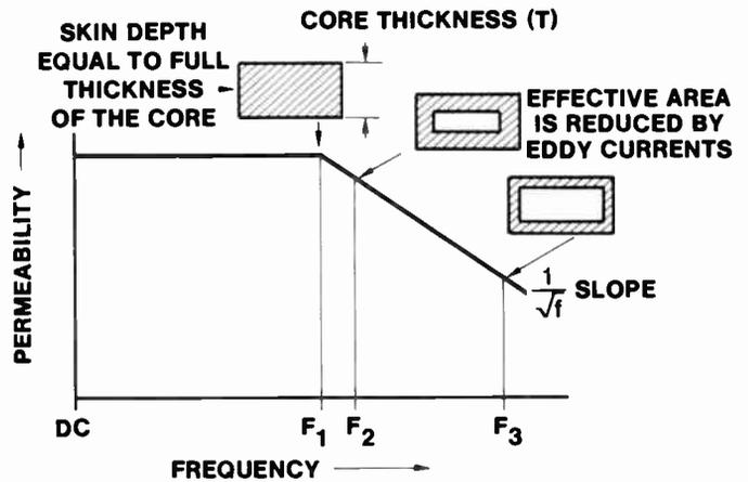
Figure 43 Effect of Eddy Currents on Permeability
