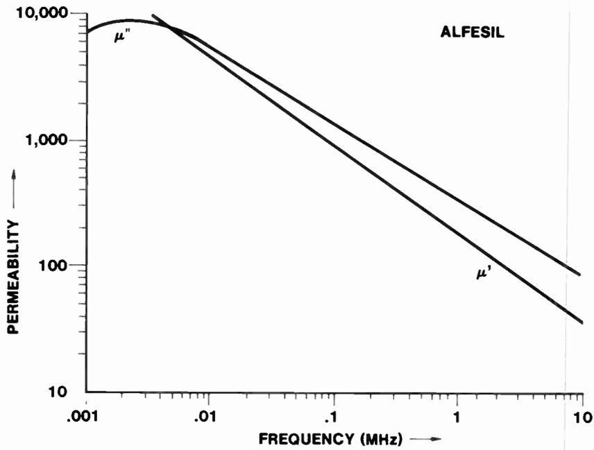
Fig. 46 Permeability vs. Frequency for Alfesil
