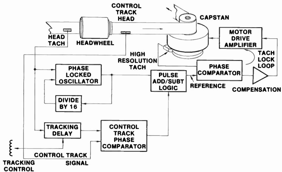
Fig. 115 Digital Capstan Servo for Quad
