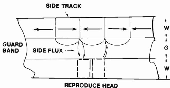
Fig. 19 Side Reading Flux Schematic
