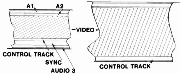
Fig. 112 Control Track Format on Tape
