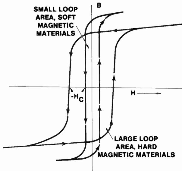
Fig. 27 B-H Loops for Hard and Soft Materials
