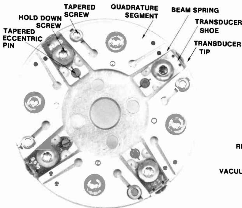
Fig. 97 Typical Head Wheel
