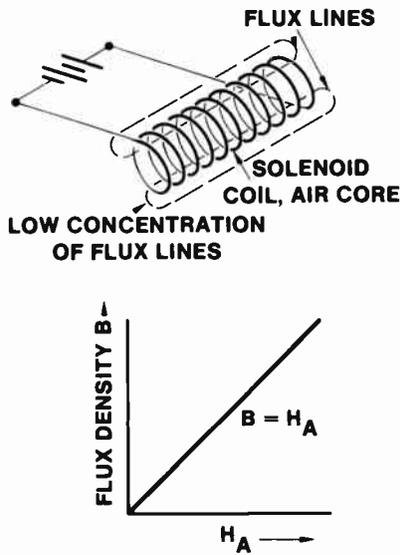
Fig. 23 Flux From Air Core Solenoid
