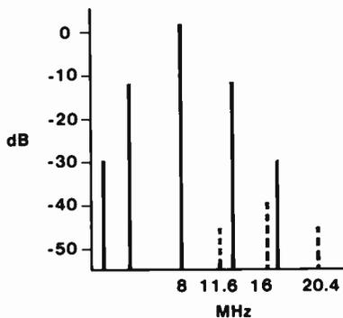
Fig. 70 FM Spectrum - 1% Second Harmonic Distortion
