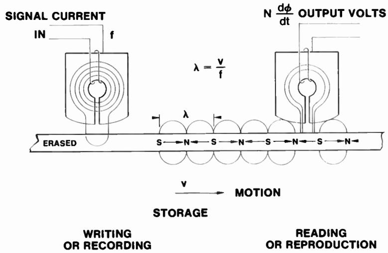
Fig. 15 Fundamental Recording and Reproducing Process
