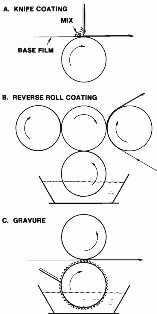
Fig. 58 Typical Coating Methods
