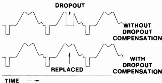
Fig. 86 Waveform Showing Without D.O.C. and with D.O.C.
