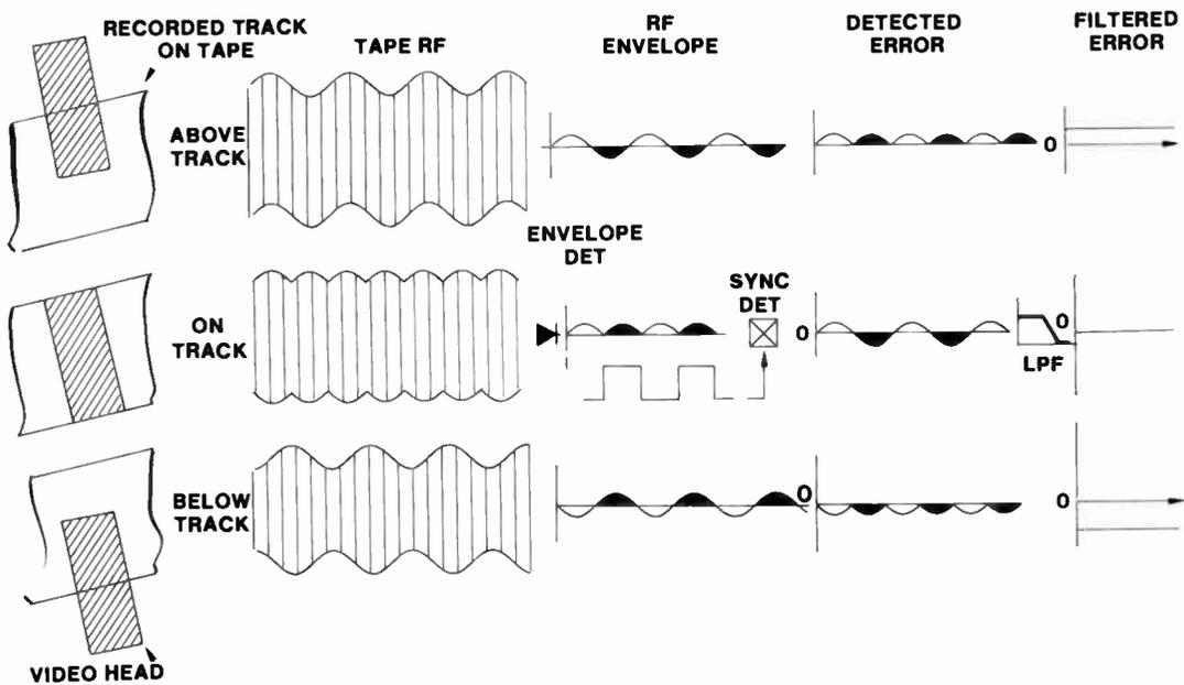
**Fig. 137 Synchronous Detection of Tracking Error**
