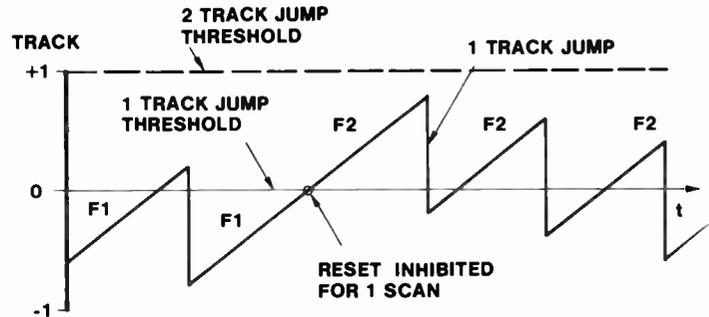
Fig. 139 Error Processing Output for 1/5 Speed Forward Mode
