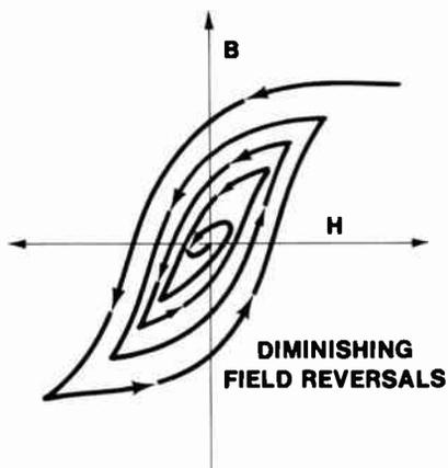
Fig. 37 Demagnetization by Reversals
