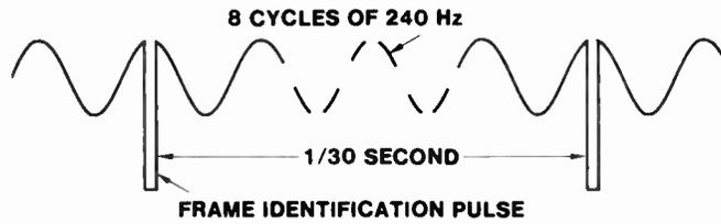
Fig. 113 a) Quad Control Track Record Waveform
