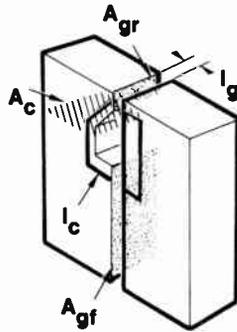
Fig. 47 Physical Parameters of Video Core
