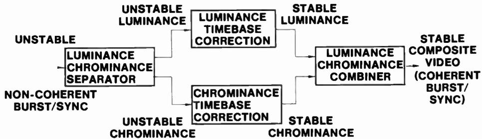
Fig. 93 Timebase Correction of Color-Under Signals
