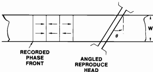
Fig. 17 Azimuth Misalignment Geometry
