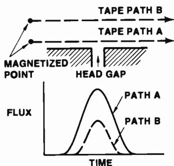
Fig. 67 Independence of timing From Head/Tape Spacing
