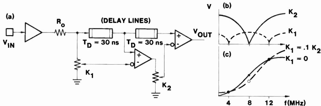
**Fig. 80 Aperture Correction by Cosine Equalizer - Two Delay Line Method**
