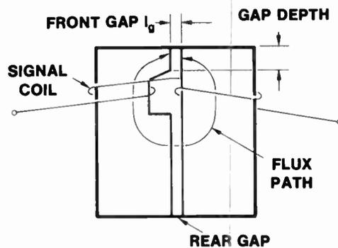
Fig. 39a Plan View of Record Head
