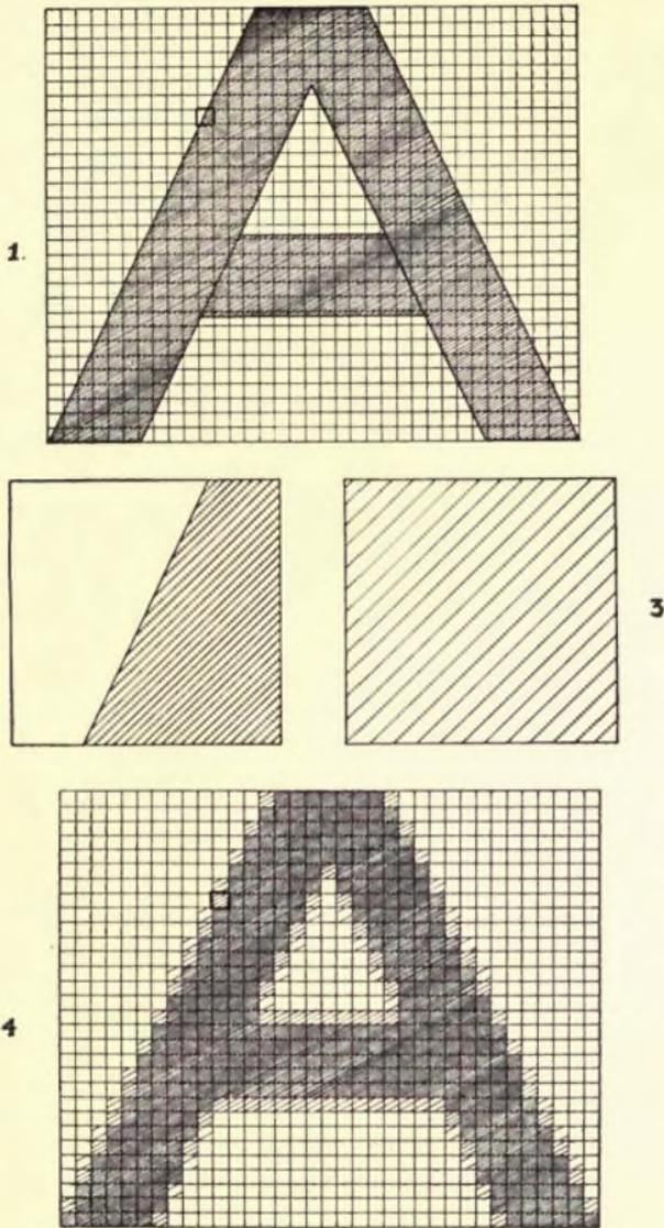
FIG. 6—The upper figure represents a letter “A” analyzed into 30 lines of 35 picture elements each. Some picture elements will be white, some black; but some—as in small square—will be partly white and black. An enlargement of this small square is shown at 2, while 3 shows the same square as it would appear on a television receiver. The complete letter “A” as it would appear on a television receiver is shown in 4.
