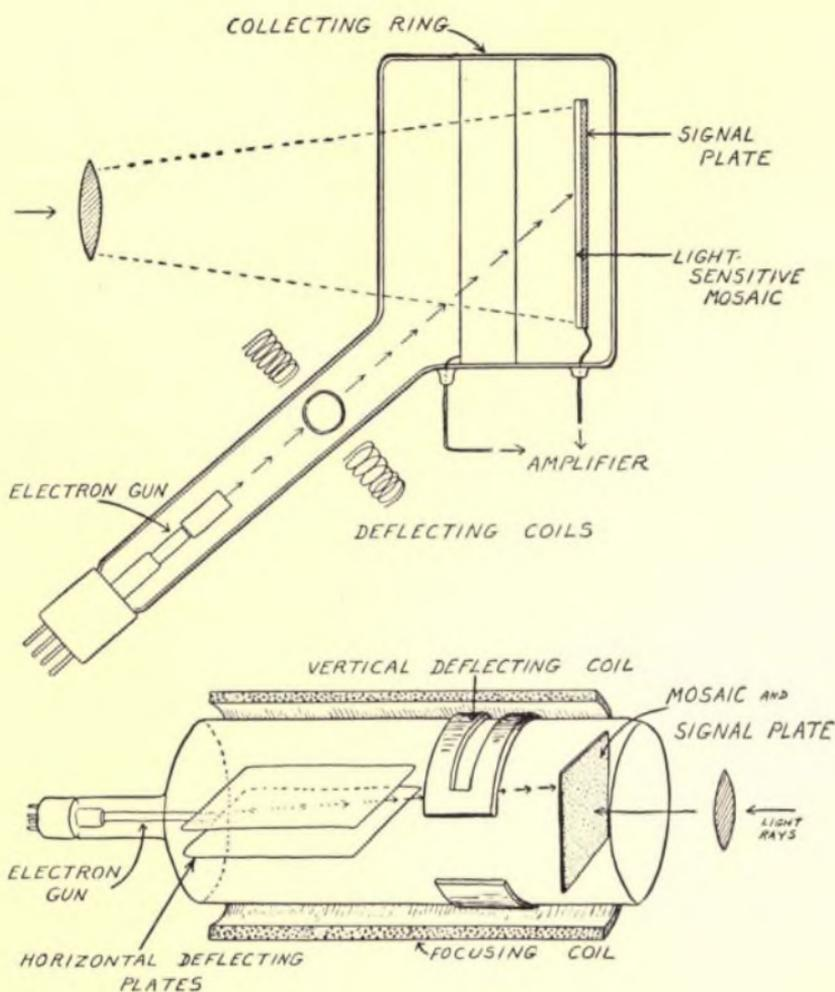
FIG. 33—Cathode ray tubes used in television cameras. Upper figure the iconoscope type, lower figure the orthiconoscope type. In both, a moving electron beam, guided by deflecting coils, scans the electron image produced upon the light-sensitive mosaic; this creates a sequence of electric impulses upon the signal plate behind the mosaic, which leave the tube as the television signals.
