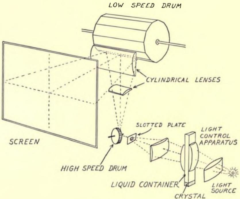
FIG. 12—The mechanical television system in use by Scophony Ltd. A high speed and a low speed mirror drum scan the image into lines and picture elements.
