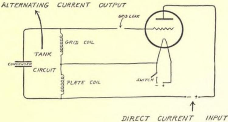
FIG. 23—Use of a vacuum tube as an oscillator, converting direct current into alternating current.
