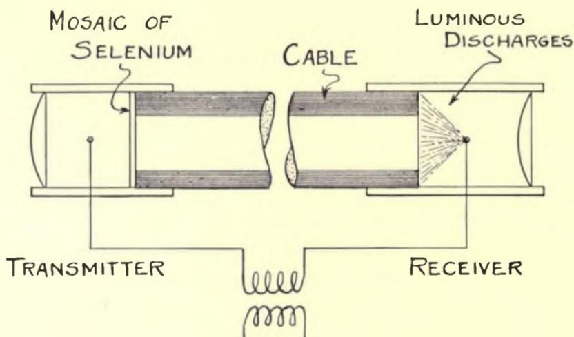
FIG. 5—Representation of the Morse system for simultaneous transmission of picture elements of a television image. 1893.
