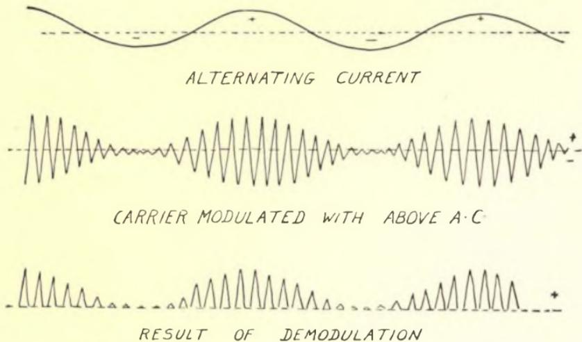
FIG. 24—Amplitude modulation of a carrier current.
