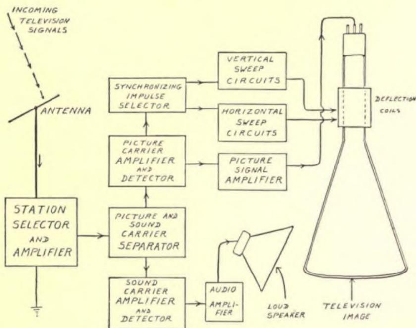
FIG. 53—Plan of a television receiver.
