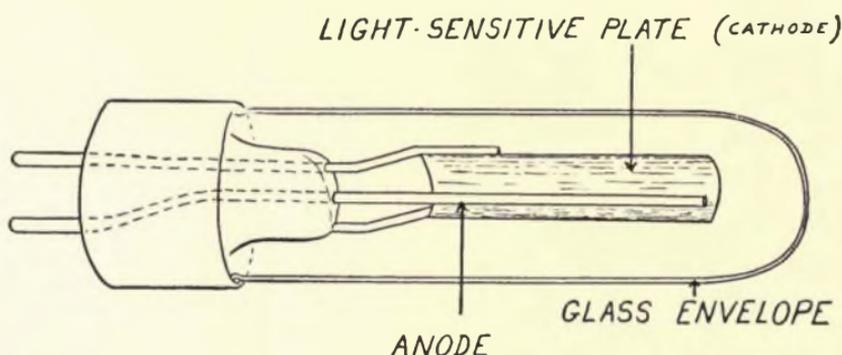
FIG. 3—Construction of a photoelectric cell.
