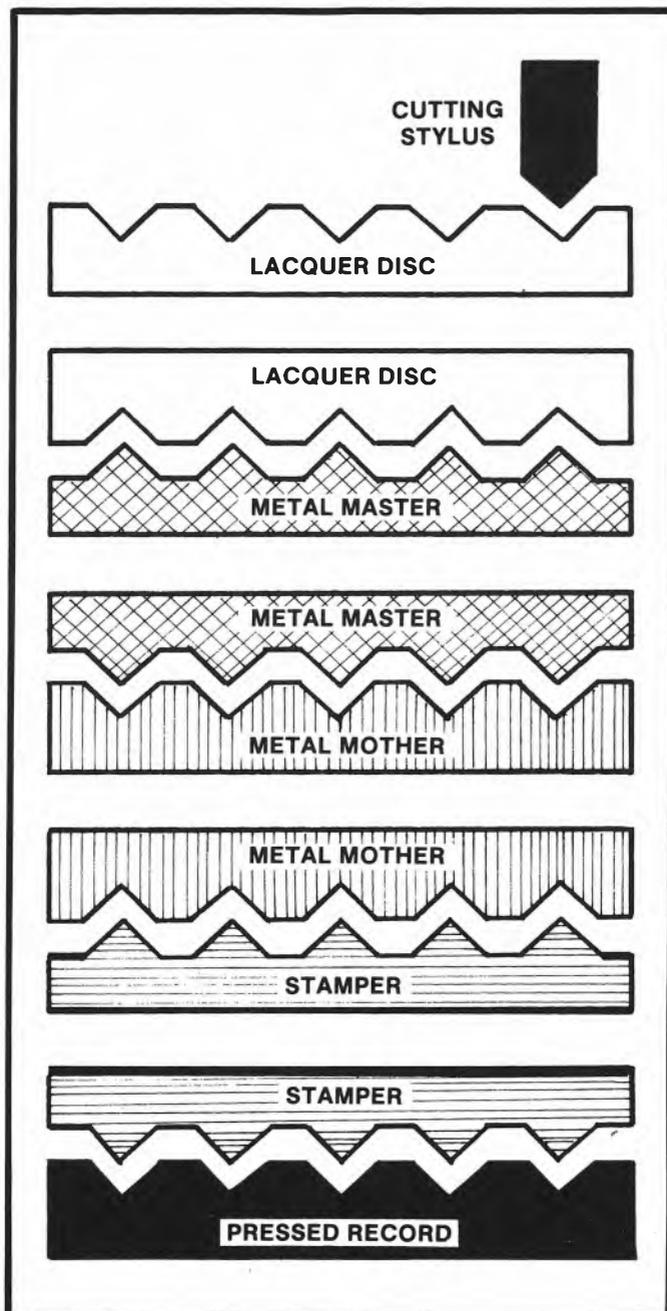
The various stages in the pressing process. Noise and other flaws can be introduced at any stage.
