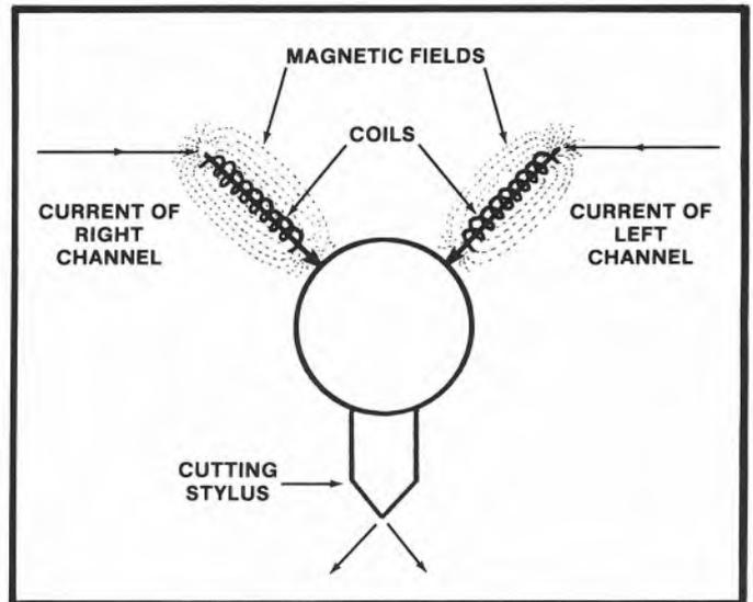
Simplified view of a stereo cutterhead.
