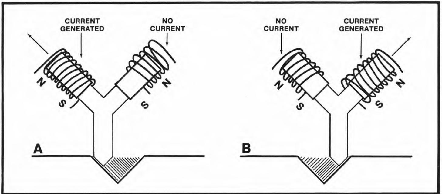
A playback stylus translates the stereo groove back into two distinct signals. "A" shows right channel output; "B" shows left channel output.
