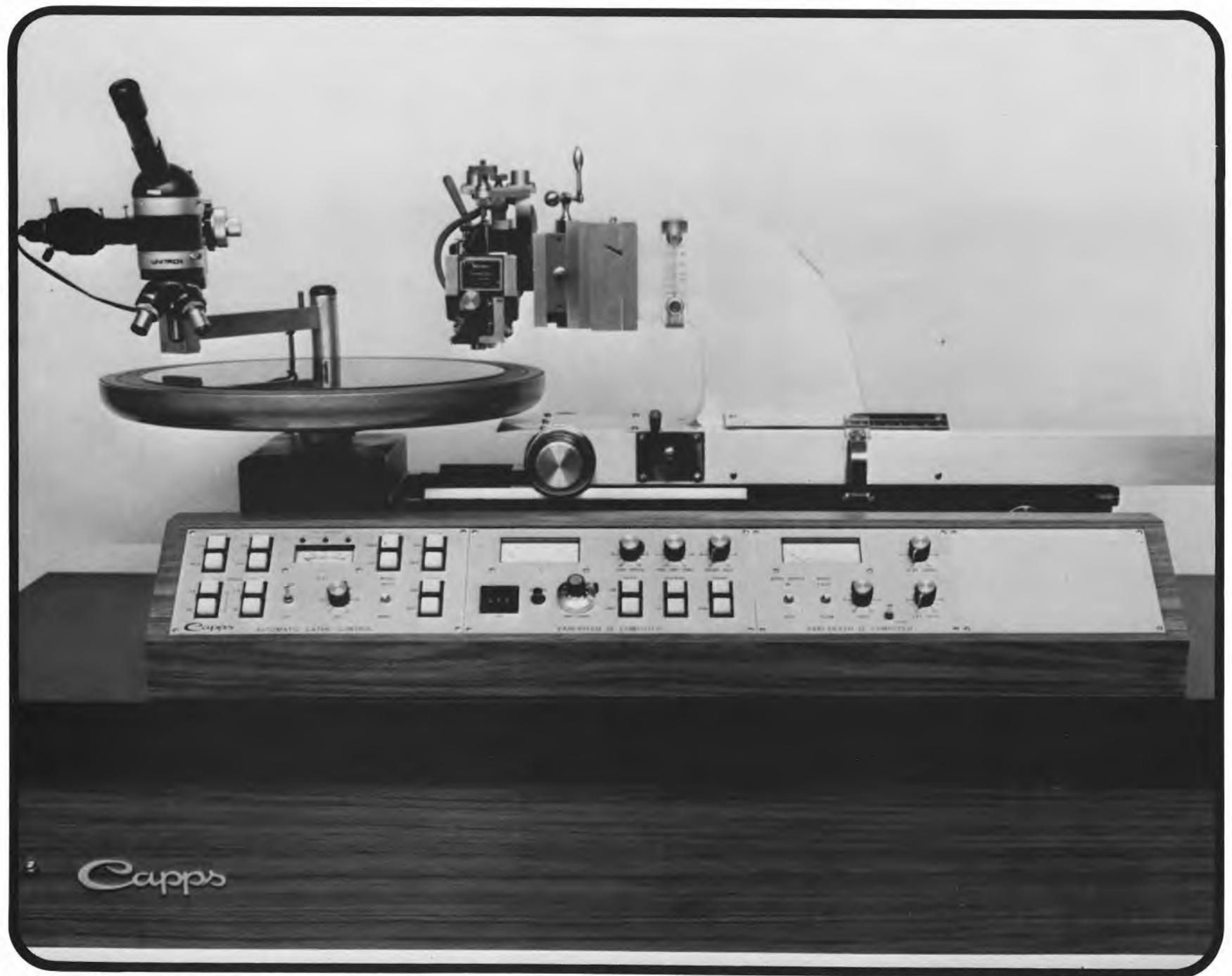
A Scully Lathe (same as on Page 6) but fitted with a new, highly sophisticated pitch and depth computer by the Capps Co. (Manufacturer's photo)
