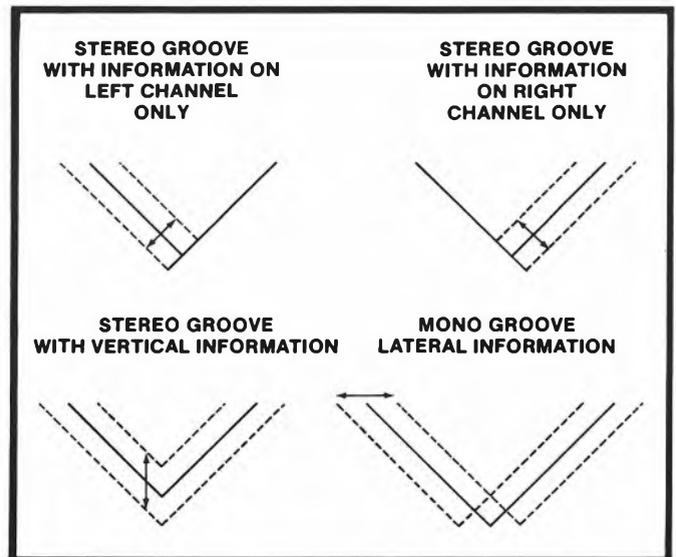
Westrex kept the 90° relationship of lateral to vertical but rotated the axis 45° to the plane of cut. This system made **physical** compatibility a reality. In addition, rumble is generally more pronounced in the vertical plane. The 45/45 system rumble is identical in both channels and lower by about 3 DB overall.
