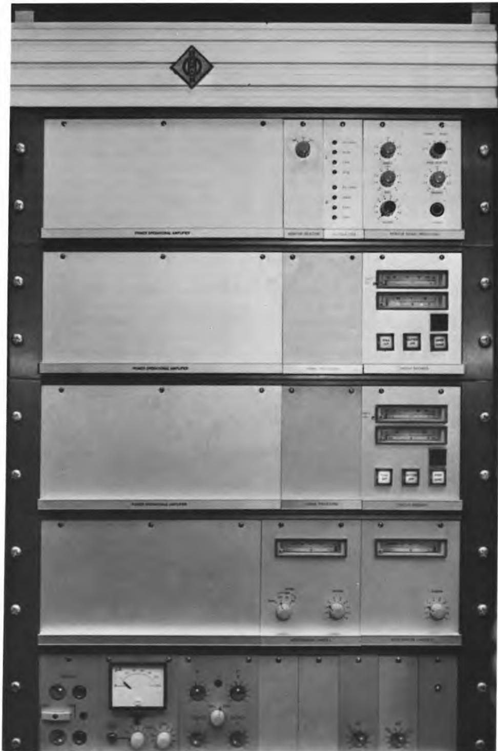
The output of the Mastering Console is fed into the cutting amplifiers, which in turn drive the cutterhead.
