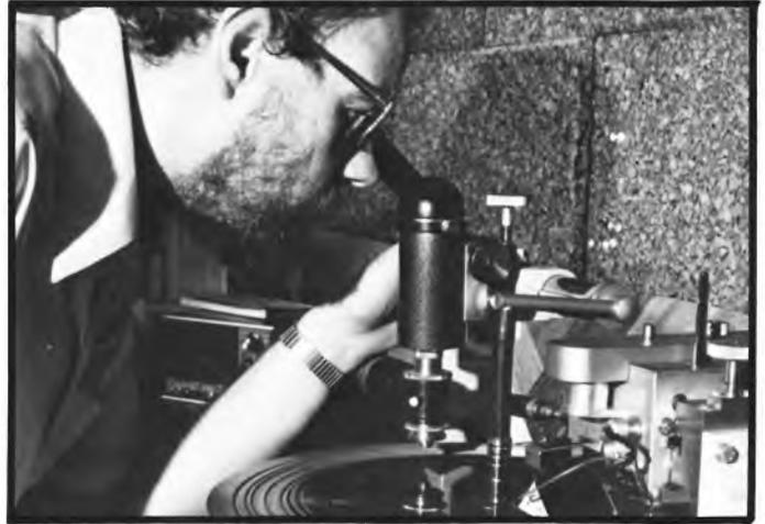
Each disc is spot-checked through the microscope after cutting.
