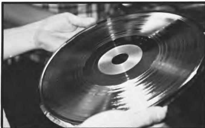
**A stamper ready to go to press. Note carefully punched center hole and fluted edge.**
