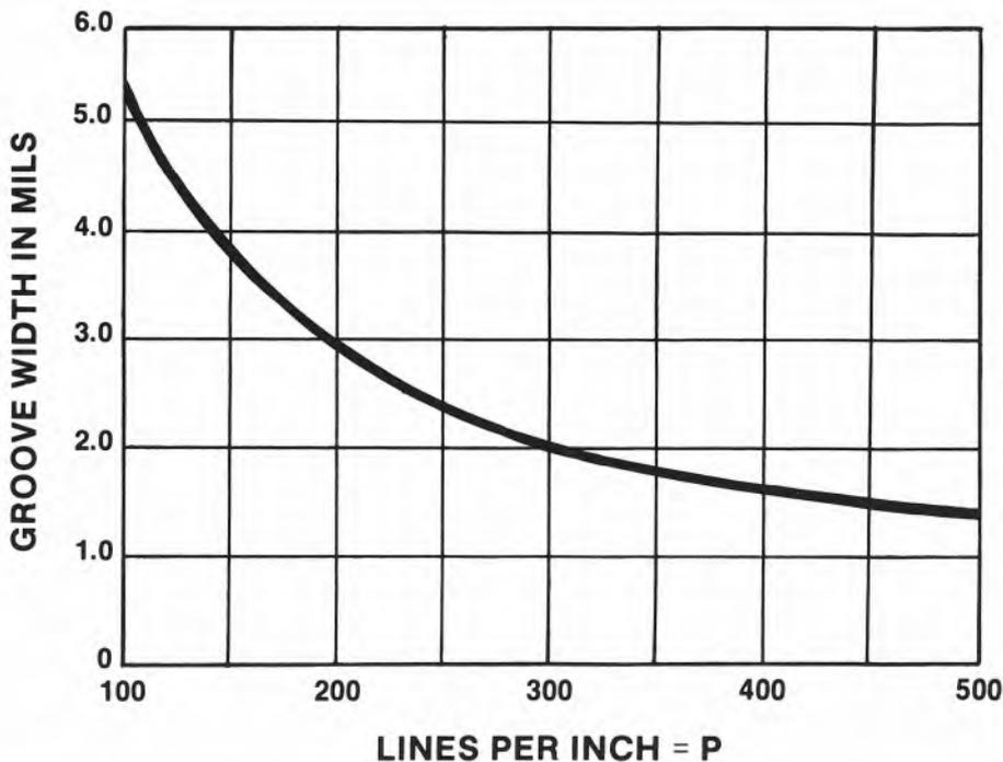
Groove width versus lines per inch. Average groove width =  $\frac{\frac{1000}{P} + 1}{2}$
