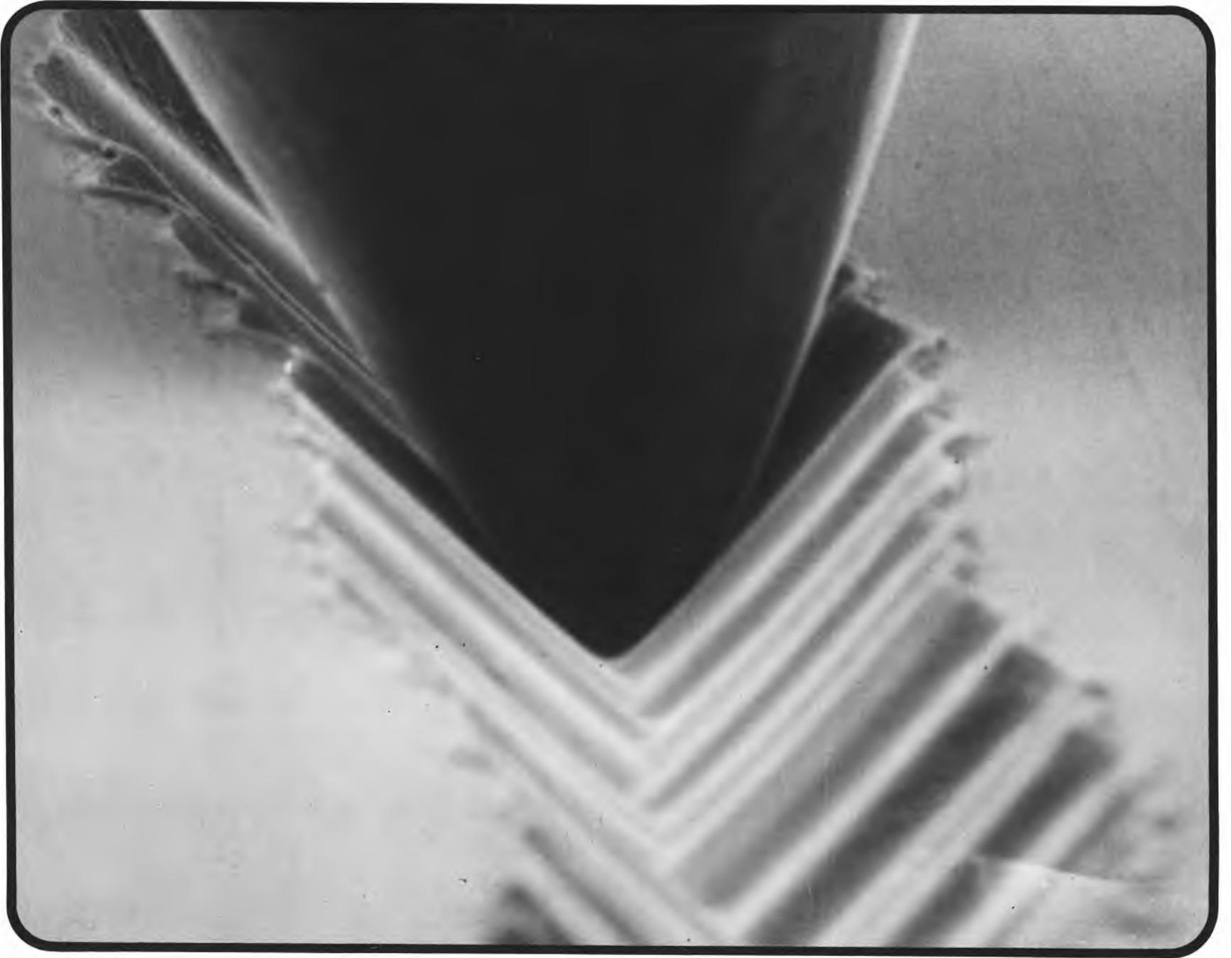
**This photo shows just how hard a task the playback stylus has. Failure to completely trace out each and every groove undulation will result in distortion (1,000 magnification). (Photo courtesy of Stanton Magnetics)**
