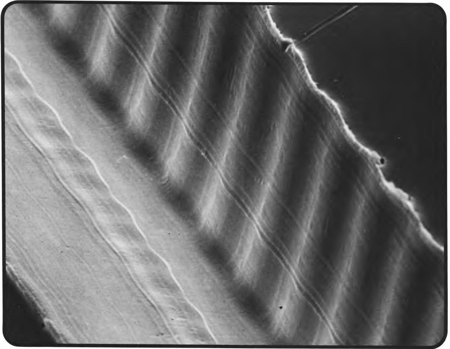
A test record after 100 plays. Note 20KHZ modulation on right groove wall, none on left (10,000 magnification). Groove wear is clearly evident. (Photo courtesy of Stanton Magnetic)
