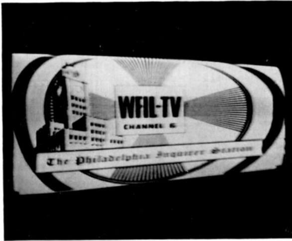
FIG. 18-41. Trapezoidal raster caused by defective deflection yoke. Keystoning at top and bottom shown here produced by shorted vertical coil. Keystoning at sides can be caused by shorted horizontal coil. (RCA.)
