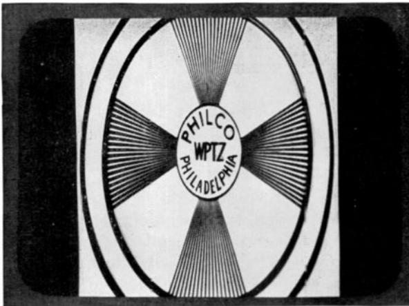
FIG. 17-22. Insufficient width. (*Philco Corporation.*)
