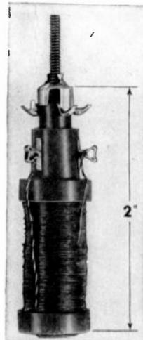
FIG. 18-25. Horizontal-linearity-control coil. Slug inside the coil varies the inductance from 1 to 8 millihenrys, approximately. (RCA.)
