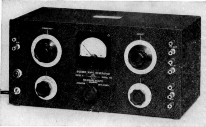
FIG. 12-17. Square-wave signal generator. Frequency range is 5 to 100,000 cps. (Measurements Corporation.)
