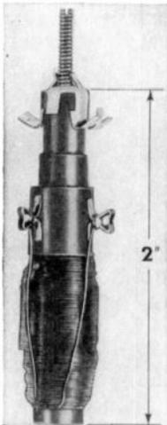
FIG. 18-24. Width-control coil. Slug inside the coil varies the inductance from 3 to 16 millihenrys, approximately. (RCA.)
