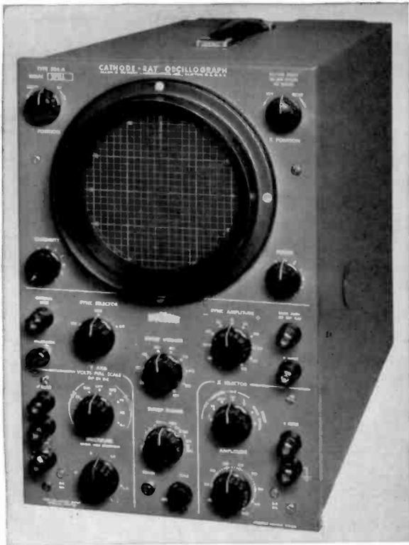
FIG. 23-10. Typical 5-in. oscilloscope. Frequency response of vertical amplifiers is from d-c to 100 kc within 1 db. Internal-sweep frequency range 2 to 30,000 cps. (Allen B. DuMont Laboratories, Inc.)
