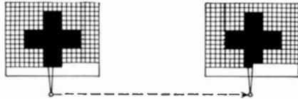
FIG. 1-2. Reproducing a picture by duplicating the picture elements.
