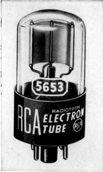
FIG. 2-3. A typical vacuum phototube. The average cathode current for such a tube is several microamperes with an anode voltage of 100–250 volts. (RCA.)
