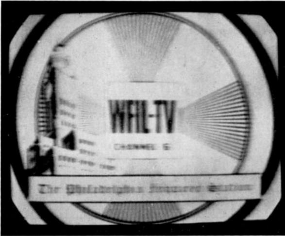
FIG. 11-10. Test pattern illustrating loss of high video frequencies. Note the lack of separation of the divisions in the top and bottom wedges. Also, they are weaker in intensity than the side wedges. (*RCA Pict-O-Guide.*)
