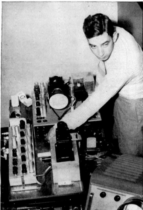
FIG. 2-7. Flying-spot camera pickup using flying-spot cathode-ray tube 5WP15. (RCA.)
