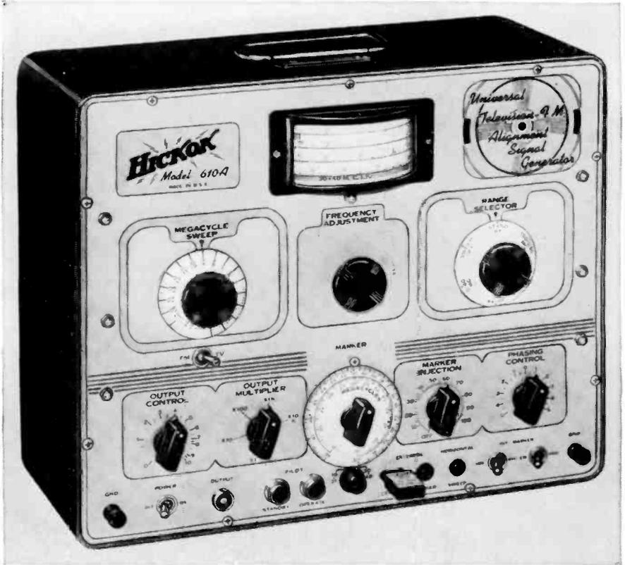
Fig. 19-16. TV sweep generator for alignment. R-f range 30 to 230 Mc; output up to 0.5 volt; 4.5 Mc crystal for intercarrier-sound i-f alignment; sweep width 15 Mc or 1.5 Mc; sweep rate 60 eps; marker absorption dip or oscillating pip frequency range 19 to 48 Mc. (Hickok Electrical Instrument Company.)
