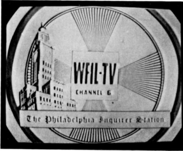
FIG. 11-11. Test pattern illustrating loss of low video signal frequencies. Background is weak, lettering is not solid, and side wedges are weaker in intensity than vertical wedges. (*RCA Pict-O-Guide.*)
