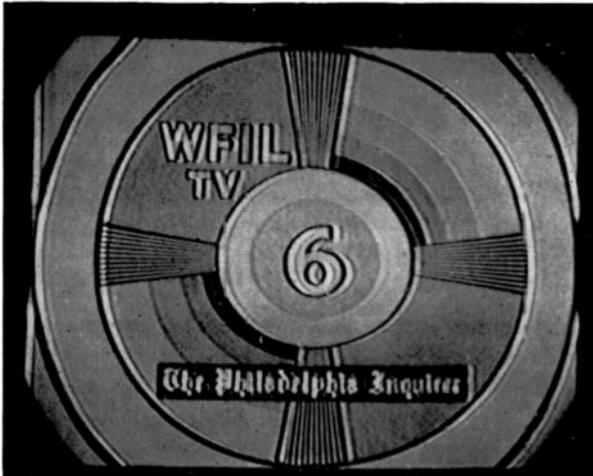
FIG. 11-29. Test pattern with outline distortion caused by ringing in the video amplifier. (RCA Pict-O-Guide.)
