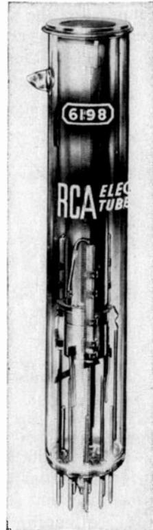
FIG. 2-13. The vidicon camera tube. It is  $6\frac{1}{4}$  in. long and 1 in. wide, approximately. (RCA.)
