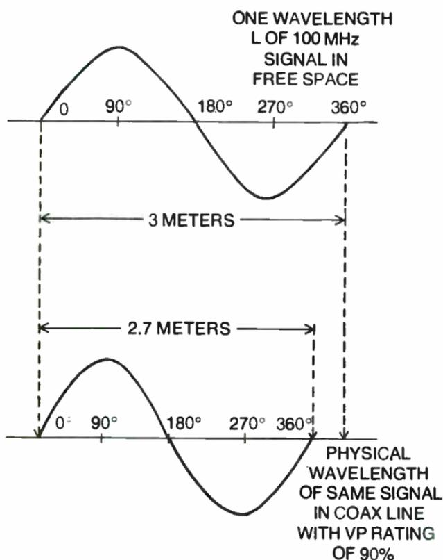
Fig. 10-1. The wavelength of the RF signal is shorter in the coax line than it is in free space. How much shorter is a function of the velocity-of-propagation (VP) factor of the line.
