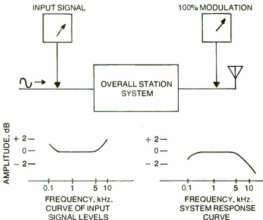
Fig. 14-1. A plot of the input signal levels for different tones while holding the output of the system constant will describe a curve exactly opposite that of the system response.
