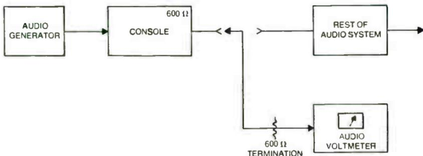
Fig. 14-8. Use the audio voltmeter to measure output of each unit in chain. Add proper termination to input of voltmeter.
