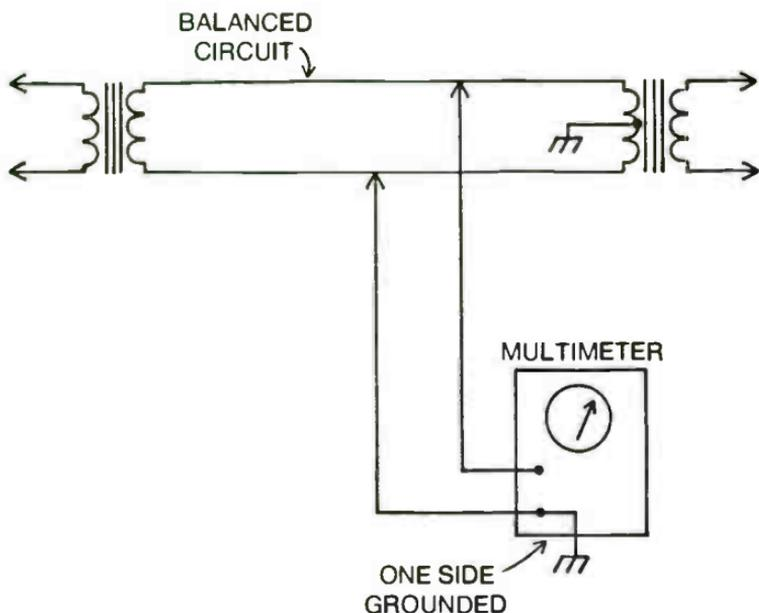
Fig. 13-5. The unbalanced input of meter can short out half of a balanced circuit. This will affect both the circuit and the readings. To avoid this, float meter case.
