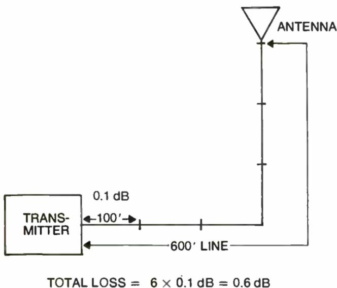
Fig. 10-3. Compute the loss for the total length of line, not just the 100-foot section.
