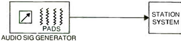
(C) WITH A GAIN MEASURING SET CONTAINING CALIBRATED PADS AND METERING
