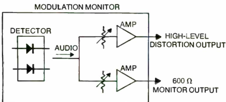
Fig. 14-12. The distortion output of the monitor often uses different circuitry than the audio monitor output.
