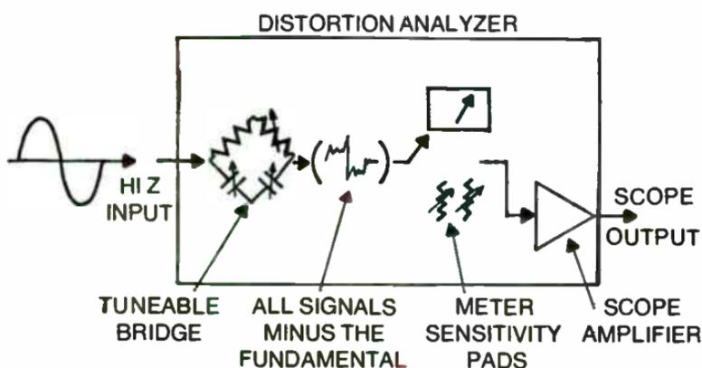
Fig. 14-5. Basic distortion analyzer. Bridge circuit cancels the fundamental tone, and the meter reads everything remaining, including noise. Analyzer will also contain an amplifier to feed an oscilloscope the same information the meter is indicating.
