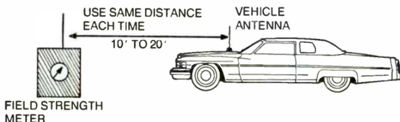
Fig. 7-7. Use a kit-type field-strength meter to measure radiated power. Do the procedure the same way each time.
