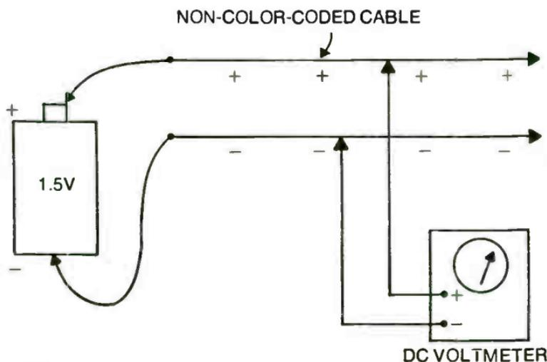
Fig. 13-9. Use a flashlight battery and voltmeter to identify the wires in an uncoded cable.
