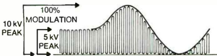
Fig. 14-7. In AM, the peak positive voltage at 100% modulation is twice that of the unmodulated carrier. Incorrectly set ball gaps will arc over.
