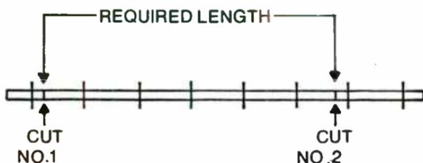
Fig. 10-7. Avoid cutting at the spacers on the inner conductor. If necessary, move the measurement down the line and make a cut at both ends.
