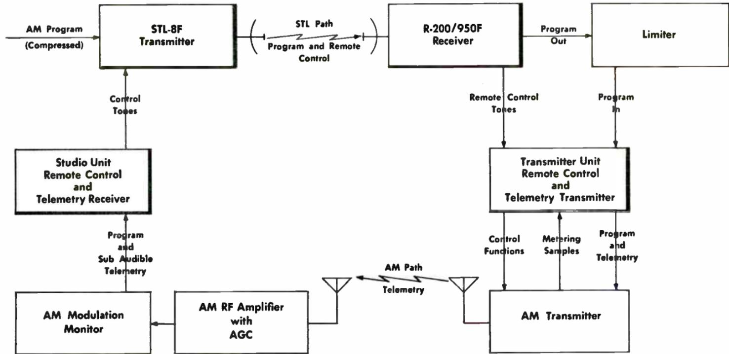
Fig. 7-17. Full over-the-air remote control for AM radio. (Courtesy Marti Electronics, Inc.)
