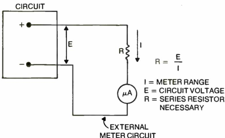
Fig. 13-6. When adding a panel meter to make a voltmeter, add enough series resistance to limit current through meter and drain from circuit. Use Ohm's law to figure resistance.
