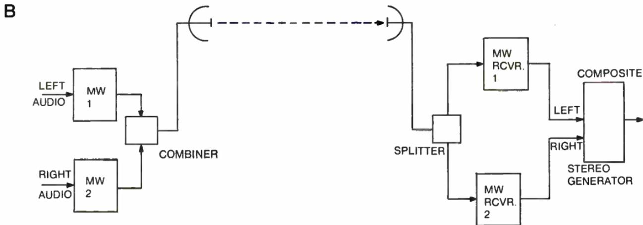
Fig. 7-19. Two ways to send stereo over the STL in A, as composite, in B, as the left and right audio.
