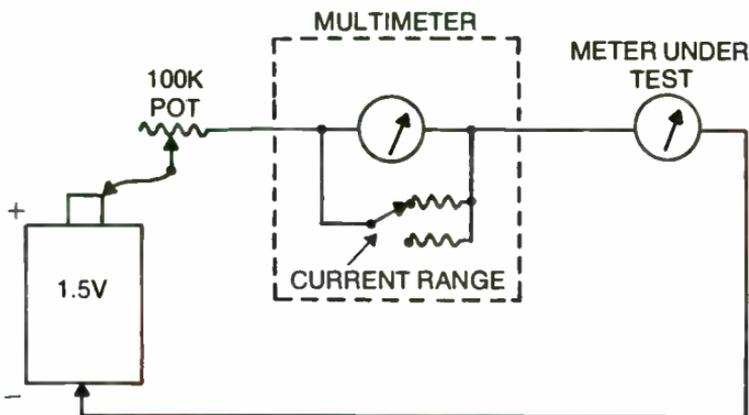
Fig. 13-4. To check unknown scale of a meter, use the ammeter section of a multimeter as a comparison. Start with a high-resistance value in the pot.
