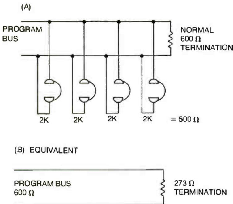
Fig. 4-18. Impedances in parallel figure the same as resistors. Here, the four earphones will cause double loading of the bus.
