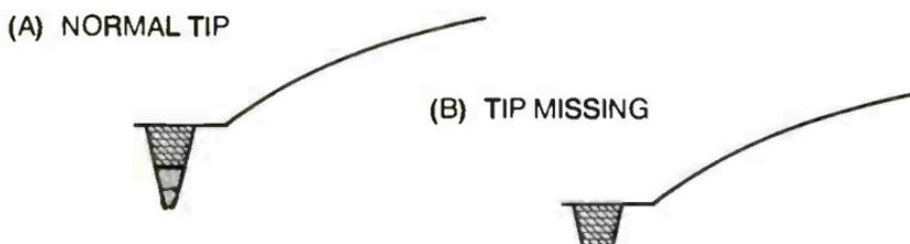
Fig. 5-12. Inspect the stylus with a microscope. If the tip of the stylus is missing, it will cause distorted sound and damage the records.
