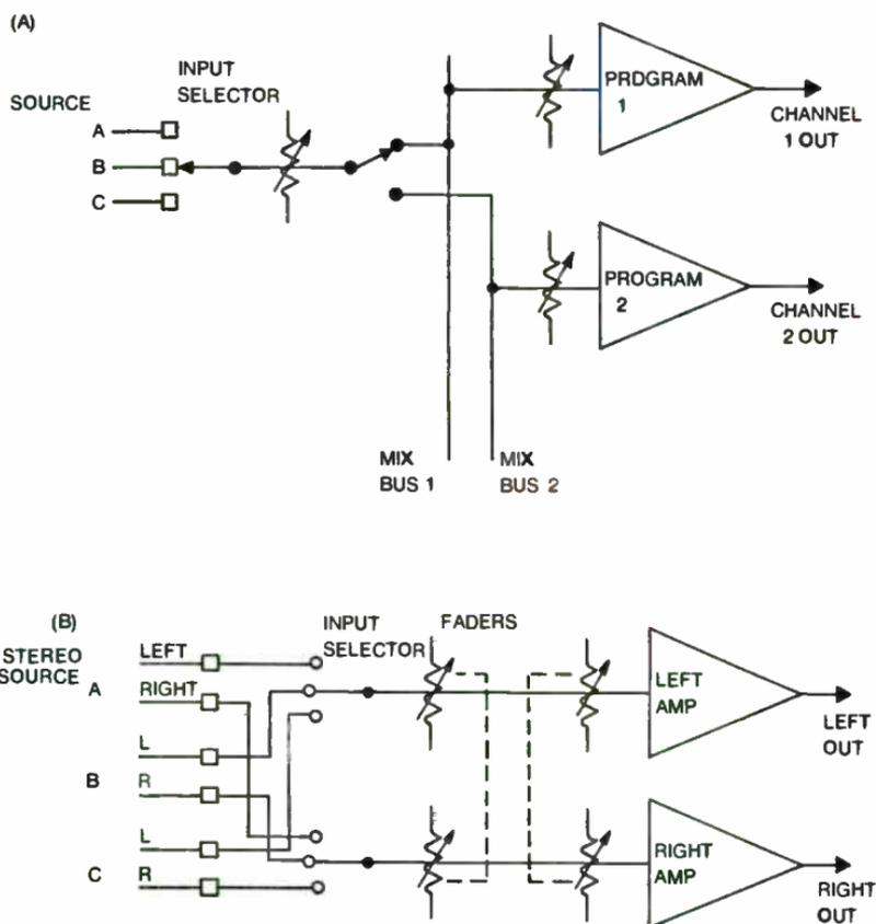
Fig. 5-3. (A) The dual-channel console selects and switches a source to either of two channels. (B) The stereo console selects the left & right channels of a source and carries this all the way through to the output.
