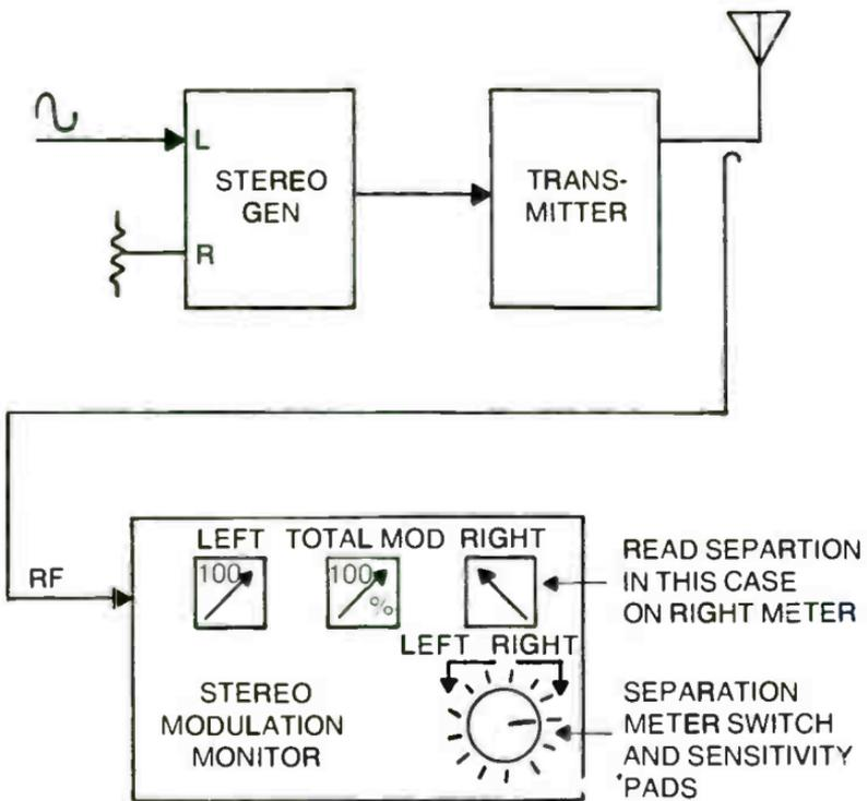
Fig. 1-20. Measure separation according to the monitor in use. Shown is a typical monitor measuring the separation of the right channel from the left channel.
