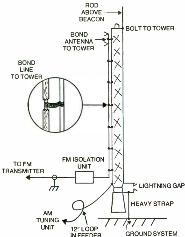
Fig. 11-10. Standard lightning protection.
