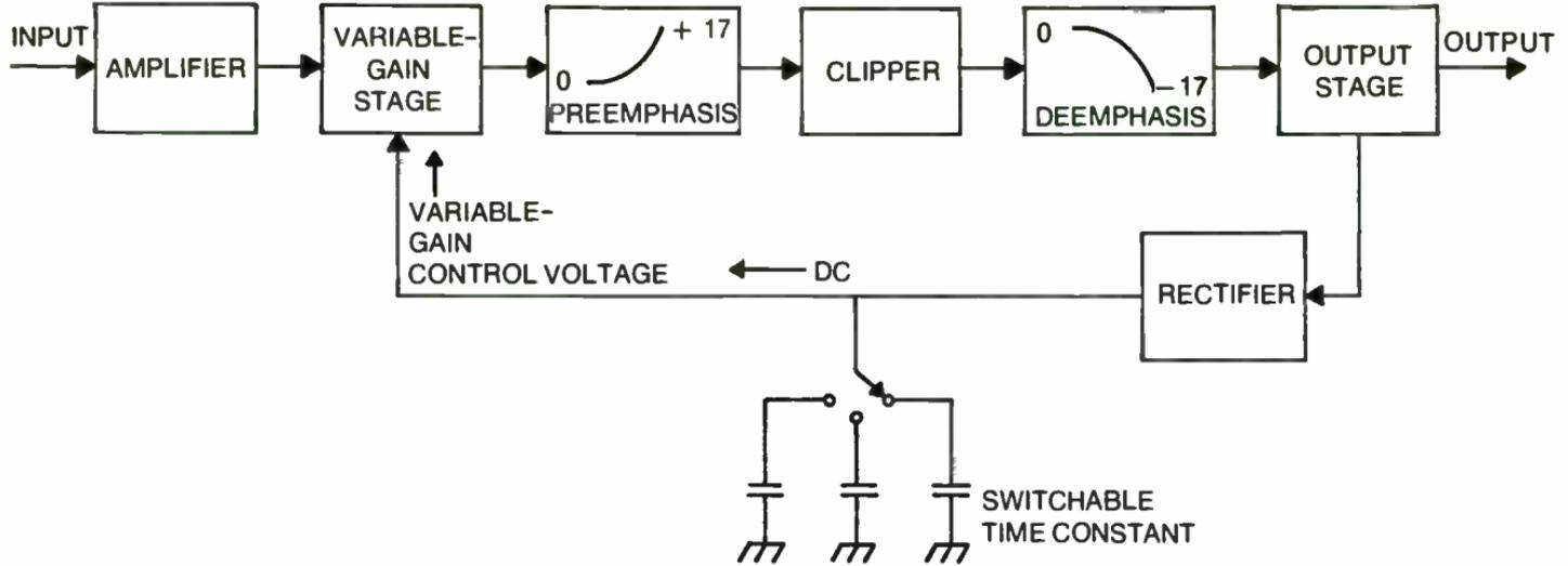
Fig. 9-7. The typical FM limiter also reshapes the audio to conform with 75  $\mu$ sec curve, clips above the curve, and restores to a flat response.
