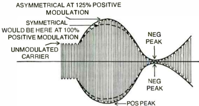
Fig. 9-6. Asymmetrical amplitude modulation. The positive and negative modulation peaks are unequal. Symmetrical modulation would have both peaks equal.
