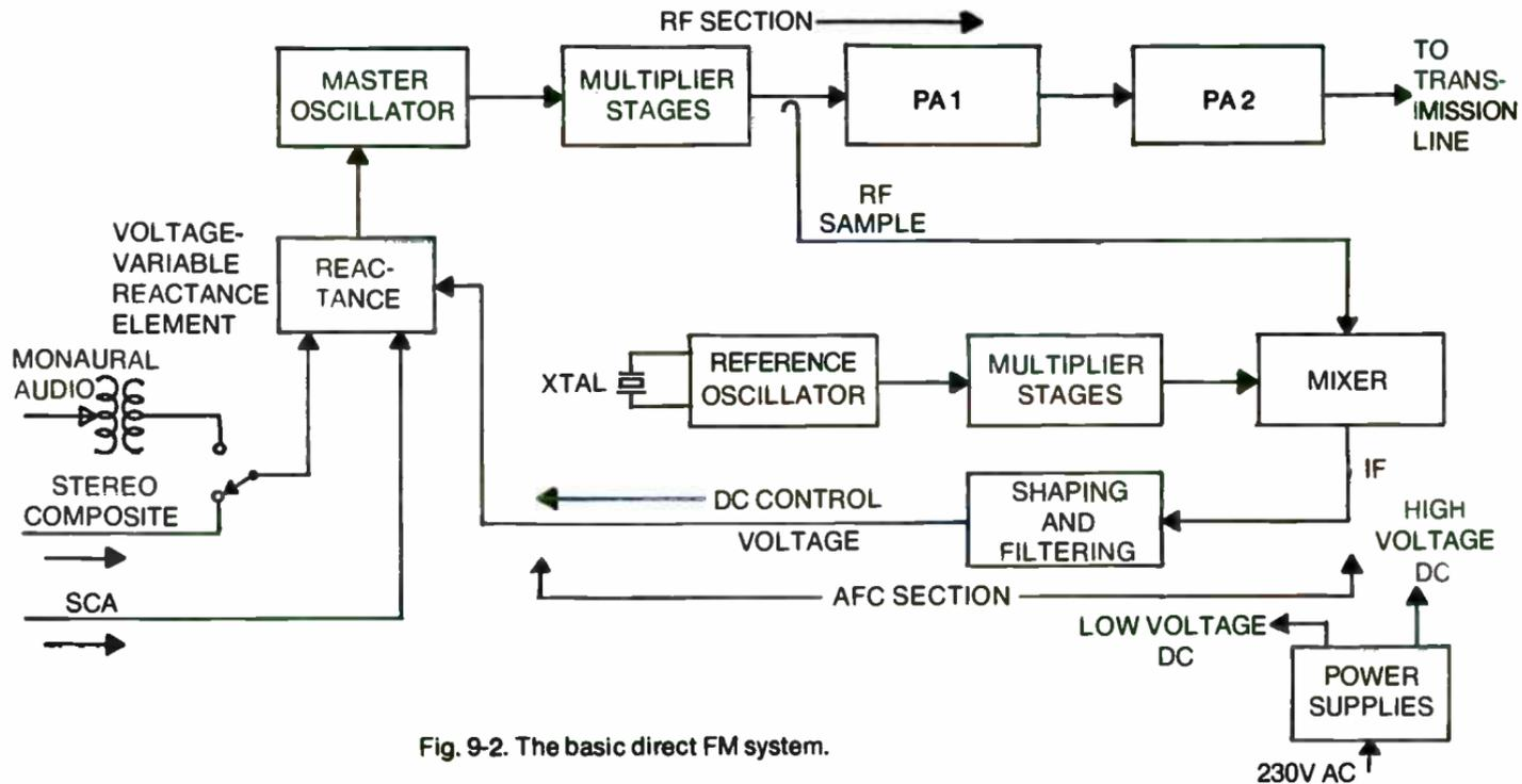
Fig. 9-2. The basic direct FM system.
