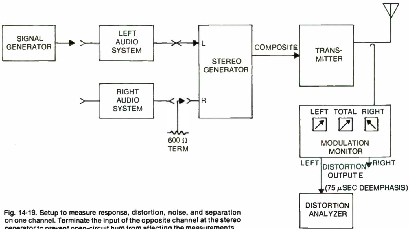
Fig. 14-19. Setup to measure response, distortion, noise, and separation on one channel. Terminate the input of the opposite channel at the stereo generator to prevent open-circuit hum from affecting the measurements.
