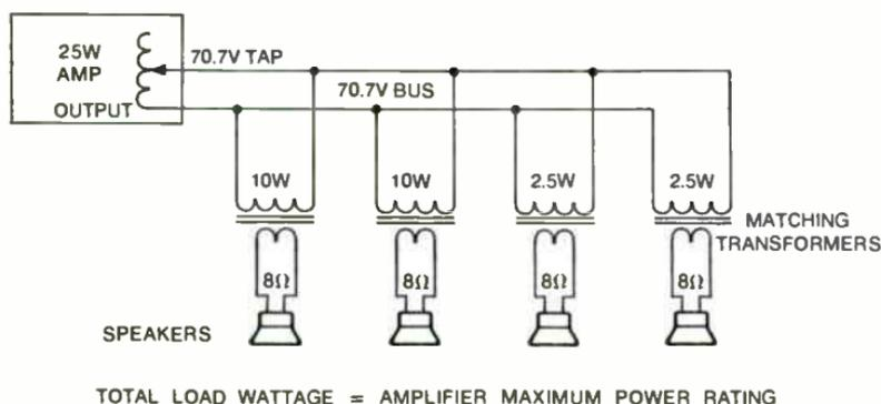
Fig. 6-12. The 70.7V distribution system. Matching transformer primaries are marked in power taps.
