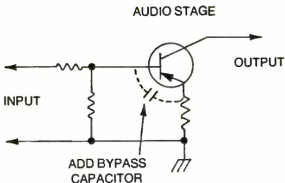
Fig. 4-25. Bypass the emitter to base at the transistor if this won't upset stage.
