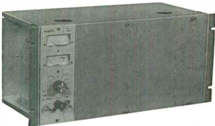
**Fig. 7-14.** The station may use a microwave unit instead of telephone lines for the interconnecting link. Shown is the Marti STL-8F transmitter unit, operating in the 950 MHz band.
