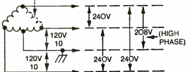
Fig. 3-12. Typical open-delta secondary connections for a 3-phase system. One transformer provides a 120V single phase. Voltages shown are the design parameters.
