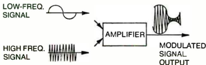
Fig. 4-14. Intermodulation distortion is a modulation process—not mixing.
