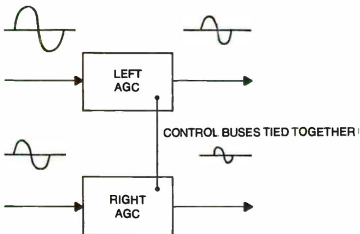
Fig. 9-9. Stereo AGC amplifiers or peak limiters should have the pairs synced together. The channel with the highest levels will control both channels.
