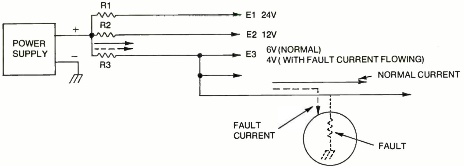
Fig. 4-15. Fault in circuit can increase current through R3, causing a higher voltage drop and lowering voltage bus E3. All circuits fed by E3 will be affected.
