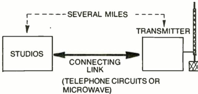
Fig. 1-3. A separated studio-transmitter arrangement. This is the most complicated and entails considerably more equipment and maintenance difficulties.
