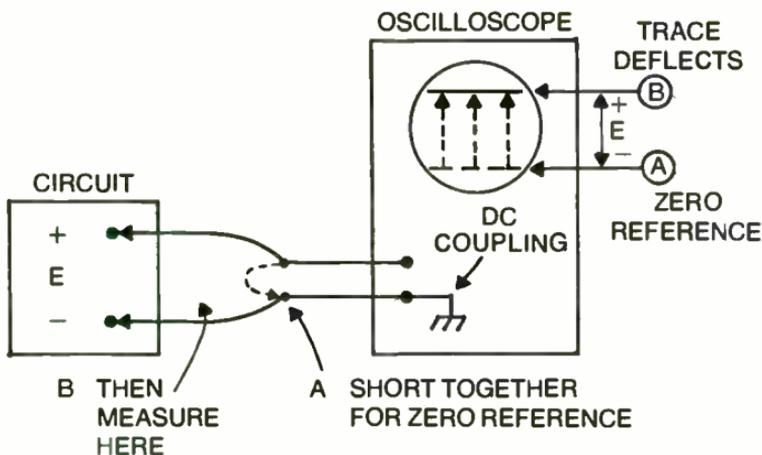
Fig. 13-7. Making DC voltage measurement with the oscilloscope. Use DC coupling and short the probe to ground for reference. Distance between zero reference and deflection of trace is directly proportional to the DC voltage.
