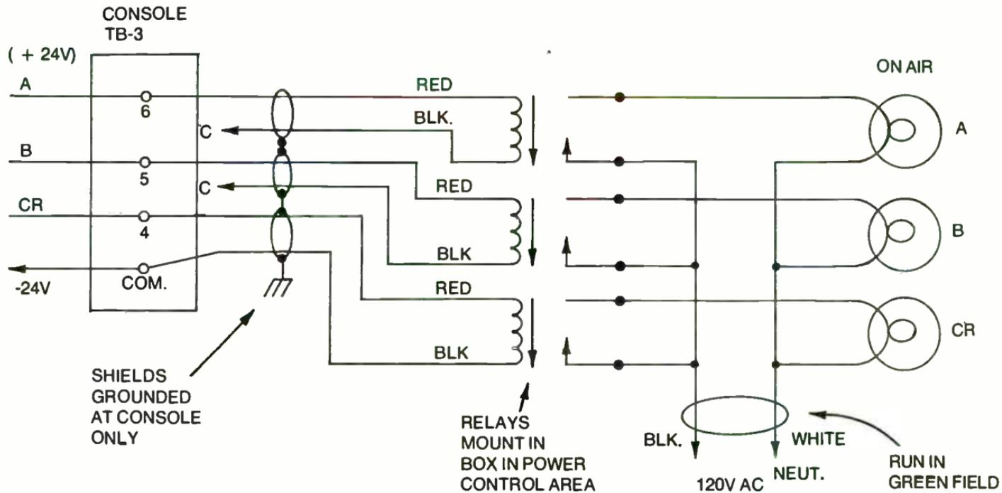
Fig. 3-2. Schematics are needed for specific sections to show the necessary installation data. Notice the information on shields, parts location, and other data.
