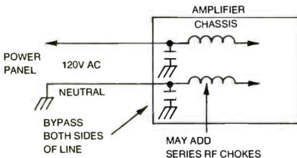
Fig. 4-28. Even though neutral is grounded at the power panel, treat AC power circuits as balanced circuits for RFI.
