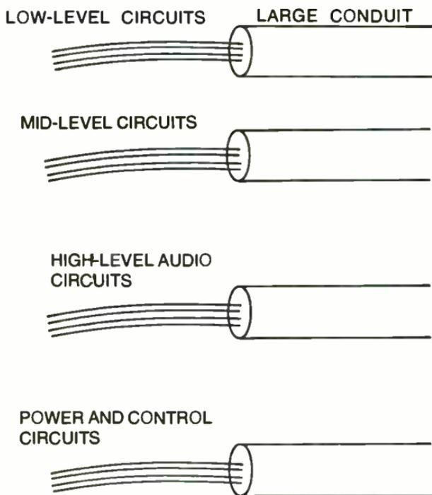
Fig. 3-7. Segregate cables by signal levels.
