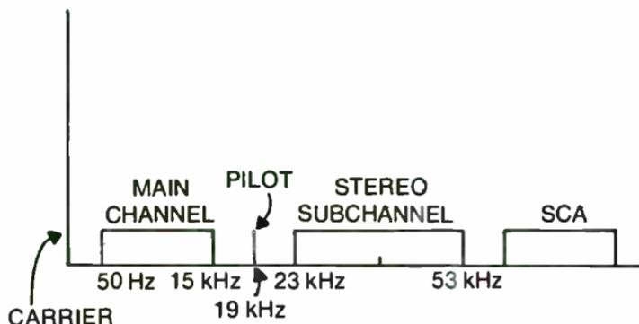
Fig.14-21. The sideband spectrum of composite modulation of the FM carrier. Crosstalk is the spillover of spurious and harmonic elements from the main channel into the subchannel, or the subchannel into the main channel.
