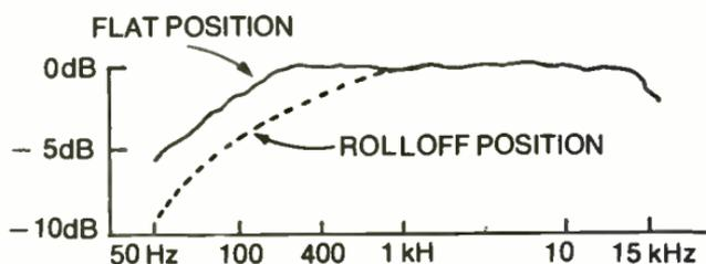
Fig. 5-7. Typical selective response curve of a cardioid microphone. When switched to its rolloff or cut position, the low frequencies are rolled off. This is useful in reducing unwanted, low-frequency room noises.
