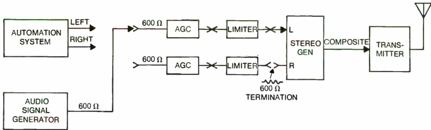
Fig. 14-14. For full-time automated stations, feed the test generator to the same point where the automation feeds the system.
