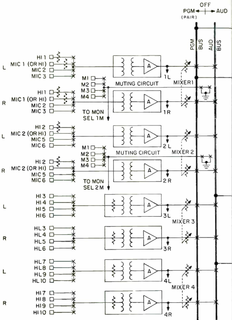
Fig. 5-2. Block diagram of the RCA BC-15 console.
