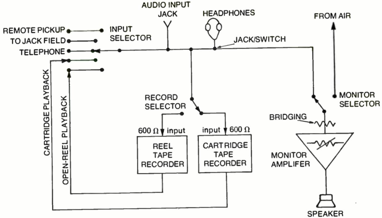
Fig. 6-1. Simple switching arrangement that can be built for the newsroom.
