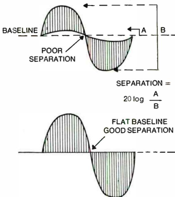
Fig. 14-18. Check the separation of the stereo generator with a scope. Feed left or right channel. Base line should be flat for good separation. Adjust separation controls on stereo generator to flatten baseline.
