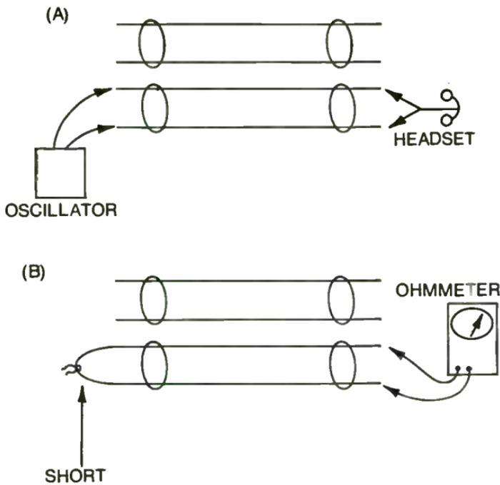
Fig. 3-15. Two different ways to ring out the cables. In A, an audio oscillator and a pair of headphones are used. In B, shorting one end of the cable and then using an ohmmeter at the other end is the method.
