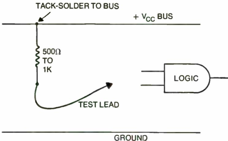
Fig. 13-10. When using the VCC voltage to create an artificial test logic pulse, use a current-limiting resistor for protection of the logic as well as the VCC bus.
