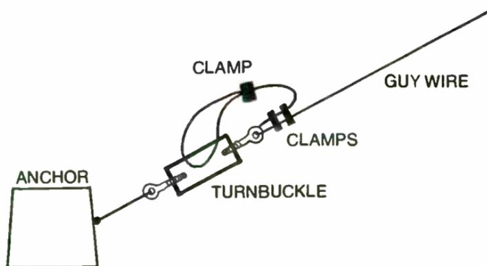
Fig. 11-11. Use a scrap of guy wire or the end of the guy to loop through the turnbuckle to keep it from turning.
