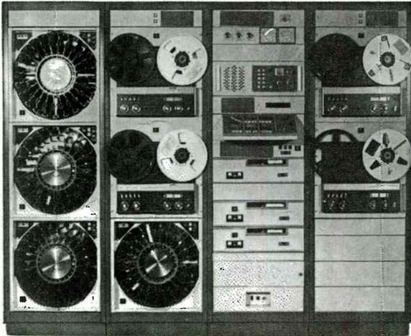
Fig. 1-5. Program automation systems increase the station's complexity and maintenance. Shown is a major program system by Systems Marketing Corp. (Model 3060), using a sequential programmer.
