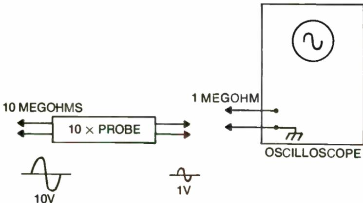
Fig. 13-3. A 10X probe on oscilloscope will provide circuit isolation, but also reduces signal amplitude to instrument.
