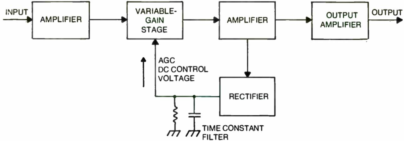
Fig. 9-5. The basic AGC amplifier. The only difference between an AGC amplifier and a peak limiter is the time constant on the control bus.
