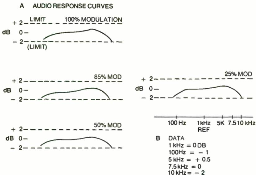
Fig. 14-3. A graph (A) is more expressive of results than a vertical row of figures. (B) Plot similar results on the same sheet.
