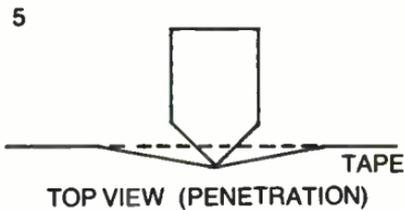
Fig. 5-16. The five conditions of head positioning which must be met in head alignment.
