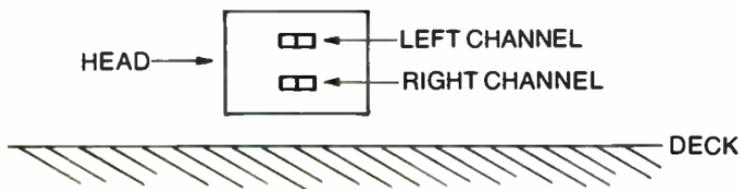
Fig. 6-5. Tape track identification on the heads.
