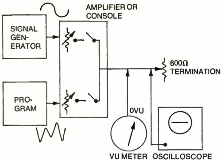
1. CALIBRATE METER & SCOPE WITH SINE WAVE
