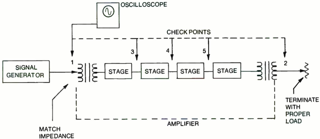
Fig. 2-11. Signal tracing. Measure the input first, then the output, then stage to stage.
