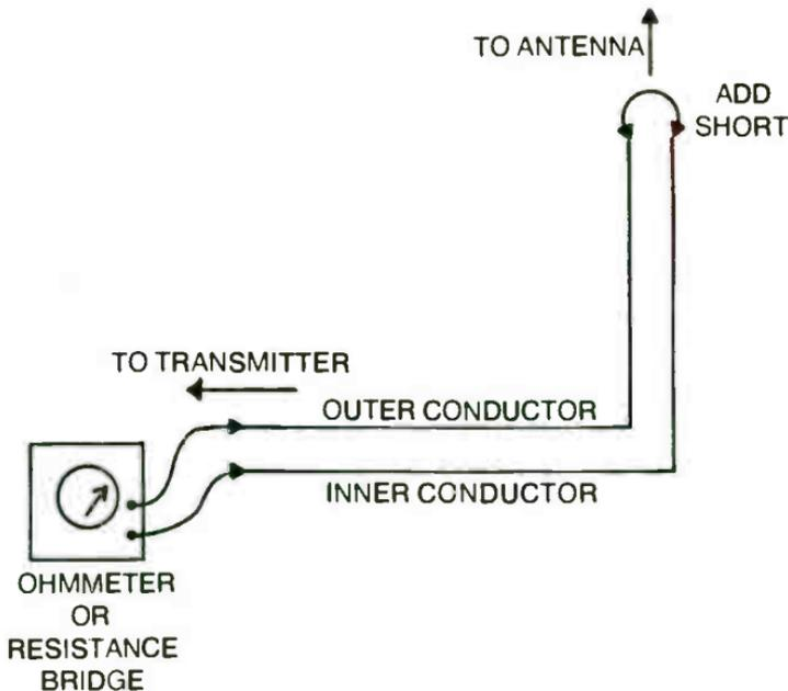
Fig. 10-10. Check line for continuity with an ohmmeter or resistance bridge.
