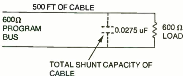
CABLE CAPACITY  $55 \text{ pF/FOOT} \times 500 \text{ FT} = 0.0275 \mu\text{F}$
