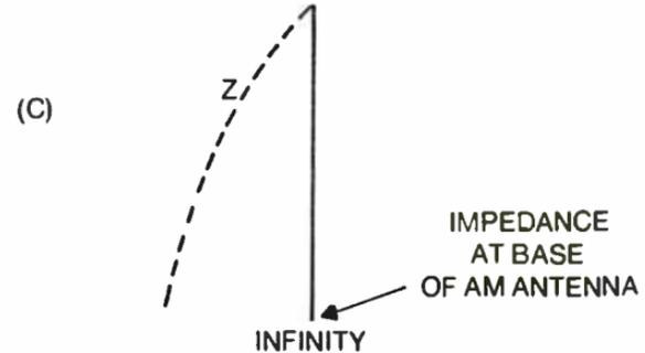
Fig. 11-4. Isolation techniques. (A) Crossing the base insulator of the AM tower with AC power requires isolation. Shown here is the Austin ring-type transformer. Also shown are lightning ball gaps. (B) Isolate FM coax line from the AM tower base with a quarter-wave tuned section. (C) The quarter-wave section presents infinite impedance to the AM carrier. (Photo courtesy Harris Corporation.)
