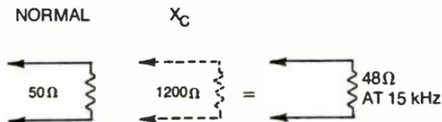
Fig. 4-26. Figure the value of the reactance of the bypass at both the offending frequency and at the highest audio frequency.
