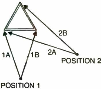
Fig. 12-9. Transit should be set up at two different positions 90 degrees apart. On a triangular tower, this may be less than 90 degrees. Check opposite legs of tower in each position.
