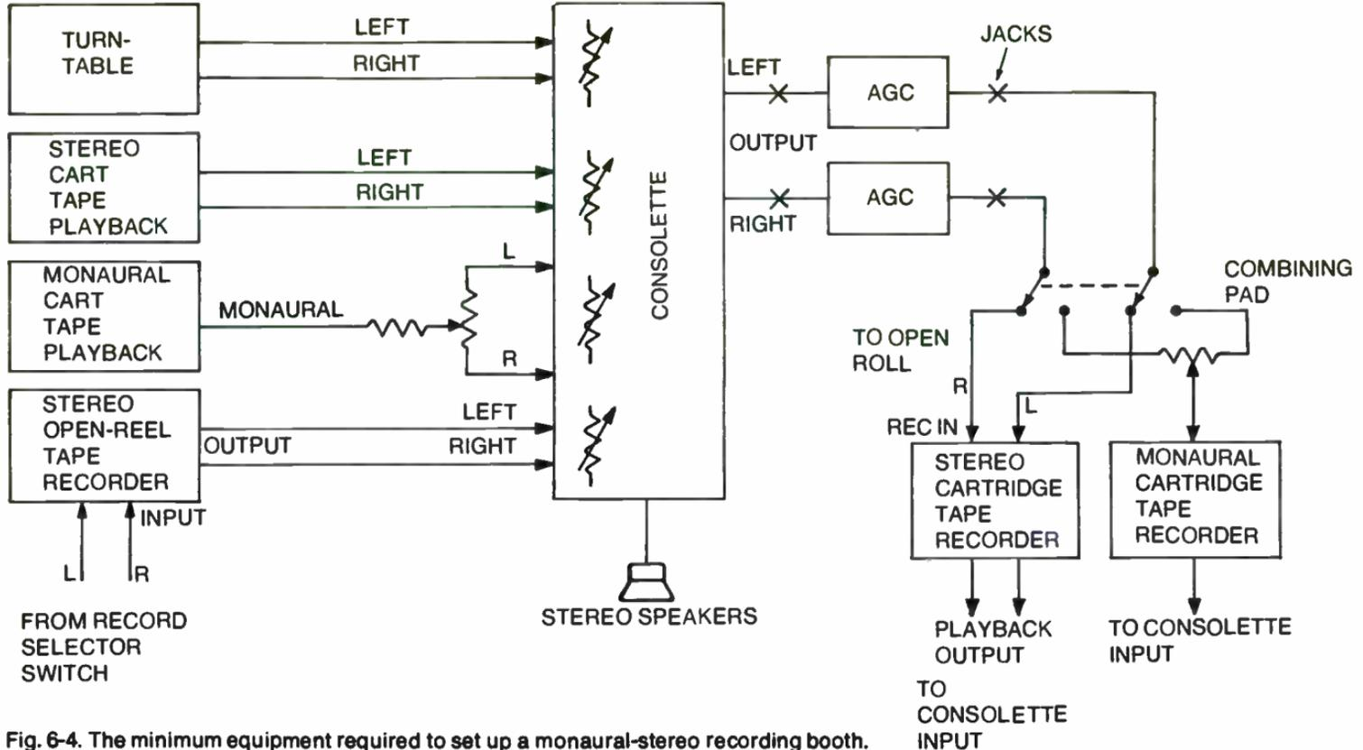
Fig. 6-4. The minimum equipment required to set up a monaural-stereo recording booth.
