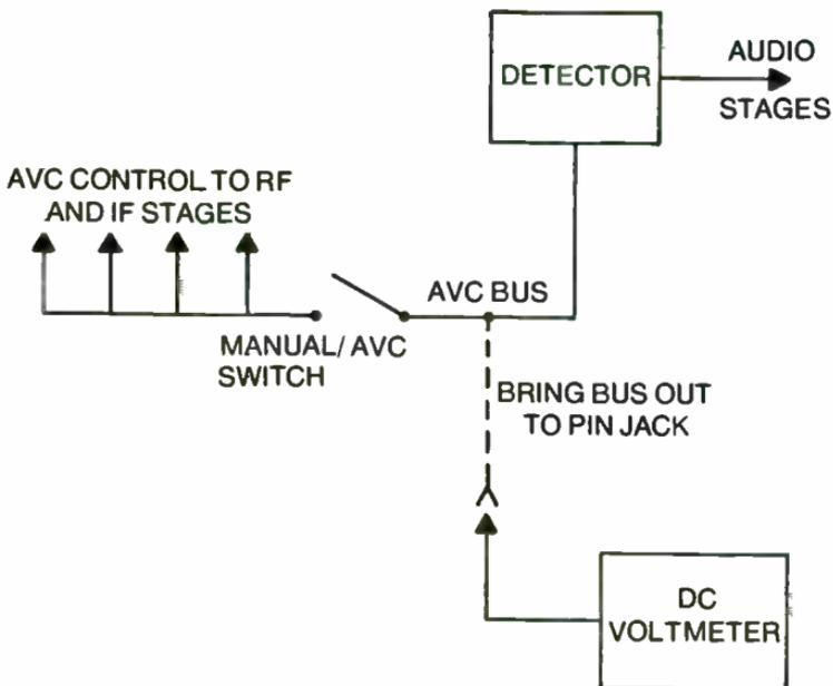
Fig. 14-11. Modify the receiver so that AVC bus can be measured.
