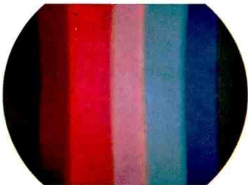
PLATE IV. Color bars with the brightness component (*Y*) missing. (RCA.)
