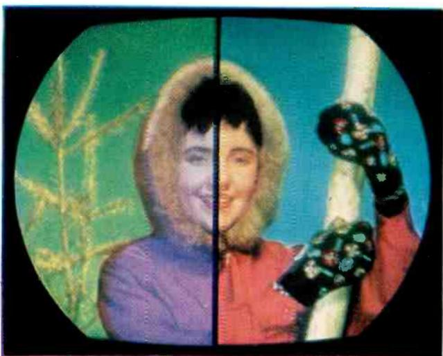
*(Above) luminance and chrominance components displayed separately; (below) complete lack of  $I'$  signal on left of picture and complete lack of  $Q'$  signal on right of picture*
