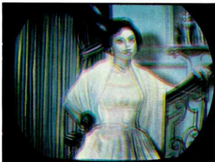
*Receiver image misregistration; (above) effect caused by excessive delay in receiver luminance channel; (below) effect on black-and-white picture reproduced on a shadow mask tube with static convergence grossly out of adjustment*
