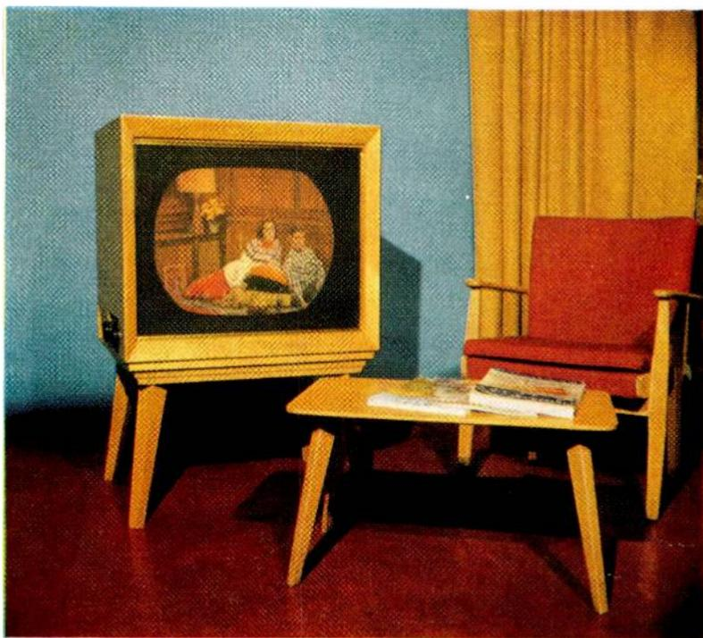
*A typical complete 21-inch shadow mask receiver of a type which could go into production. This type of receiver will accept either N.T.S.C. colour transmissions or monochrome signals*
