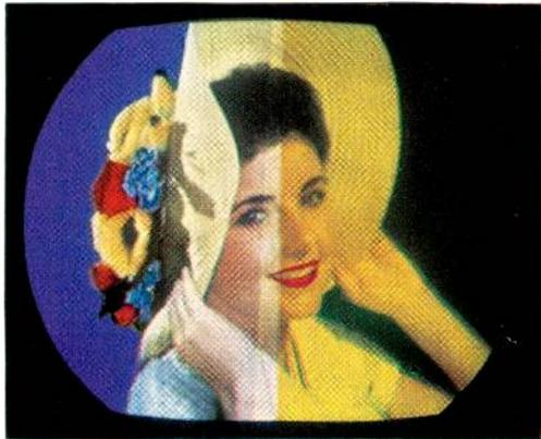
*Effect of removing each primary colour from a correctly balanced picture; (above) red absent from picture; (centre) green absent from picture; (below) blue absent from picture*
