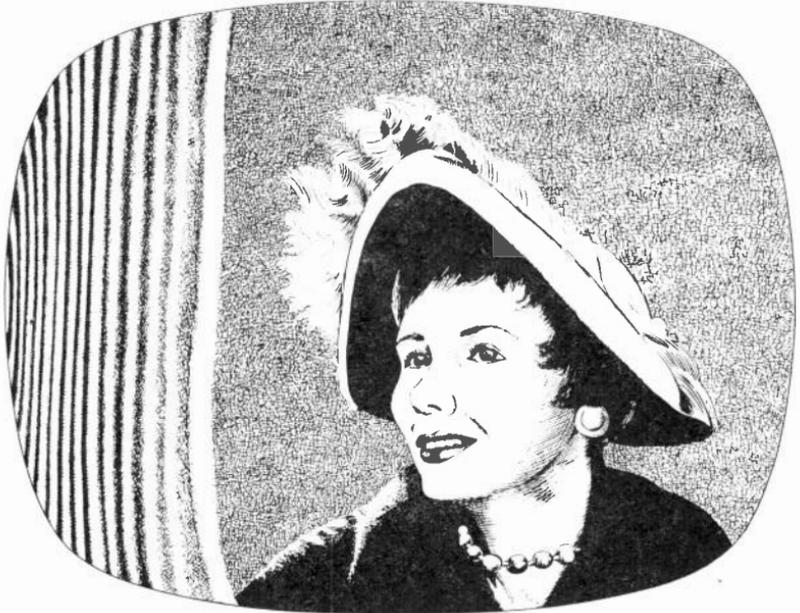
*Fig. 15.4. Display of colour burst on a monochrome receiver. The effect has been emphasized for clarity*
