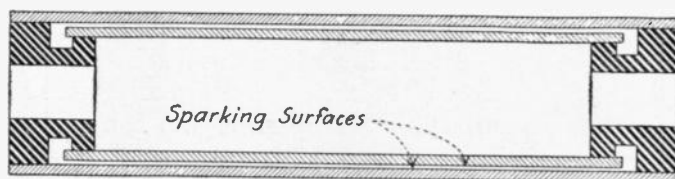
Fig. 30.—A Sectional View of the Lowenstien Type Quenched Spark Gap.
